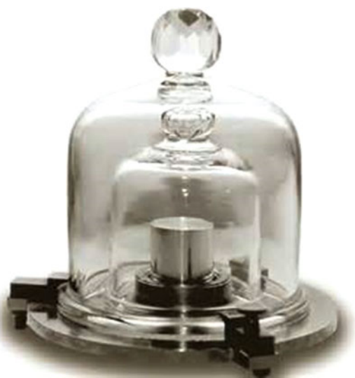
Figure 1.27 Standard kilogram of platinum-iridium, kept under vacuum in Paris ( https://en.wikipedia.org/wiki/Kilogram#International_prototype_kilogram )
