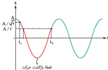
$$x = A \cos \omega t \Rightarrow \frac{A}{\sqrt{2}} = A \cos \omega t_2 \Rightarrow \cos \omega t_2 = \frac{1}{\sqrt{2}}$$
