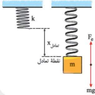
$$F_e = mg \Rightarrow kx = mg \Rightarrow k \times 0/1 = m \times 10 \Rightarrow k = m \times 100$$
