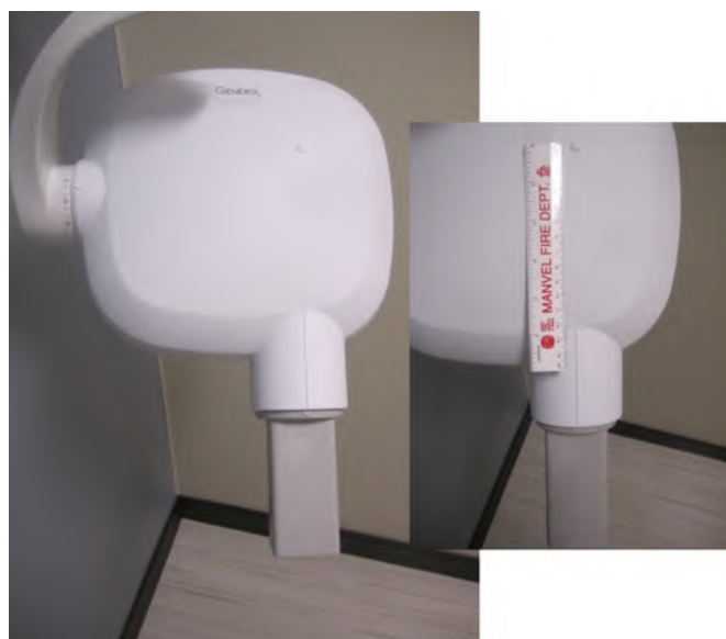
• Fig. 3.1 X-ray tube head with position dot indicating the position of the focal spot that is inside the x-ray tube head (red arrow). The inset image demonstrates the increased length of the focal distance. This increased length offers sharper image outlines and reduced patient dose.
