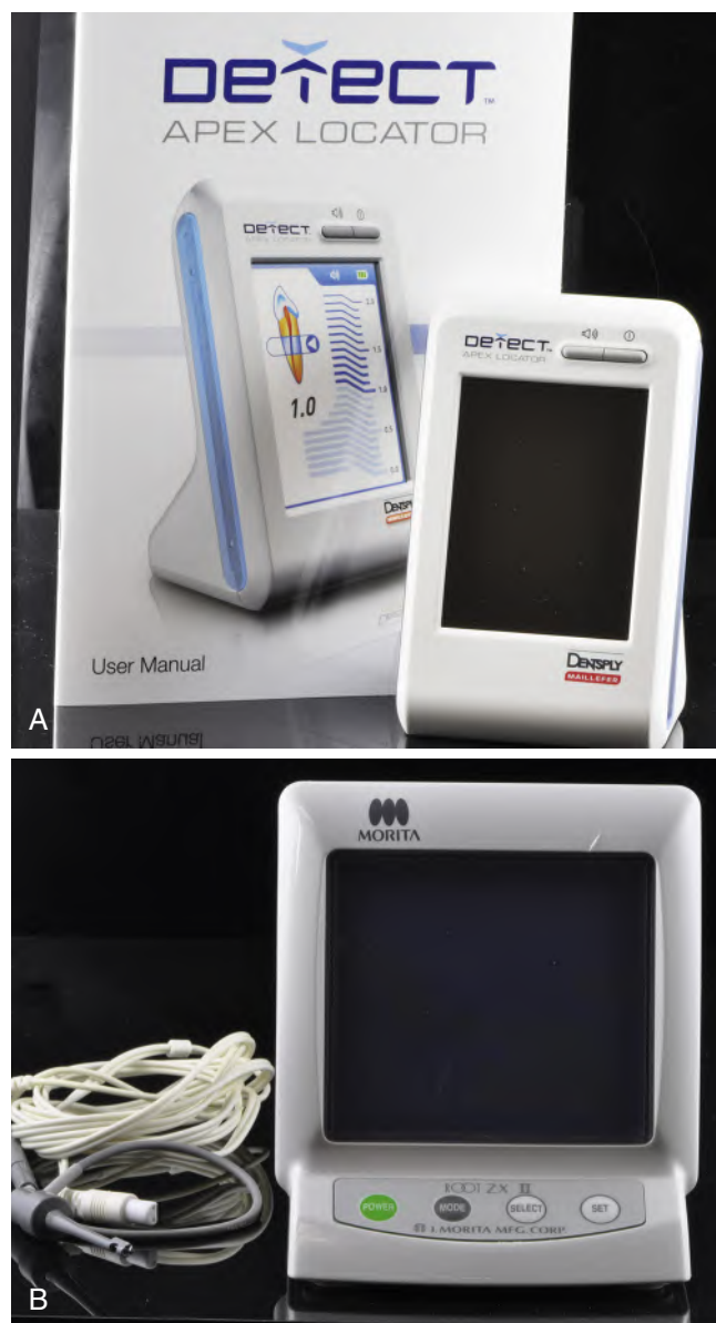
• Fig. 13.46 A and B, Two impedance apex locators.
