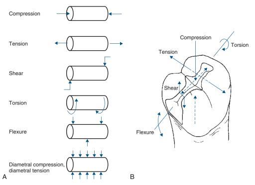
Online Fig. 18-10 Examples of directions of loading. A, Uniaxial loading of cylinder. B, Uniaxial loading of a mesio-occlusal amalgam restoration.
