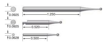
**Fig. 6-18** Characteristics and typical dimensions (in inches) of three common instrument shank designs for straight handpiece (*A*), latchangle handpiece (*B*), and friction-grip angle handpiece type (*C*).
