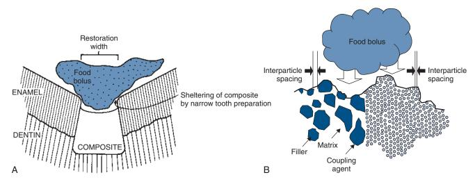
Online Fig. 18-81 Protection theory of contact-free area (CFA) wear. A, Macroprotection of composite by sheltering effect of narrow tooth preparation. B, Microprotection of matrix resin from small abrasive particles in a food bolus is created by close interparticle spacing of filler particles. Interparticle spacing is reduced from midifill composites (left) to minifill composites (right). (Adapted from Bayne SC, et al: Protection hypothesis for composite wear, Dent Mater 8:305–309, 1992.)
