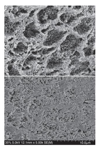
**Fig. 4-6 A,** Scanning electron micrograph of enamel etched with 35% phosphoric acid for 15 seconds, denoting a type I etching pattern. **B,** Scanning electron micrograph of enamel etched with 35% phosphoric acid for 15 seconds, denoting a type III etching pattern.
