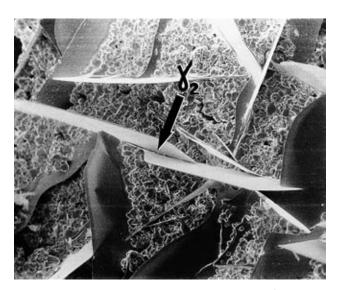
Online Fig. 18-28 Scanning electron microscopy view of tin–mercury (Sn-Hg) (g2) crystals that occur in a matrix of set low-copper amalgams. Note the blade-like crystals that penetrate amalgam and touch each other to create a continuous matrix (arrow). (Courtesy of D.F. Taylor, School of Dentistry, University of North Carolina, Chapel Hill, NC.)
