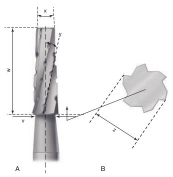
**Fig. 6-21** Design features of bur heads (illustrated using No. 701 bur). **A,** Lateral view—neck diameter (*v*), head length (*w*), taper angle (*x*), and spiral angle (*y*). **B,** End view—head diameter (*z*).
