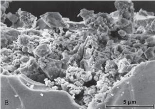
**Fig. 4-26** Scanning electron micrograph of Vita (Vita/Vident) dental ceramic etched with 9.6% hydrofluoric acid for 2 minutes. **A,** Top view. **B,** Lateral view.
