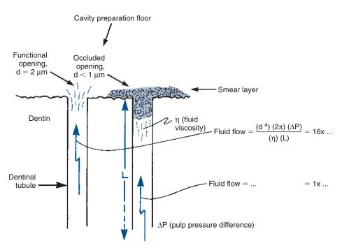
Online Fig. 18-47 Schematic view of fluid flow physics for dentinal tubules. The flow rate is a function of tubule diameter (d), pulpal pressure difference ( $\Delta P$ ) to ambient pressure, viscosity of dentinal fluid ( $\eta$ ), and tubule length (L). A twofold reduction in opening diameter results in a 16-fold reduction in fluid flow.
