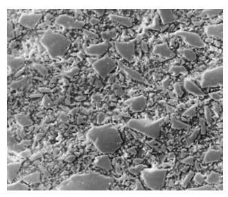
Fig. 8-2 Scanning electron micrograph of polished surface of a conventional composite (×300).
