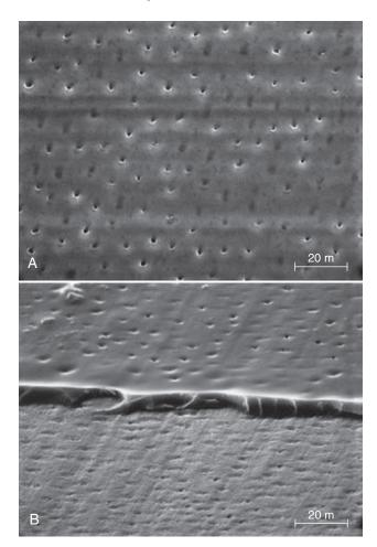
Online Fig. 18-48 Copalite varnish partially occluding the dentinal tubules. A, Scanning electron microscopy of one layer of Copalite varnish over the smear layer that seals approximately 55% of the tubules. B, Scanning electron microscopy of two layers of Copalite varnish adjacent to region protected only by the smear layer. (Courtesy of S.C. Bayne, School of Dentistry, University of Michigan, Ann Arbor, MI.)
