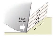
**Fig. 6-25** Schematic representation of bur blade (*end view*) cutting a ductile material by shearing mechanism. Energy is required to deform the material removed and produce new surface.
