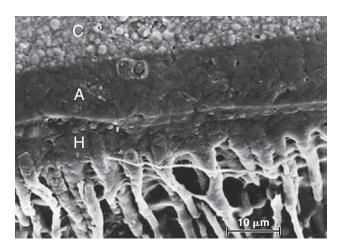
Fig. 4-15 Scanning electron micrograph of the transition between composite resin (*C*)–adhesive (*A*), adhesive–hybrid layer (*H*), and hybrid layer–dentin.
