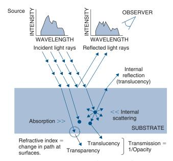
Online Fig. 18-7 Schematic summary of interactions of electromagnetic radiation with materials. The color perceived by the observer is the result of several interactions between substrate and incoming radiation producing reflection, internal scattering, absorption, fluorescence, and transmission.
