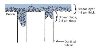
Online Fig. 18-46 Schematic view of the dentin smear layer.
