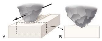
**Fig. 6-26** Schematic representation of an abrasive particle cutting ductile material. **A,** Lateral view. **B,** Cross-sectional view. Material is displaced laterally by passage of an abrasive particle, work hardened, and subsequently removed by other particles.
