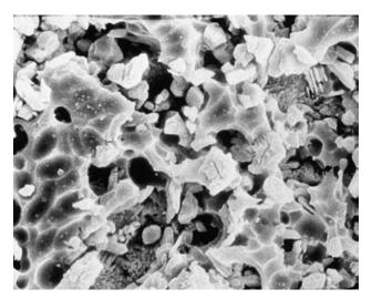
Fig. 12-38 Scanning electron micrograph (×31,000) of feldspathic porcelain etched with hydrofluoric acid. (Courtesy of Dr. Steven Bayne.)
