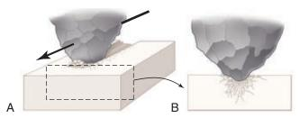
**Fig. 6-27** Schematic representation of abrasive particle cutting brittle material. **A,** Lateral view. **B,** Cross-sectional view. Subsurface cracks caused by the passage of abrasive particles intersect, undermining small pieces of material, which are removed easily by following abrasive particles.
