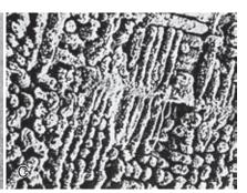
Online Fig. 21-9 Acid-etched, resin-bonded metal bridges. A, Rochette type. B, Maryland type. C, Scanning electron micrograph of etched metal surface. (Courtesy of Dr. John Sturdevant.)
