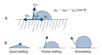
**Online Fig. 18-9** Interfacial interactions of materials. **A,** Interaction quantified as contact angle (see *formula*). **B,** Interaction described in terms of good wetting (spreading), partial (poor) wetting, or nonwetting.
