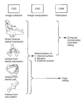
**Online Fig. 18-88** Schematic summary of computer-aided design/computer-aided manufacturing (CAD/CAM) and copy-milling operations.
