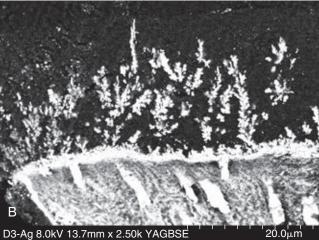
**Fig. 4-24** Nanoleakage under the electron microscope. **A,** Spotted pattern in the hybrid layer formed by a one-step self-etch adhesive under the transmission electron microscope (TEM). **B,** Reticular pattern and "water trees" in the adhesive layer formed by a one-step self-etch adhesive under the scanning electron microscope (SEM) in backscattered mode.
