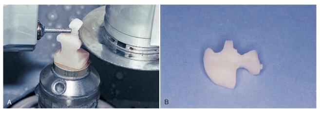
Fig. 11-14 A, Ceramic onlay being milled. B, Milled onlay.
