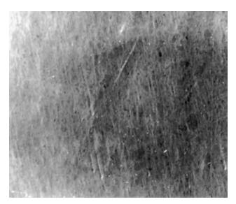
Fig. 8-3 Scanning electron micrograph of polished surface of a microfill composite (x300).
