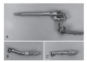
**Online Fig. 23-9** Conventional designs of handpieces. **A**, Belt-driven straight handpiece. **B**, Gear-driven angle handpiece that attaches to front end of the straight handpiece. **C**, Gear-driven angle handpiece designed for cleaning and polishing procedures.
