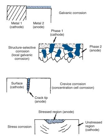
Online Fig. 18-15 Types of electrochemical cells. Dotted regions indicate anodic material being lost during corrosion. (From Tomashov ND: Theory of corrosion and protection of metals, ed 1, New York, 1966, Macmillan.)
