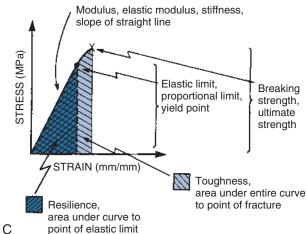
Online Fig. 18-11 Schematic summary of mechanical properties with respect to amalgam restoration in function. A, Occlusal loading of Class I amalgam restoration. B, Load or deformation curve describing the behavior of amalgam. C, Normalization of load or deformation curve to stress—strain curve with the important characteristics of curve indicated. (Mechanical responses depend on temperature and strain rate involved.)
