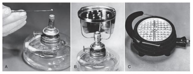
Online Fig. 22-4 A, Pellet of gold foil is degassed in pure ethanol flame. B, Mica tray mounted over alcohol lamp for degassing several increments of gold simultaneously. C, Gold foil degassed on an electric annealer. (Courtesy of Terkla and Cantwell.)
