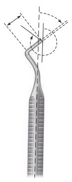
Fig. 6-3 Instrument shank and blade design (with primary cutting edge positioned close to handle axis to produce balance). The complete instrument formula (four numbers) is expressed as the blade width (1) in 0.1-mm increments, cutting edge angle (2) in centigrades, blade length (3) in millimeters, and blade angle (4) in degrees.
