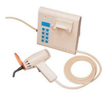
Online Fig. 18-71 Example of visible light–curing unit for use with composites, bonding agents, and other light-curing materials. The main power supply is connected to a pistol-grip light gun that generates a beam that is passed through the fiberoptic light guide. A shield is supplied to protect against direct observation of high-intensity light at the tip. Note: Always reference the manufacturer's directions for use for the curing unit and composite. (Courtesy of Kerr Corp., Orange, CA.)
