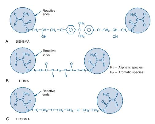
Online Fig. 18-63 Chemical formulas of di-functional monomers commonly used in composites. A, Bisphenylglycidyl dimethacrylate (BIS-GMA) monomer. B, Urethane dimethacrylate (UDMA) monomer. C, Triethylene glycol dimethacrylate (TEGDMA) monomer. (Courtesy of S.C. Bayne, School of Dentistry, University of Michigan, Ann Arbor, MI.)
