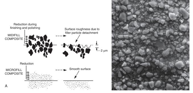
Online Fig. 18-65 Schematic summary of the microscopic events during finishing and polishing operations. A, Schematic illustration of effect of abrasive particle size on surface finishing of midifill versus microfill composite surfaces. B, Scanning electron microscopy view of coarsely finished midifill composite surface. (Courtesy of S.C. Bayne, School of Dentistry, University of Michigan, Ann Arbor, Ml.)
