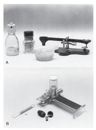
**Online Fig. 18-22** Earlier methods of dental trituration. **A,** Equipment for hand mixing of alloy powder and mercury in mortar and pestle using excess mercury (circa 1900–1940). **B,** Equipment for mixing of alloy pellets and controlled mercury in reusable capsules with mechanical mixing in amalgamator (circa 1940–1970).
