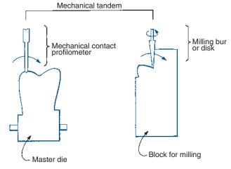
Online Fig. 18-87 Schematic representation of copy-milling.
