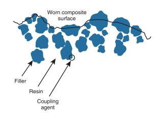
Online Fig. 18-80 Schematic view of wear of composite restoration. (From Bayne SC, et al: Protection hypothesis for composite wear, Dent Mater 8:305–309, 1992.)
