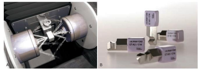
Fig. 11-8 A, Computer-driven software controls small, diamond-coated milling devices that mill the restoration out of a block of high-quality ceramic (as shown in B). (Courtesy of D4D Technologies, LLC, Richardson, TX.)
