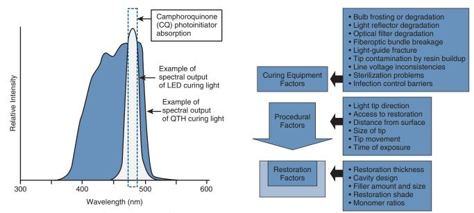
Online Fig. 18-73 Example of spectral output of quartz—tungsten—halogen (QTH) versus light-emitting diode (LED) light-curing units compared with absorption range for camphoroquinone photo-initiator, which is used in most light-cured bonding agents and composites. Unabsorbed light is converted principally into heat energy. (Courtesy of S.C. Bayne, School of Dentistry, University of Michigan, Ann Arbor, MI.)
