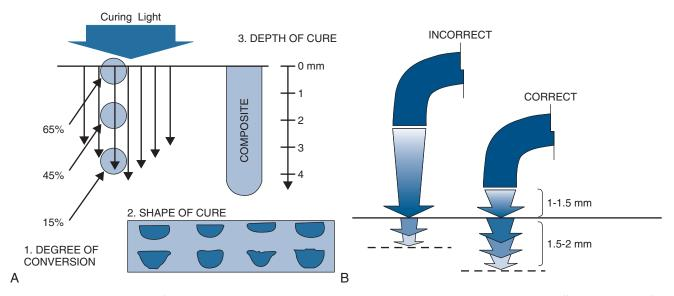
Online Fig. 18-76 Light intensity influences on the polymerization zone. **A,** Varying light intensity with width and depth affects the degree of conversion of monomer to polymer, shape of cure, and depth of cure. **B,** Proximity of curing light to the surface affects the depth of penetration of light into the surface.
