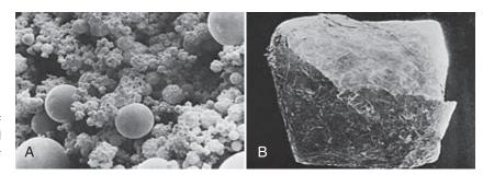
Online Fig. 22-3 Scanning electron micrographs of direct-filling golds. A, Spheres of E-Z Gold. B, Wrapped E-Z pellet that contains spheres. (Courtesy of Ivoclar-Williams Company, Inc., Amherst, NY.)
