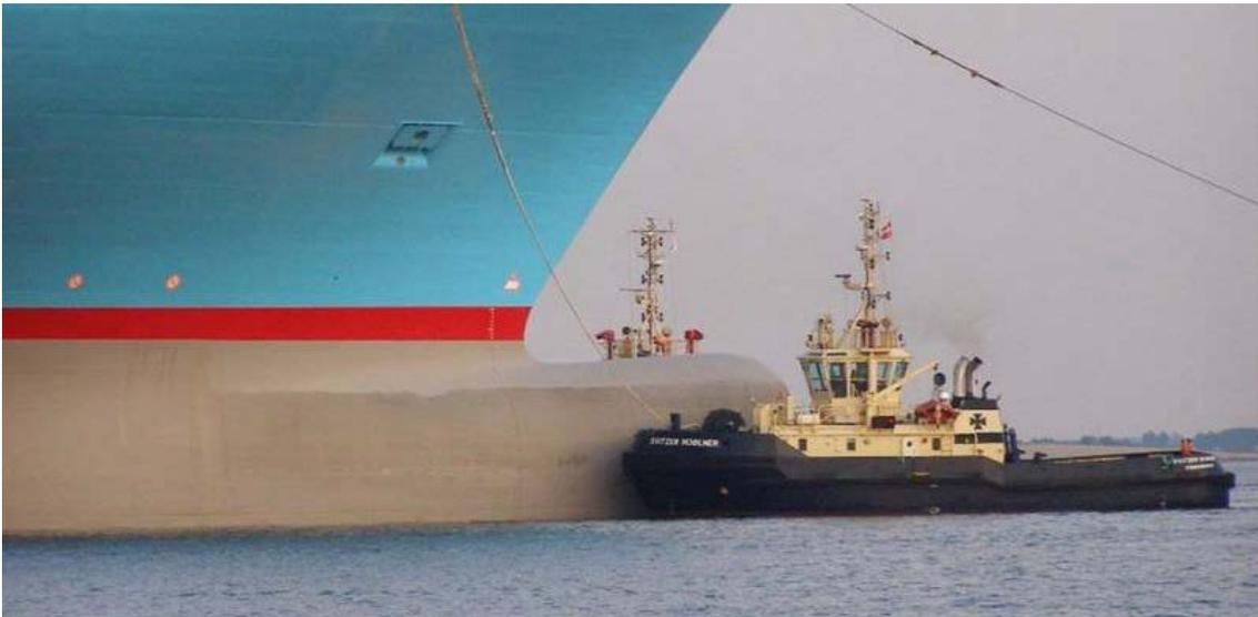
This container-ship is under construction and not loaded. The red line is the water line under normal load.
