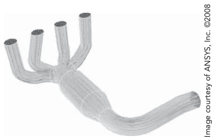
Fig. 5.11 Flow through a catalytic converter.
