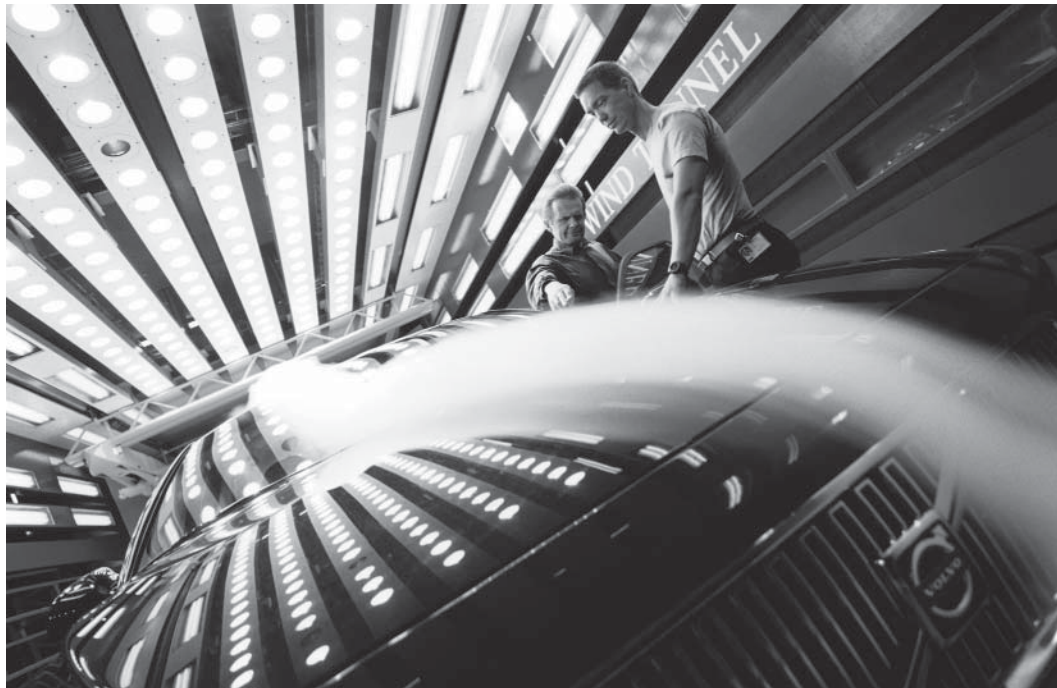
Fig. 7.4 Full-scale automobile under test in Volvo wind tunnel, using smoke streaklines for flow visualization.
