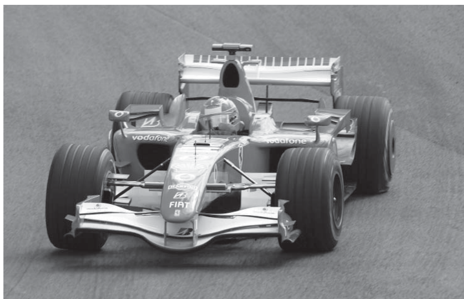
Fig. 9.26 Contemporary racing car showing aerodynamic features. The car's front and rear wings are designed to provide significant downforce at speed to improve traction. Also visible are fairings to direct hot air from the radiators around the rear tires, and at the front of the car, cool air toward the brakes. Not shown are other aerodynamic features such as the fuselage bottom, which is designed to route the airflow carefully, using diffusers, to develop the most negative pressure, and to cause this negative pressure to act over the largest possible area under the car, to develop additional downforce.
