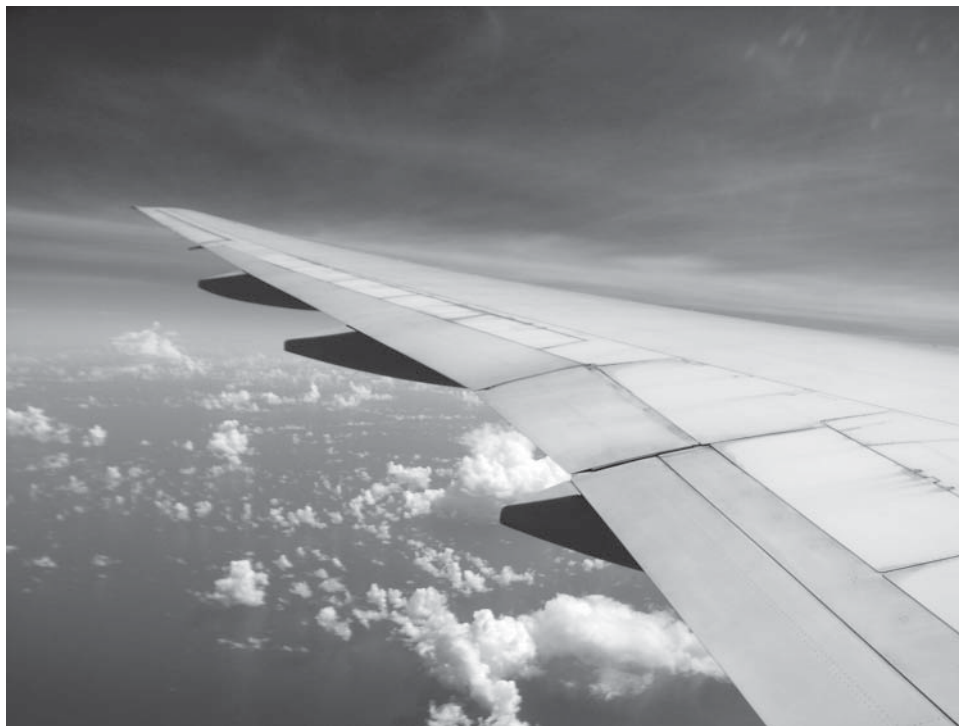
Fig. 9.24 (b) Application of high-lift boundary-layer control devices to reduce takeoff speed of a jet transport aircraft. This is another view of the Boeing 777 wing. In the takeoff configuration, large slotted trailing-edge flaps deflect to increase the lift coefficient. The low-speed aileron near the wingtip also deflects to improve span loading during takeoff. This view also shows the single-slotted outboard flap, the high-speed aileron, and nearest the fuselage, the double-slotted inboard flap.
