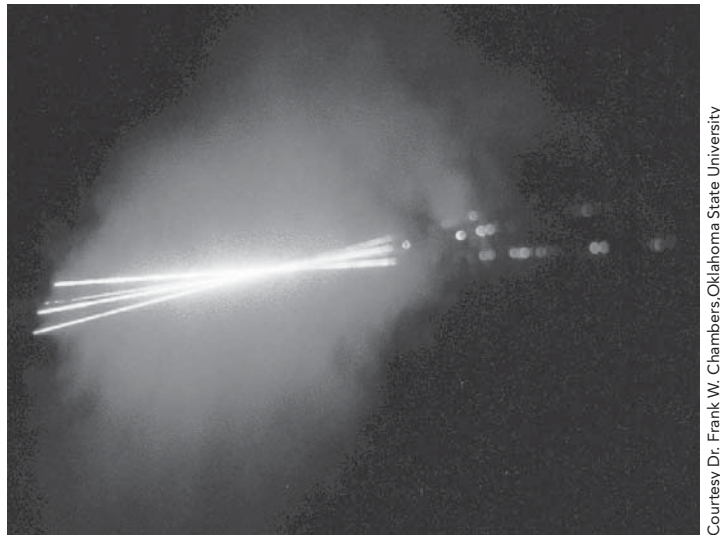
Fig. 8.26 A 2-component Laser Doppler Anemometer Probe Volume.
