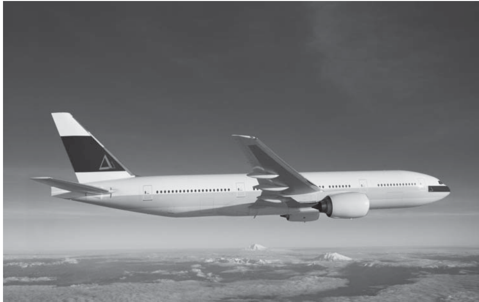
Fig. 9.24 (a) Application of high-lift boundary-layer control devices to reduce landing speed of a jet transport aircraft. The wing of the Boeing 777 is highly mechanized. In the landing configuration, large slotted trailing-edge flaps roll out from under the wing and deflect downward to increase wing area and camber, thus increasing the lift coefficient. Slats at the leading edge of the wing move forward and down, to increase the effective radius of the leading edge and prevent flow separation, and to open a slot that helps keep air flow attached to the wing's upper surface. After touchdown, spoilers (not shown in use) are raised in front of each flap to decrease lift and ensure that the plane remains on the ground, despite use of the lift-augmenting devices. (This photograph was taken during a flight test. Flow cones are attached to the flaps and ailerons to identify regions of separated flow on these surfaces.)
