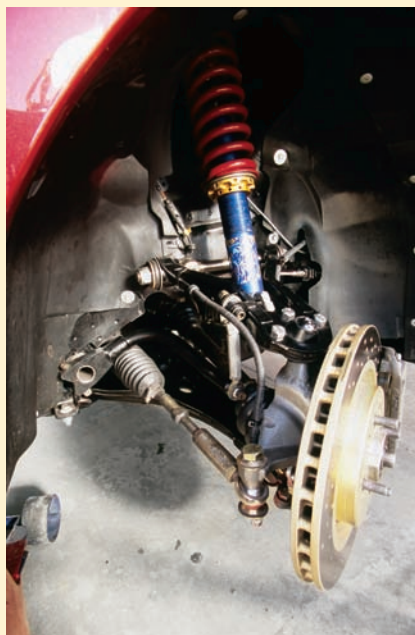
■ FIGURE 9.32 Typical automotive suspension system. © Transtock Inc./Alamy.
