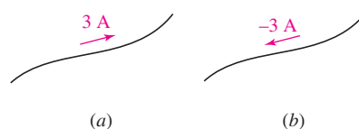
■ FIGURE 2.5 Two methods of representation for the exact same current.
