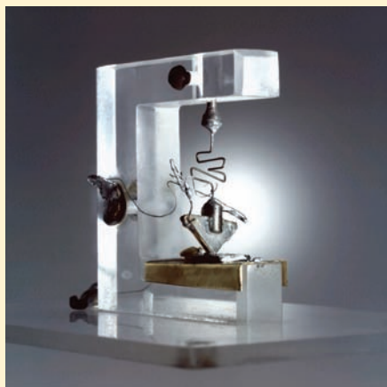
■ FIGURE 17.27 Photograph of the first demonstrated bipolar junction transistor ("bjt").
