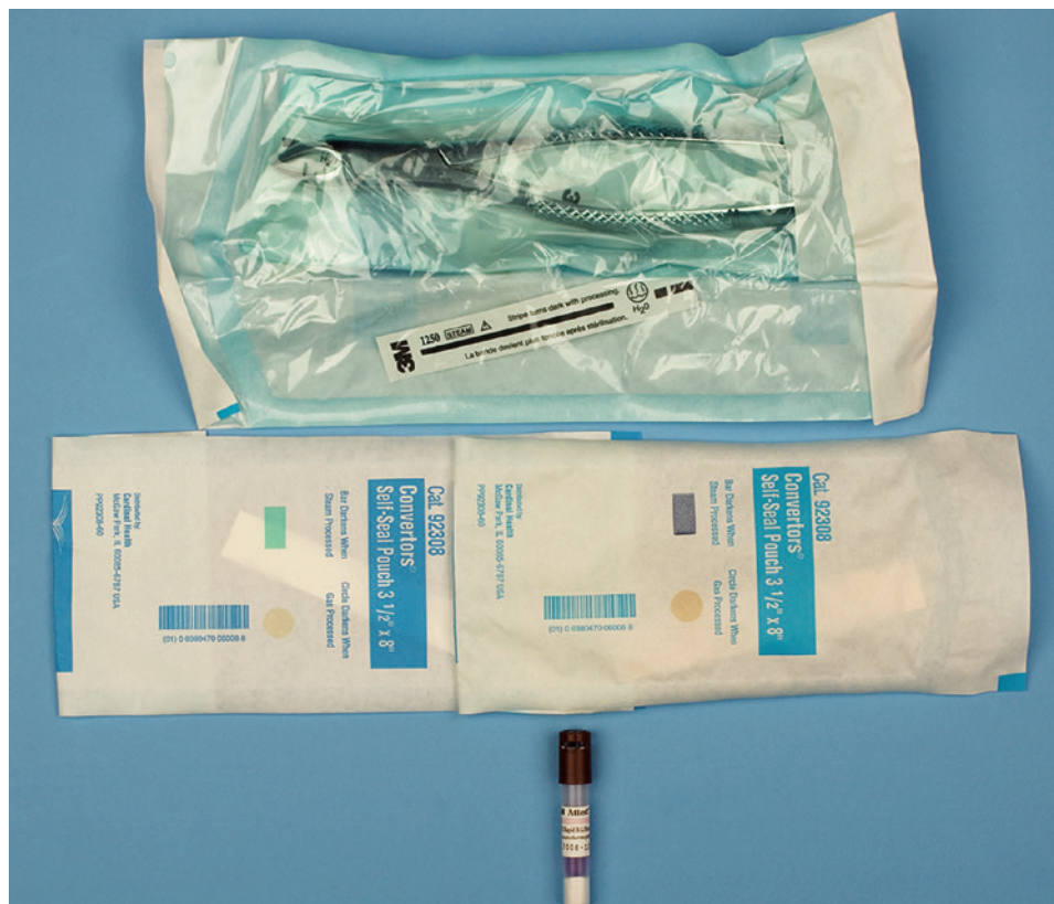
• Fig. 5.1 Tests of sterilization equipment. Color-coded packaging is made of paper and cellophane; test areas on package change color on exposure to sterilizing temperatures or to ethylene oxide gas (top and center). Vial contains spores of Bacillus stearothermophilus , which is used for testing efficiency of heat sterilization equipment (bottom).
