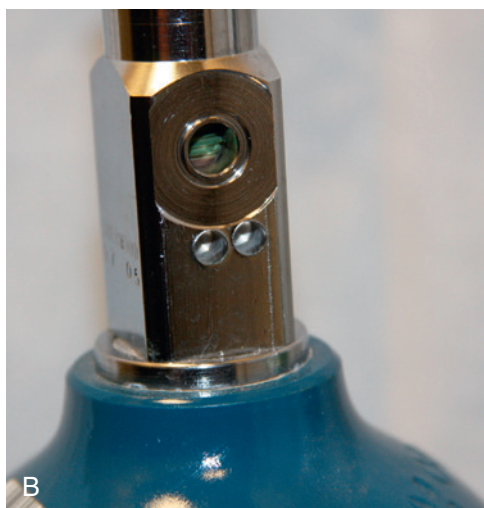
• Fig. 6.21 Pin index system is used to prevent attaching the wrong gas to the wrong port of the continuous-flow sedation unit/controller. Note the differing patterns of depression below the gas exit port for (A) oxygen and (B) nitrous oxide.
