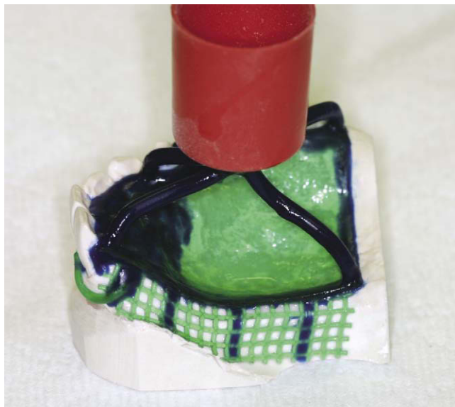
FIGURE 18-24 For a maxillary framework, multiple 8-gauge sprues or a single main sprue located posteriorly can be used. When a single main sprue is used, additional sprues can feed critical regions for casting completeness.
