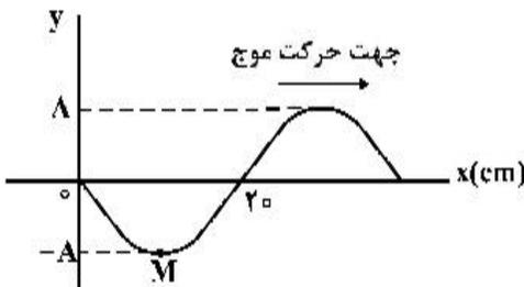
$$\frac{\lambda}{2} = 20(\text{cm}) \Rightarrow \lambda = 40(\text{cm}) = 0.4(\text{m}), v = 2 \frac{\text{m}}{\text{s}}, v = \lambda f \Rightarrow f = 5(\text{Hz}) \Rightarrow T = \frac{1}{f} = 0.2(\text{s})$$
