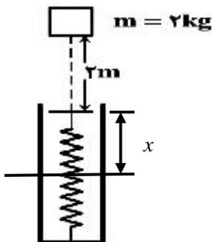
$$E_1 = E_2 \Rightarrow \frac{1}{2}mv_1^2 + mgh_1 = U_{\text{max-spring}}$$
