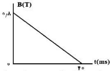
$$\bar{\varepsilon} = -N \frac{\Delta\Phi}{\Delta t} = -N \frac{\Delta(BA)}{\Delta t} = -NA \frac{\Delta B}{\Delta t} = -500 \times (40 \times 10^{-4}) \times \left( \frac{-0.8}{40 \times 10^{-3}} \right) = 40(\text{V})$$
