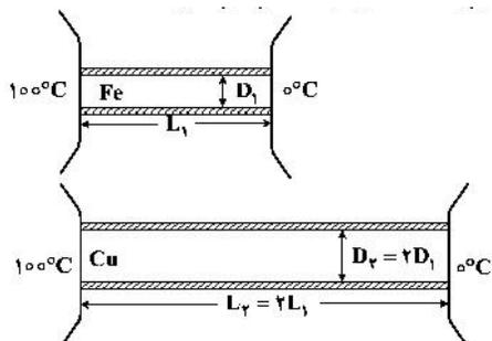
$$H_{Fe} = K \frac{A \times \Delta T}{L} = 80 \left( \frac{\pi \left(\frac{D_1}{2}\right)^2 \times 100}{L_1} \right) = 40 \left( \frac{\pi \times D_1^2 \times 100}{2L_1} \right)$$
