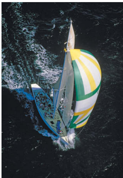
The designers of high-performance sailboats must consider both air-pressure distributions on the sails and water-pressure distributions on the hull.
