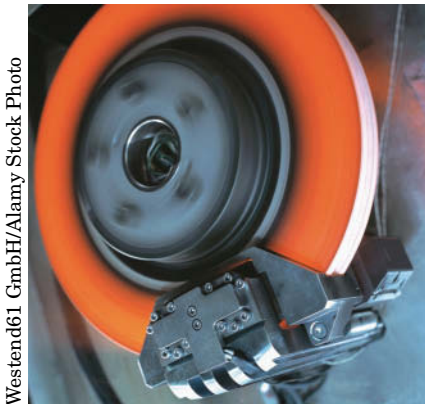
The change from mechanical energy to heat energy is evident in this view of a disk brake.
