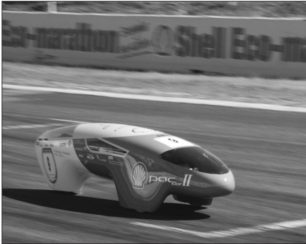
P7.109 The world's best mileage set by PAC-Car II of ETH Zurich. (Courtesy of Lino Guzzella, ETH Zurich, 2005)
