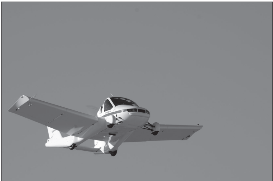
Fig. 7.30 The Transition ® car-plane in flight on March 23, 2012. It has a gross weight of 1,430 lbf and a cruise velocity of 105 mi/h. (Terrafugia, Inc.)
