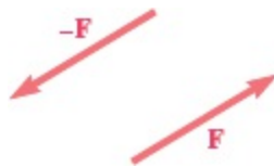
Fig. 3.25 A couple consists of two forces with equal magnitude, parallel lines of action, and opposite sense.
