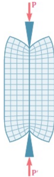
Fig. 9.45 Concentrated axial load applied to rubber model.
