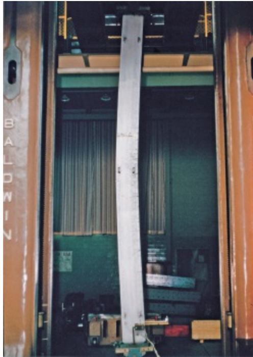
Photo 16.1 Laboratory test showing a buckled column.
