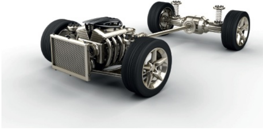
Photo 10.1 In this automotive power train, the shaft transmits power from the engine to the rear wheels.
