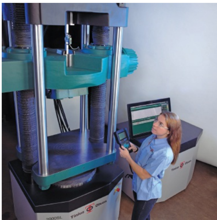
Photo 9.2 Universal test machine used to test tensile specimens.
