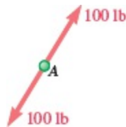
Fig. 2.22 When a particle is in equilibrium, the resultant of all forces acting on the particle is zero.
