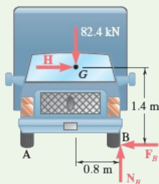
Fig. 1 Free-body diagram of truck.
