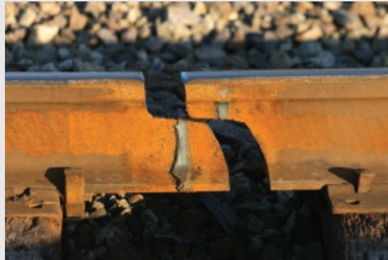
CS Photo 9.3 Rail that fractured due to low ambient temperature conditions.
