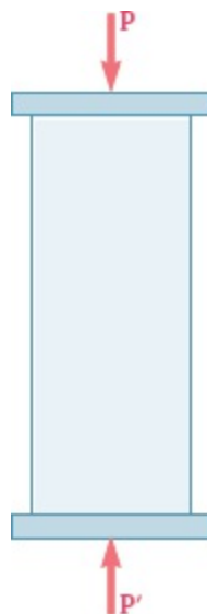
Fig. 9.43 Axial load applied by rigid plates.
