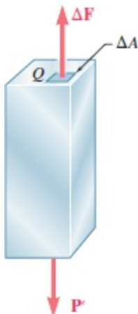
Fig. 8.2 Small area \Delta A , at an arbitrary point in the cross section, carries \Delta F in this axial member.
