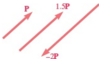
Fig. 2.9 Multiplying a vector by a scalar changes the vector's magnitude, but not its direction (unless the scalar is negative, in which case the direction is reversed).
