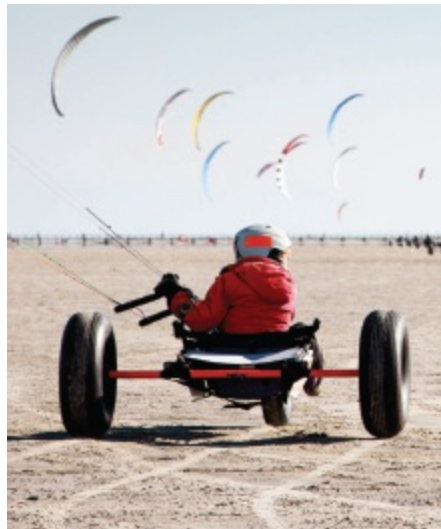
Photo 11.1 The center portion of the rear axle of the sport buggy is in pure bending.
