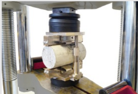
CS Photo 11.1 Split cylinder testing machine.
