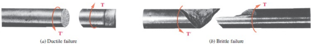
Photo 10.2 Shear failure of shaft subject to torque.
