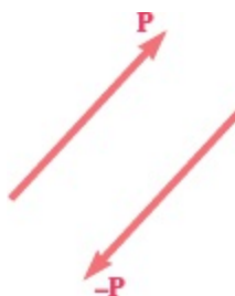
Fig. 2.4 The negative vector of a given vector has the same magnitude but the opposite direction of the given vector.
