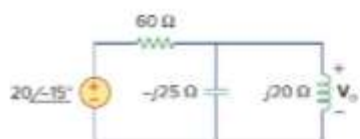
Figure 9.26 The frequency domain equivalent of the circuit in Fig. 9.25.
