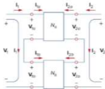
Figure 19.39 Series connection of two two-port networks.
