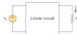
Figure 4.1 A linear circuit with input v_s and output i .
