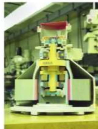
A three-dimensional printing of the output of an AutoCAD model of a NASA flywheel.
