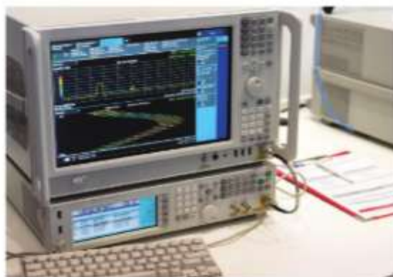
Figure 17.42 Modern analyzer of a signal and signal generator. Aleksey Dmetsov/Alamy Stock Photo
