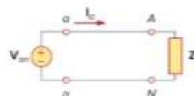
Figure 12.12 A single-phase equivalent circuit.
