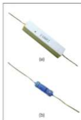
Figure 2.3 Fixed resistors: (a) wirewound type, (b) carbon film type. Mark Dierker/McGraw-Hill Education
