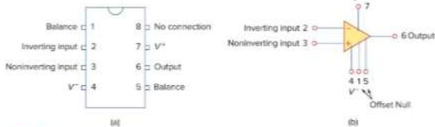
Figure 5.2 A typical op amp: (a) pin configuration, (b) circuit symbol.
