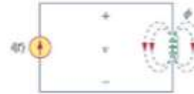
Figure 13.1 Magnetic flux produced by a single coil with N turns.
