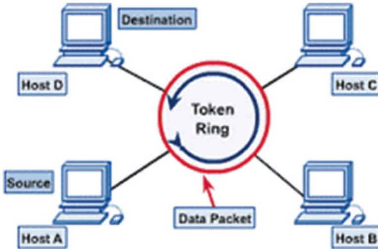
Fig. 4.4 Diagram of a token ring LAN. (Source: https://www.pinterest.com/pin/828662400161615931/ )
