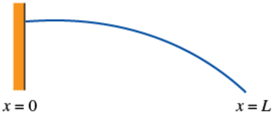
(b) Cantilever beam: embedded at the left end, free at the right end
