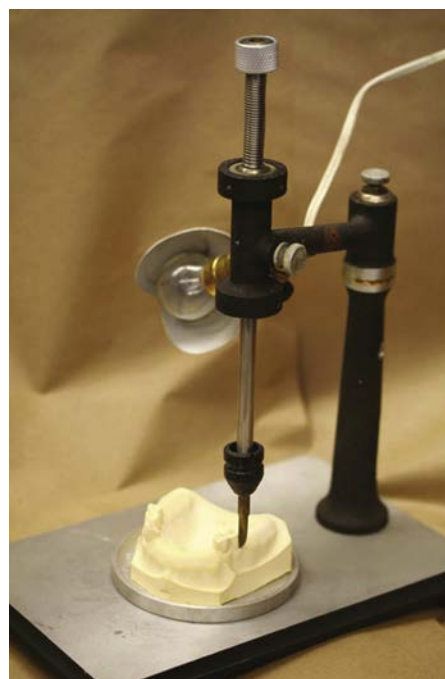
FIGURE 11-2 The Jelenko Surveyor. Note the spring-mounted paralleling tool and swivel at the top of the vertical arm. The horizontal arm may be fixed in any position by tightening the nut at the top of the vertical arm.
