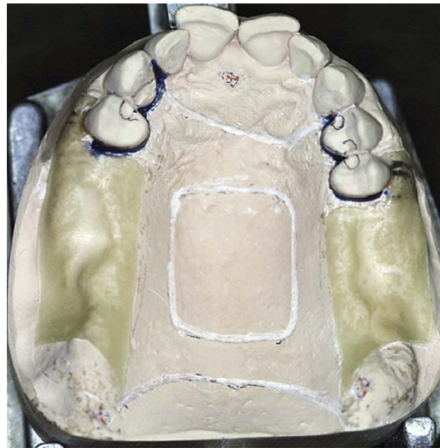
FIGURE 5-28 Framework design on master cast before preparation for duplication in refractory investment. A shallow groove (0.5 mm) has been scribed on the outline of anterior and posterior borders of the major connector. The anterior outline follows the valleys of rugae. Beading is readily accomplished with a cleoid carver. A slightly rounded groove is preferred to a V-shaped groove.
