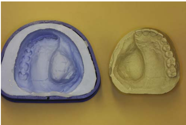
FIGURE 19-4 Refractory cast ( right ) following removal from the duplication mold ( left ). This cast incorporates all the features of the relieved and blockout master cast generated from the clinical framework impression.
