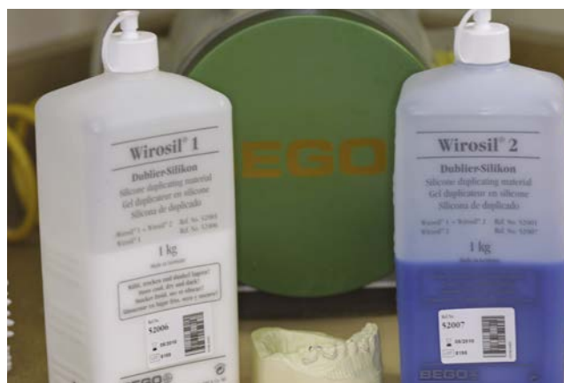
FIGURE 19-2 Duplicating material with a vacuum curing unit in the background, which is used to ensure a dense mold.
