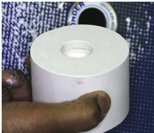
FIGURE 19-27 Investment mold has been trimmed to prepare the sprue end for burnout and subsequent complete adaptation to the casting machine.
