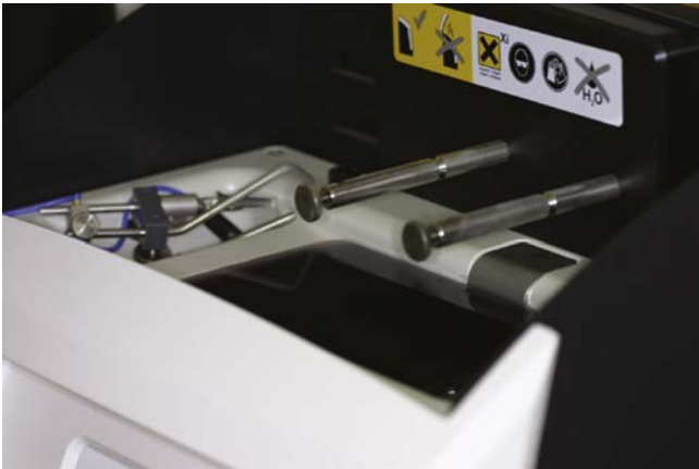
FIGURE 19-32 Electropolishing unit used for the final surface polish of frameworks in a heated polishing liquid.
