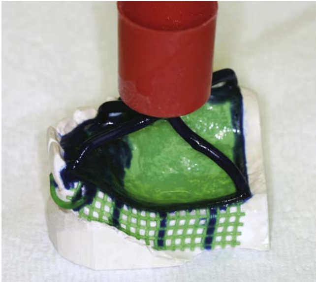
FIGURE 19-24 For a maxillary framework, multiple 8-gauge sprues or a single main sprue located posteriorly can be used. When a single main sprue is used, additional sprues can feed critical regions for casting completeness.
