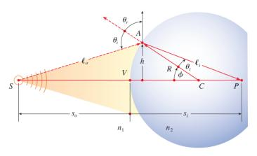
FIGURE 8 Refraction at a spherical interface
