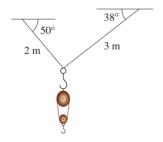
**36.** The tension vector at each end of a chain has magnitude 25 N (see the figure). What is the weight of the chain?
