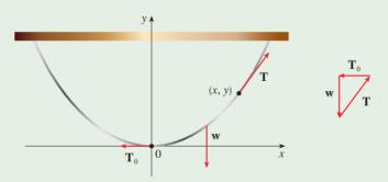
Consider the section of the chain from the origin to (x, y). The forces that act on the section are the downward gravitational force  $\mathbf{w}$  and the tensions  $\mathbf{T}_0$  and  $\mathbf{T}$  at each end of the section—each of which is tangent to the curve. Because the section of chain is in equilibrium, we know that
