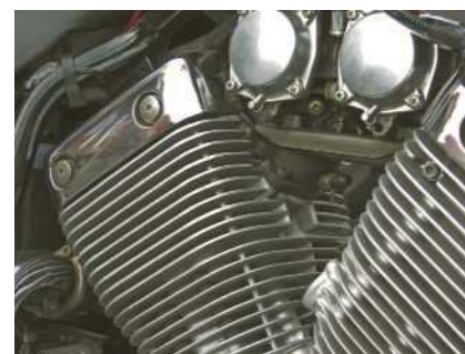
FIGURE 6.R.1 Cooling fins on a motorcycle engine
