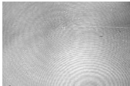
Figure 15: A waveform interference pattern that holds the information that transforms into a hologram.
