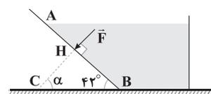
$$\Delta BHC: \alpha + 42^\circ + 90^\circ = 180^\circ \Rightarrow \alpha = 48^\circ$$
