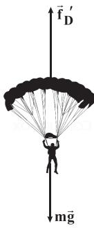
$$\begin{aligned} F_{\text{net}} &= ma' \Rightarrow mg - f'_D = ma' \\ &\Rightarrow mg - 16.00 = ma' \Rightarrow a' = g - \frac{16.00}{m} \end{aligned}$$
