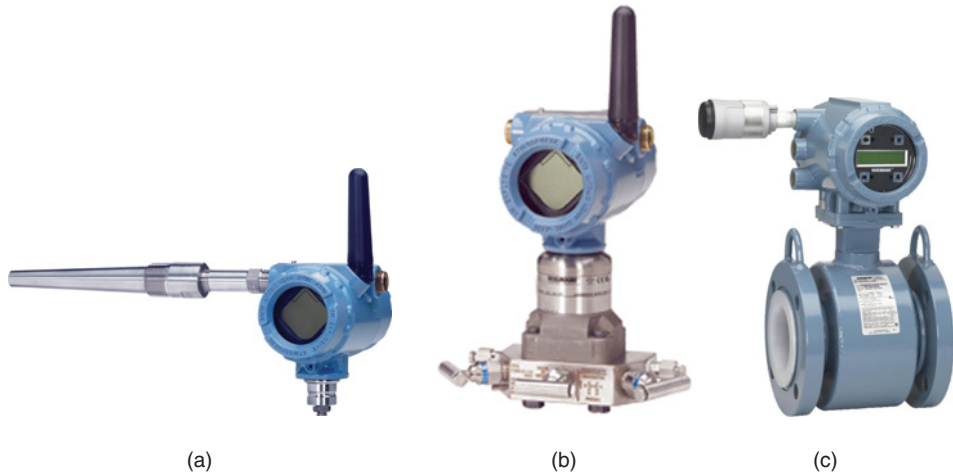
Figure C.13 Wireless field instruments: (a) wireless temperature transmitter assembled to RTD thermowell sensor; (b) wireless pressure transmitter assembled to integral coplanar manifold; (c) 8705 magnetic flowmeter with supplementary wireless antennae (THUM) for diagnostics (Reproduced with permission of Emerson Process Management).
