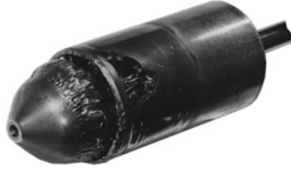
Figure 2.31 Typical appearance of flashing damage (Reproduced by permission of Emerson Process Management).
