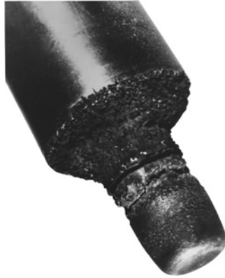
Figure 2.32 Typical appearance of cavitation damage (Reproduced by permission of Emerson Process Management).
