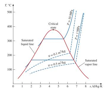
**FIGURE 7–11** Schematic of the *T-s* diagram for water.
