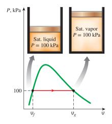
FIGURE 3–30 Schematic and *P-U* diagram for Example 3–3.
