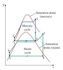
FIGURE 11–28 Mercury–water binary vapor cycle.
