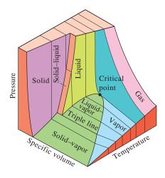
**FIGURE 3–23** *P-U-T* surface of a substance that *contracts* on freezing.
