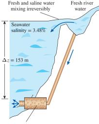
Fresh and saline water mixing reversibly through semipermeable membranes, and producing power.
