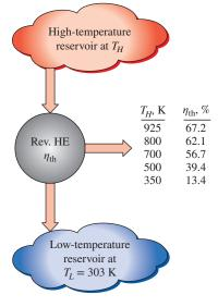
The fraction of heat that can be converted to work as a function of source temperature (for  $T_L = 303 \text{ K}$ ).
