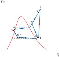
FIGURE 12-7 Schematic and T-s diagram for the actual vapor-compression refrigeration cycle.
