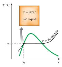
FIGURE 3–28 Schematic and *T-v* diagram for Example 3–1.
