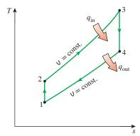
**FIGURE 10–16** *T-s* diagram of the ideal Otto cycle.
