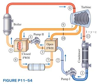
Reconsider Prob. 11–54. Using appropriate software, investigate the effects of turbine and pump efficiencies as they are varied from 70 percent to 100 percent on the mass flow rate and thermal efficiency. Plot the mass flow rate and the thermal efficiency as a function of turbine efficiency for pump efficiencies of 70, 85, and 100 percent, and discuss the results. Also plot the *T-s* diagram for turbine and pump efficiencies of 85 percent.
