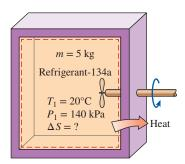
FIGURE 7–12 Schematic and *T-s* diagram for Example 7–3.
