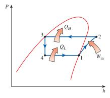
FIGURE 12-5 The P-h diagram of an ideal vaporcompression refrigeration cycle.
