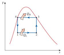
FIGURE 12–2 Schematic of a Carnot refrigerator and *T-s* diagram of the reversed Carnot cycle.
