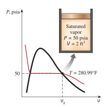
FIGURE 3–29 Schematic and *P-U* diagram for Example 3–2.
