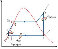
**FIGURE 11–2** The simple ideal Rankine cycle.
