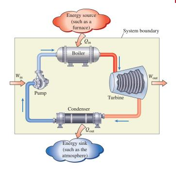
FIGURE 6–10 Schematic of a steam power plant.
