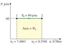
**FIGURE 4–7** Schematic and *P-U* diagram for Example 4–2.
