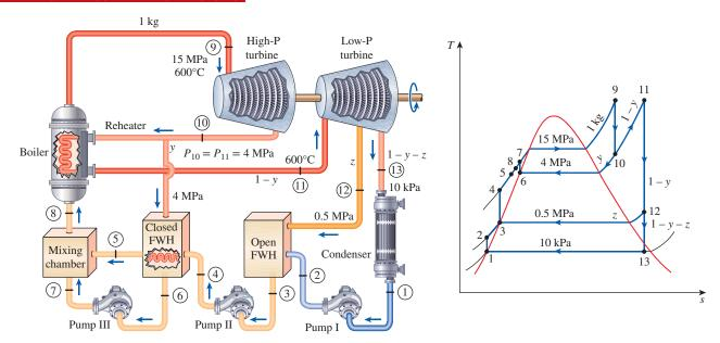
**FIGURE 11–20** Schematic and *T-s* diagram for Example 11–6.
