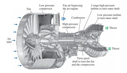
of sound. In a turbofan engine, the high-speed exhaust gases are mixed with the lower-speed air, which results in a considerable reduction in noise.
