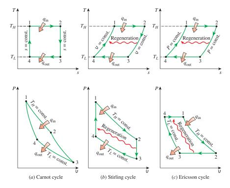
FIGURE 10–27 *T-s* and *P-v* diagrams of Carnot, Stirling, and Ericsson cycles.
