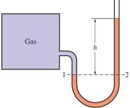
FIGURE 1-55 The basic manometer.
