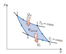
**FIGURE 6–37** *P-V* diagram of the Carnot cycle.
