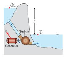
$\dot{W}_{\rm max} = \dot{m} \Delta e_{\rm mech} = \dot{m}g \ (z_1 - z_4) = \dot{m}gh$ since  $P_1 \approx P_4 = P_{\rm atm}$  and  $V_1 = V_4 \approx 0$ (a)
