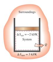
$S_{\text{gen}} = \Delta S_{\text{total}} = \Delta S_{\text{sys}} + \Delta S_{\text{surr}} = 1 \text{ kJ/K}$
