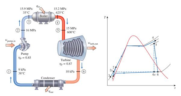
**FIGURE 11–5** Schematic and *T-s* diagram for Example 11–2.
