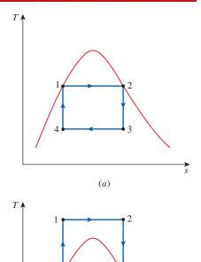
**FIGURE 11–1** *T-s* diagram of two Carnot vapor cycles.
