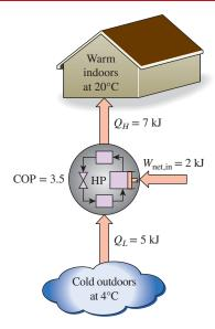
The work supplied to a heat pump is used to extract energy from the cold outdoors and carry it into the warm indoors.
