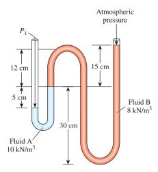
**1–76** Consider the manometer in Fig. P1–75. If the specific weight of fluid A is 100 kN/m<sup>3</sup>, what is the absolute pressure, in kPa, indicated by the manometer when the local atmospheric pressure is 90 kPa?
