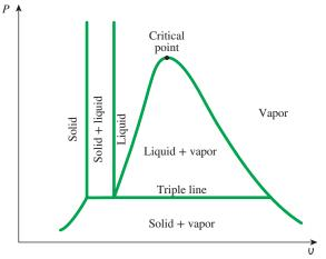
(a) P-U diagram of a substance that contracts on freezing
