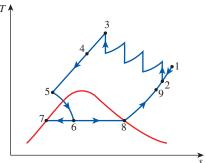
FIGURE 12–17 Linde-Hampson system for liquefying gases.
