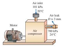
FIGURE 8–35 Schematic for Example 8–11.
