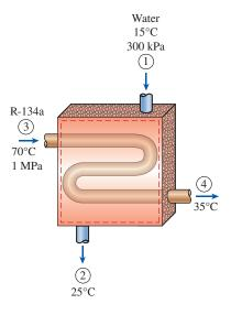
**FIGURE 5-40** Schematic for Example 5–10.
