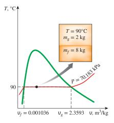
FIGURE 3–35 Schematic and *T-V* diagram for Example 3–4.
