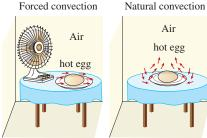
The cooling of a boiled egg by forced
