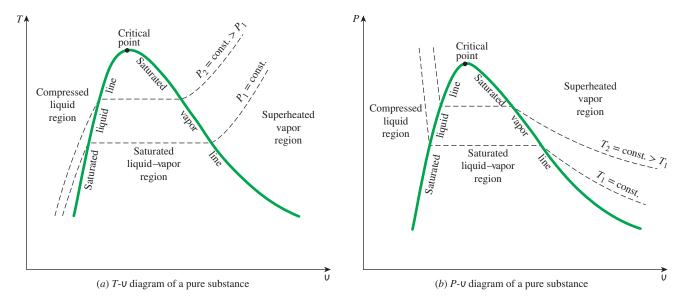
FIGURE 3–17 Property diagrams of a pure substance.
