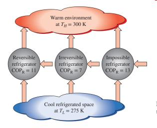
No refrigerator can have a higher COP than a reversible refrigerator operating between the same temperature limits.
