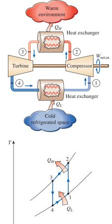
FIGURE 12–19 Simple gas refrigeration cycle.
