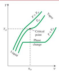
FIGURE 3–16 At supercritical pressures  $(P > P_{cr})$ , there is no distinct phase-change (boiling) process.
