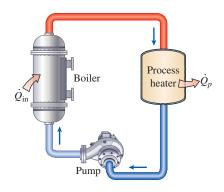
FIGURE 11–22 A simple process-heating plant.
