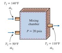
FIGURE 5-36 Schematic for Example 5–9.
