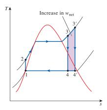
FIGURE 11–7 superheating the steam
