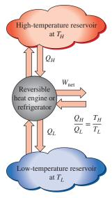
For reversible cycles, the heat transfer ratio  $Q_H/Q_L$  can be replaced by the absolute temperature ratio  $T_H/T_L$ .
