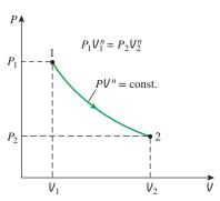
FIGURE 4–9 Schematic and *P-V* diagram for a polytropic process.
