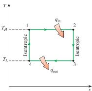
**FIGURE 10–5** *P*-U and *T-s* diagrams of a Carnot cycle.
