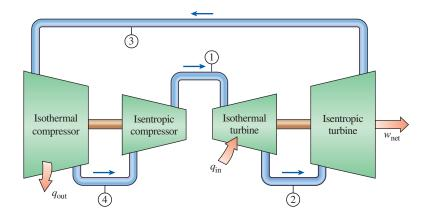
FIGURE 10-6 A steady-flow Carnot engine.
