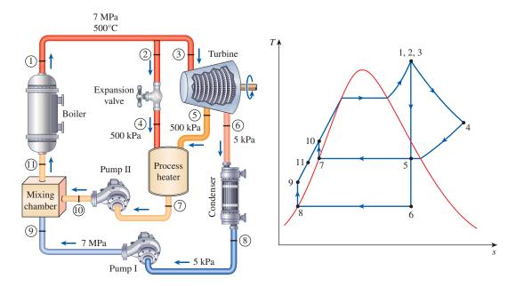
**FIGURE 11–25** Schematic and *T-s* diagram for Example 11–8.
