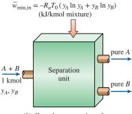
(b) Complete separation of 1 kmol mixture into its components A and B
