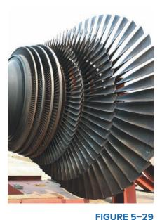
Turbine blades attached to the turbine shaft.
