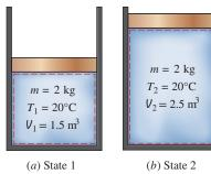
FIGURE 1–26 A system at two different states.
