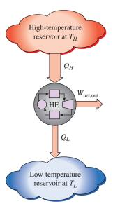
FIGURE 6-13 Schematic of a heat engine.
