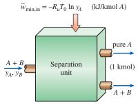
(a) Separating 1 kmol of A from a large body of mixture
