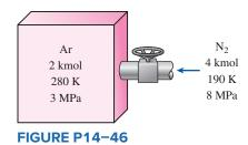
Reconsider Prob. 14-46. Using appropriate software, study the effect of varying the moles of nitrogen supplied to the tank over the range of 1 to 10 kmol of  $N_2$ . Plot the final pressure of the mixture as a function of the amount of nitrogen supplied using the ideal-gas equation of state and the compressibility chart with Dalton's law.
