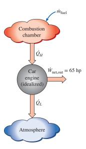
**FIGURE 6–17** Schematic for Example 6–2.
