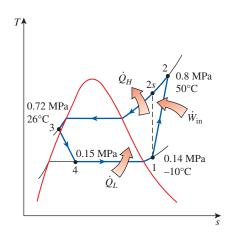
**FIGURE 12–8** *T-s* diagram for Example 12–2.
