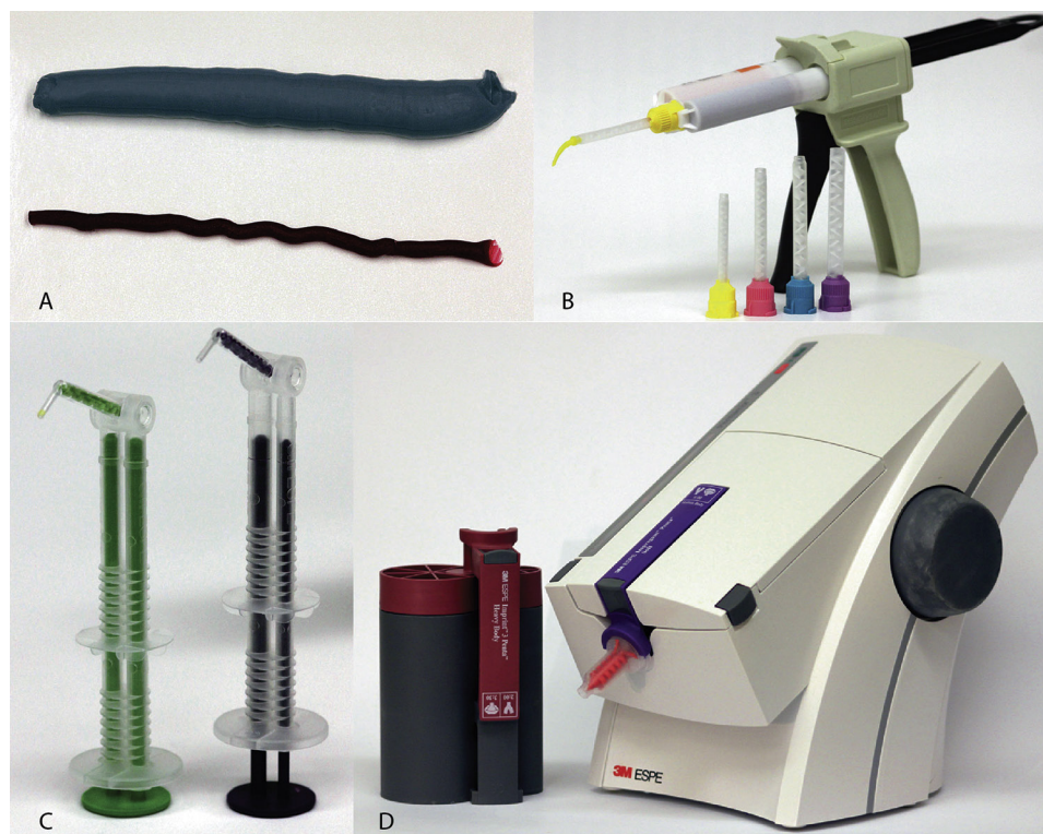
• Figure 13-7 Mixing systems. A , Hand mixing. Two equal lengths of the material are dispensed on the mixing pad with the mixing spatula. B , Static mixing. When the trigger is pulled, the plunger is driven forward (to the left) so that the base and catalyst pastes are forced from the cartridge into the mixing tip ( extreme left ). The pastes pass through the bore and exit the nozzle as a uniform mixed paste. Four different sizes of mixing tips are shown; the more viscous the material, the larger is the mixing tip that should be used. Syringe tips can be fit to the nozzle to deliver the mixed paste directly to the prepared teeth. C , Static mixing syringe. These syringes fit the cartridge, such as the mixing tips shown in ( B ). The base and catalyst are first injected into the respective barrel. A plunger then forces the material through a smaller static mixing tip. It can deliver the light-body material directly onto the abutment(s). D , Dynamic mechanical mixing. The motor-driving mechanism forces the material into the mixing tip and makes the impeller ( insert ) inside the tip rotate. The function of the impeller is only to mix the material.
