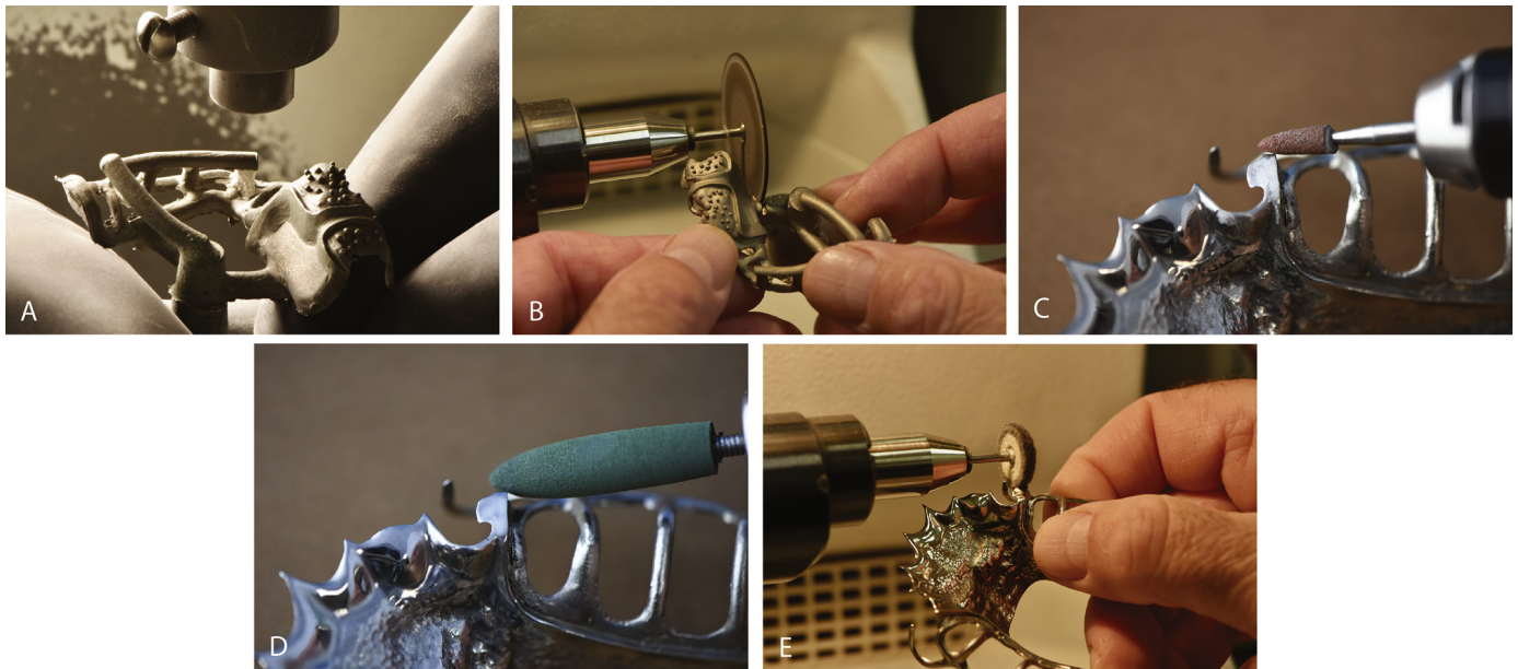
• Figure 16-1 Abrasive types used to finish hard metal restorations with complex forms such as Co-Cr alloy partial denture frameworks. A , The partial denture framework casting is sandblasted (air-particle abraded) to remove residual casting investment. B , A silicon carbide disc is used on a dental lathe to cut the casting sprues. C , Mounted corundum stones are used to grind excess metal left from cutting. D , A series of rubber bonded abrasives containing progressively smaller silicon carbide grits is used to provide a fine finish to the framework. E , Using felts with bar-type abrasives applied to bring the external finish of the framework to a final high-luster polish. (Courtesy Bego USA.)
