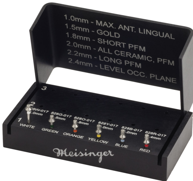
• Figure 16-10 Specialized diamond burs for occlusal reduction of tooth surfaces. Color-coded bands refer to the depth of occlusal reduction that will be created when grinding to the depth of the wide stop above the diamond-coated portion of the bur. (Courtesy Meisinger USA.)
