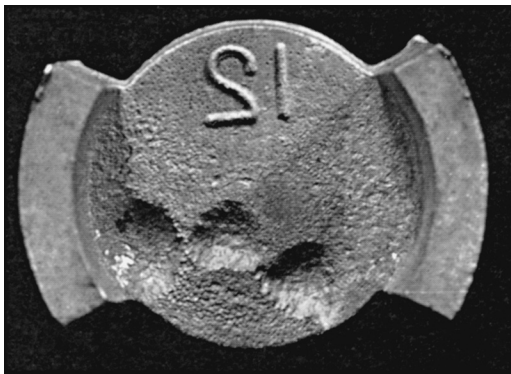
• Figure 14-25 Surface irregularity on the cavity side of a casting caused by back-pressure porosity.
