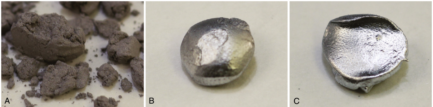
• Figure 8-10 Appearance of freshly triturated amalgam mixture. A , A grainy, undertriturated mixture; a restoration made of such a mixture has low strength and poor resistance to corrosion. The mixture may appear as a solid mass, but the surface remains without luster, as shown. B , A properly triturated amalgam that appears rounded, with a smooth, shiny surface. C , An overtriturated amalgam mixture, which is shinier than that of the properly triturated one, and because of more fluid consistency, the mass appears flattened by the force of trituration.
