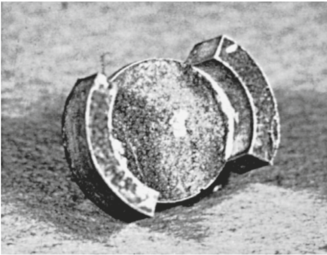
• Figure 14-22 A black-coated noble-metal alloy casting resulting from sulfur contamination or oxidation during alloy melting.
