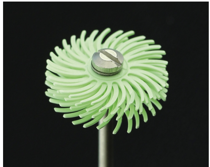
• Figure 16-9 Spiral wheel polishers are designed for maximal flexibility of use on most areas of a restoration. These polishers have a polyamide rubber construction and are available in different diameters with several types and grits of embedded abrasive. Laboratory and clinic polishers are available for use on denture acrylics, composites, ceramics, and precious metals. (Courtesy Dr. Farzan Pouranfar.)
