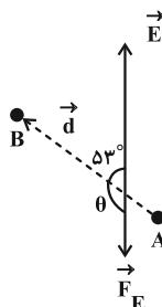
$$W_E = |q| |E| d \cos \theta \xrightarrow[|q|=5\times 10^{-3} \text{ C}, E=6\times 10^4 \frac{\text{N}}{\text{C}}]{d=20 \text{ cm}=0.2 \text{ m}, \theta=127^\circ} W_E = 5 \times 10^{-3} \times 6 \times 10^4 \times 0.2 \cos(127^\circ)$$
