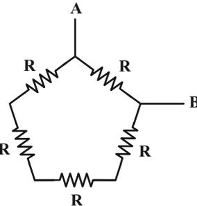
$$R_{eq} = R_{min} = \frac{4R \times R}{4R + R} = \frac{4}{5}R$$
