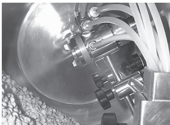
Fig. 33.3 Example of spray coating in a pan coater.
