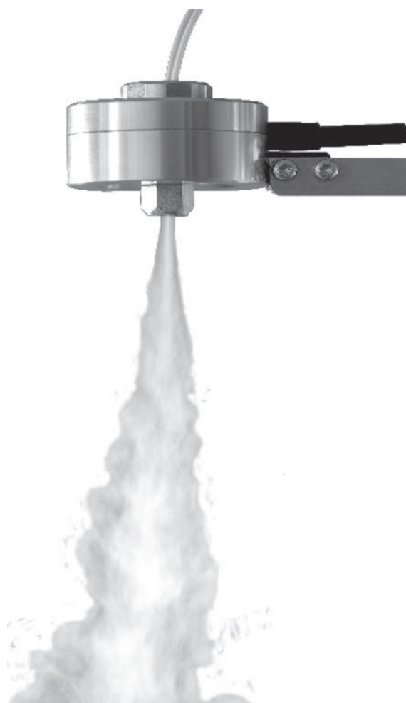
Fig. 30.8 Two-fluid nozzle atomization. (Courtesy of Buchi.)
