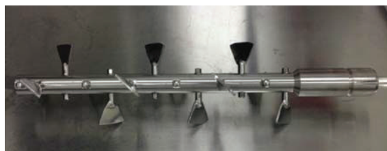
Fig. 34.8 Mixer shaft with 12 impeller blades. (Reproduced with permission from Roth, W.J., Almaya, A., Kramer, T.T., Hofer, J.D. 2017. A demonstration of mixing robustness in a direct compression continuous manufacturing process. J. Pharm. Sci. 106, 1339–1346.)
