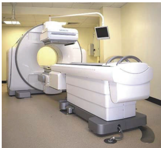
Fig. 47.3 A positron emission tomography (PET)/single photon emission computed tomography (SPECT) scanner. (From http://www.newcastle-hospitals.org.uk/news/news-item-21763.aspx )
