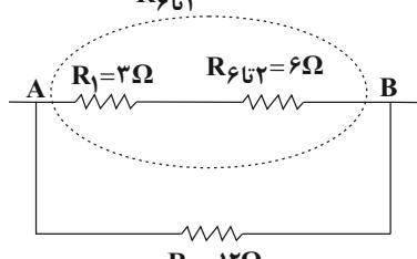
$$R_{eq} = \frac{12 \times 9}{12 + 9} = \frac{9 \times 12}{21} \Rightarrow R_{eq} = \frac{36}{7}\Omega$$
