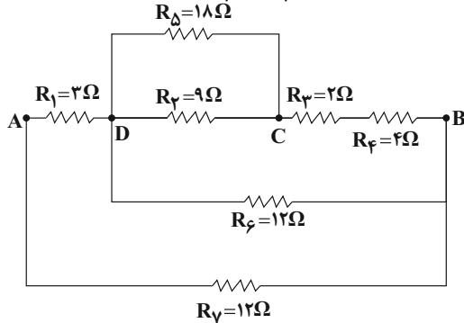
$$R_{2,5} = \frac{9 \times 12}{9 + 12} = 6\Omega, R_{3,4} = 2 + 4 = 6\Omega$$
