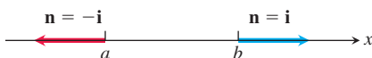
FIGURE 15.84 The outward unit normals at the boundary of [a, b] in one-dimensional space.
