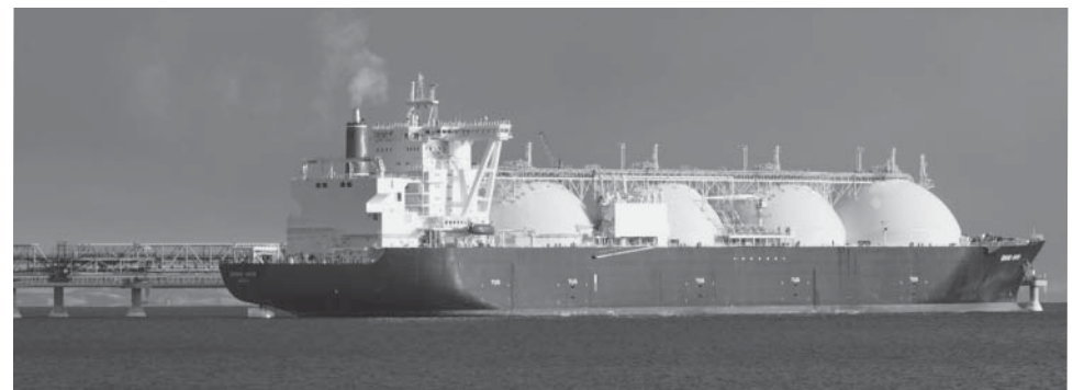
FIGURE 2.25 A tanker to transport liquefied natural gas (LNG), which is mainly methane.
