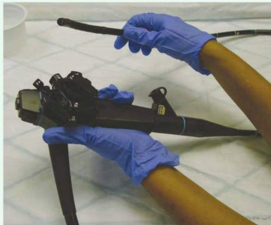
Fig. 4.69 The endoscope is a flexible plastic tube that can be controlled from the proximal end. Through a side portal various devices can be inserted, which run through the endoscope and can be used to obtain biopsies and to perform minor endoluminal surgical procedures (e.g., excision of polyps).
