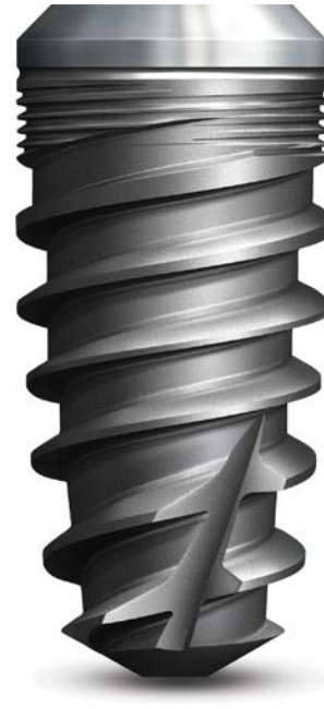
• Fig. 3.24 Implant with helical self-tapping feature designed to reduce tapping force and collect bone chips. (Image courtesy of Glidewell Dental, Newport Beach, California)
