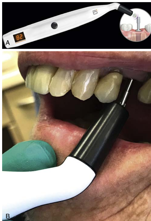
• Fig. 42.7 (A, B) Penguin Resonance Frequency Analysis Unit (Aseptico) which measures the ISQ (Implant Stability Quotient) implant stability using reusable, calibrated MultiPegs.
