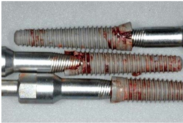
• Fig. 3.8 Implants that fractured during insertion and had to be removed. (Image courtesy of Glidewell Dental, Newport Beach, California)
