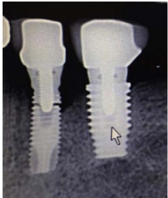
• Fig. 7.29 Implant prosthesis splinting. Radiograph showing implant fracture in a patient with parafunction. Most likely if the implants were splinted, then the implant body fracture would not have occurred.
