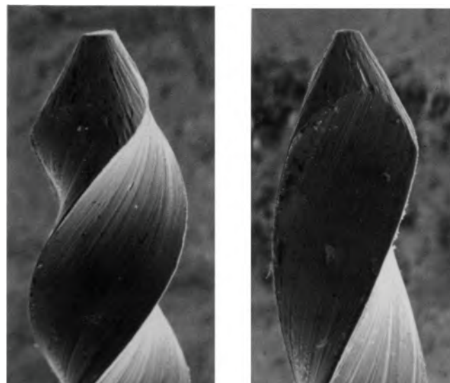
FIGURE 20-35 Scanning electron microscopy image of the flexible stainless steel Flexoreamer (left) and K-Flexofile, both having a non-cutting tip.
