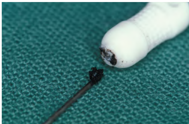
FIGURE 20-42 Severe corrosion of a nickel-titanium hand instrument following sterilization.
