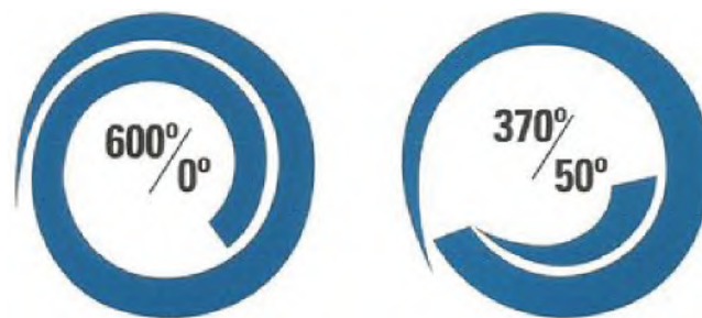
FIGURE 20-57 TF Adaptive instruments work with a full rotation of maximum 600 degrees if no friction is present. Under friction, the rotation is changed into a 370° clockwise and 50° counterclockwise motion.
