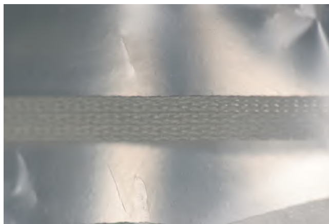
FIGURE 35-21 Close-up of polyethylene fiber-reinforced post material in its original package. (Reprinted with permission from Baba NZ. 331 )
