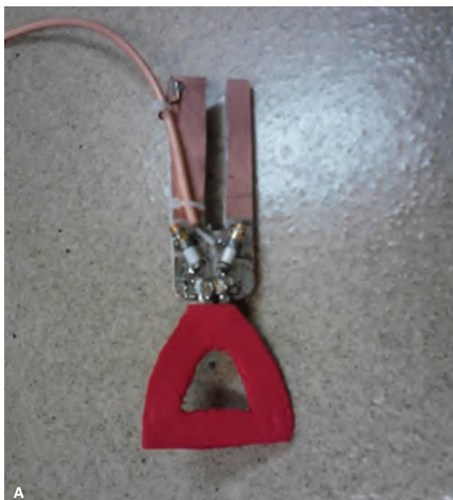
FIGURE 9D-5 A , Intraoral RF loop coil containing copper foil of 10 mm in width. Its design was fit to the average adult maxillary arch. B , In-vivo experimental coil set. Loop coil was placed in occlusal position. (Adapted from Idiyatullin D, Corum CA, Nixdorf DR, Garwood M. Intraoral approach for imaging teeth using the transverse B1 field components of an occlusally oriented loop coil. Magn Reson Med 2014;72:160-5. Used with permission.)
