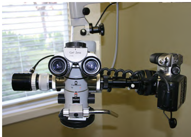
FIGURE 19-6 A beam splitter on the microscope allows the addition of adapters to accommodate video and SLR photography. (Courtesy of Dr. Terrell F. Pannkuk, Santa Barbara, CA.)
