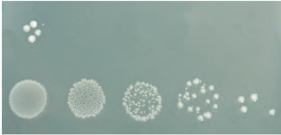
FIGURE 21-3 The size of the initial inoculum and the depth of the 10-fold dilution series determine the accuracy of measurement of the colony forming units. In this example, killing effectiveness can be calculated to a level of about 99.99%. Upper row: medication has killed so many bacteria that only in the non-diluted specimen (leftmost) a few cells can be seen. Lower row: control specimen (water: no killing).
