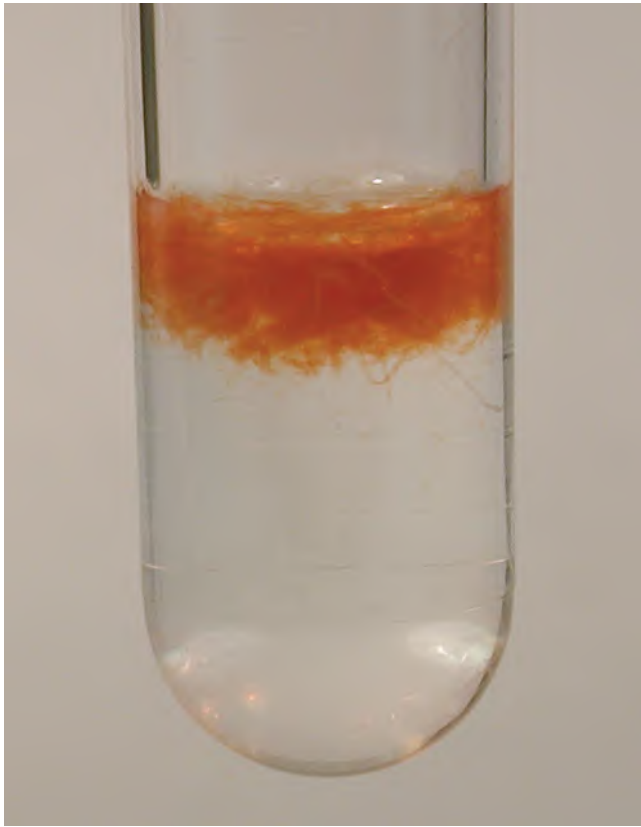
FIGURE 21-12 Orange-brown precipitate forms immediately when CHX and NaOCl are mixed together. The precipitate may contain toxic substances such as para-chloroaniline.
