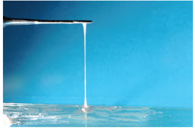
FIGURE 22-44 Properly prepared sealer must not "drip," but make at least a 8–10 cm "string."
