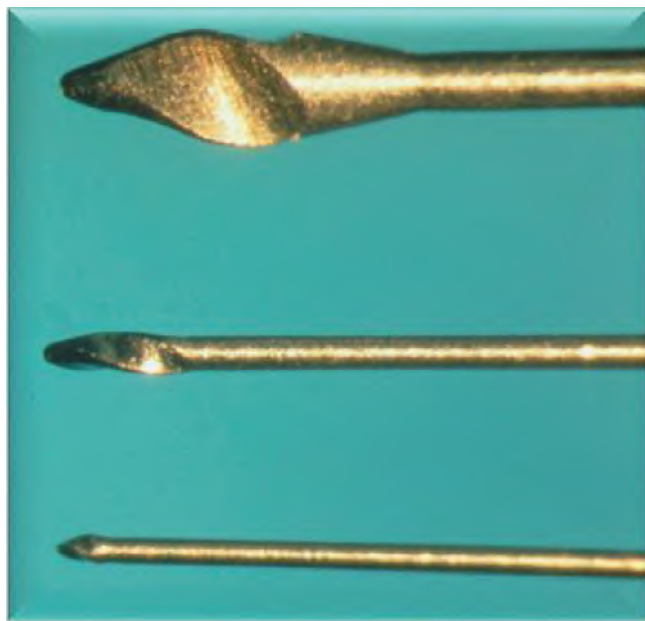
FIGURE 20-49 Each LightSpeed file shows a unique tip with tip size, conicity and length increasing slightly from one instrument to the next.
