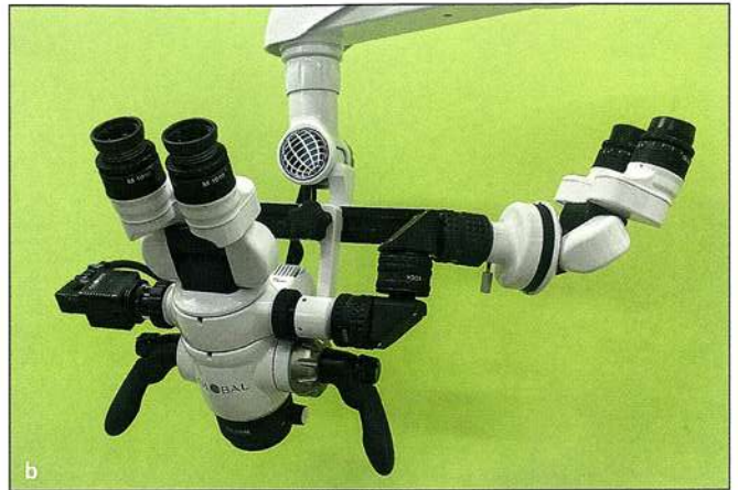
Fig 7-8 (a) JEDMED V-Series SOM with assistant binoculars, three-chip video camera, and counterbalanced arms. (b) Global A-6 SOM with assistant observation scope, high-definition digital camera, and 100,000-lux illumination. (c) Zeiss OPMI PROergo SOM with magnetic clutches, power zoom, and power focus on the handgrips.
