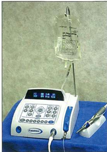
Fig 10-16 Aseptico 7000 motor and NSK 2:1 nose-cone handpiece.
