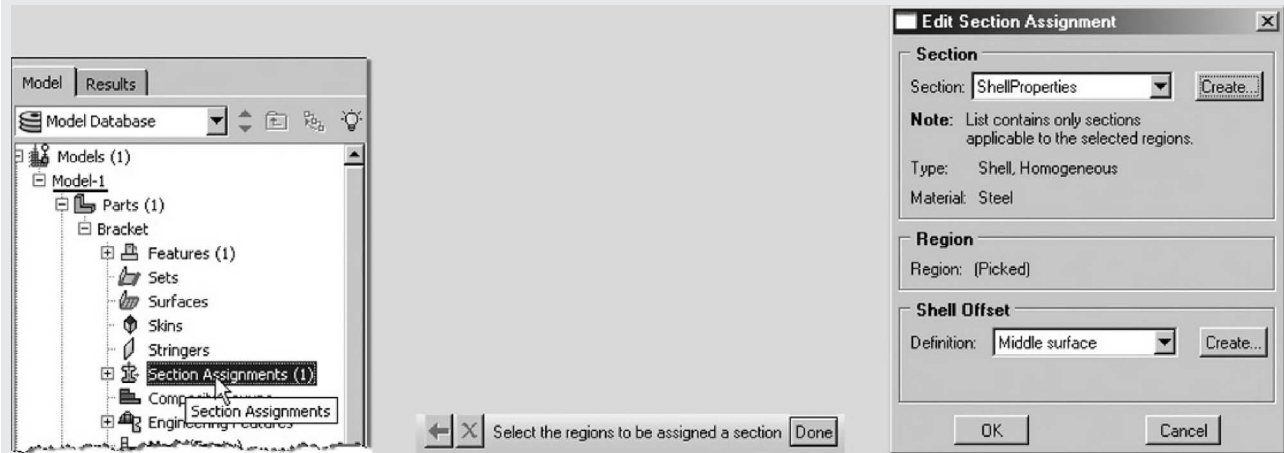
FIGURE 21.17 Section assignment in model dialogue box.
