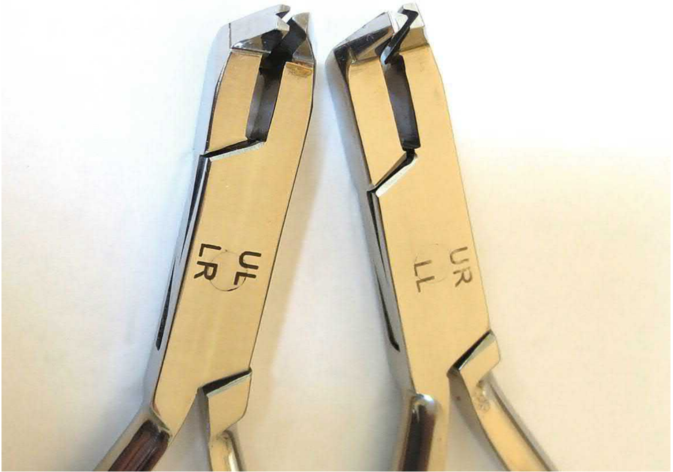
Fig. 3.15 Khouri Bendistal pliers are reliable tools for bending wire ends and V bends.
