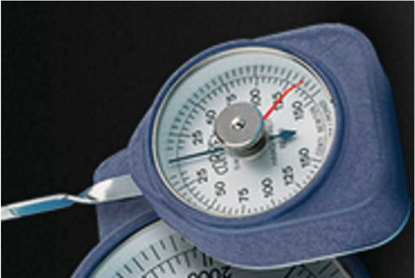
Fig. 3.14 The use of a Correx tension gauge is recommended to measure/control the level of the applied forces with cantilevers.
