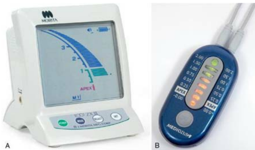
FIG. 8.36 Root ZX apex locator with lip clip and file holder.
