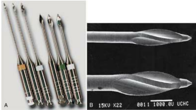
FIG. 8.24 Various Gates-Glidden (GG) burs made of stainless steel (A) and scanning electron micrograph (B, working tip).
