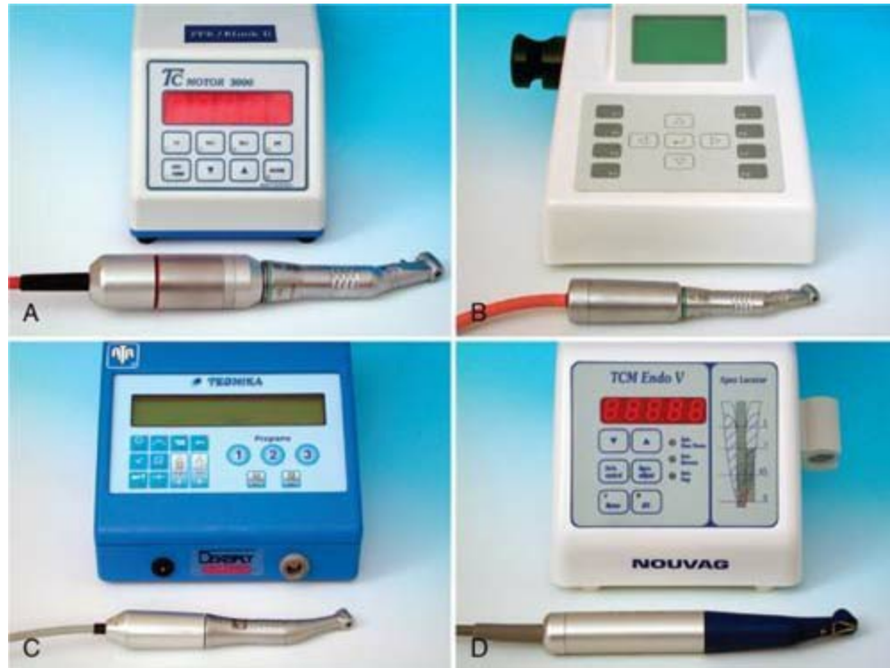
FIG. 8.30 Examples of motors used with rotary nickel-titanium endodontic instruments. A , First-generation motor without torque control. B , Fully electronically controlled second-generation motor with sensitive torque limiter. C , Frequently used simple torque-controlled motor. D , Newer-generation motor with built-in apex locator and torque control.
