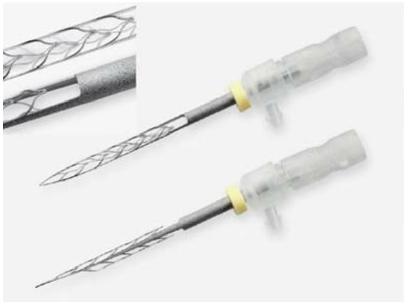
FIG. 8.26 The SAF instrument. The instrument is made as a hollow, thin NiTi lattice cylinder that is compressed when inserted into the root canal and adapts to the canal's cross section. It is attached to a vibrating handpiece. Continuous irrigation is applied through a special hub on the side of its shank.
