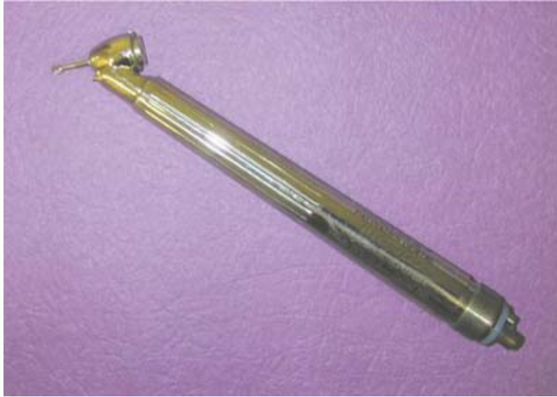
FIG. 11.33 Surgical handpiece with 45-degree angle head and rear air exhaust (Impact Air 45).
