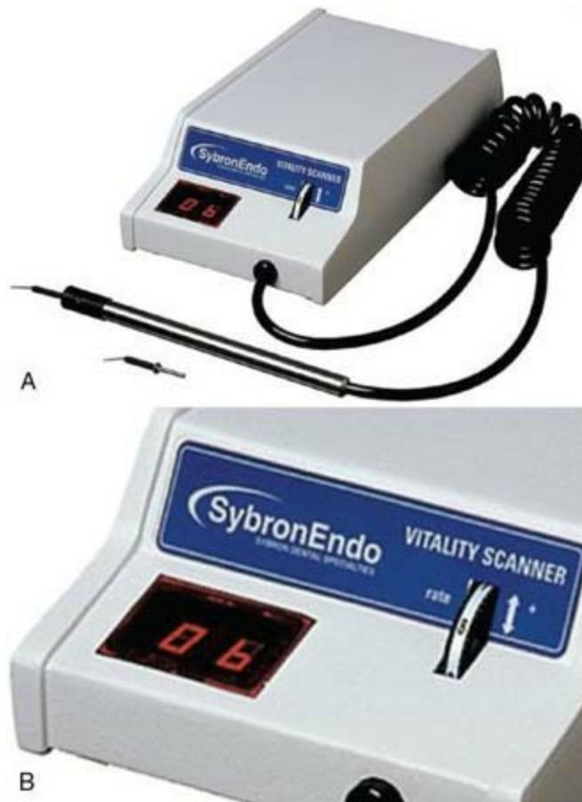
FIG. 1.20 A , Electric pulp tester with probe. The probe tip will be coated with a conducive medium, such as toothpaste, and placed in contact with the tooth surface. The patient will activate the unit by placing a finger on the metal shaft of the probe. B , View of the electric pulp tester control panel; the knob on the front right of the unit controls the rate at which the electric current is delivered to the tooth. The plastic panel on the left front displays the digital numerical reading obtained from the pulp test. The digital scale runs from 0 to 80.
