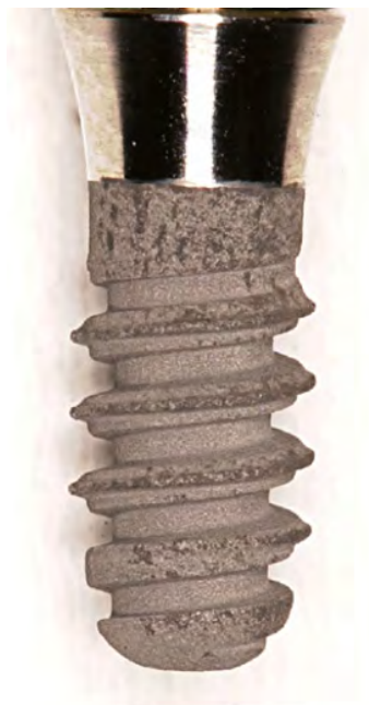
Fig. 5-7 Device used in the dog experiment. The implant is a modification of a solid screw. The distance between two consecutive threads is 1.25 mm. The depth of the trough is 0.4 mm.
