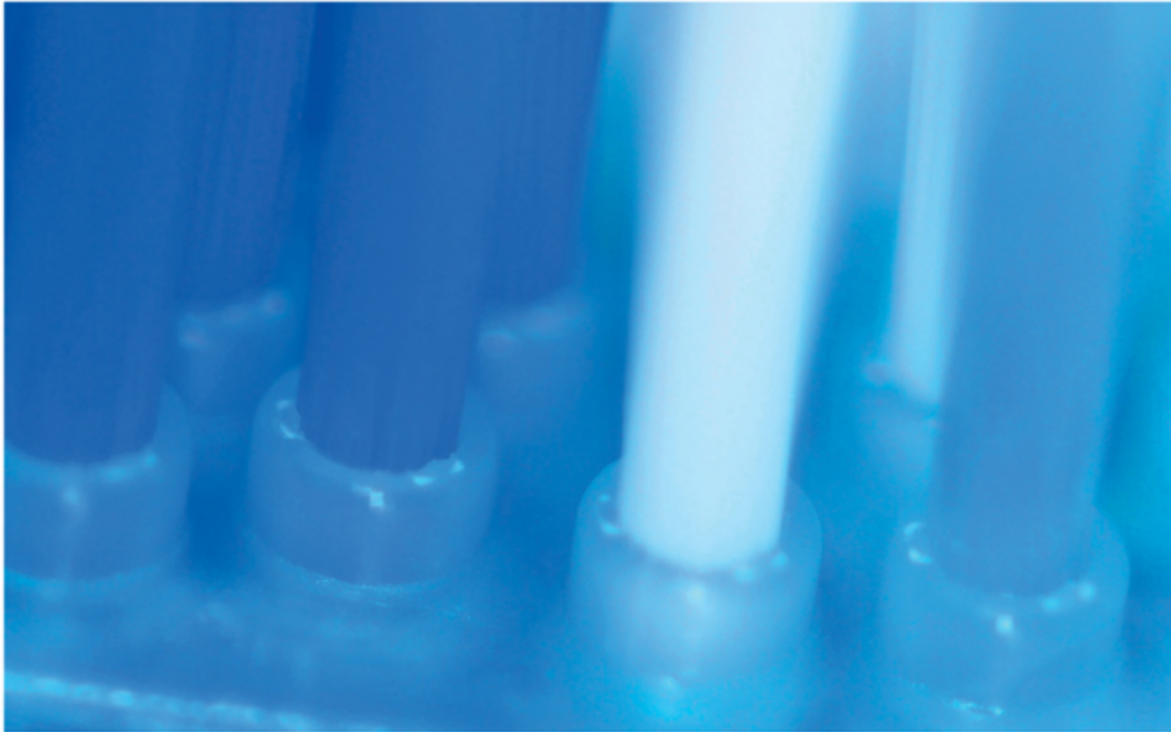
Fig 8-4 Anchorless gap free fixation of tufts.
