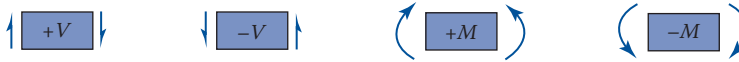
FIGURE 3.9 Sign convention for beams: definitions of positive and negative shear and moment.
