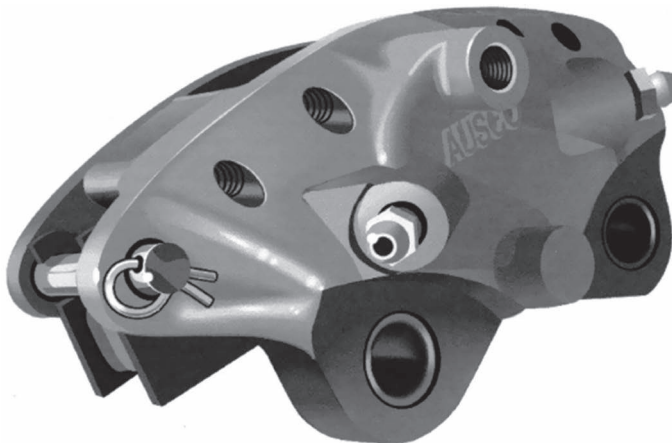
FIGURE 13.17 Caliper disk brake, hydraulically operated (Courtesy: Ausco Products, Inc., Benton Harbor, MI).
