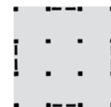
The locations of braced frames or shear walls must be considered in relation to the elevation and plan of a building.
