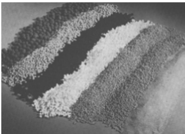
Figure 10-4(a) Catalyst particles of different shapes (spheres, cylinders) and sizes (0.1–1 cm). (Photo courtesy of BASF Corporation.)
