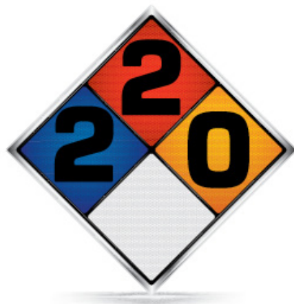
Figure 2-14 NFPA Diamond Levels of Concern for DDT. (Image: Idea.s/Shutterstock)
