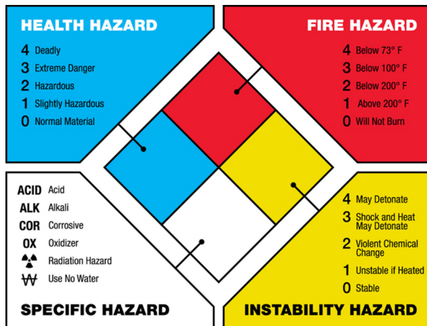
Figure 2-13 Components of each color of the NFPA Diamond. (Image: Dmitry Kovalchuk/Shutterstock)
