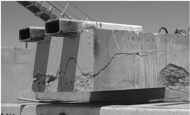
FIGURE 21.4 Tension anchor failure of a Cazaly hanger. (Photograph by Charles W. Dolan.)
