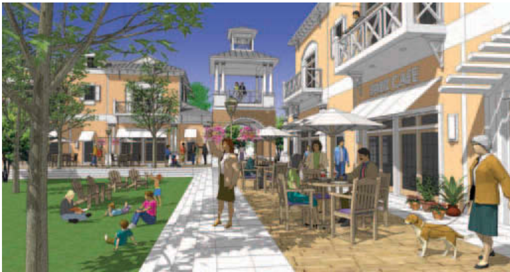
Figure 3.22 Park Café final model with all lines, shadows, and materials turned on. Three different tiffs were then exported from the model to be manipulated in Photoshop (SketchUp model and tradigital drawing by Jim Leggitt, FAIA).
