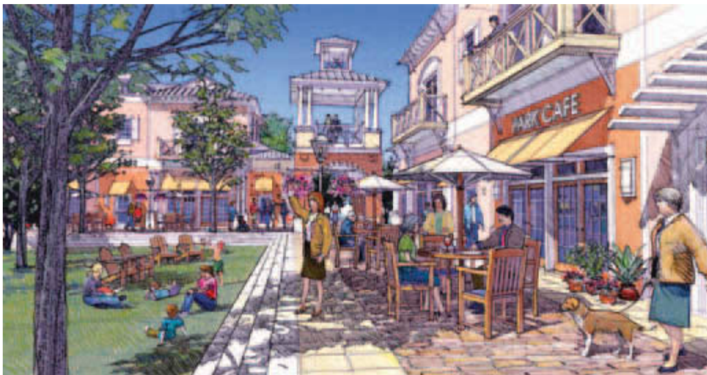
Figure 3.24 Park Café final color drawing—the large plot was colored with a combination of Chartpak AD markers, Copic markers, and Prismacolor pencils. Much of the image was retraced with a casual line technique. White pencil highlighted certain edges and pencil hatching throughout gave the image character and the much-needed informality of a hand drawing (SketchUp model and tradigital drawing by Jim Leggitt, FAIA).
