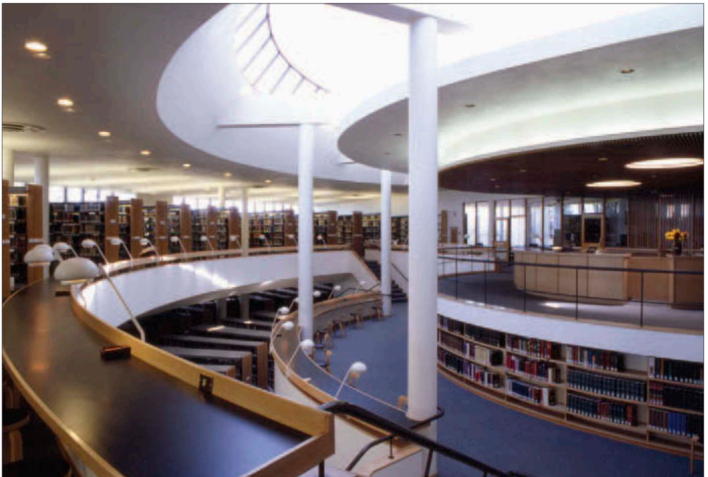
Figure 2.18 Daylight artfully penetrates multiple levels in the Mount Angel library in St. Benedict, Oregon, designed by Alvar Aalto. Splayed surfaces facilitate distribution of daylight within the space (© Lara Swimmer/ESTO).
