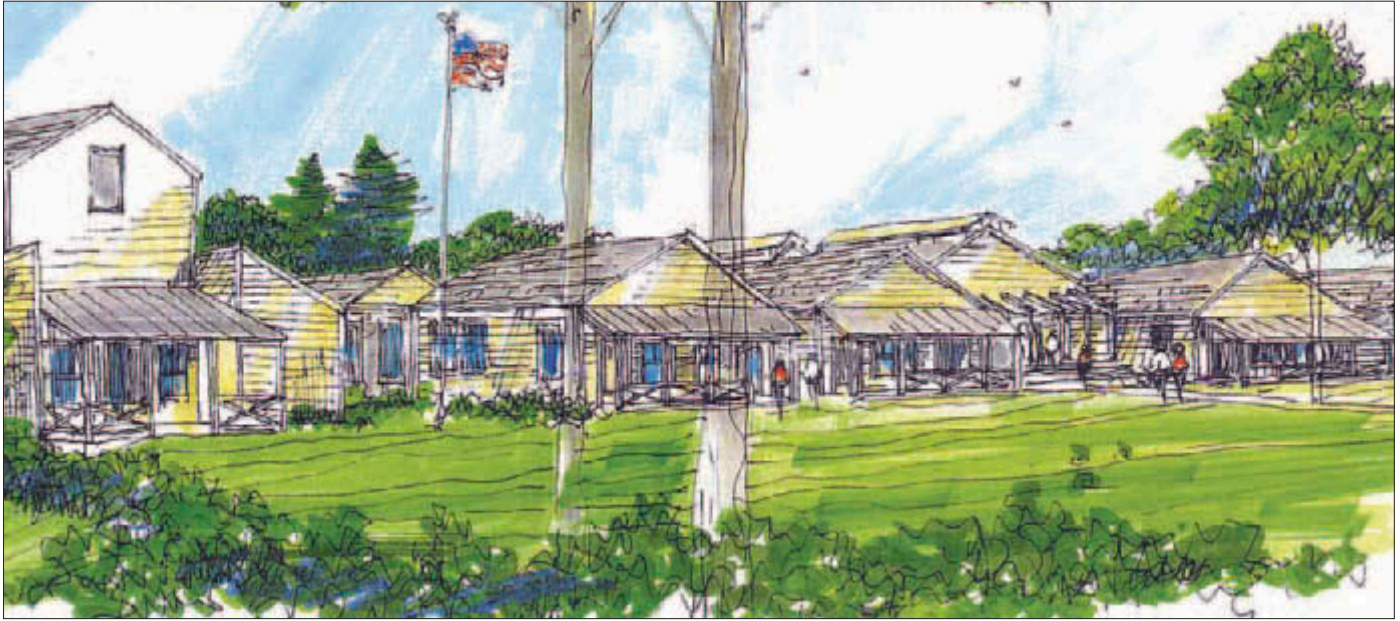
Figure 3.6 There is nothing like the ambiguous, conceptual, freehand perspective sketch to capture the spirit of a very preliminary design investigation. Shown here is a proposal for a 20,000-square-foot classroom facility in Maine (rendering by Gary Irish Graphics).
