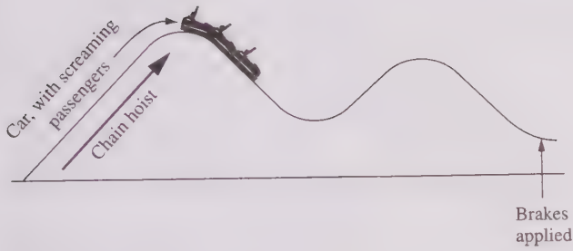
FIGURE 5.2 A simple roller coaster, which illustrates four of the five terms in Bernoulli's equation.
