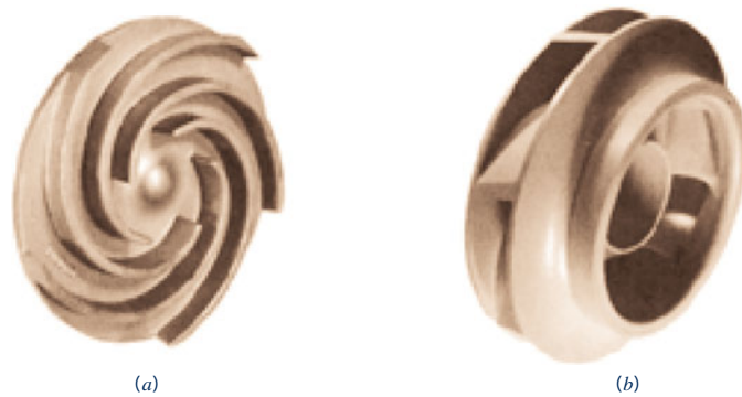
■ Figure 12.7 (a) Open impeller, (b) enclosed or shrouded impeller. (Courtesy of Flowserve Corporation)
