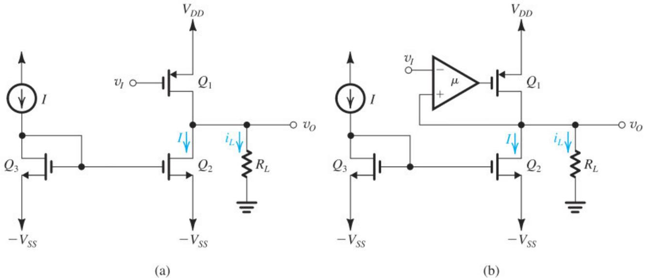
**Figure 12.21** (a) A common-source circuit offers more swing at  $v_O$ . (b) Introducing an amplifier with negative feedback reduces the output resistance and keeps  $v_O \cong v_I$ .
