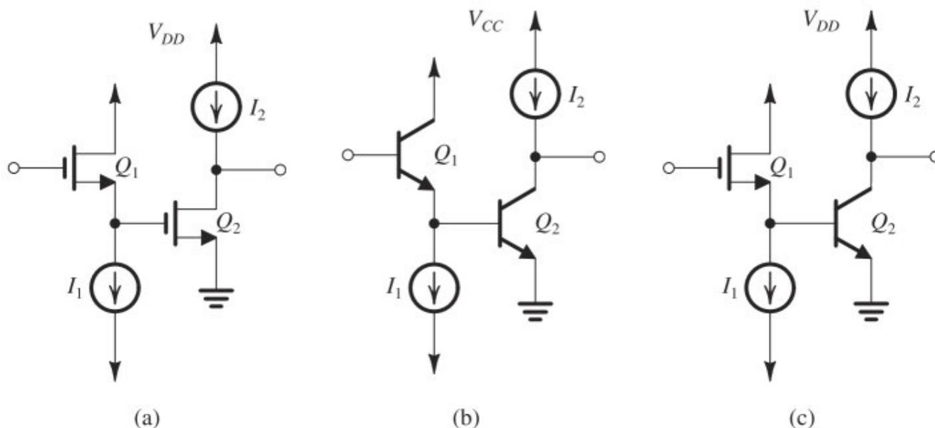
**Figure 10.32** (a) CD–CS amplifier. (b) CC–CE amplifier. (c) CD–CE amplifier.
