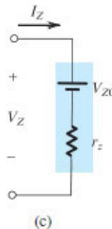
**Figure 4.13 (c)** Model for the zener diode.
