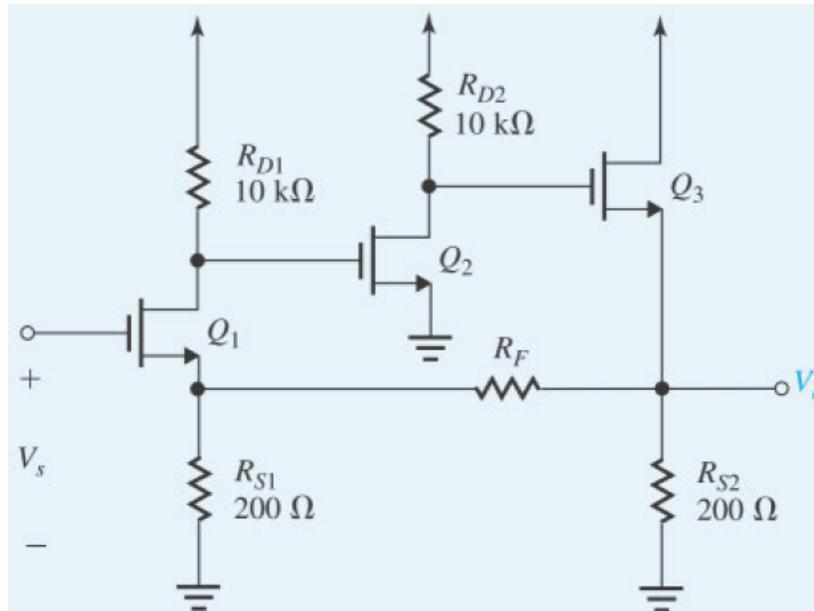
Figure VE11.1 Circuit for Video Example 11.1.
