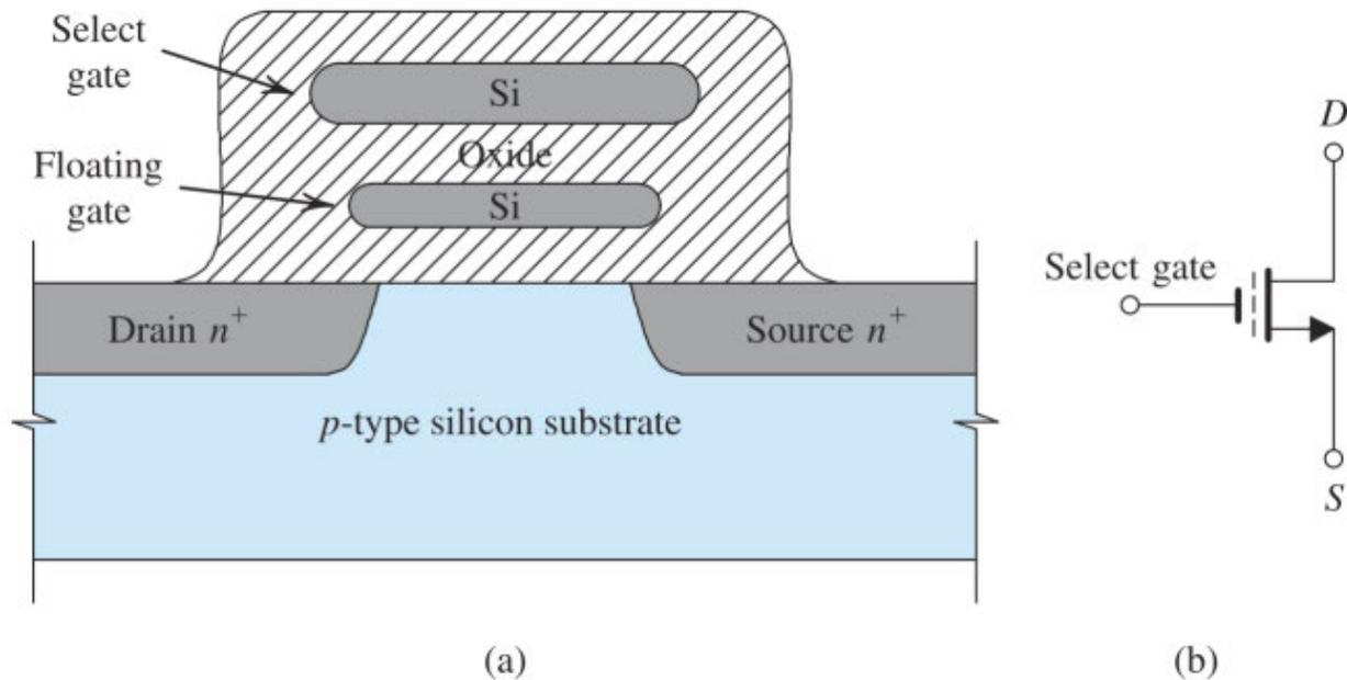
**Figure 18.30** (a) Cross section and (b) circuit symbol of the floating-gate transistor used as a Flash cell.
