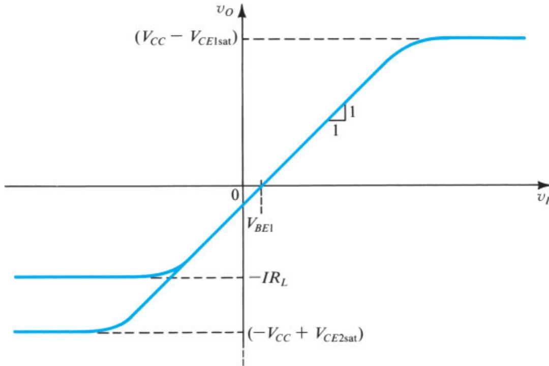
**Figure 12.4** Transfer characteristic of the emitter follower in Fig. 12.3. We obtain a linear characteristic by neglecting the change in  $v_{BE1}$  with  $i_L$ . The maximum positive output is determined by the saturation of  $Q_1$ . In the negative direction, the limit of the linear region is determined either by  $Q_1$  turning off or by  $Q_2$  saturating, depending on the values of  $I$  and  $R_L$ .
