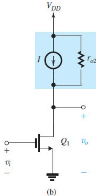
**Figure 8.15 (b)** The circuit with  $Q_2$  replaced with its large-signal model.
