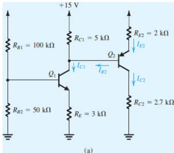
Figure 6.30 (a) Circuit for Example 6.11.
