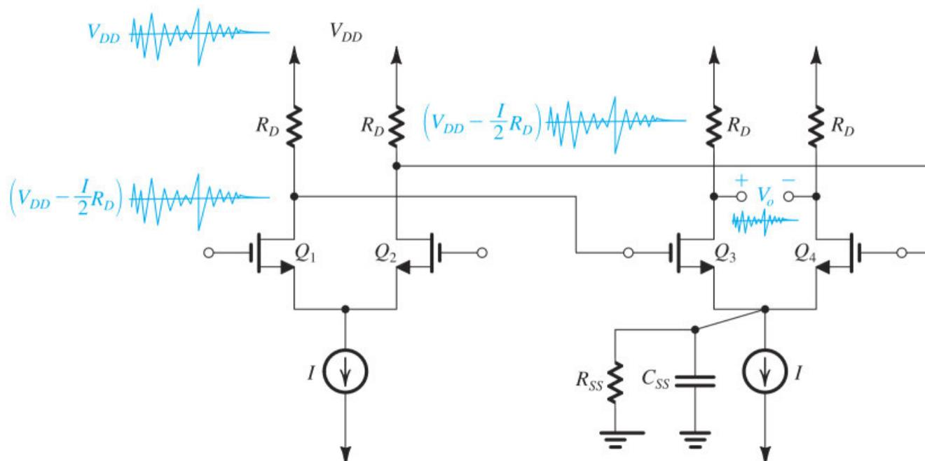
**Figure 10.28** The second stage in a differential amplifier, which is relied on to suppress high-frequency noise injected by the power supply of the first stage, and therefore must maintain a high CMRR at higher frequencies.
