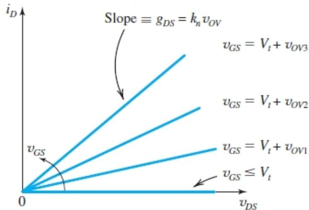
**Figure 5.4** The  $i_D$ - $v_{DS}$  characteristics of the MOSFET in Fig. 5.3 when the voltage applied between drain and source,  $v_{DS}$ , is kept small. The device operates as a linear resistance whose value is controlled by  $v_{GS}$ .
