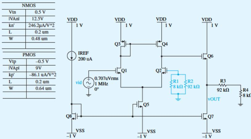
Figure B.50 Schematic capture of the A-circuit.
