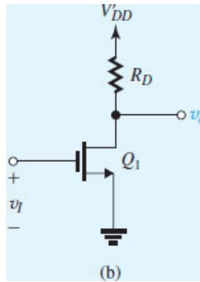
**Figure 8.16 (b)** Replacing the current-source load with a resistance  $R_D$  connected to a new power-supply voltage  $V'_{DD}$ .
