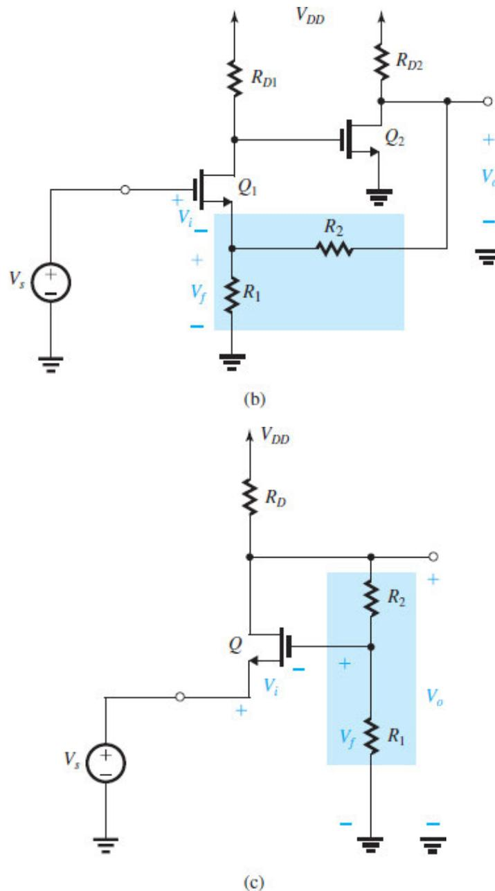
**Figure 11.9** Examples of a feedback voltage amplifier. All these circuits use series–shunt feedback. Note that the dc bias circuits are only partially shown
