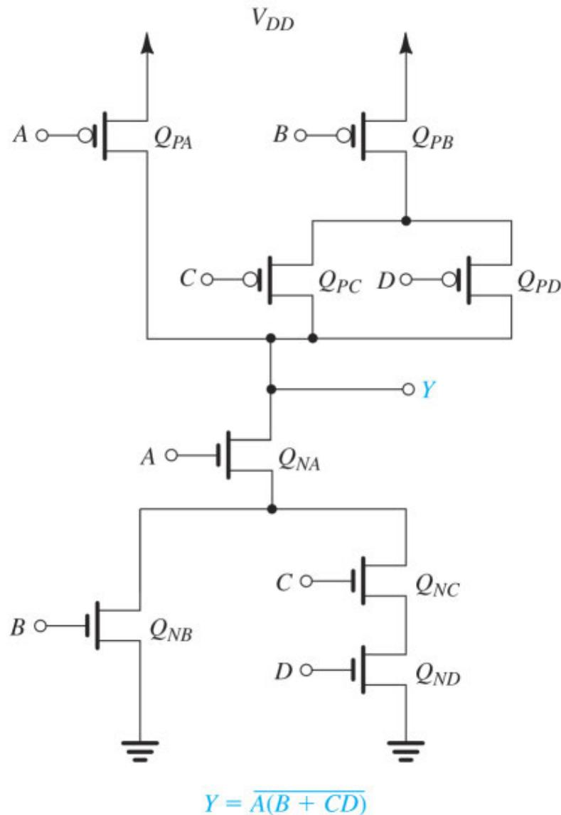
**Figure 16.9** CMOS realization of a complex gate.
