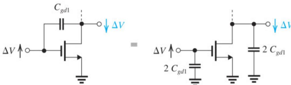
**Figure 17.7** The Miller multiplication of the feedback capacitance  $C_{gd1}$ .
