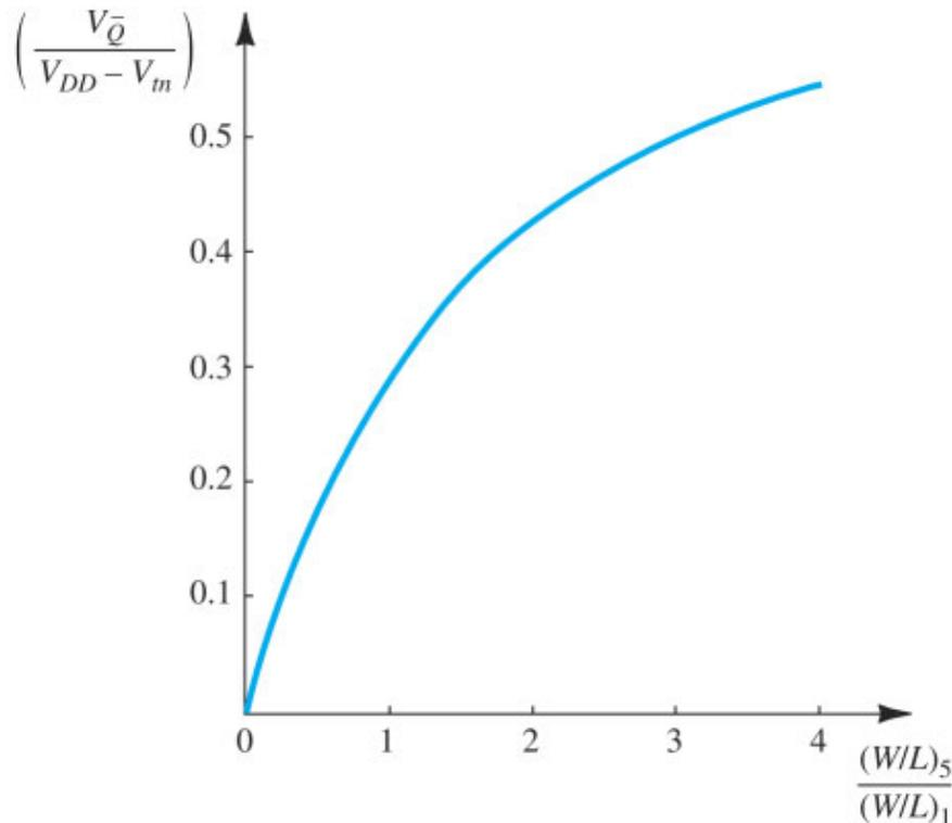
**Figure 18.24** The normalized value of  $V_{\bar{Q}}$  versus the ratio  $(W/L)_5/(W/L)_1$  for the circuit in Fig. 18.23. This graph can be used to determine the maximum value permitted for  $(W/L)_5/(W/L)_1$  so that  $V_{\bar{Q}}$  is kept below a desired level.
