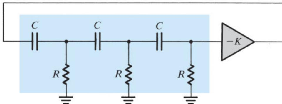
**Figure 15.9** A phase-shift oscillator.
