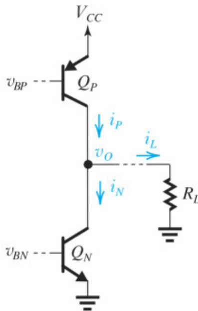
**Figure 13.28** In order to provide  $v_O$  that can swing to within 0.1 V of  $V_{CC}$  and ground, a near rail-to-rail operation, the output stage uses common-emitter transistors. Note that the driving signals  $v_{BP}$  and  $v_{BN}$  are separate but identical.
