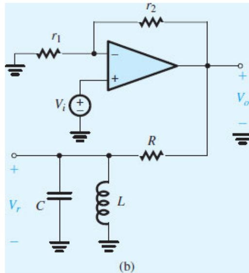
**Figure 15.2 (b)** Breaking the feedback loop at the input of the op amp to determine  $A(s) \equiv V_o(s)/V_i(s)$  and  $\beta(s) \equiv V_r(s)/V_o(s)$ , and hence the loop gain  $A(s)\beta(s)$ .
