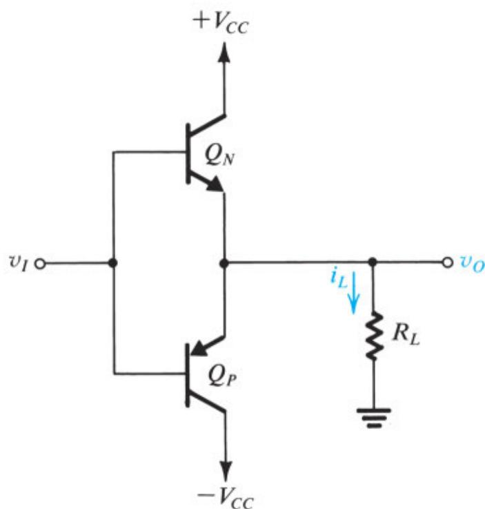
Figure 12.6 A class B output stage.
