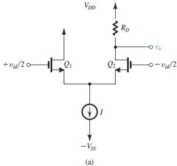
**Figure 9.30 (a)** A simple but inefficient approach for differential-to-single-ended conversion.
