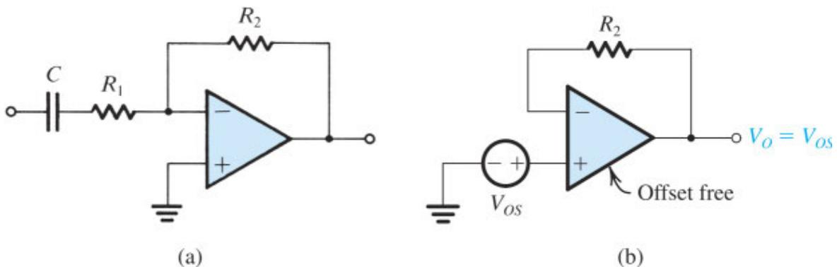
**Figure 2.32 (a)** A capacitively coupled inverting amplifier. **(b)** The equivalent circuit for determining its dc output offset voltage  $V_O$ .
