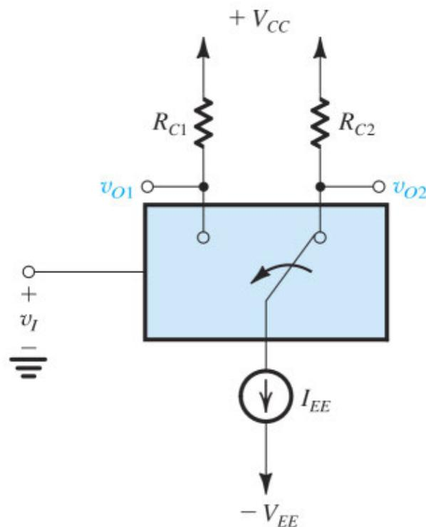
**Figure 16.19** Another inverter implementation utilizing a double-throw switch to steer the constant current  $I_{EE}$  to  $R_{C1}$  (when  $v_I$  is high) or  $R_{C2}$  (when  $v_I$  is low). This is the basis of a family of logic circuits called emitter-coupled logic (ECL).
