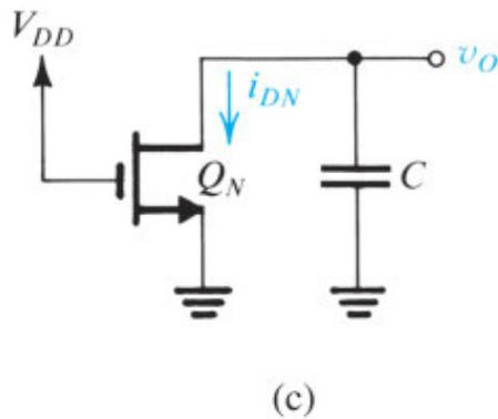
**Figure 17.4 (c)** Dynamic operation of a capacitively loaded CMOS inverter: equivalent circuit during the capacitor discharge.
