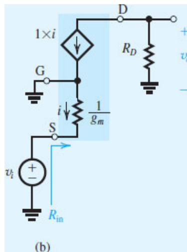
Figure 7.19 (b) Small-signal equivalent circuit of the amplifier in (a).
