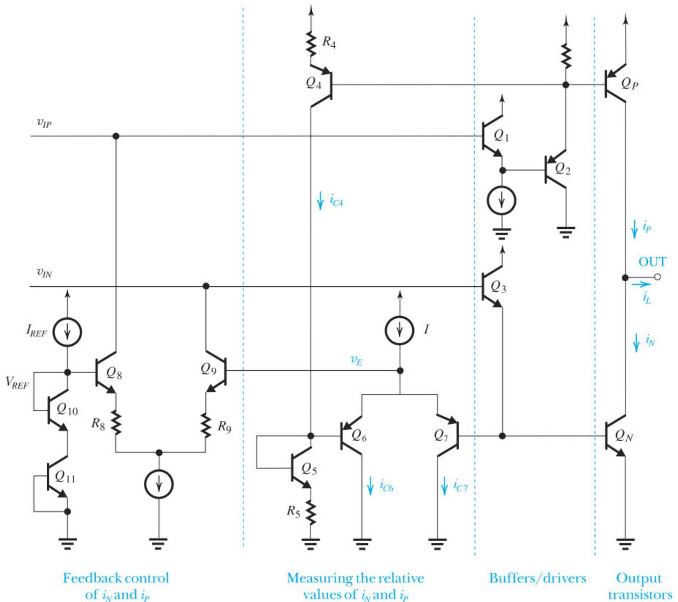
**Figure 13.30** A more complete version of the output stage showing the circuits that establish the quiescent current in  $Q_P$  and  $Q_N$ . As well, this circuit forces a minimum current of  $(I_Q/2)$  to follow in the inactive output transistor, preventing the transistor from turning off and thus minimizing crossover distortion.
