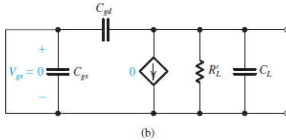
**Figure 10.12 (b)** The circuit with  $V_{sig}$  reduced to zero to determine the pole.
