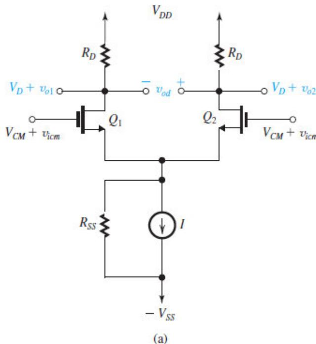
**Figure 9.24 (a)** A MOS differential amplifier with a common-mode input signal  $v_{icm}$  superimposed on the input dc common-mode voltage  $V_{CM}$ .
