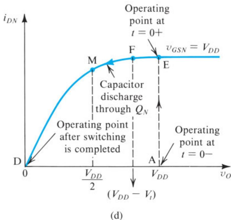
**Figure 17.4 (d)** Dynamic operation of a capacitively loaded CMOS inverter: trajectory of the operating point as the input goes high and  $C$  discharges through  $Q_N$ .
