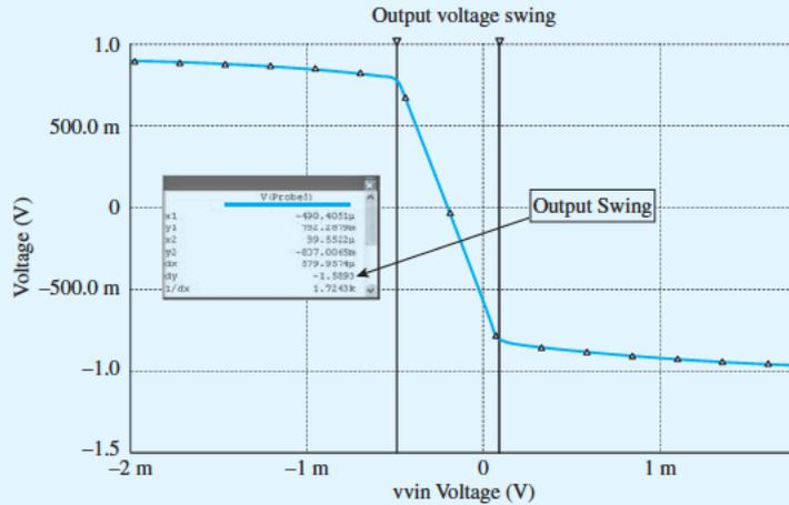
Figure B.35 Output-voltage range of the two-stage CMOS op amp.
