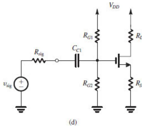
**Figure 7.50 (d)** Biasing using a fixed voltage at the gate,  $V_G$ , and a resistance in the source lead,  $R_S$ : coupling of a signal source to the gate using a capacitor  $C_{C1}$ .
