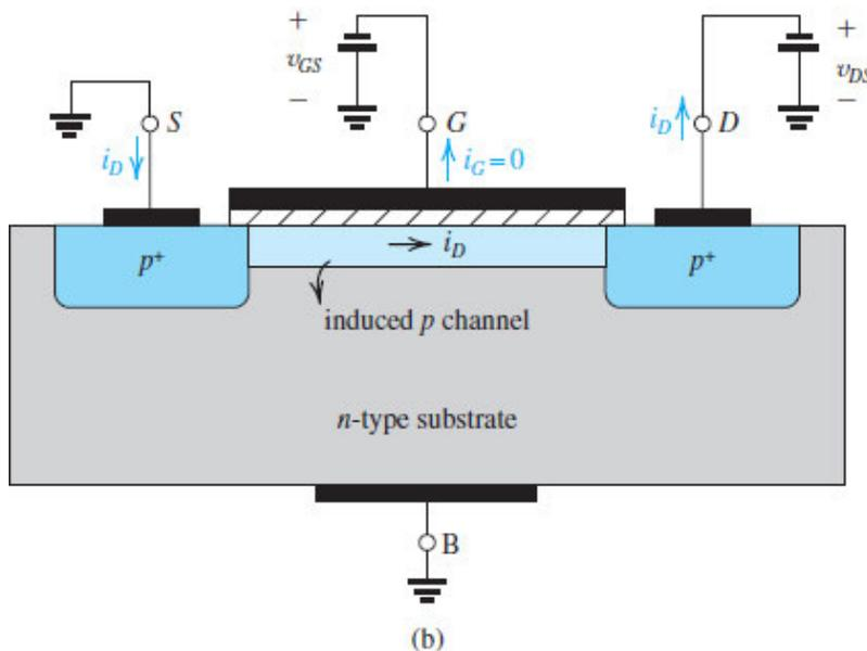
**Figure 5.9 (b)** A negative voltage  $v_{GS}$  of magnitude greater than  $|V_{tp}|$  induces a  $p$  channel, and a negative  $v_{DS}$  causes a current  $i_D$  to flow from source to drain.
