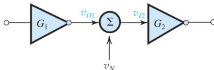
**Figure 16.14** Noise voltage  $v_N$  is coupled to the interconnection between the output of inverter  $G_1$  and the input of inverter  $G_2$ .
