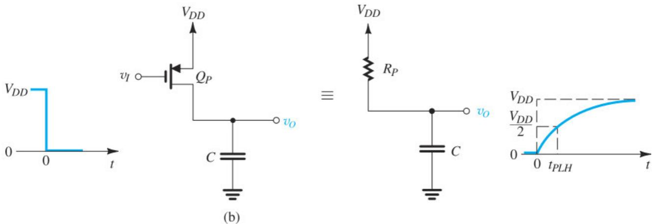
**Figure 17.5 (b)** Equivalent circuit for determining the propagation delay  $t_{PLH}$  of the inverter.
