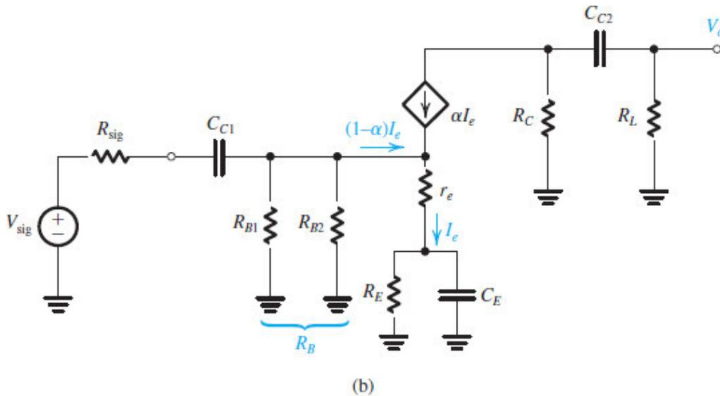
Figure 10.41 (b) Equivalent circuit of the amplifier in (a).
