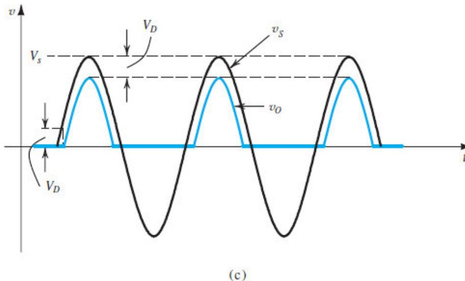
Figure 4.21 (c) Input and output waveforms.
