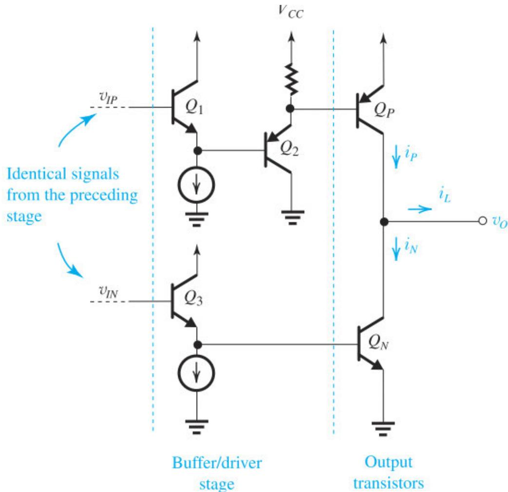
**Figure 13.29** The output stage that is operated as class AB needs emitter-follower buffers/drivers to reduce the loading on the preceding stage and to provide the current gain necessary to drive  $Q_P$  and  $Q_N$ .
