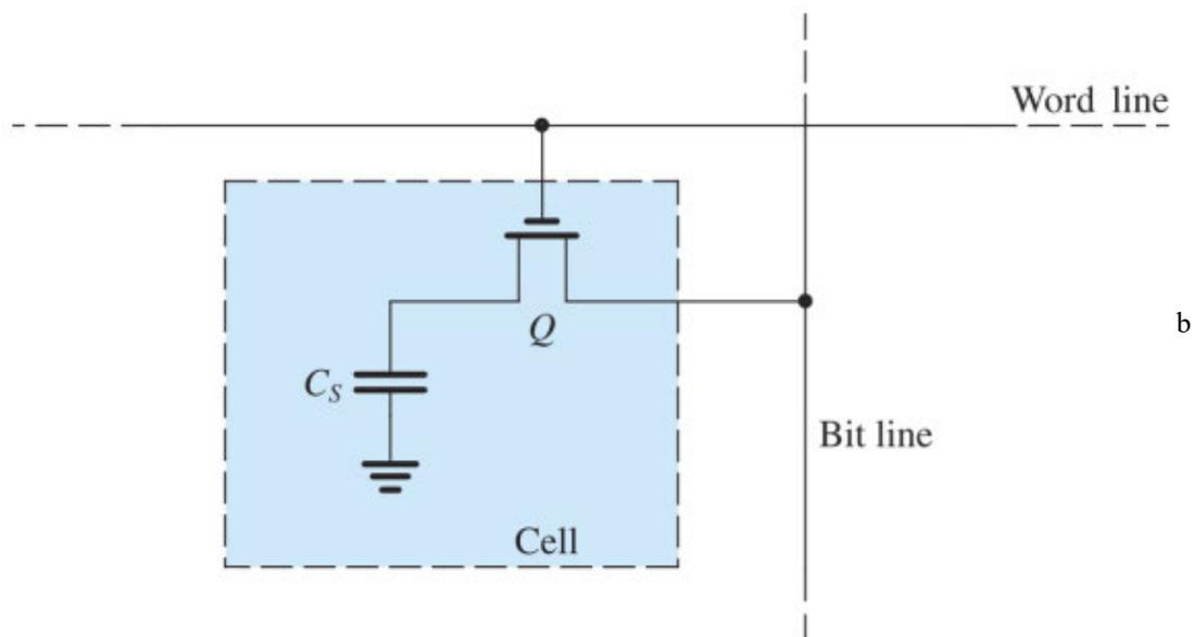
**Figure 18.28** The one-transistor dynamic RAM (DRAM) cell.
