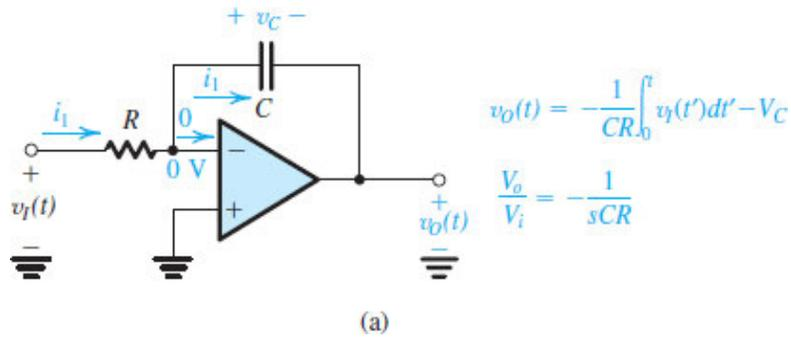
**Figure 2.24 (a)** The Miller or inverting integrator.
