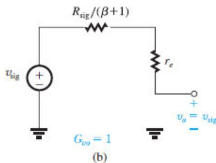
Figure 7.46 (b) Obtaining  $G_{v_o}$  from the equivalent circuit in Fig. 7.45(b).
