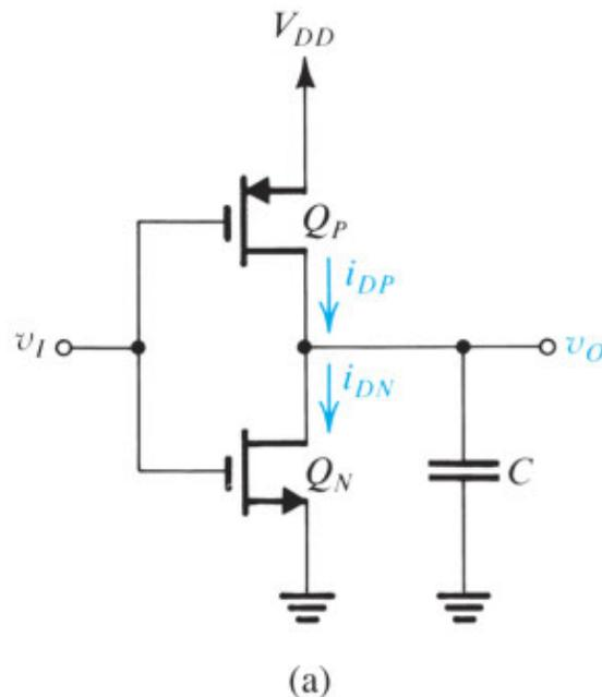
**Figure 17.4 (a)** Dynamic operation of a capacitively loaded CMOS inverter: circuit.
