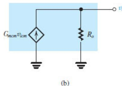
**Figure 9.36 (b)** Analysis of the current-mirror-loaded MOS differential amplifier to determine its common-mode gain: Output equivalent circuit.
