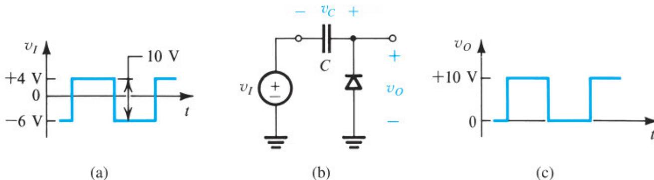
**Figure 4.29** The clamped capacitor or dc restorer with a square-wave input and no load.
