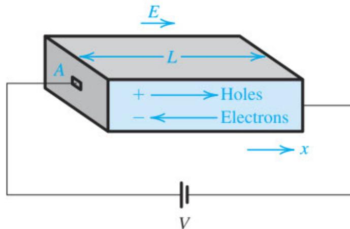
**Figure 3.5** An electric field  $E$  established in a bar of silicon causes the holes to drift in the direction of  $E$  and the free electrons to drift in the opposite direction. Both the hole and electron drift currents are in the direction of  $E$ .
