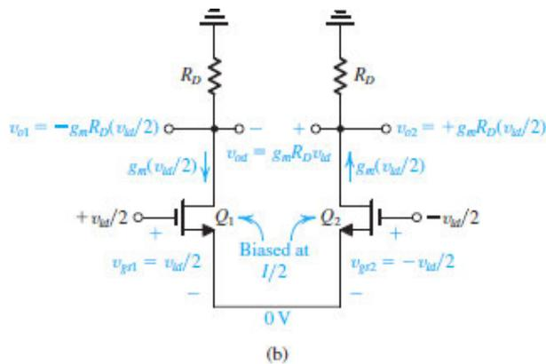
**Figure 9.8 (b)** Small-signal analysis of the MOS differential amplifier: The circuit prepared for small-signal analysis.
