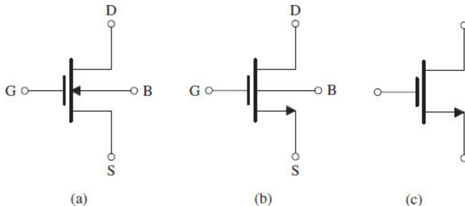
**Figure 5.11** (a) Circuit symbol for the  $n$ -channel enhancement-type MOSFET. (b) Modified circuit symbol with an arrowhead on the source terminal to distinguish it from the drain and to indicate device polarity (i.e.,  $n$  channel). (c) Simplified circuit symbol to be used when the source is connected to the body or when the effect of the body on device operation is unimportant.
