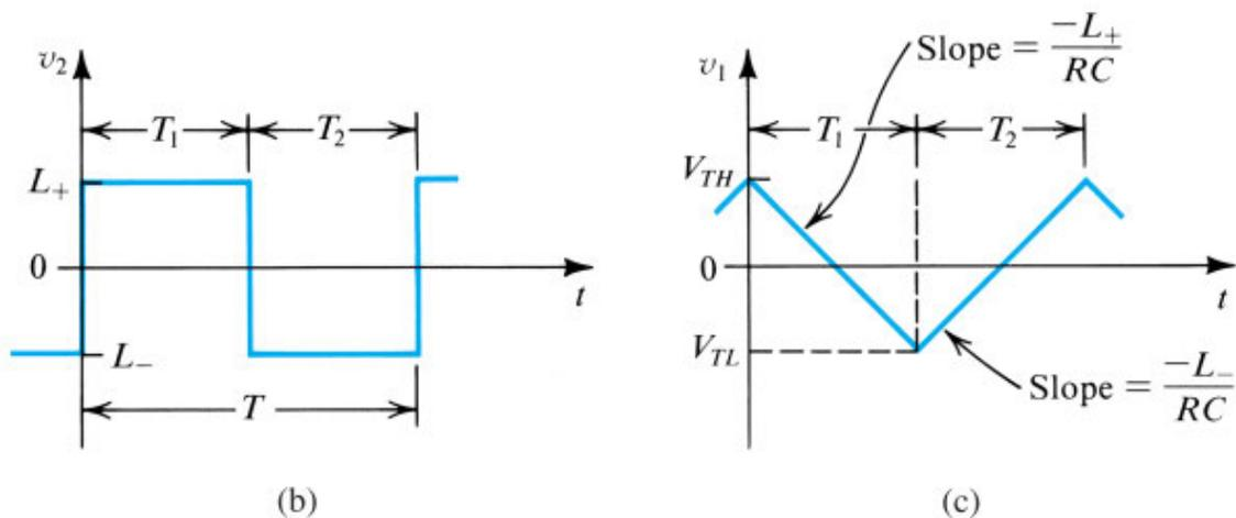
**Figure 15.24** A general scheme for generating triangular and square waveforms. The circuit in Fig. 15.22(a) can be used to implement the non-inverting bistable.
