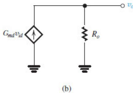
Figure 9.35 (b) Small-signal equivalent circuit of the amplifier output when a differential signal  $v_{id} \equiv v_{B1} - v_{B2}$  is applied.
