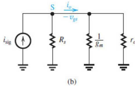
**Figure 8.20 (b)** A simplified version of the circuit in (a).
