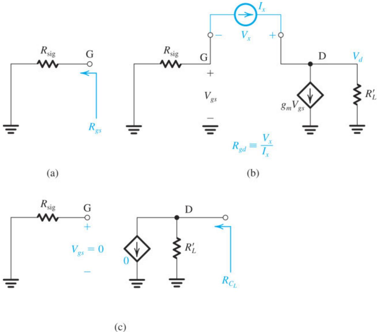
**Figure 10.17** Application of the open-circuit time-constants method to the CS equivalent circuit of Fig. 10.16.
