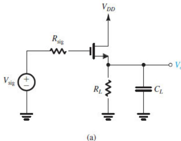
Figure 10.23 (a) A directly coupled source follower without the bias detail.
