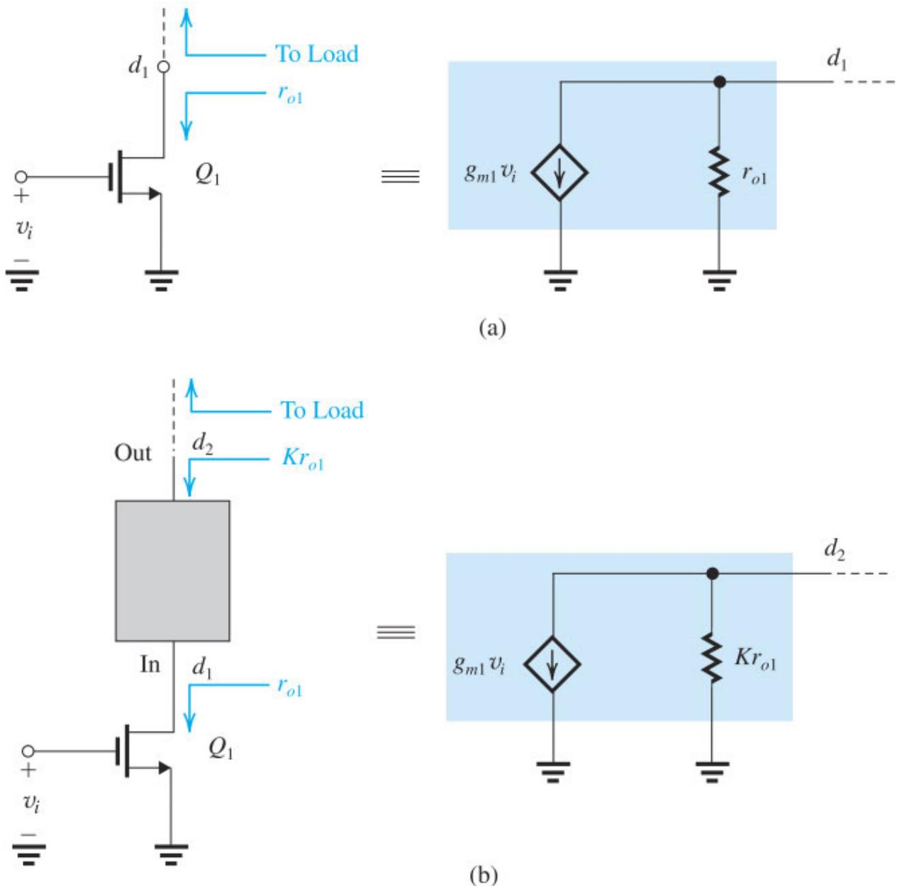
**Figure 8.17** To increase the voltage gain realized in the basic gain cell shown in (a), a functional block, shown as a black box in (b), is connected between  $d_1$  and the load. This new block is required to pass the current  $g_{m1}v_i$  right through but raise the resistance level by a factor  $K$ . The functional block is a current buffer and can be realized with a common-gate transistor, as demonstrated in the next section.
