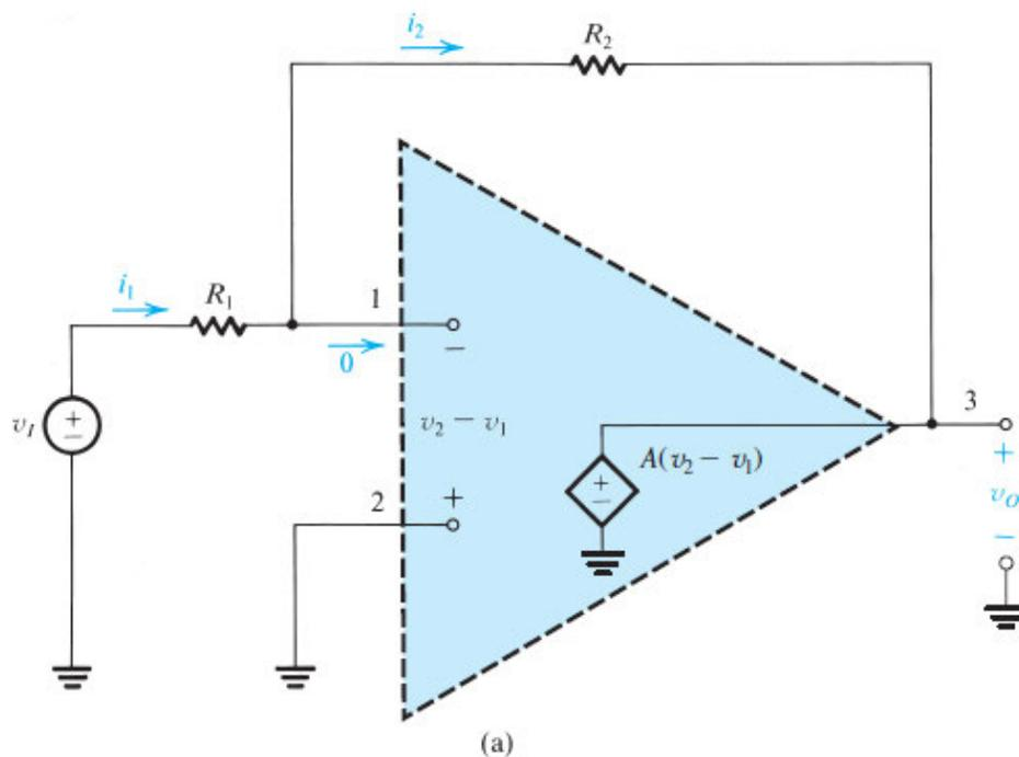
Figure 2.6 (a) Analysis of the inverting configuration.
