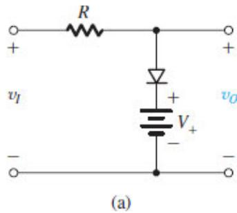
**Figure 4.5 (a)** A simple limiter circuit.
