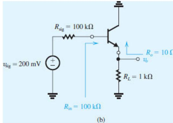
Figure 7.47 (b) Circuit for Example 7.10.
