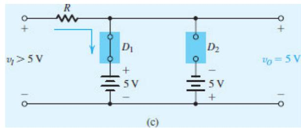
Figure 4.6 (c) The equivalent circuit when  $v_I > 5$  V.
