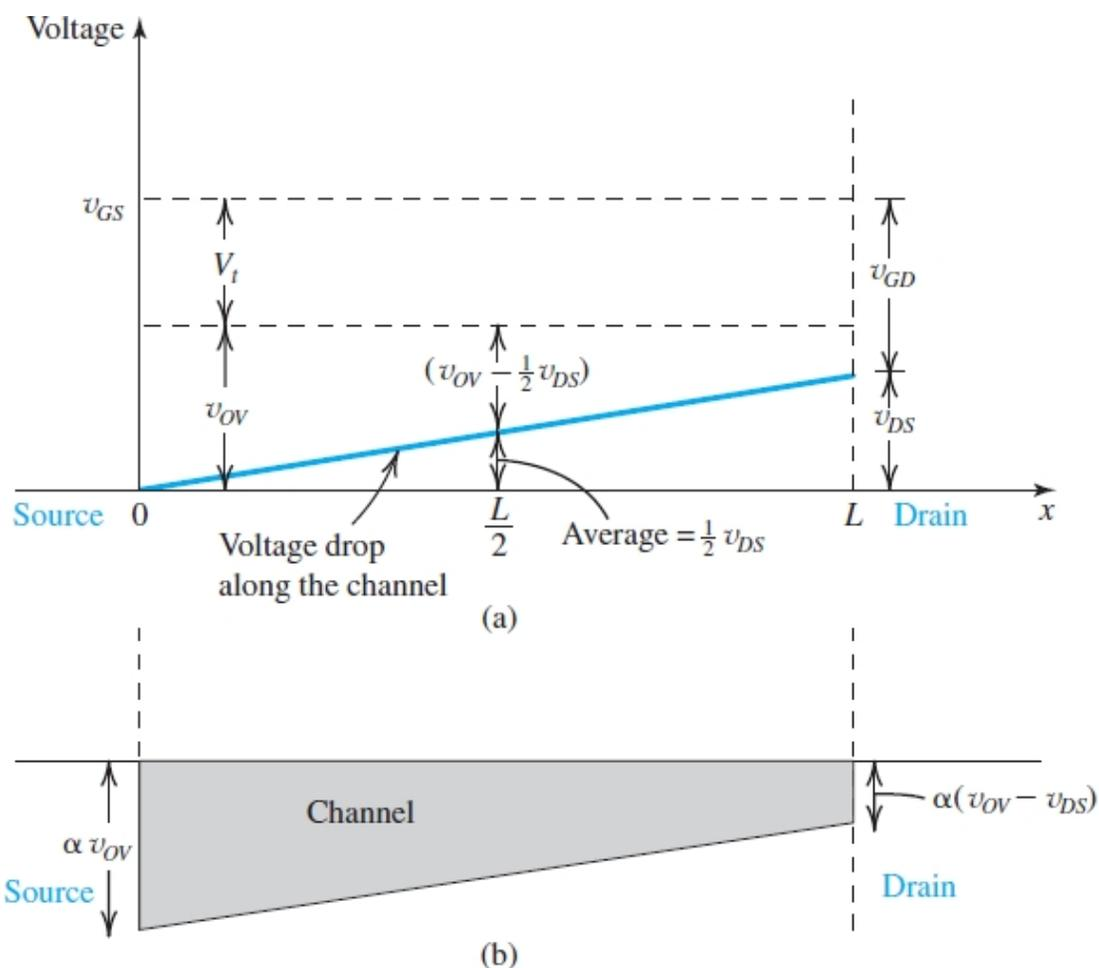
**Figure 5.6 (a)** For a MOSFET with  $v_{GS} = V_t + v_{OV}$ , applying of  $v_{DS}$  causes the voltage drop along the channel to vary linearly, with an average value of  $\frac{1}{2} v_{DS}$  at the midpoint. Since  $v_{GD} > V_t$ , the channel still exists at the drain end. **(b)** The channel shape corresponding to the situation in **(a)**. While the depth of the channel at the source end is still proportional to  $v_{OV}$ , that at the drain end is proportional to  $(v_{OV} - v_{DS})$ .
