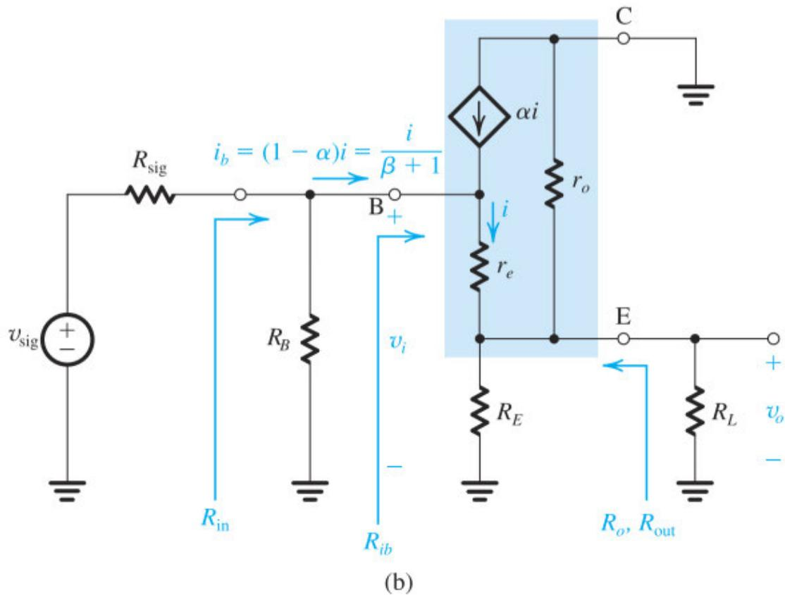
**Figure 7.61 (b)** Small-signal equivalent circuit of the emitter follower with the transistor replaced by its T model. Note that  $r_o$  is included because it is easy to do so. Normally, its effect on performance is small.
