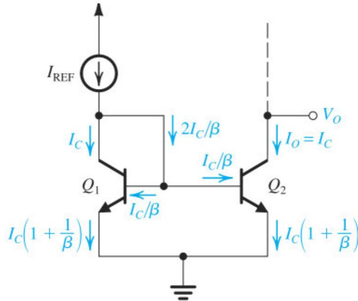
**Figure 8.8** Analysis of the current mirror taking into account the finite  $\beta$  of the BJTs.
