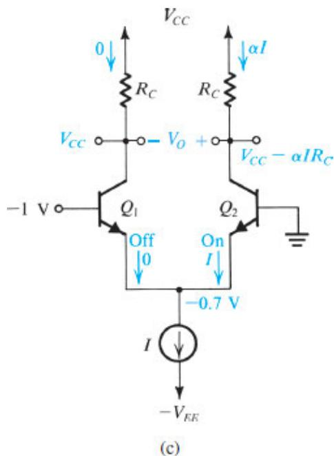
**Figure 9.15 (c)** Different modes of operation of the BJT differential pair: the differential pair with a large differential input signal of polarity opposite to that in (b).
