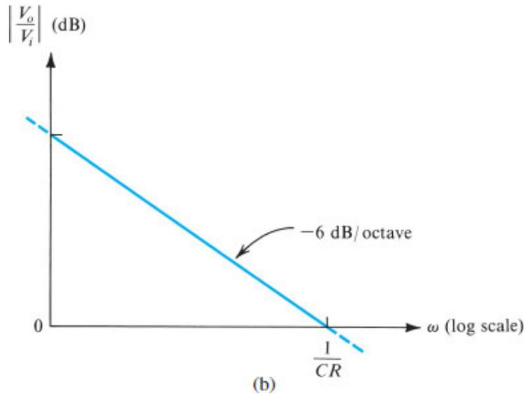
**Figure 2.24 (b)** Frequency response of the integrator.
