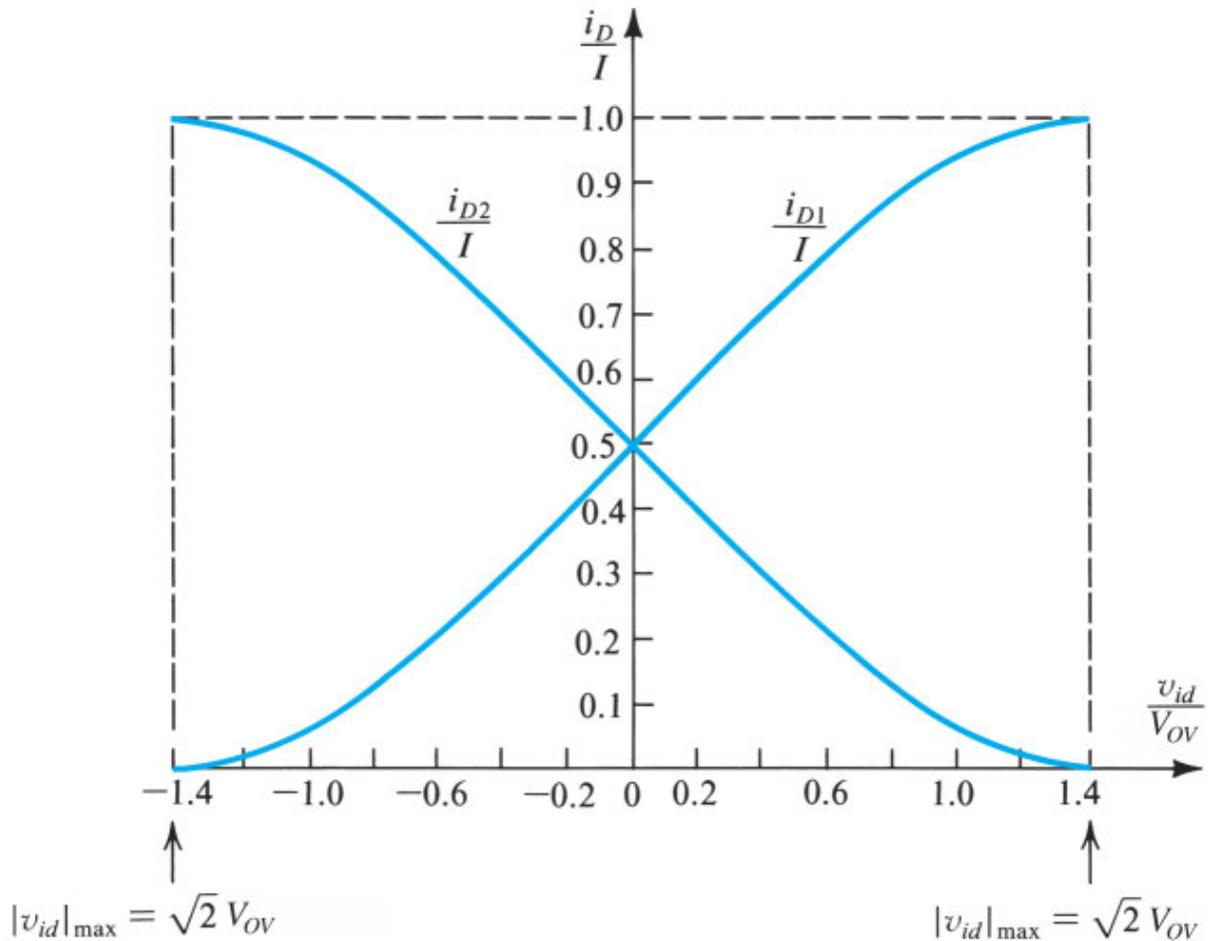
**Figure 9.6** Normalized plots of the currents in a MOSFET differential pair. Note that  $V_{OV}$  is the overdrive voltage at which  $Q_1$  and  $Q_2$  operate when conducting drain currents equal to  $I/2$ , the equilibrium situation. These graphs are universal and apply to any MOS differential pair.
