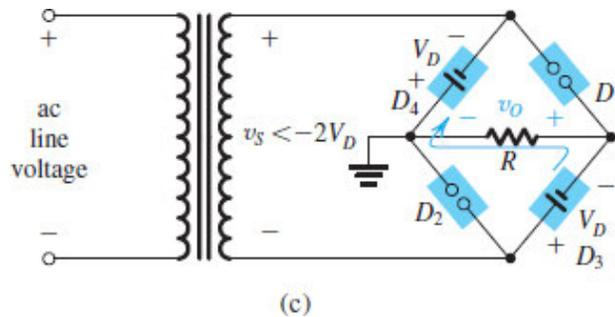
**Figure 4.23 (c)** The bridge rectifier: the equivalent circuit during negative half-cycles.
