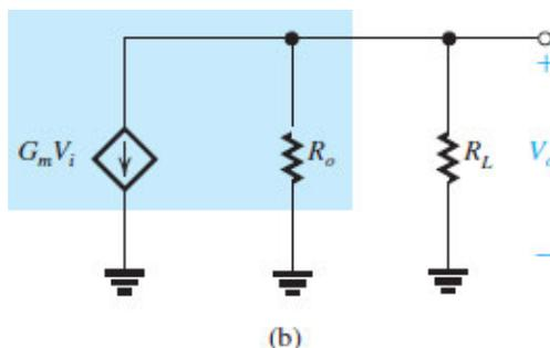
**Figure 10.30 (b)** Equivalent-circuit representation of the amplifier output.
