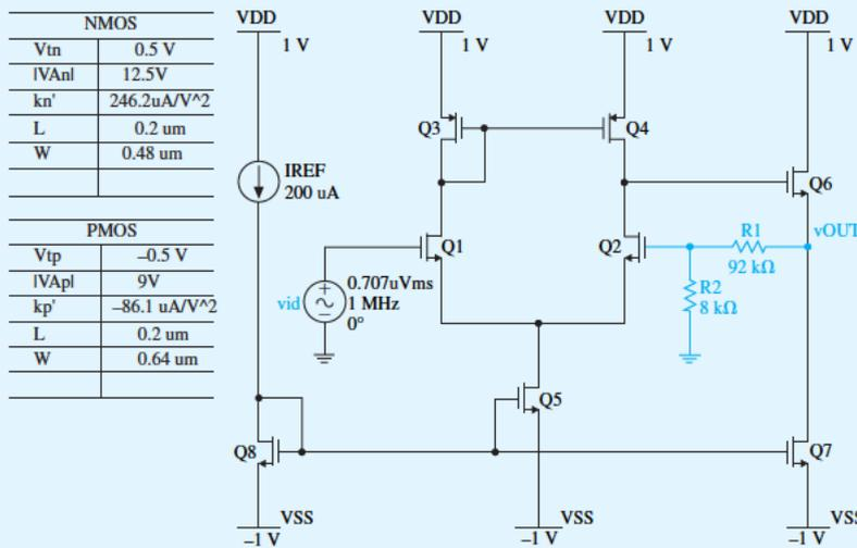
Figure B.52 Schematic capture of the closed-loop circuit.
