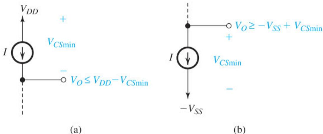
**Figure 8.6** (a) A current source; and (b) a current sink.
