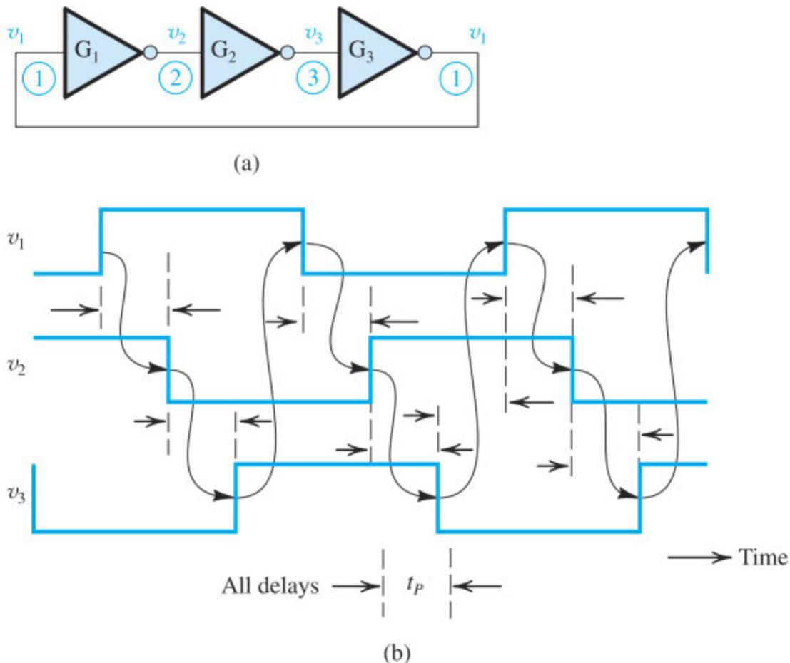
**Figure 18.32 (a)** A ring oscillator formed by connecting three inverters in cascade. (Normally at least five inverters are used.) **(b)** The resulting waveform. Observe that the circuit oscillates with frequency  $1/6t_p$ .
