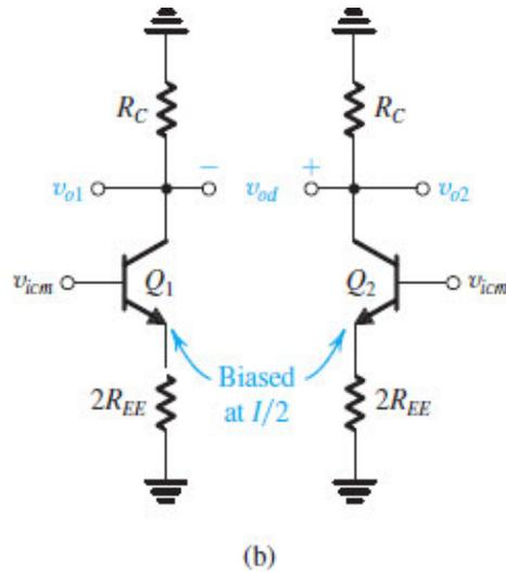
**Figure 9.25 (b)** Equivalent “half-circuits” for common-mode calculations.
