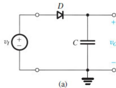
**Figure 4.24 (a)** A simple circuit used to illustrate the effect of a filter capacitor.
