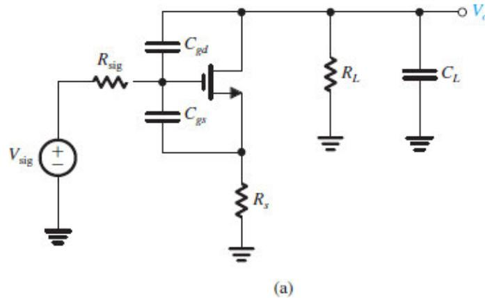
**Figure 10.31 (a)** The source-degenerated CS amplifier with all capacitances shown.
