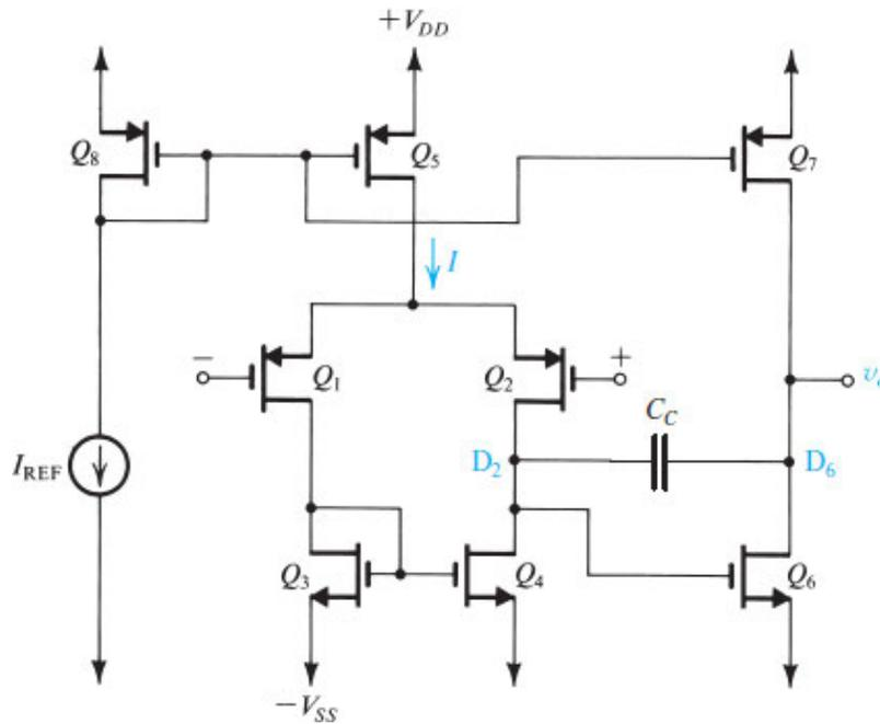
**Figure 9.37** Two-stage CMOS op-amp configuration.
