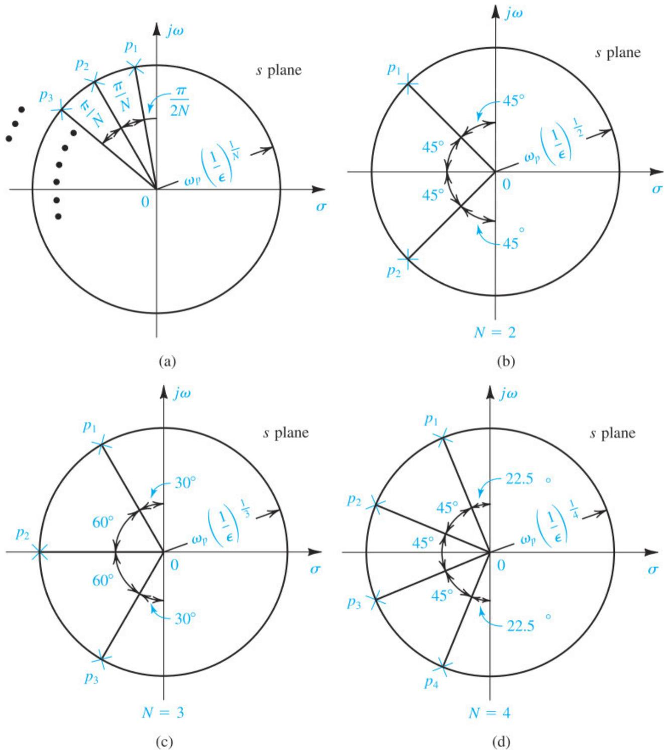
**Figure 14.15** Graphical construction for determining the poles of a Butterworth filter of order  $N$ . All the poles lie in the left half of the  $s$  plane on a circle of radius  $\omega_0 = \omega_p(1/\epsilon)^{1/N}$ , where  $\epsilon$  is the passband deviation parameter ( $\epsilon = \sqrt{10^{A_{\max}/10} - 1}$ ): (a) the general case; (b)  $N = 2$ ; (c)  $N = 3$ ; (d)  $N = 4$ .
