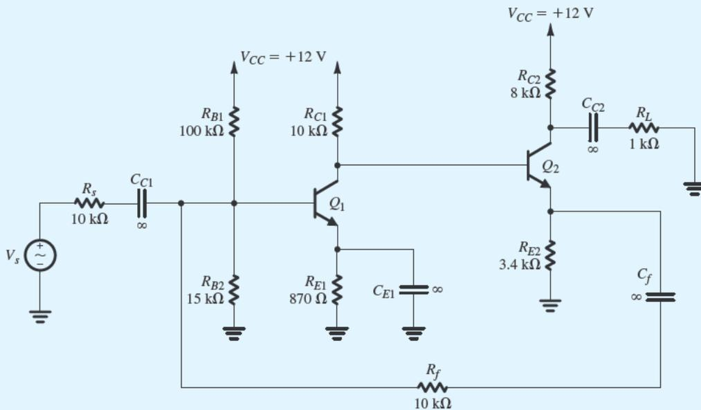
**Figure B.43** Circuit of the shunt–series feedback amplifier in Example S.11.1.
