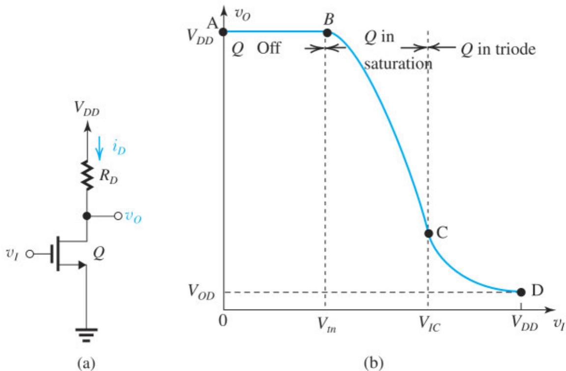
**Figure 16.12** The simple resistively loaded MOS amplifier can be used as a logic inverter when operated in cutoff ( $v_I < V_m$ ) and in triode ( $v_I > V_{IC}$ ). The output high level is  $V_{DD}$  and the low level is  $V_{OD}$ .
