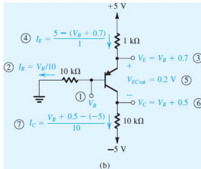
Figure 6.28 (b) Example 6.9: analysis with steps numbered.
