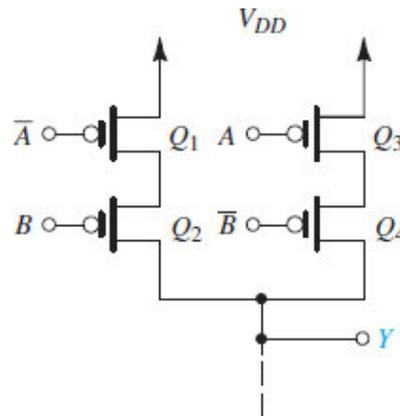
**Figure 16.10 (a)** Realization of the exclusive-OR (XOR) function. (a) The PUN synthesized directly from the expression in Eq. (16.5).
