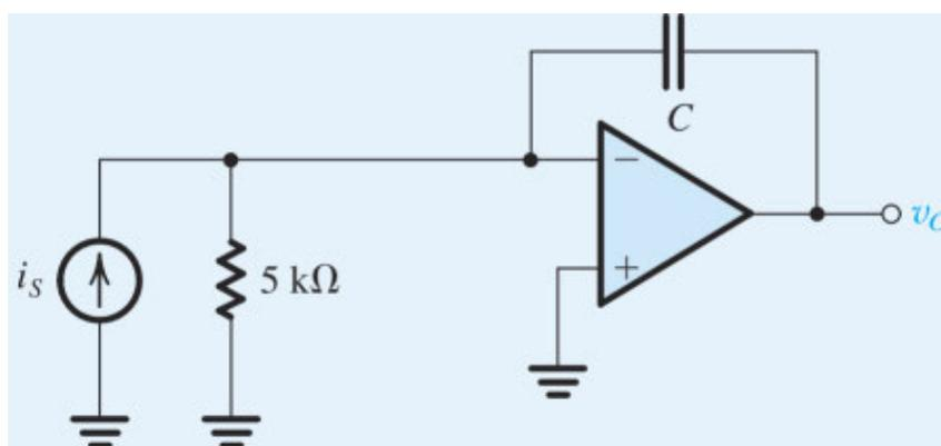
Figure 2.25 The integrator with input current source (Example 2.5).
