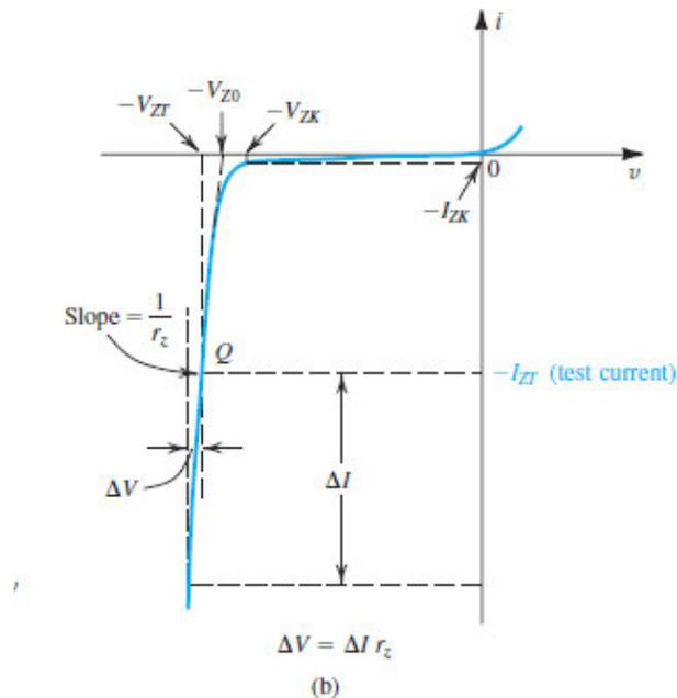
**Figure 4.13 (b)** The diode  $i-v$  characteristic with the breakdown region shown in some detail.
