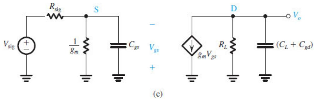
Figure 10.18 (c) Equivalent circuit for the case in which  $r_o$  is neglected.
