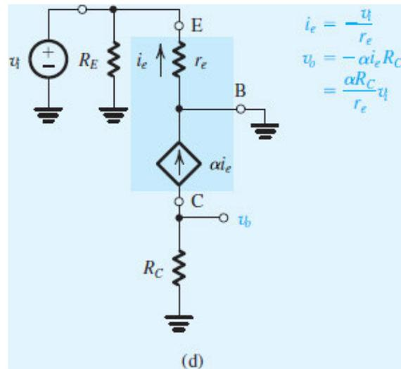
**Figure 7.31 (d)** Example 7.7: small-signal analysis using the T model for the BJT.
