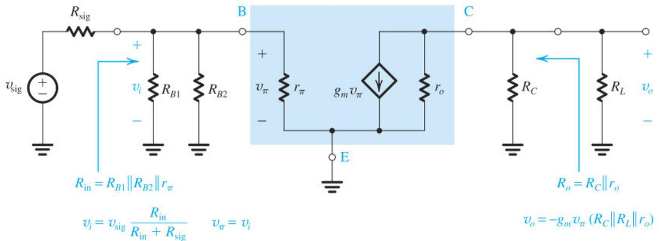
**Figure 7.58 (b)** Equivalent circuit and analysis.
