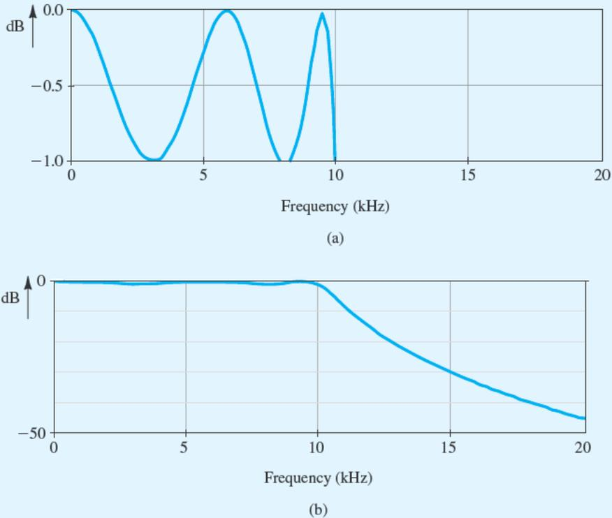
**Figure B.67** Magnitude response of the fifth-order lowpass filter circuit shown in Fig. B.66: (a) an expanded view of the passband region; (b) a view of both the passband and stopband regions.
