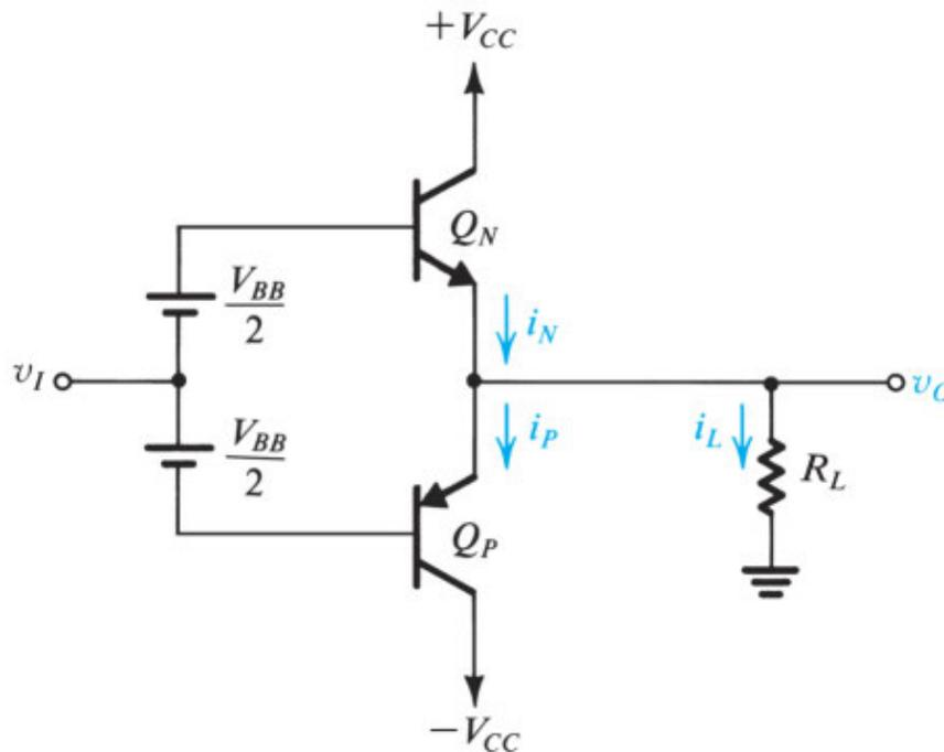
**Figure 12.10** Class AB output stage. A bias voltage  $V_{BB}$  is applied between the bases of  $Q_N$  and  $Q_P$ , giving rise to a bias current  $I_Q$  given by Eq. (12.23). Thus, for small  $v_I$ , both transistors conduct and crossover distortion is almost completely eliminated.
