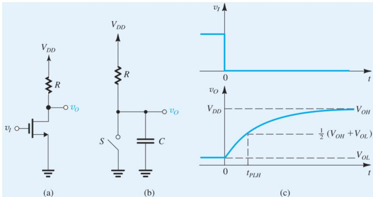
**Figure 17.2** Example 17.1: **(a)** Inverter schematic circuit. **(b)** The inverter circuit after  $v_I$  goes low and the switch opens (i.e., for  $t > 0$ ). **(c)** Waveforms of  $v_I$  and  $v_O$ . Observe that the switch is assumed to operate instantaneously.  $v_O$  rises exponentially, starting at  $V_{OL}$  and heading toward  $V_{OH}$ .
