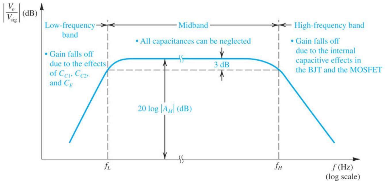
**Figure 7.62** Sketch of the magnitude of the gain of a CS (Fig. 7.57) or CE (Fig. 7.58) amplifier versus frequency. The graph delineates the three frequency bands relevant to frequency-response determination.
