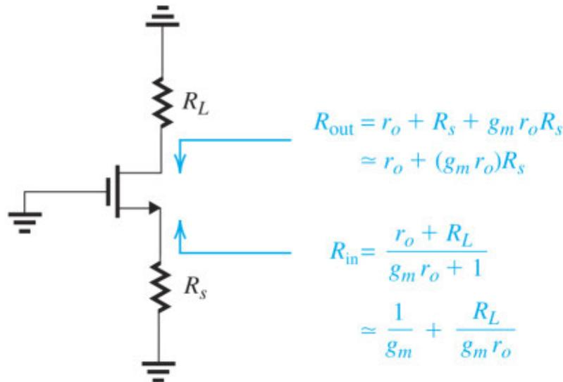
**Figure 8.22** The impedance transformation properties of the common-gate amplifier. Depending on the values of  $R_s$  and  $R_L$ , we can sometimes write  $R_{\text{in}} \simeq R_L / (g_m r_o)$  and  $R_o \simeq (g_m r_o) R_s$ . However, such approximations are not always justified.
