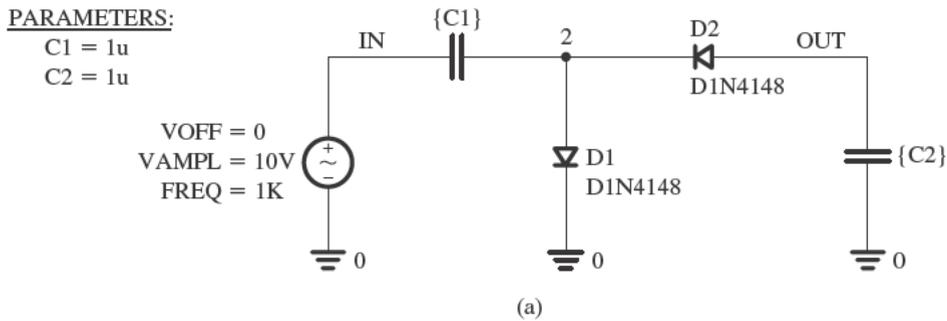
**Figure EB.16** (a) Schematic capture of the voltage-doubler circuit in Exercise B.1. (b) Various voltage waveforms in the voltage-doubler circuit. The top graph displays the input sine-wave voltage signal, the middle graph displays the voltage across diode  $D_1$ , and the bottom graph displays the voltage that appears at the output.
