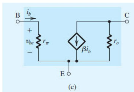
**Figure 1.19 (c)** An alternative small-signal circuit model for the BJT.
