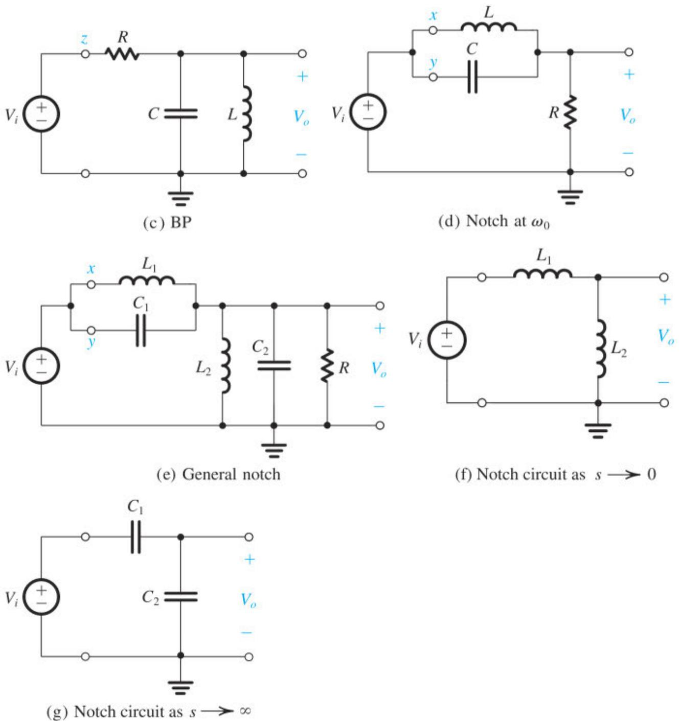
**Figure 14.19** Realization of various second-order filter functions using the LCR resonator of Fig. 14.18(a): (a) general structure, (b) LP, (c) BP, (d) notch at  $\omega_0$ , (e) general notch, (f) notch circuit in (e) as  $s \rightarrow 0$ , (g) notch circuit in (e) as  $s \rightarrow \infty$ .
