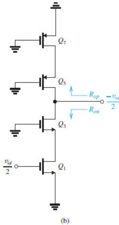
**Figure 9.13 (b)** Differential half-circuit of the cascode differential amplifier in (a).
