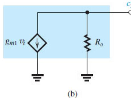
**Figure 8.33 (b)** Small-signal equivalent circuit of the output of the cascode amplifier.
