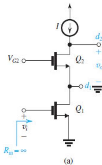
**Figure 8.28 (a)** A cascode amplifier with a constant-current source load.
