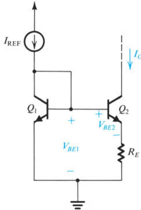
**Figure 8.39** The Widlar current source.
