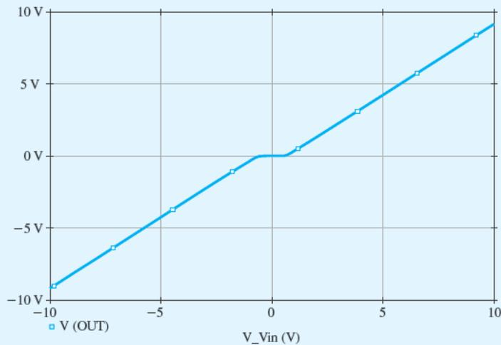
**Figure B.58** Transfer characteristic of the class B output stage of Fig. B.54.
