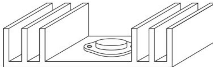
**Figure 12.26** Typical heat sink.
