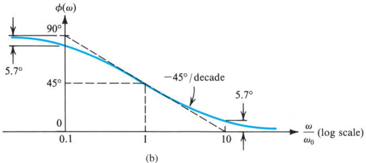
Figure 1.24 (b) Phase response of STC networks of the high-pass type.
