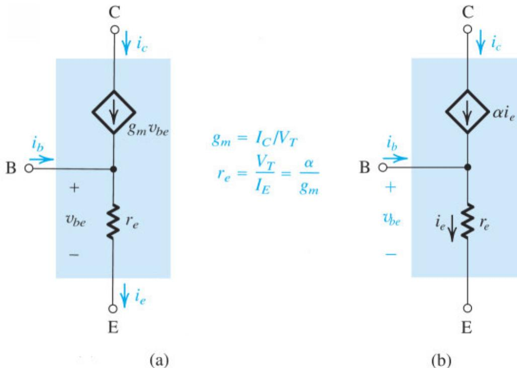
**Figure 7.27** Two slightly different versions of what is known as the *T model* of the BJT. The circuit in (a) is a voltage-controlled current source representation and that in (b) is a current-controlled current source representation. These models explicitly show the emitter resistance  $r_e$  rather than the base resistance  $r_\pi$  featured in the hybrid- $\pi$  model.
