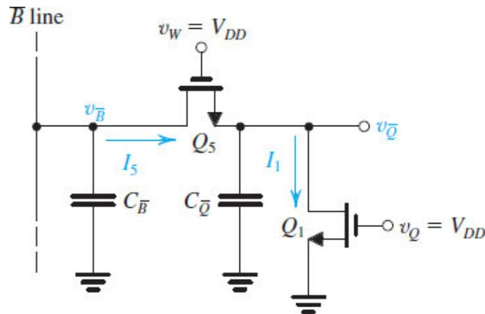
**Figure 18.23** Relevant parts of the SRAM cell circuit during a read operation when the cell is storing a logic 1. Note that initially  $v_Q = V_{DD}$  and  $v_{\bar{Q}} = 0$ . Also note that the  $B$  and  $\bar{B}$  lines are precharged to a voltage  $V_{DD}$ .
