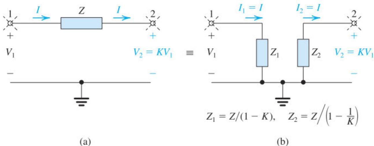
**Figure 10.14** The Miller equivalent circuit.
