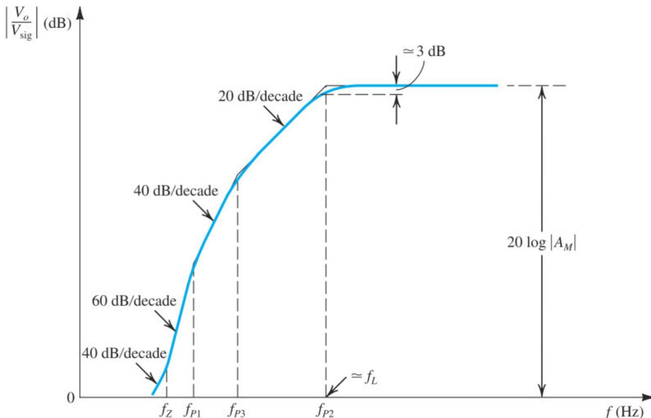
**Figure 10.39** Sketch of the low-frequency magnitude response of a CS amplifier for which the three pole frequencies are sufficiently separated for their effects to appear distinct.
