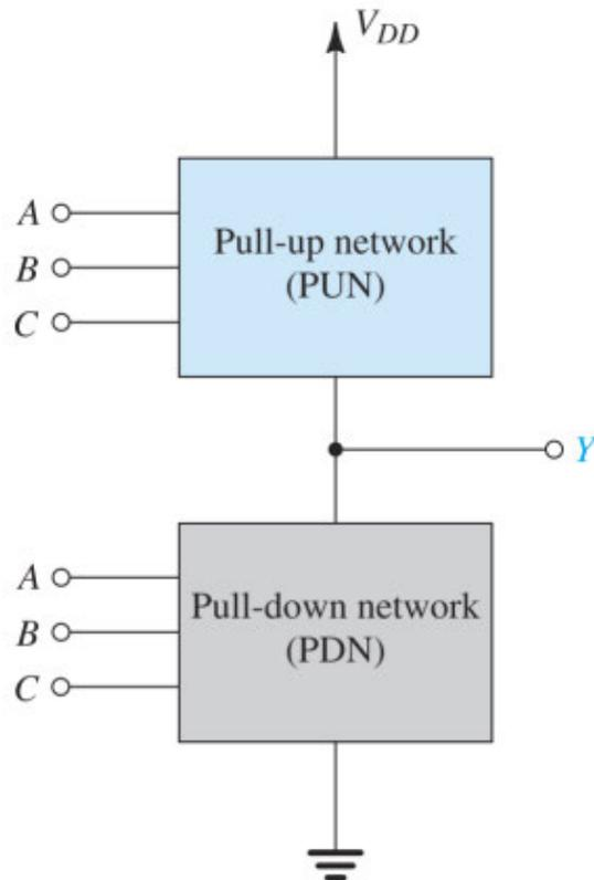
**Figure 16.3** Representation of a three-input CMOS logic gate. The PUN comprises PMOS transistors, and the PDN comprises NMOS transistors.
