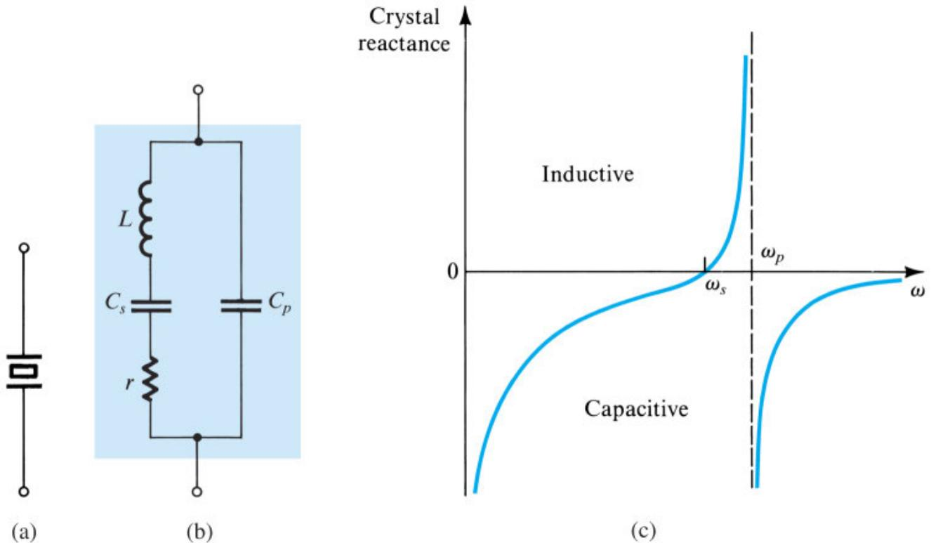
**Figure 15.17** A piezoelectric crystal. (a) Circuit symbol. (b) Equivalent circuit. (c) Crystal reactance versus frequency [note that, neglecting the small resistance  $r$ ,  $Z_{\text{crystal}} = jX(\omega)$ ].
