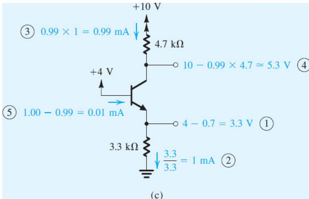
**Figure 6.23 (c)** Analysis of the circuit for Example 6.4: analysis with the steps numbered.
