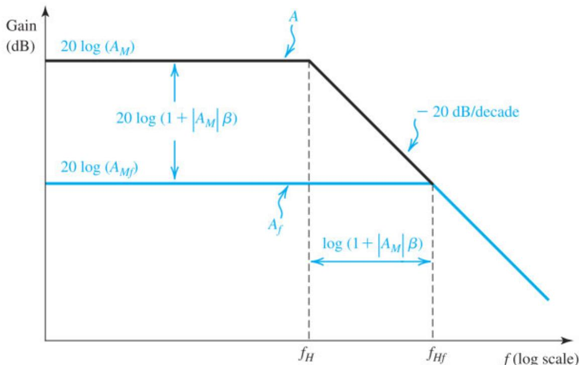
**Figure 11.5** Application of negative feedback increases the amplifier bandwidth at the expense of decreasing the midband gain. Both changes are by the factor  $(1 + |A_M|\beta)$  which is the amount of feedback. Notice that the gain–bandwidth product remains unchanged.
