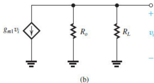
**Figure 8.29 (b)** Equivalent circuit at the amplifier output.
