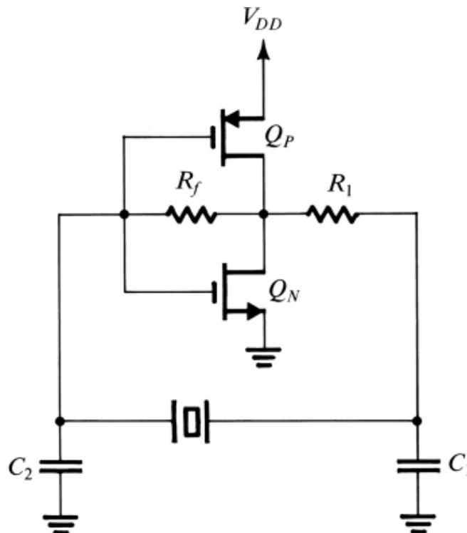
**Figure 15.18** A Pierce crystal oscillator using a CMOS inverter as an amplifier.
