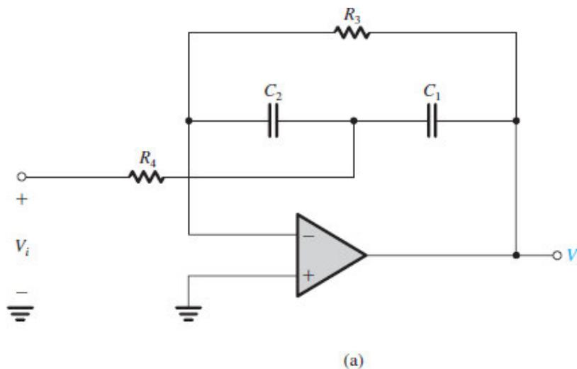
**Figure 14.27 (a)** Circuit for the realization of a second-order bandpass filter.
