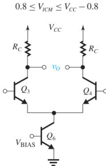
**Figure 13.17** The complement of the circuit in Fig. 13.16. While the input common-mode range of the circuit in Figure 13.16 extends below ground, here it extends above  $V_{CC}$ . Connecting the two circuits in parallel, as we will show, results in a rail-to-rail  $V_{ICM}$  range.
