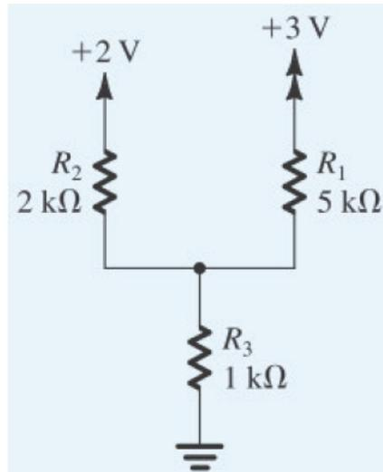
**Figure VE1.1** The circuit for Video Example 1.1.
