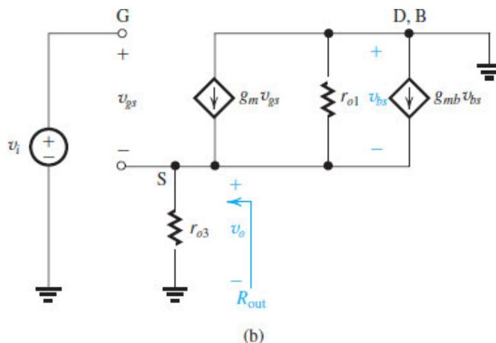
**Figure 8.35 (b)** Equivalent circuit.
