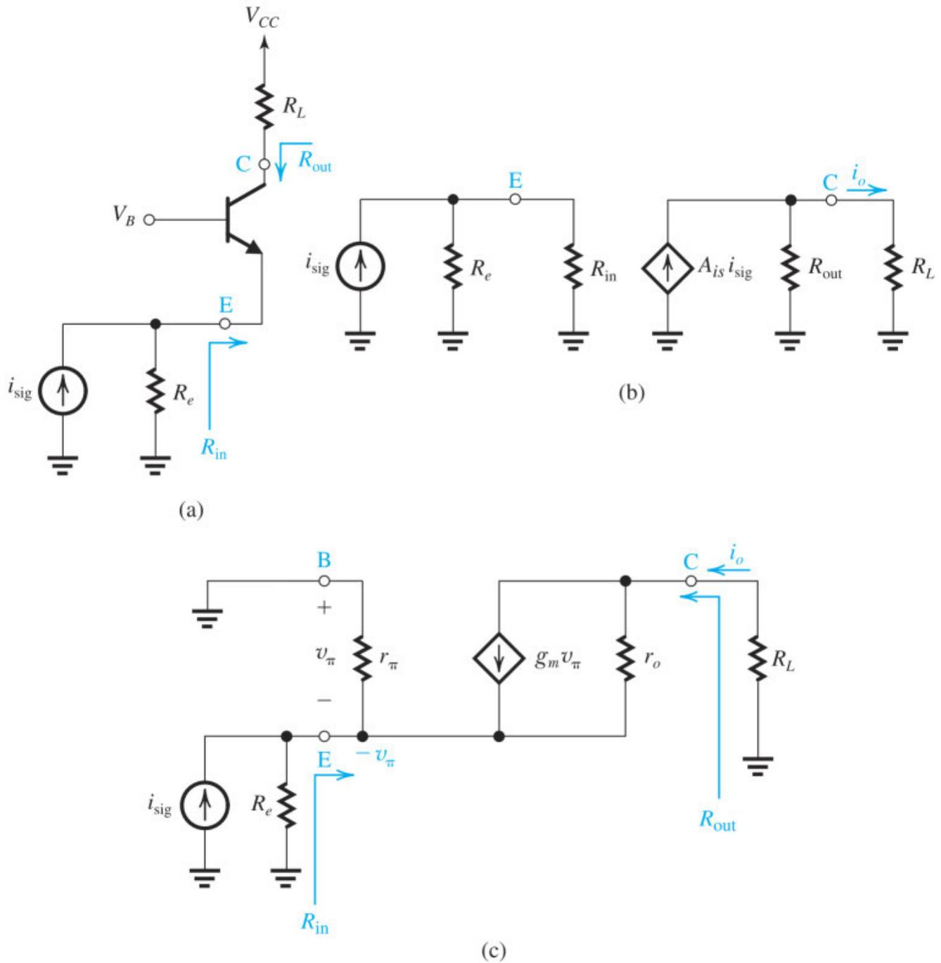
**Figure 8.25** (a) A CB amplifier. (b) Equivalent circuit model of the CB amplifier in (a). (c) The CB amplifier in (a) with the transistor replaced with its  $\pi$  model.
