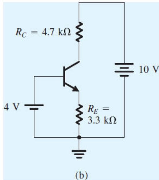
**Figure 6.23 (b)** Analysis of the circuit for Example 6.4: the circuit redrawn to show the convention used in this book to show connections to the dc sources.
