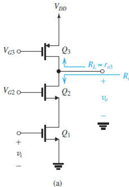
**Figure 8.29 (a)** A MOS cascode amplifier loaded in a simple PMOS current source  $Q_3$ .
