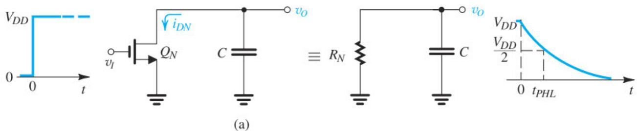
**Figure 17.5 (a)** Equivalent circuit for determining the propagation delays  $t_{PHL}$  of the inverter.
