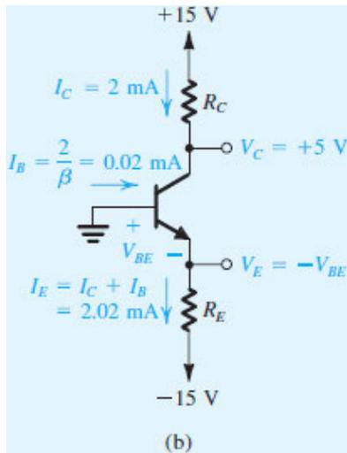
**Figure 6.15 (b)** Circuit for Example 6.2.
