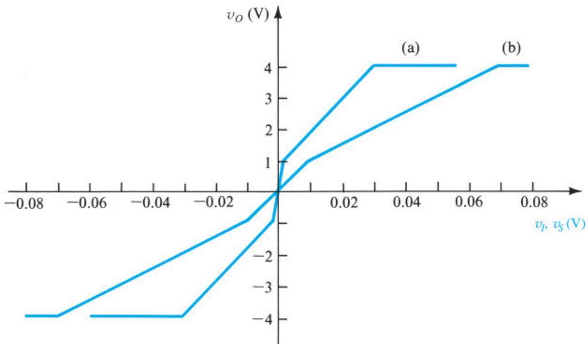
**Figure 11.6** Illustrating the application of negative feedback to reduce the nonlinear distortion in amplifiers. Curve (a) shows the amplifier transfer characteristic ( $v_O$  versus  $v_I$ ) without feedback. Curve (b) shows the characteristic ( $v_O$  versus  $v_S$ ) with negative feedback ( $\beta = 0.01$ ) applied.
