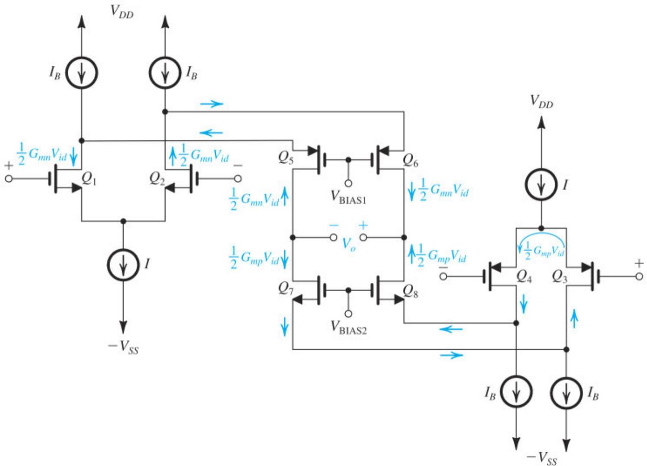
**Figure 13.12** A folded-cascode op amp that employs two parallel complementary input stages to achieve rail-to-rail input common-mode operation. Note that the two “+” terminals are connected together and the two “-” terminals are connected together.
