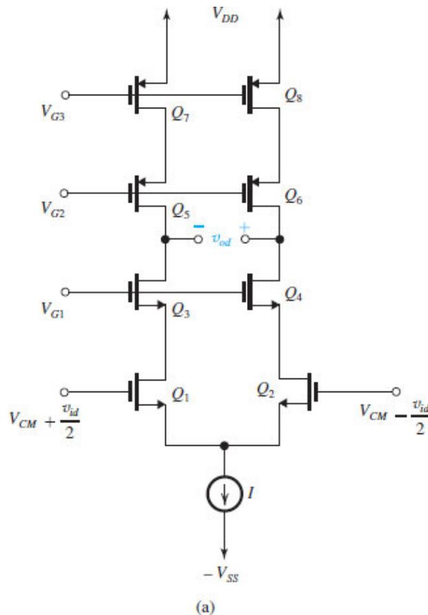
Figure 9.13 (a) Cascode differential amplifier.
