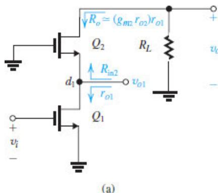
**Figure 8.32 (a)** The cascode amplifier with a load resistance  $R_L$ . Only signal quantities are shown.
