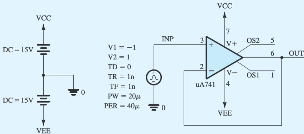
Figure B.11 Circuit for determining the slew rate of the  $\mu$ A741 op amp in Example S.2.2.
