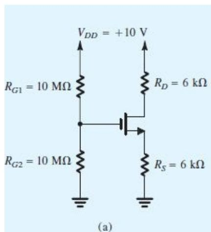
Figure 5.24 (a) Circuit for Example 5.6.
