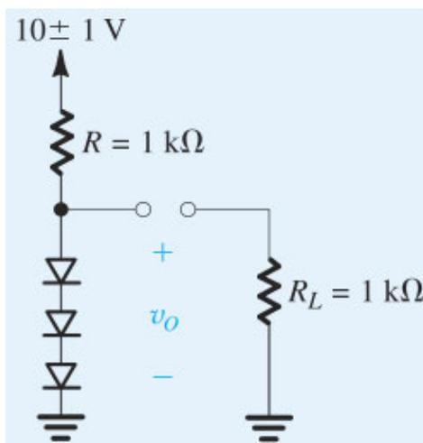
**Figure 4.18** Circuit for Example 4.6.
