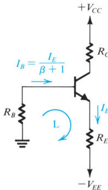
**Figure 7.55** Biasing the BJT using two power supplies. Resistor  $R_B$  is needed only if the signal is to be capacitively coupled to the base. Otherwise, the base can be connected directly to ground, or to a grounded signal source, resulting in almost total  $\beta$ -independence of the bias current.
