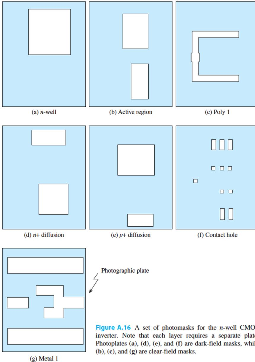
**Figure A.16** A set of photomasks for the  $n$ -well CMOS inverter. Note that each layer requires a separate plate. Photoplates (a), (d), (e), and (f) are dark-field masks, while (b), (c), and (g) are clear-field masks.
