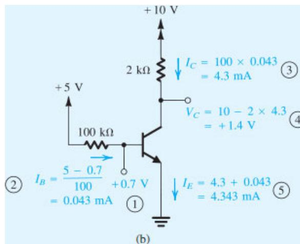
Figure 6.27 (b) Example 6.8: analysis with steps numbered.
