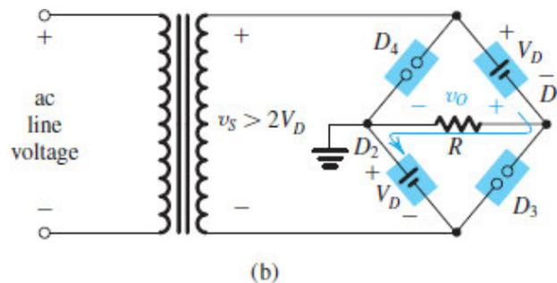
**Figure 4.23 (b)** The bridge rectifier: the equivalent circuit during positive half-cycles.
