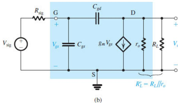
Figure 10.11 (b) Equivalent circuit of (a).
