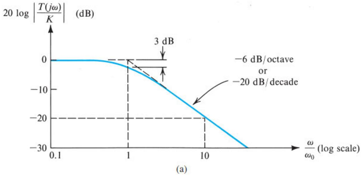
Figure 1.23 (a) Magnitude of STC networks of the low-pass type.
