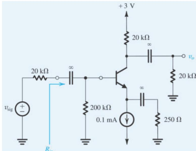
Figure VE7.4 Circuit for Video Example 7.4.
