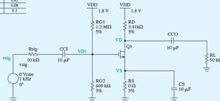
**Figure B.23** Capture schematic of the CS amplifier.
