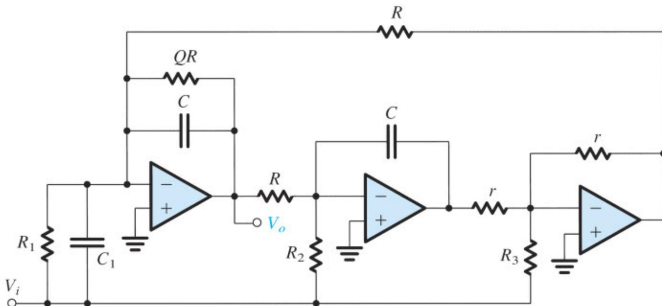
**Figure 14.26** The Tow–Thomas biquad with feedforward. The transfer function of Eq. (14.70) is realized by feeding the input signal through appropriate components to the inputs of the three op amps. This circuit can realize all special second-order functions. The design equations are given in Table H.2 in Appendix H on the website.
