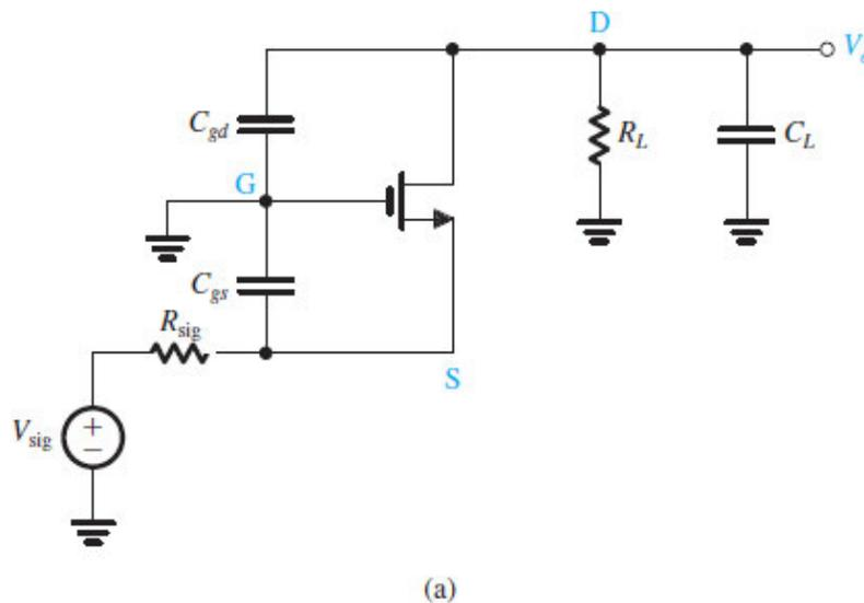
**Figure 10.18 (a)** The common-gate amplifier with the transistor internal capacitances shown. A load capacitance  $C_L$  is also included.
