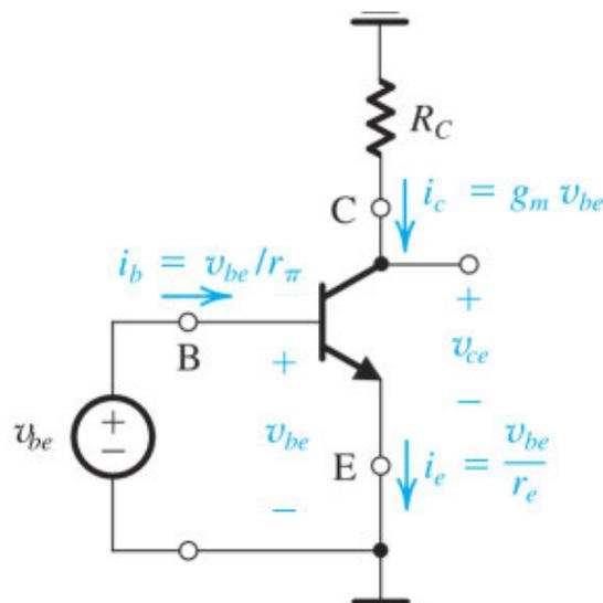
**Figure 7.24** The amplifier circuit of Fig. 7.21(a) with the dc sources ( $V_{BE}$  and  $V_{CC}$ ) eliminated (short-circuited). Thus only the signal components are present. Note that this is a representation of the signal operation of the BJT and not an actual amplifier circuit.
