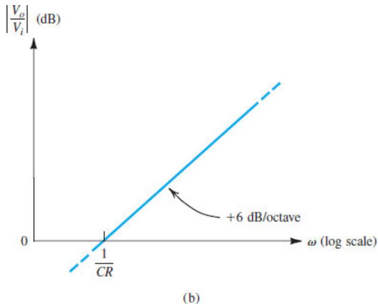
Figure 2.28 (b) Frequency response of a differentiator with a time constant  $CR$ .
