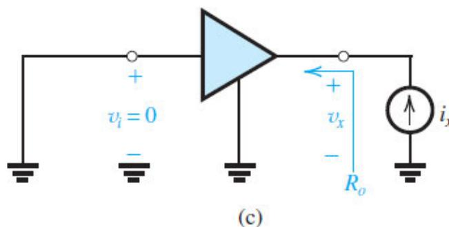
Figure 7.35 (c) Characterization of the amplifier as a functional block: determining the amplifier output resistance  $R_o$ .
