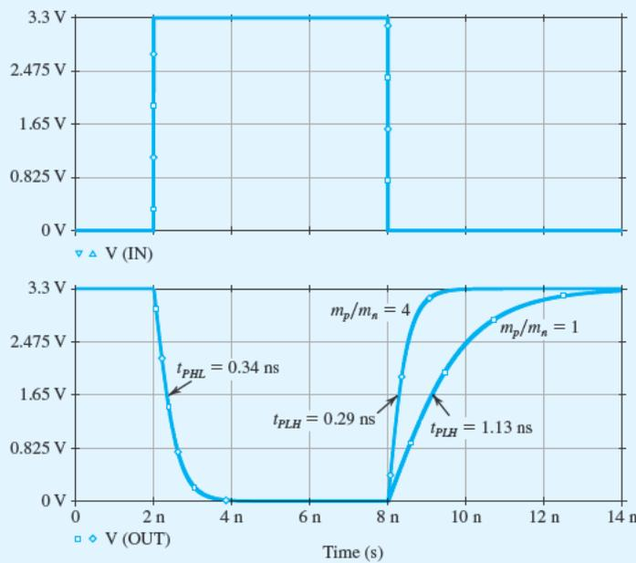
**Figure B.79** Transient response of the CMOS inverter in Example S.16.1 with  $m_p/m_n = 1$  and  $m_p/m_n = 4$ .
