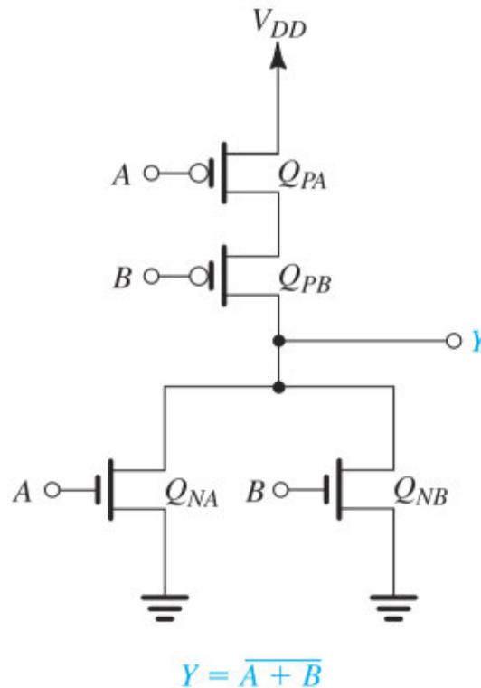
**Figure 16.7** A two-input CMOS NOR gate.
