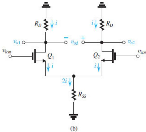
Figure 9.24 (b) The amplifier circuit prepared for small-signal analysis.
