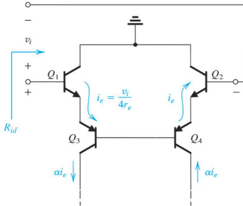
**Figure 13.24** Small-signal analysis of the 741 input stage.
