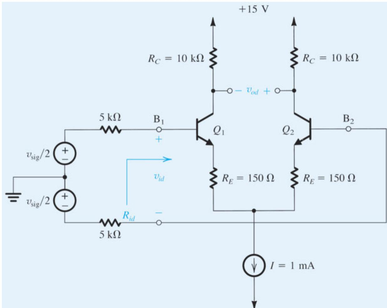
Figure 9.23 Circuit for Example 9.3.
