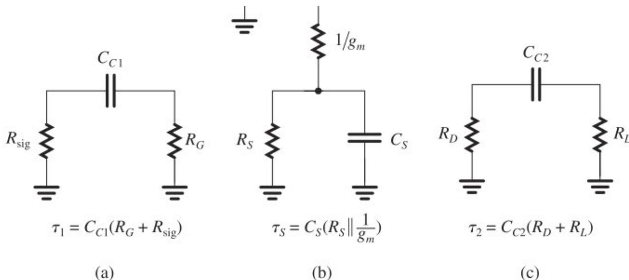
**Figure 10.40** Circuits for determining the time constant of each of the three capacitors, and hence the pole associated with each one. Note that this determination is possible because in the circuit of Fig. 10.37, the capacitors do not interact; that is, each is responsible for only one of the three poles (and zeros).
