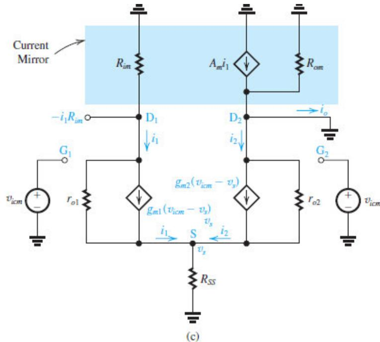
**Figure 9.36 (c)** Analysis of the current-mirror-loaded MOS differential amplifier to determine its common-mode gain: Circuit for determining  $G_{mcm}$ .
