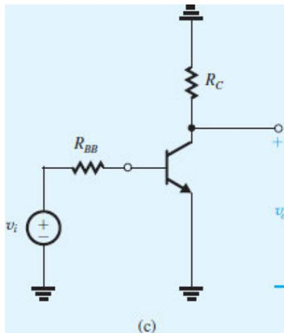
Figure 7.29 (c) Example 7.5: amplifier circuit with dc sources replaced by short circuits.
