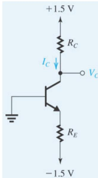
Figure VE6.1 Circuit for Video Example 6.1.
