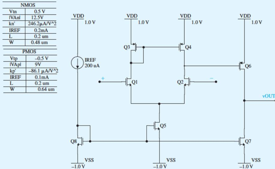
Figure B.33 Schematic capture of the two-stage CMOS op amp.
