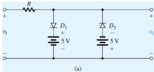
Figure 4.6 (a) Simple limiter circuit in Example 4.2.
