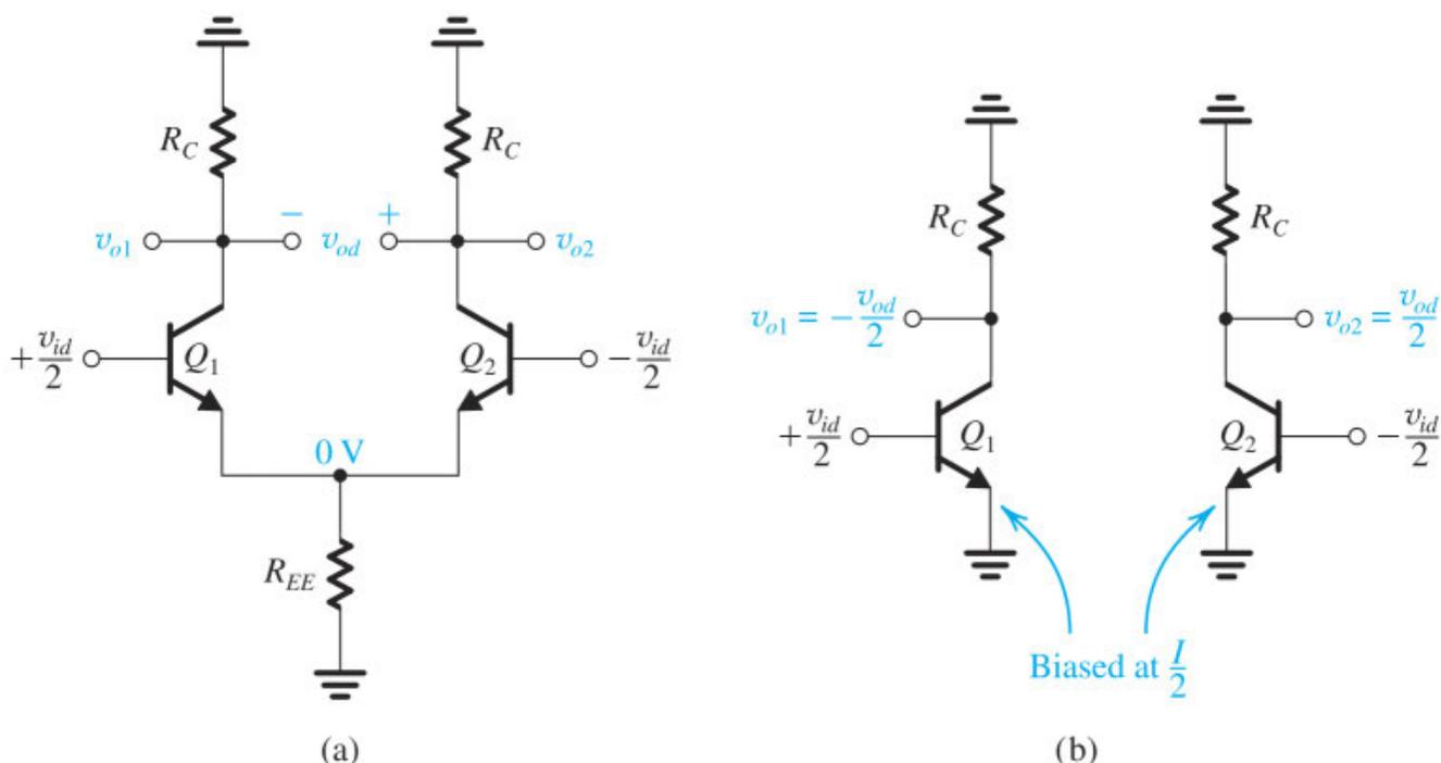
**Figure 9.21** Equivalence of the BJT differential amplifier in (a) to the two common-emitter amplifiers in (b). This equivalence applies only for differential input signals. Either of the two common-emitter amplifiers in (b) can be used to find the differential gain, differential input resistance, frequency response, and so on, of the differential amplifier.
