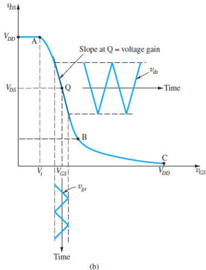
**Figure 7.4 (b)** The MOSFET operates on a short, almost-linear segment of the VTC around the bias point Q and provides an output voltage  $v_{ds} = A_v v_{gs}$ .
