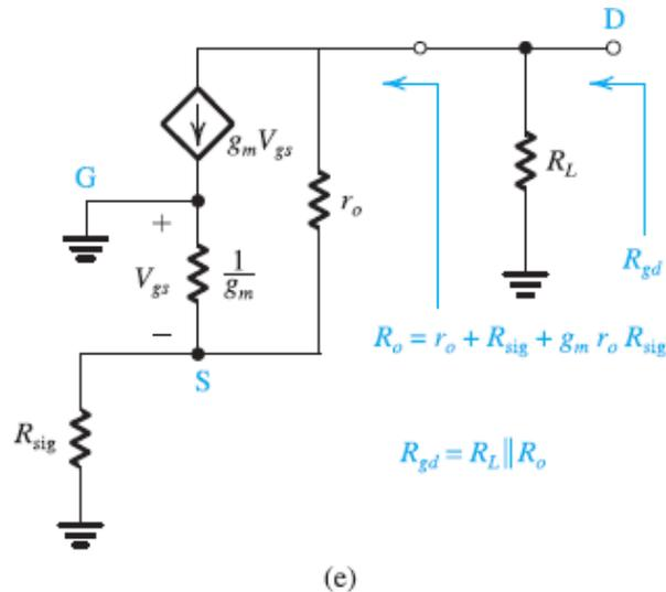
**Figure 10.18 (e)** Circuit for determining the resistance  $R_{gd}$  seen by  $(C_L + C_{gd})$ .
