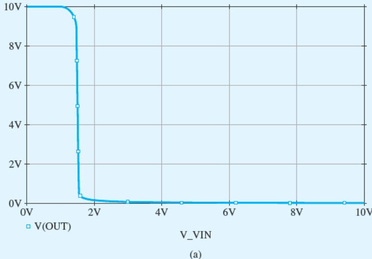
**Figure B.28** (a) Voltage transfer characteristic of the CS amplifier in Example S.8.1. (b) Expanded view of the transfer characteristic in the high-gain region. Also shown are the transfer characteristics where process variations cause the width of transistor  $M_1$  to change by  $+15\%$  and  $-15\%$  from its nominal value of  $W_1 = 12.5 \mu\text{m}$ .
