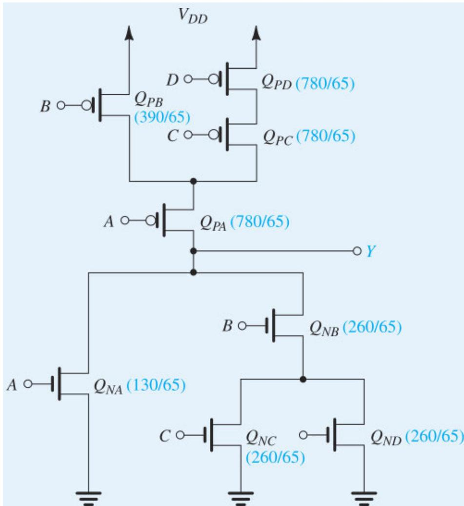
Figure 17.10 Circuit for Example 17.4.
