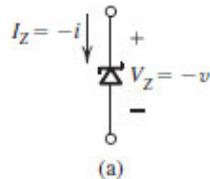
**Figure 4.13 (a)** Circuit symbol for the zener diode.
