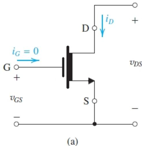
**Figure 5.29 (a)** The circuit symbol for an  $n$ -channel depletion-type MOSFET. Note that  $I_{DSS}$  denotes the drain current when  $v_{GS} = 0$ .
