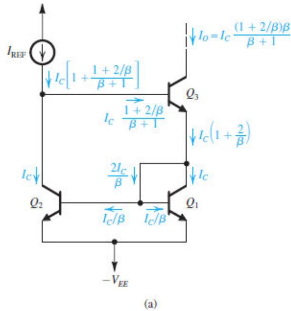
**Figure 8.37 (a)** The Wilson bipolar current mirror: circuit showing analysis to determine the current transfer ratio.
