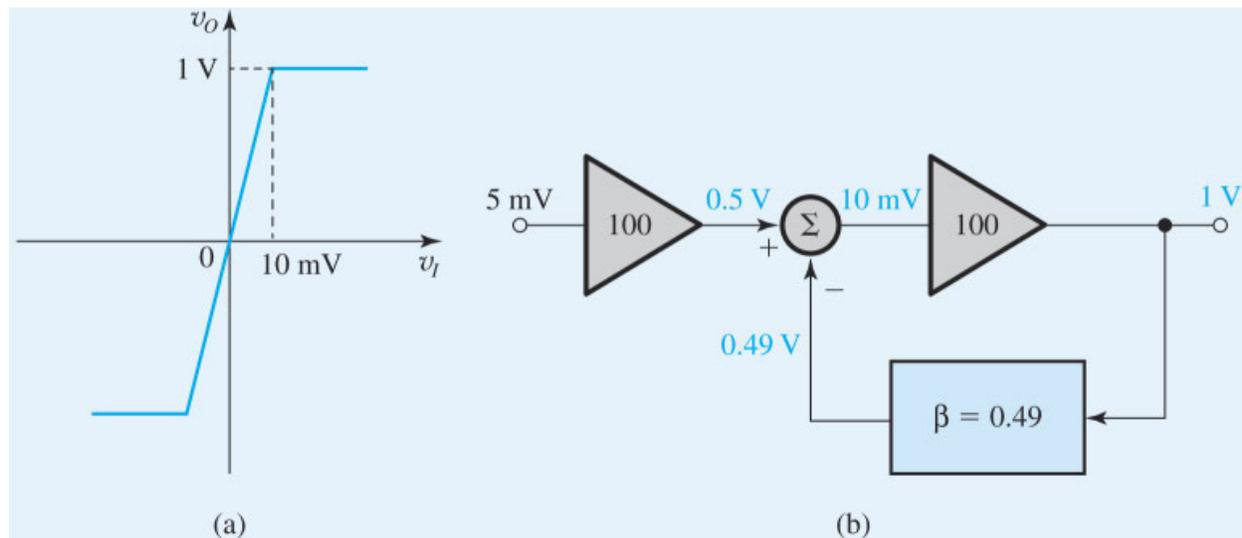
**Figure 11.7** (a) Transfer characteristic of available amplifier. (b) Block diagram of an amplifier with a gain of 200 V/V that is linear for input signals as large as 5 mV.
