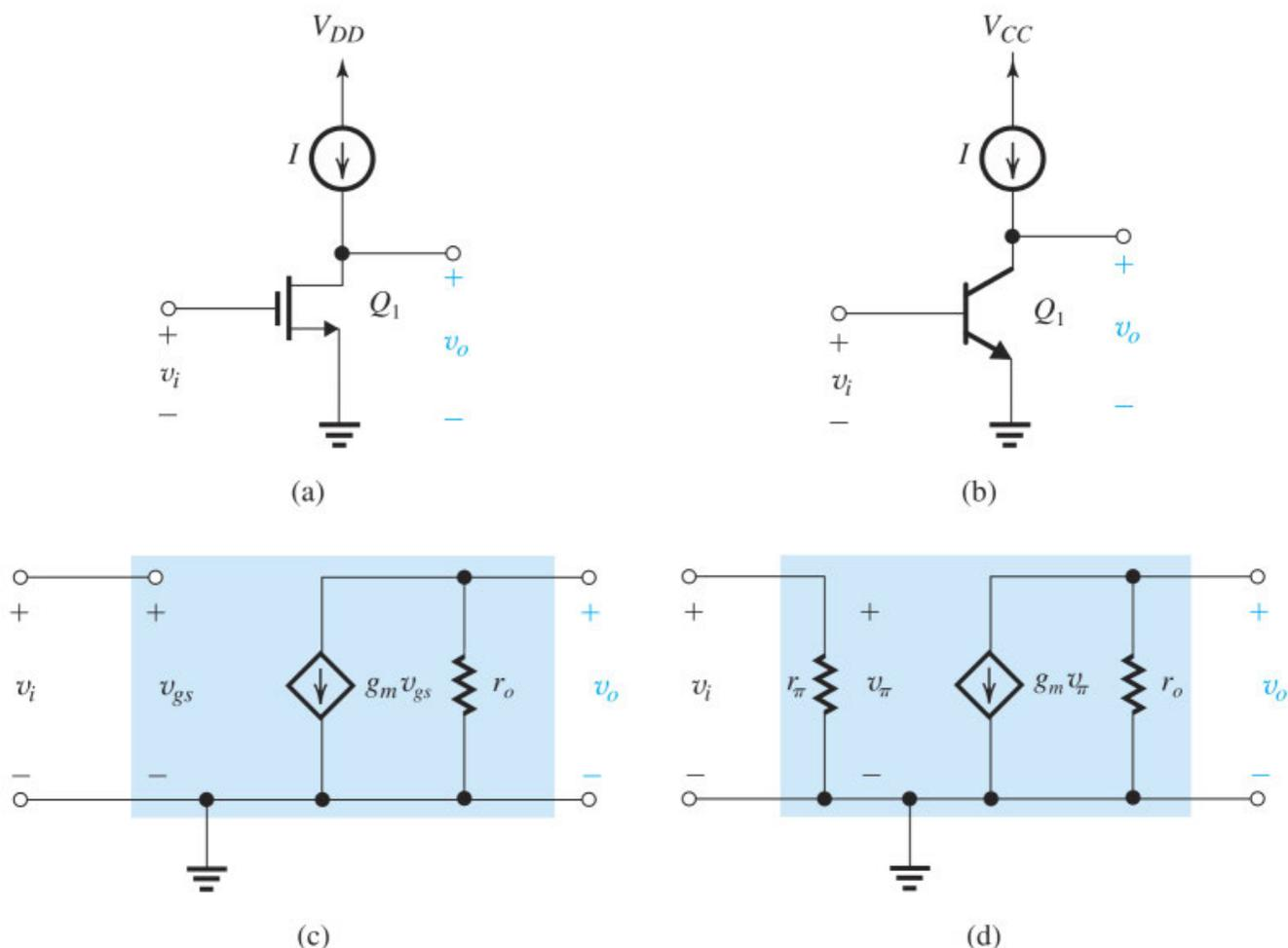
**Figure 8.13** The basic gain cells of IC amplifiers: (a) current-source- or active-loaded common-source amplifier; (b) current-source- or active-loaded common-emitter amplifier; (c) small-signal equivalent circuit of (a); and (d) small-signal equivalent circuit of (b).
