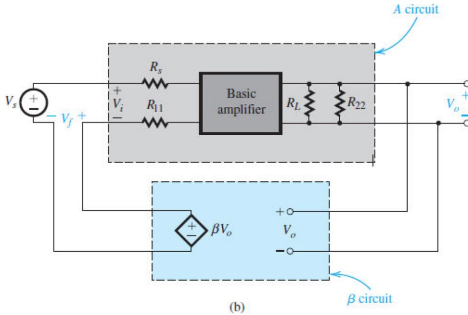
Figure 11.16 (b) The circuit in (a) represented by the ideal structure of Fig. 11.12(a).
