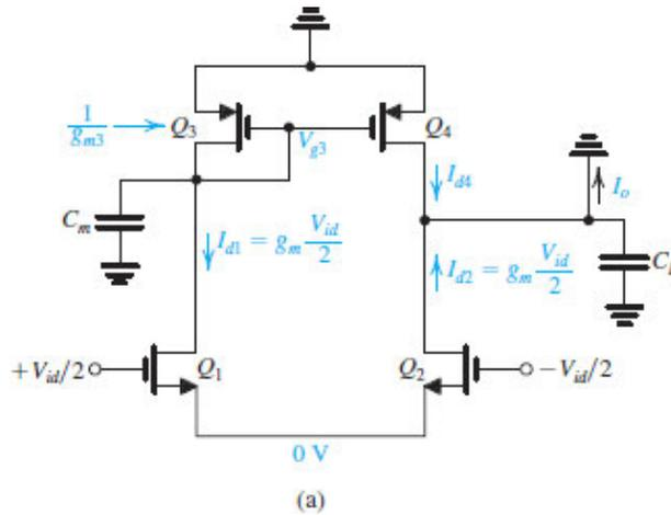
**Figure 10.29 (a)** Frequency–response analysis of the active-loaded MOS differential amplifier.
