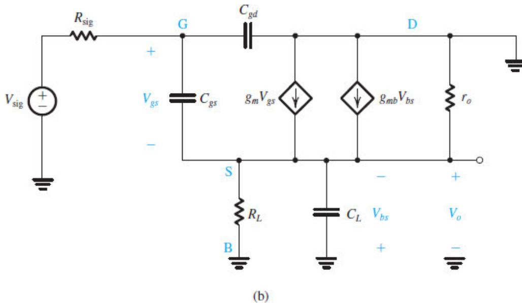
**Figure 10.23 (b)** High-frequency equivalent circuit of the source follower.
