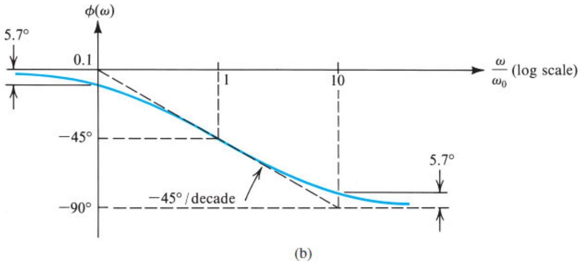
Figure 1.23 (b) Phase response of STC networks of the low-pass type.
