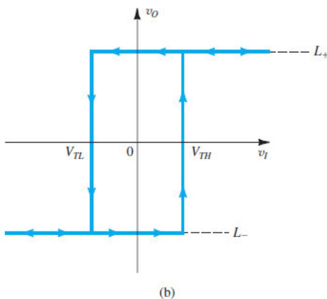
**Figure 15.22 (b)** The transfer characteristic of the circuit in (a) is noninverting. [Compare it to the inverting characteristic in Fig. 15.21(d).]
