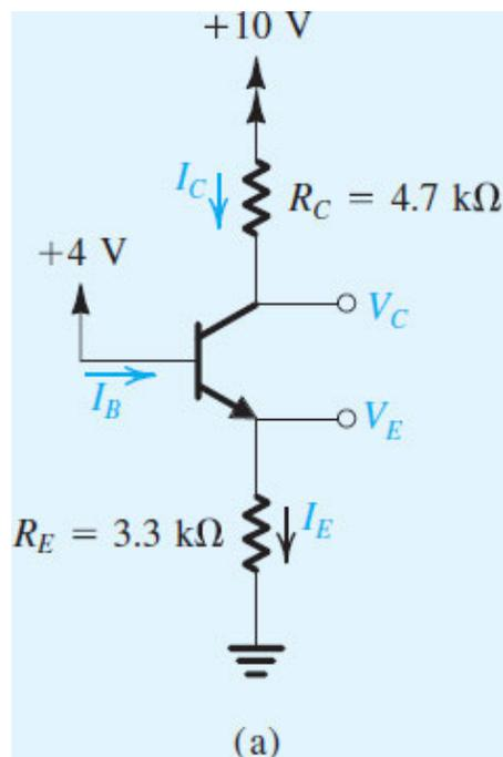
**Figure 6.23 (a)** Analysis of the circuit for Example 6.4: a circuit.
