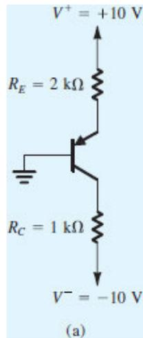
Figure 6.26 (a) Example 6.7: circuit.
