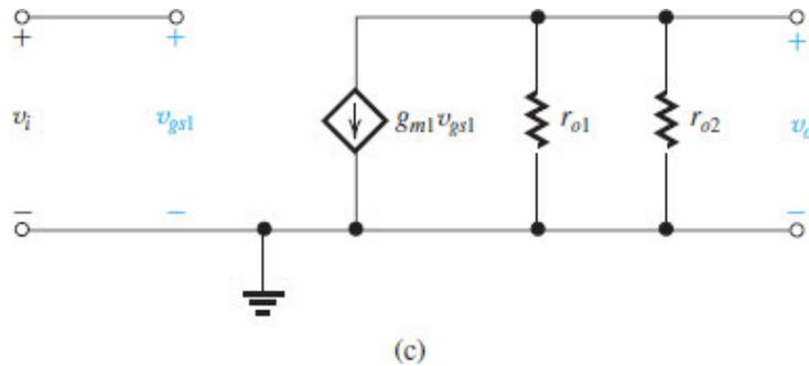
**Figure 8.15 (c)** small-signal equivalent circuit of the amplifier.
