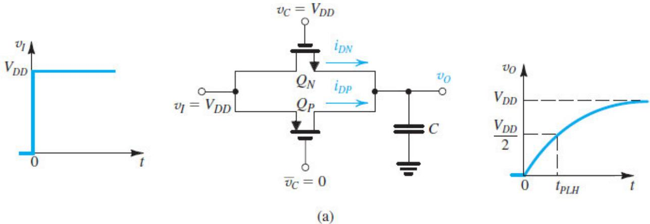
**Figure 18.7 (a)** Operation of the transmission gate as a switch with  $v_I$  high.
