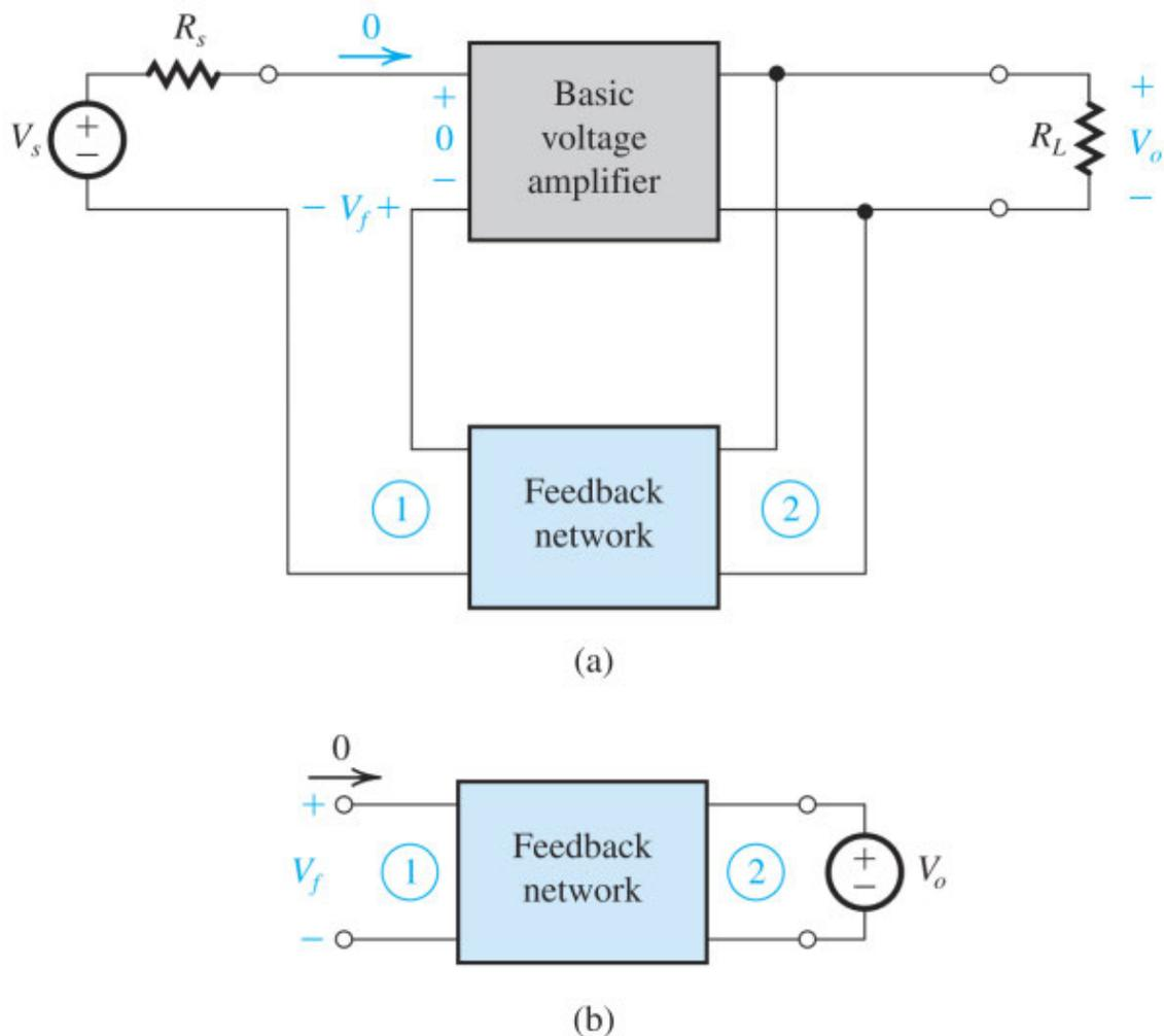
**Figure 11.10 (a)** The general feedback voltage amplifier under the assumption that the open-loop gain  $A$  of the basic amplifier is infinite. The resulting 0 V between the input terminals and the correspondingly zero current in the input series loop enable us to determine  $\beta$  as shown in **(b)**.
