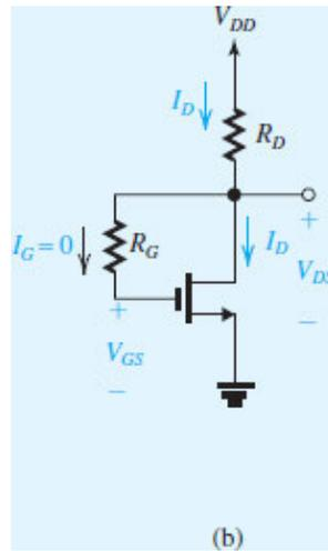
Figure 7.16 (b) Example 7.3: circuit for determining the dc operating point.
