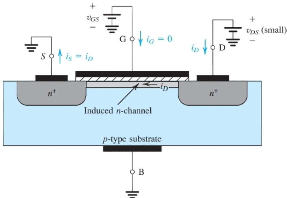
**Figure 5.3** An NMOS transistor with  $v_{GS} > V_t$  and with a small  $v_{DS}$  applied. The device acts as a resistance whose value is determined by  $v_{GS}$ . Specifically, the channel conductance is proportional to  $v_{GS} - V_t$ , and thus  $i_D$  is proportional to  $(v_{GS} - V_t)v_{DS}$ . Note that the depletion region is not shown (for simplicity).
