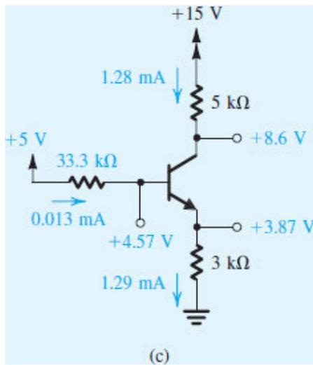
Figure 6.29 (c) Circuit for Example 6.10.
