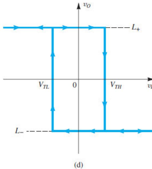
**Figure 15.21 (d)** The complete transfer characteristics.
