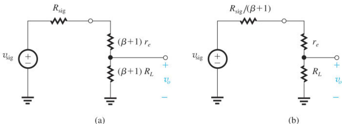
**Figure 7.45** Simple equivalent circuits for the emitter follower obtained by (a) reflecting  $r_e$  and  $R_L$  to the base side, and (b) reflecting  $v_{\text{sig}}$  and  $R_{\text{sig}}$  to the emitter side. Note that the circuit in (b) can be obtained from that in (a) by simply dividing all resistances by  $(\beta + 1)$ .
