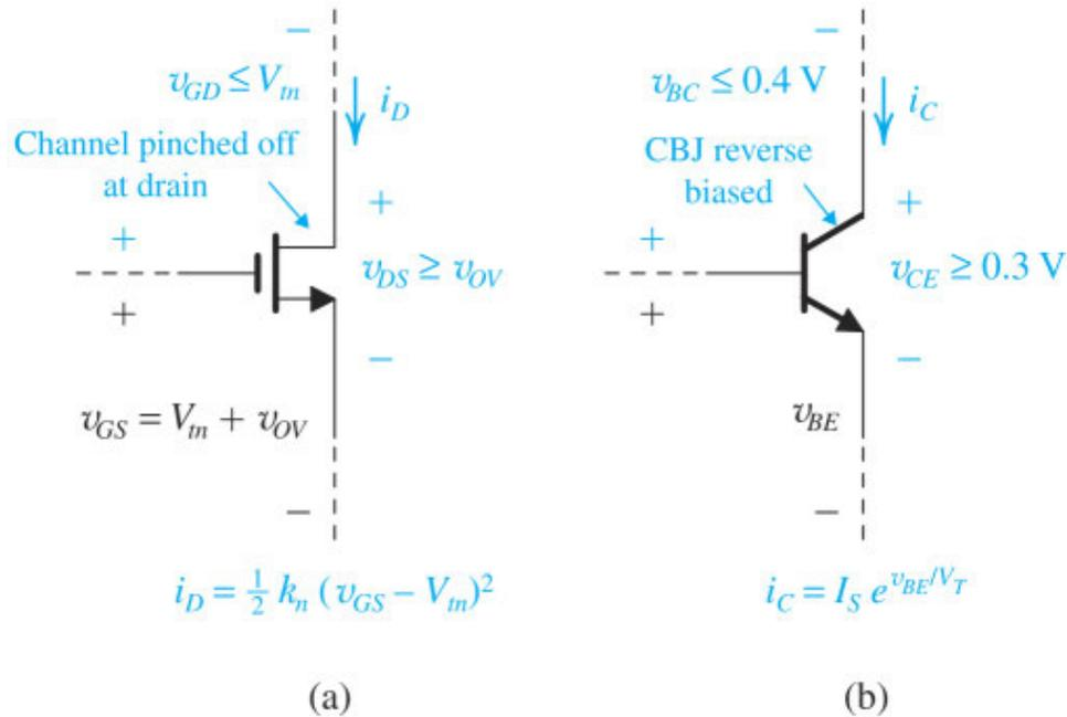
**Figure 7.1** Operating (a) an NMOS transistor and (b) an *npn* transistor in the active mode. Note that  $v_{GS} = V_m + v_{OV}$  and  $v_{DS} \geq v_{OV}$ ; thus  $v_{GD} \leq V_m$ , which ensures channel pinch-off at the drain end. Similarly,  $v_{BE} \simeq 0.7$  V, and  $v_{CE} \geq 0.3$  V results in  $v_{BC} \leq 0.4$  V, which is sufficient to keep the CBJ from conducting.
