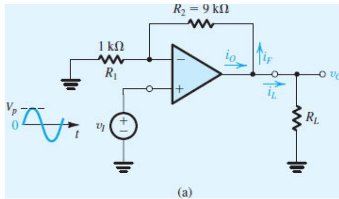
**Figure 2.43 (a)** A noninverting amplifier with a nominal gain of 10 V/V designed using an op amp that saturates at  $\pm 13$ -V output voltage and has  $\pm 20$ -mA output current limits.
