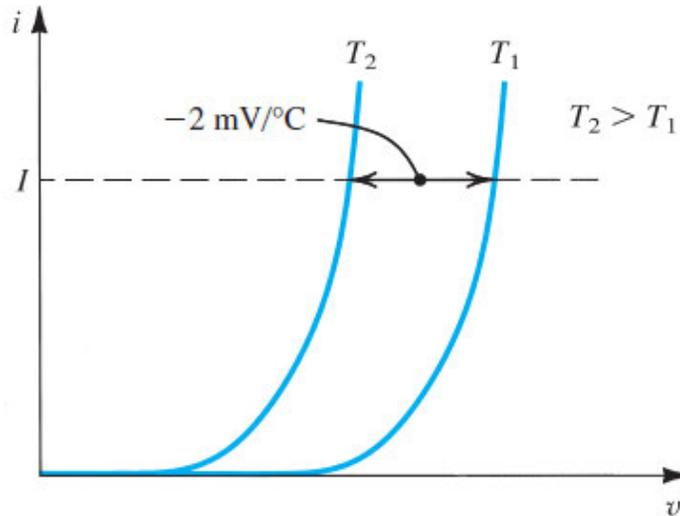
**Figure 4.9** Temperature dependence of the diode forward characteristic. At a constant current, the voltage drop decreases by approximately 2 mV for every  $1^\circ\text{C}$  increase in temperature.
