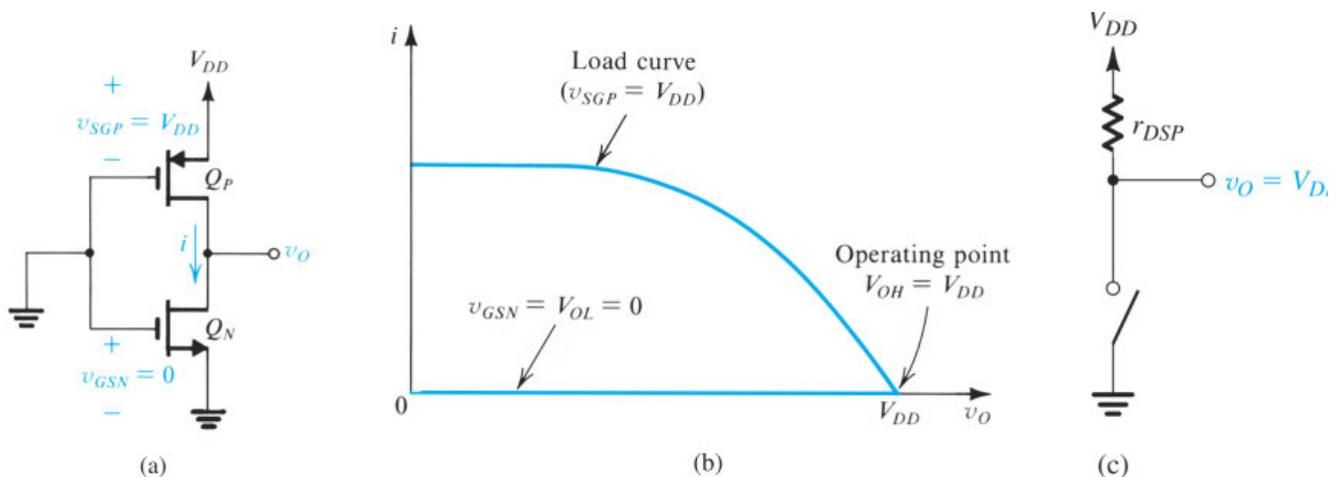
**Figure 16.24** Operation of the CMOS inverter when  $v_I$  is low: (a) circuit with  $v_I = 0$  V (logic-0 level, or  $V_{OL}$ ); (b) graphical construction to determine the operating point; (c) equivalent circuit.
