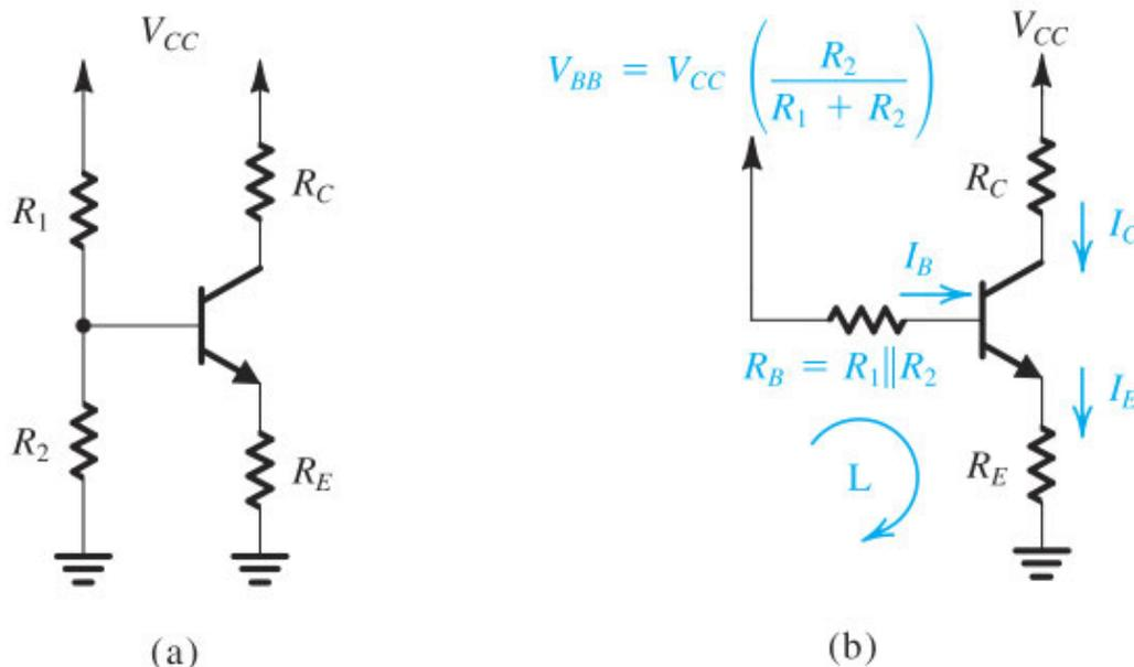
**Figure 7.54** Classical biasing for BJTs using a single power supply: (a) circuit; (b) circuit with the voltage divider supplying the base replaced with its Thévenin equivalent.
