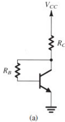
**Figure 7.56 (a)** A common-emitter transistor amplifier biased by a feedback resistor  $R_B$ .
