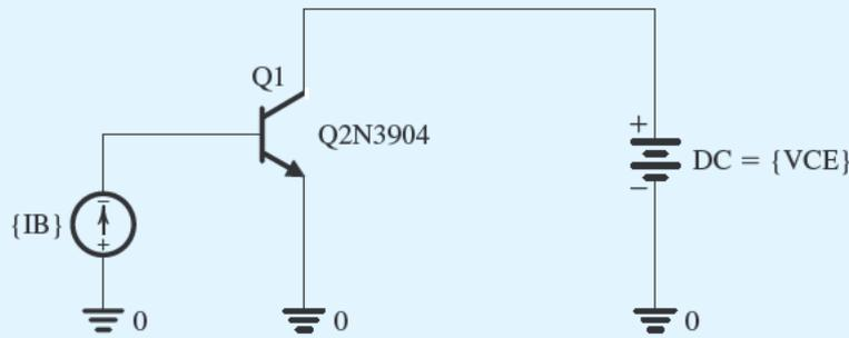
**Figure B.17** The SPICE test bench used to demonstrate the dependence of  $\beta_{dc}$  on the collector bias current  $I_C$  for the Q2N3904 discrete BJT (Example S.6.1).
