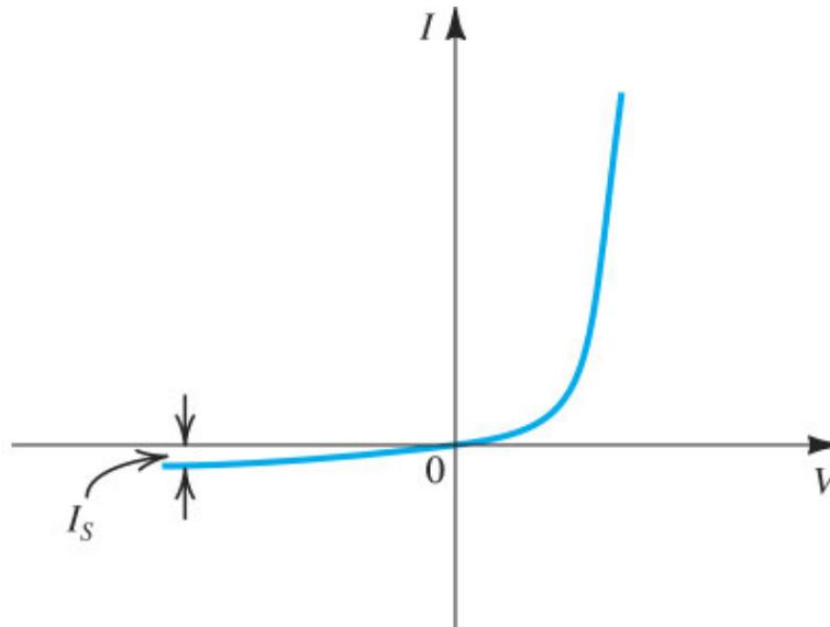
**Figure 3.13** The  $pn$  junction  $I$ - $V$  characteristic.
