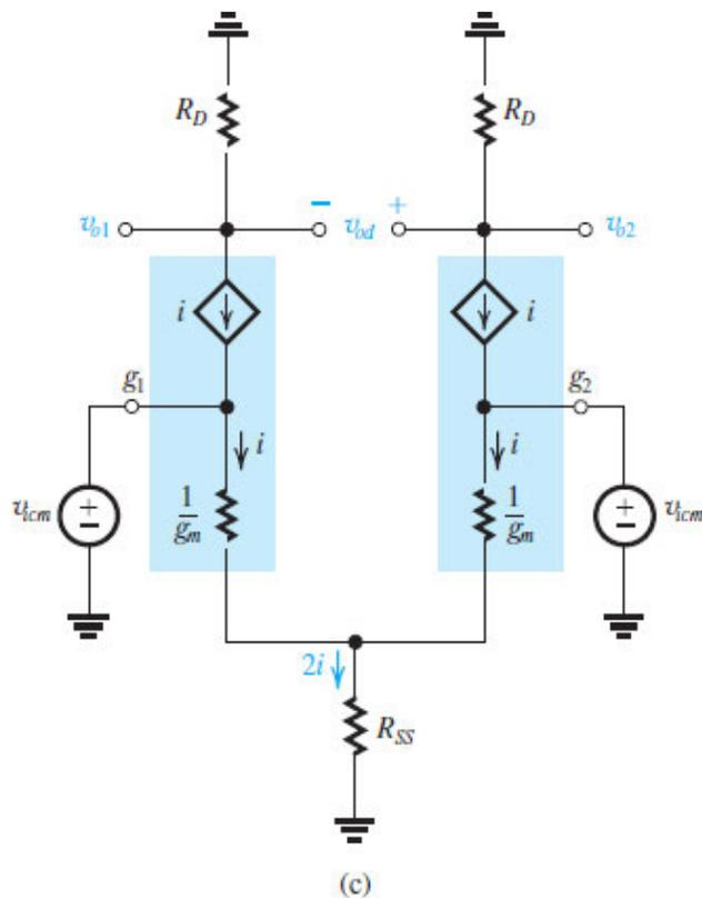
Figure 9.24 (c) The amplifier circuit with the transistors replaced with their T model and  $r_o$  neglected.
