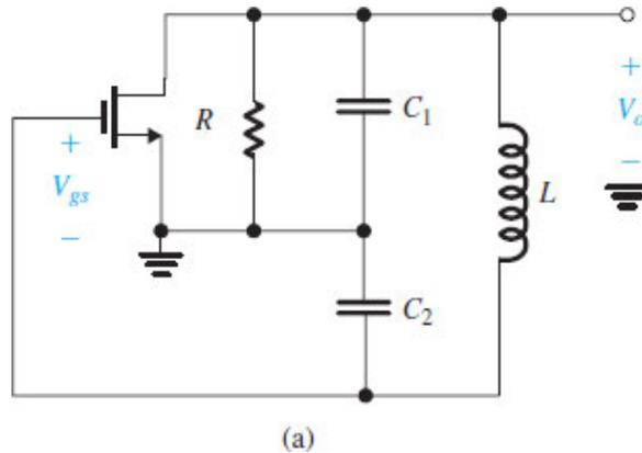
**Figure 15.15 (a)** A Colpitts oscillator in which the source is grounded and the output is taken at the drain.
