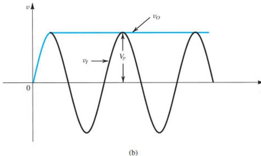
**Figure 4.24 (b)** Input and output waveforms assuming an ideal diode. Note that the circuit provides a dc voltage equal to the peak of the input sine wave. The circuit is therefore known as a *peak rectifier* or a *peak detector*.
