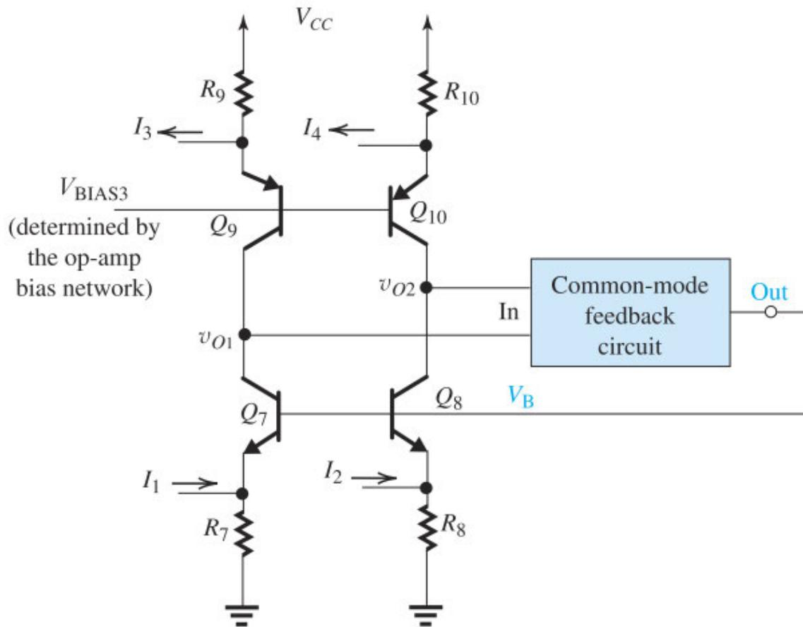
**Figure 13.20** The cascode output circuit of the input stage and the CMF circuit that responds to the common-mode component  $V_{CM} = \frac{1}{2}(v_{O1} + v_{O2})$  by adjusting  $V_B$  so that  $Q_7$ – $Q_8$  conduct equal currents to  $Q_9$ – $Q_{10}$ , and  $Q_7$ – $Q_{10}$  operate in the active mode.
