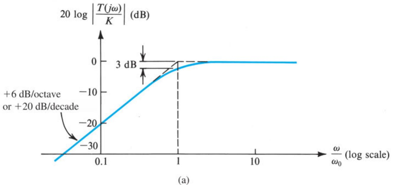
Figure 1.24 (a) Magnitude of STC networks of the high-pass type.
