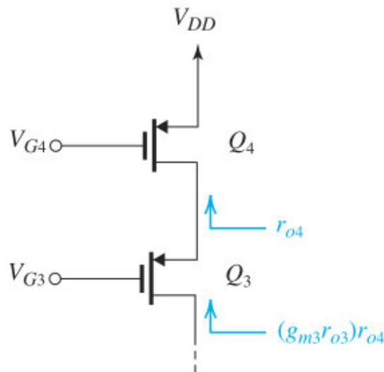
**Figure 8.30** Employing a cascode transistor  $Q_3$  to raise the output resistance of the current source  $Q_4$ .
