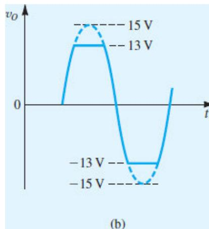
**Figure 2.43 (b)** When the input sine wave has a peak of 1.5 V, the output is clipped off at  $\pm 13$  V.
