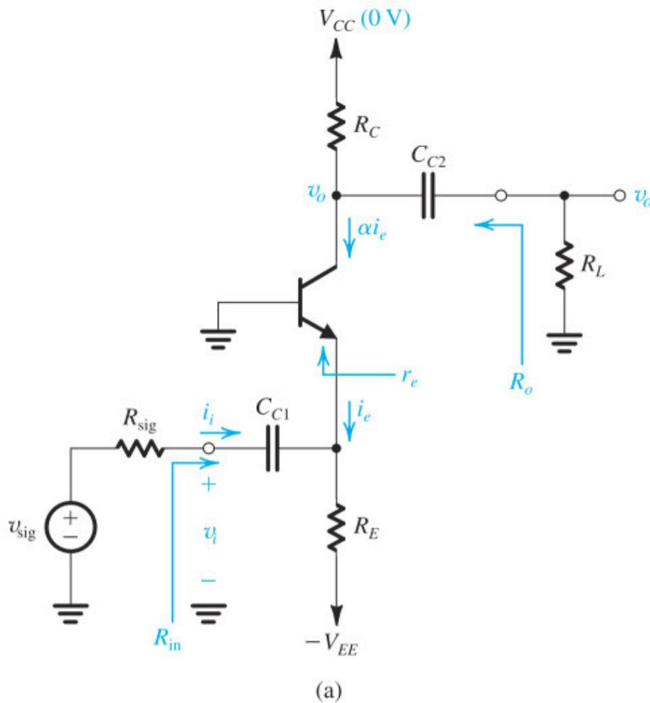
**Figure 7.60 (a)** A common-base amplifier using the structure of Fig. 7.55 with  $R_B$  omitted (since the base is grounded). Small-signal quantities are shown in color.
