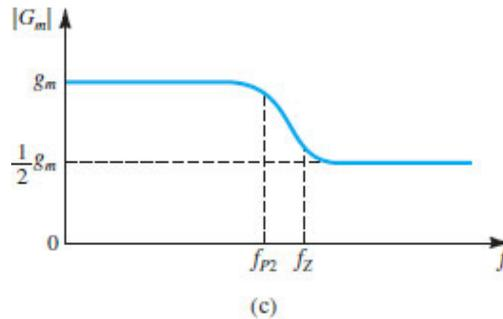
**Figure 10.29 (c)** The overall transconductance  $G_m$  as a function of frequency.
