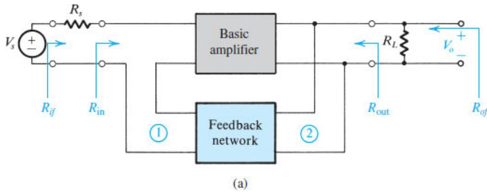
Figure 11.16 (a) Block diagram of a practical series–shunt feedback amplifier.
