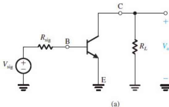
**Figure 10.13 (a)** CE amplifier circuit.
