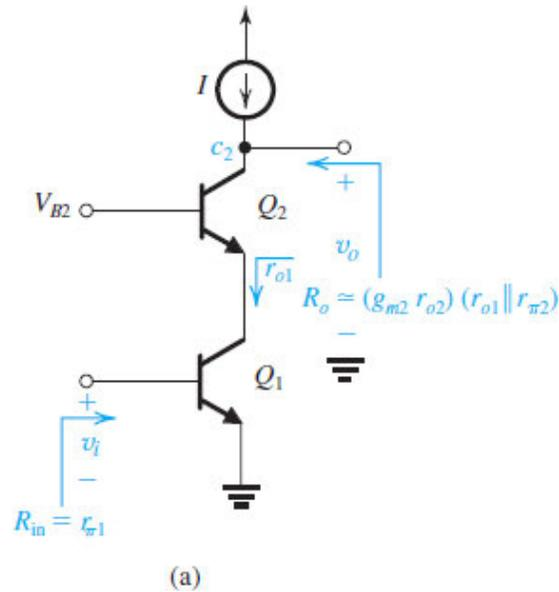
**Figure 8.33 (a)** A BJT cascode amplifier with an ideal current-source load.
