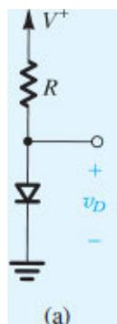
**Figure 4.17 (a)** Circuit for Example 4.5.
