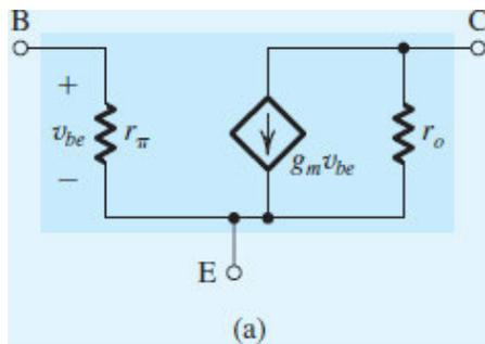
**Figure 1.19 (a)** Small-signal circuit model for a bipolar junction transistor (BJT).
