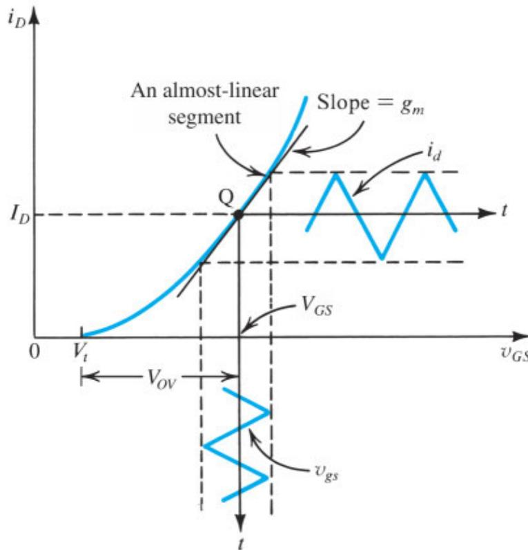
Figure 7.11 Small-signal operation of the MOSFET amplifier.
