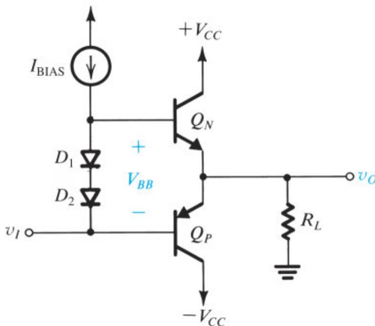
**Figure 12.13** A class AB output stage using diodes for biasing. If the junction area of the output devices,  $Q_N$  and  $Q_P$ , is  $n$  times that of the biasing devices  $D_1$  and  $D_2$ , a quiescent current  $I_Q = nI_{BIAS}$  flows in the output devices.
