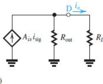
Figure 8.18 (b) Equivalent circuit model of the CG amplifier in (a).
