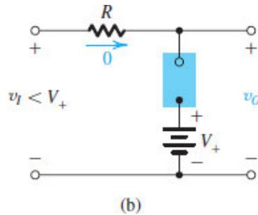
**Figure 4.5 (b)** When  $v_I < V_+$ , the diode is reverse biased. Hence, it is an open circuit.
