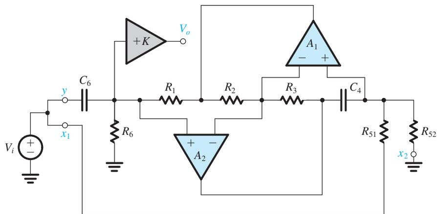
(f) HPN,  $\omega_n \leq \omega_0$ **Figure H.6** continued (d) Notch at  $\omega_0$ ; (e) LPN,  $\omega_n \geq \omega_0$ ; (f) HPN,  $\omega_n \leq \omega_0$ .
