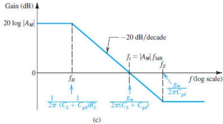
**Figure 10.12 (c)** Bode plot for the gain of the circuit in (a).
