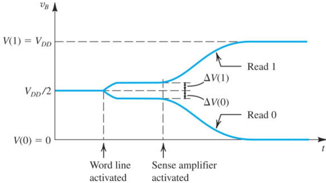
**Figure 18.35** Waveforms of  $v_B$  before and after the activation of the sense amplifier. In a read-1 operation, the sense amplifier causes the initial small increment  $\Delta V(1)$  to grow exponentially to  $V_{DD}$ . In a read-0 operation, the negative  $\Delta V(0)$  grows to 0. Complementary signal waveforms develop on the  $\overline{B}$  line.
