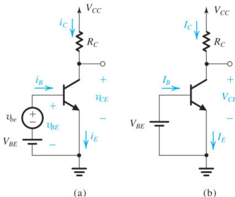
**Figure 7.21** (a) Conceptual circuit to illustrate the operation of the transistor as an amplifier. (b) The circuit of (a) with the signal source  $v_{be}$  eliminated for dc (bias) analysis.
