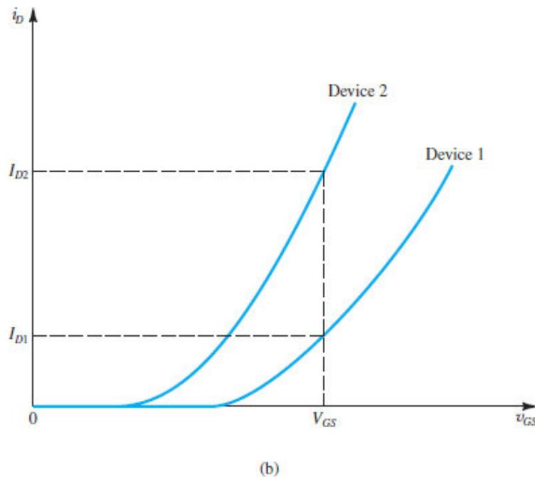
**Figure 7.49 (b)** The use of fixed bias (constant  $V_{GS}$ ) can result in a large variability in the value of  $I_D$ . Devices 1 and 2 represent extremes among units of the same type.
