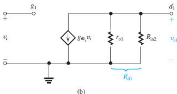
**Figure 8.32 (b)** Determining  $v_{o1}$ .
