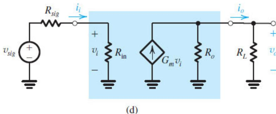
**Figure 7.35 (d)** Characterization of the amplifier as a functional block: alternative representation of the circuit in (a).
