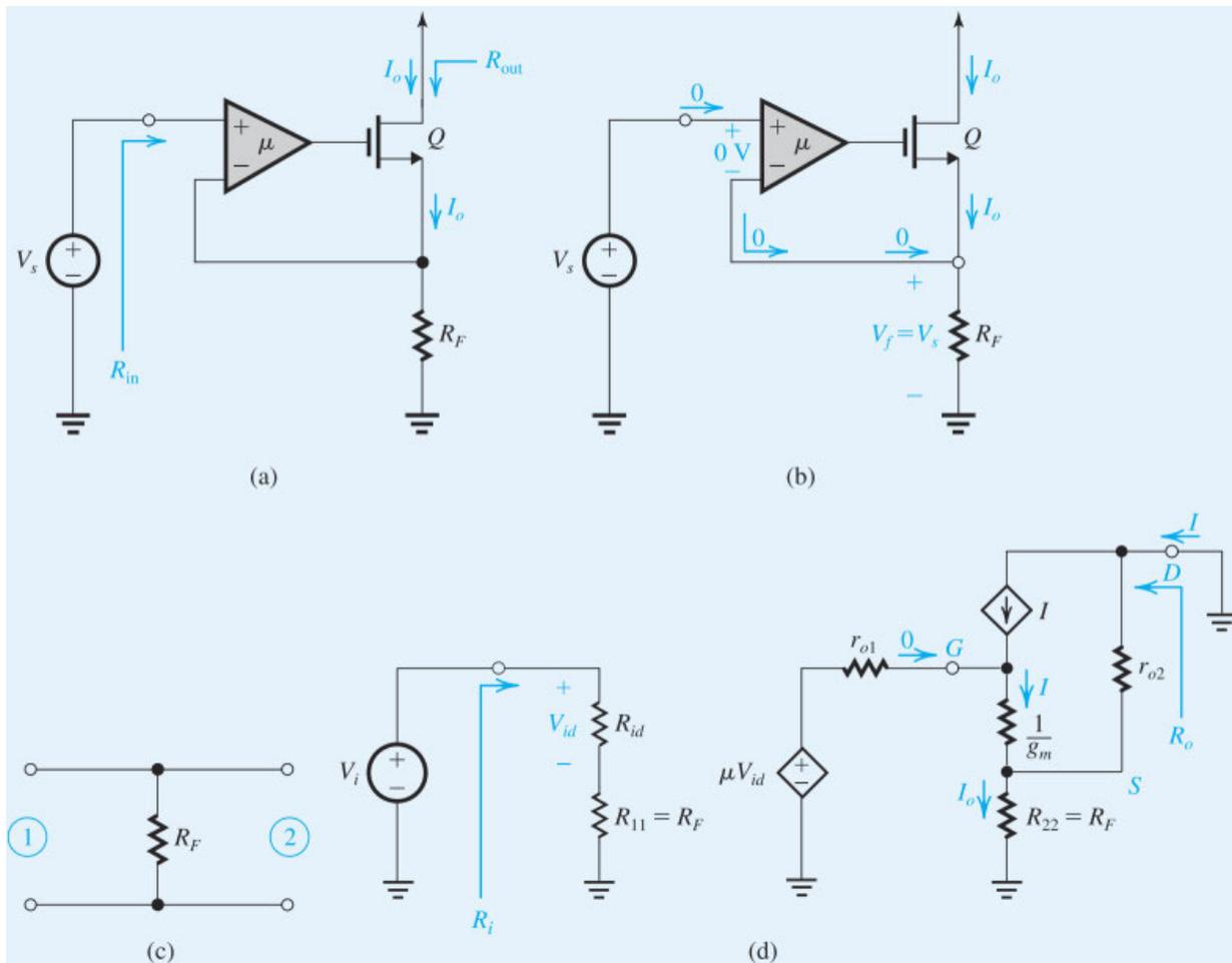
**Figure 11.23** (a) Feedback transconductance amplifier for Example 11.7; (b) determining  $A_f|_{ideal}$  by setting the open-loop gain to infinity; (c) the feedback network; (d) the A circuit with the op amp and the MOSFET replaced with their equivalent circuit models.
