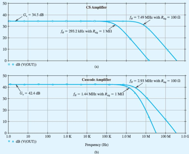
**Figure B.38** Frequency response of (a) the CS amplifier and (b) the folded-cascode amplifier in Example S.10.1, with  $R_{\text{sig}} = 100 \Omega$  and  $R_{\text{sig}} = 1 \text{ M}\Omega$ .
