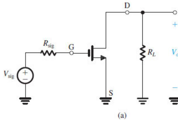
Figure 10.11 (a) A common-source amplifier.
