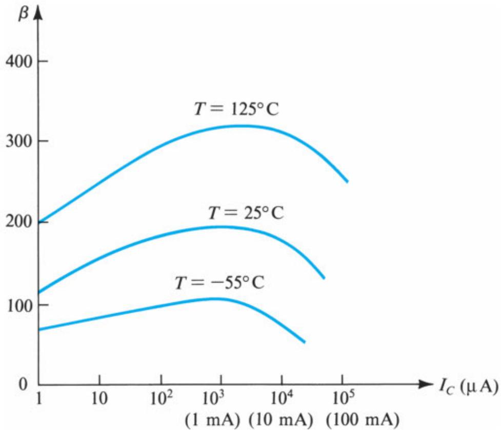
**Figure 6.34** Typical dependence of  $\beta$  on  $I_C$  and on temperature in an integrated-circuit *npn* silicon transistor intended for operation around 1 mA.
