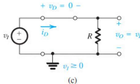
Figure 4.3 (c) Equivalent circuit when  $v_I \geq 0$ .
