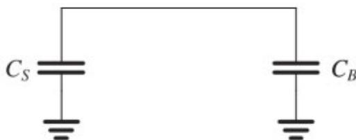
**Figure 18.29** When the voltage of the selected word line is raised, the transistor conducts, thus connecting the storage capacitor  $C_S$  to the bit-line capacitor  $C_B$ .
