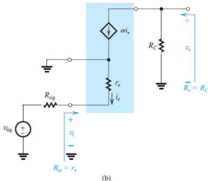
Figure 7.41 (b) Amplifier equivalent circuit with the BJT represented by its T model.
