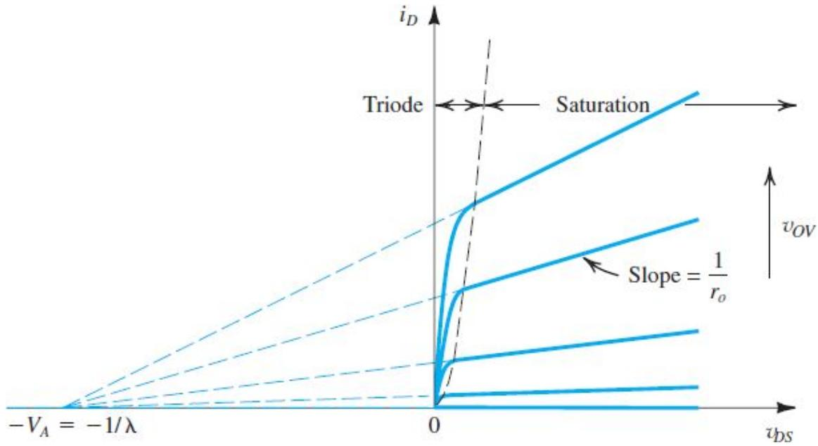
**Figure 5.17** Effect of  $v_{DS}$  on  $i_D$  in the saturation region. The MOSFET parameter  $V_A$  depends on the process technology and, for a given process, is proportional to the channel length  $L$ .
