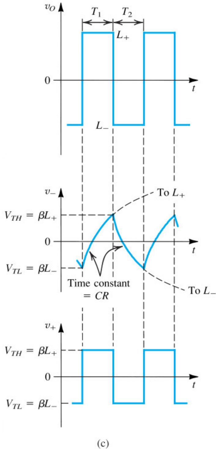
**Figure 15.23 (c)** Waveforms at various nodes of the circuit in (b). This circuit is called an astable multivibrator.
