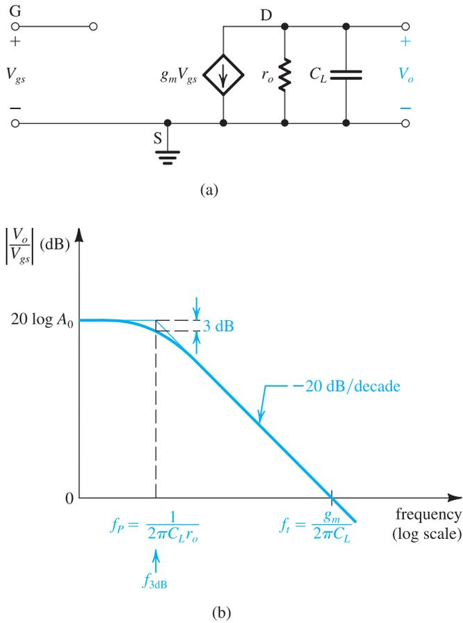
**Figure G.2** Frequency response of a CS amplifier loaded with a capacitance  $C_L$  and fed with an ideal voltage source. It is assumed that the transistor is operating at frequencies much lower than  $f_T$ , and thus the internal capacitances are not taken into account.
