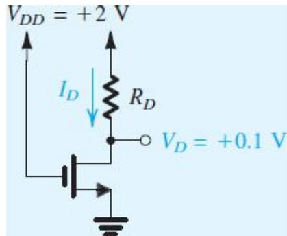
Figure 5.23 Circuit for Example 5.5.
