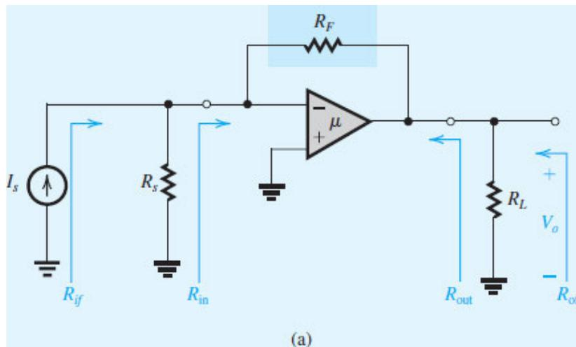
**Figure 11.27 (a)** A feedback transresistance amplifier.
