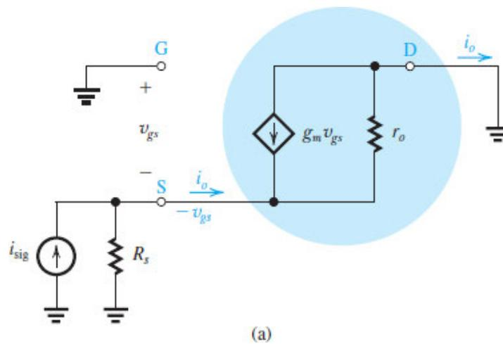
**Figure 8.20 (a)** Determining the short-circuit current gain  $A_{is} = i_o/i_{sig}$  of the CG amplifier.
