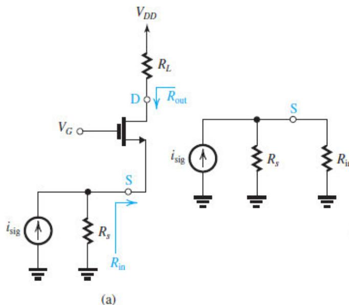
Figure 8.18 (a) A CG amplifier with the bias arrangement only partially shown.
