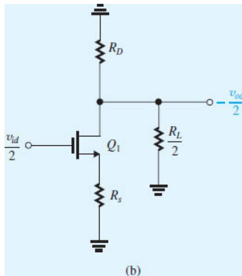
Figure 9.11 (b) Differential half-circuit.
