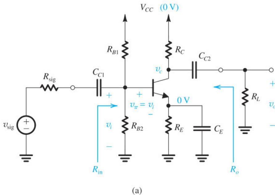
**Figure 7.58 (a)** A common-emitter amplifier using the classical biasing arrangement of Fig. 7.54(a). Signal quantities are shown in color.
