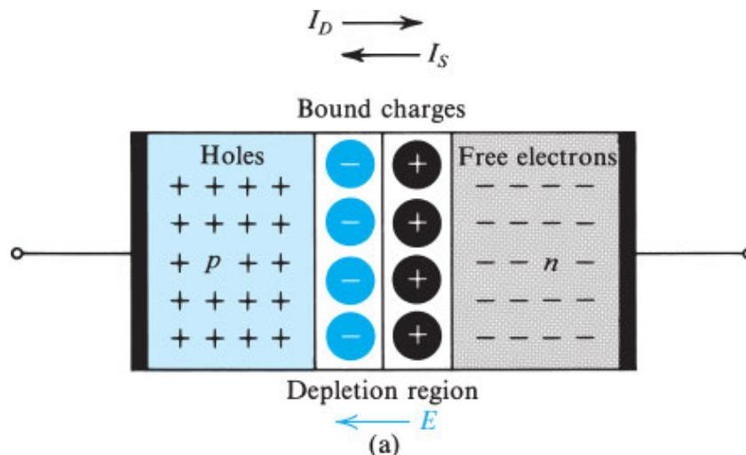
**Figure 3.9 (a)** The  $pn$  junction with no applied voltage (open-circuited terminals).
