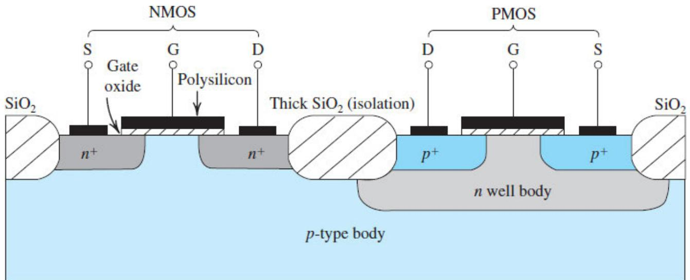
**Figure 5.10** Cross section of a CMOS integrated circuit. Note that the PMOS transistor is formed in a separate  $n$ -type region, known as an  $n$  well, which functions as the body for the PMOS transistor. Not shown are the connections made to the  $p$ -type body and to the  $n$  well body.
