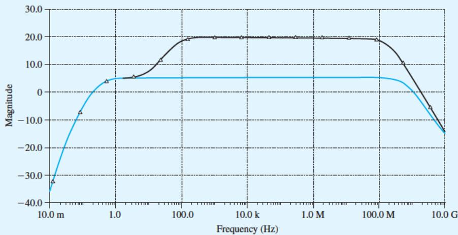
Figure B.42 Frequency response of the CS amplifier with  $C_s = 10 \mu\text{F}$  and  $C_s = 0$ .
