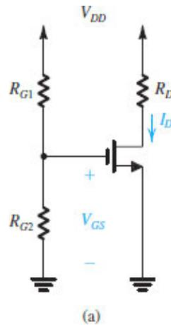
**Figure 7.49 (a)** Biasing the MOSFET with a constant  $V_{GS}$  generated from  $V_{DD}$  using a voltage divider ( $R_{G1}, R_{G2}$ ).
