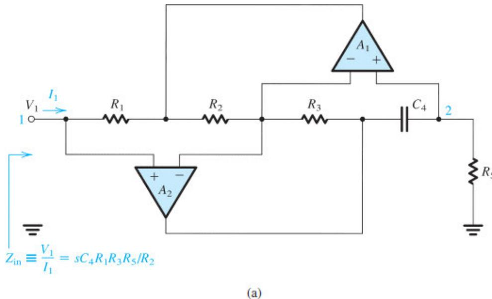
**Figure 14.20 (a)** The Antoniou inductance-simulation circuit.
