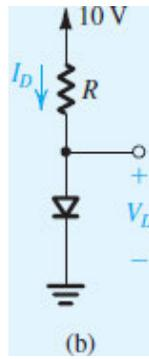
**Figure 4.17 (b)** Circuit for calculating the dc operating point.
