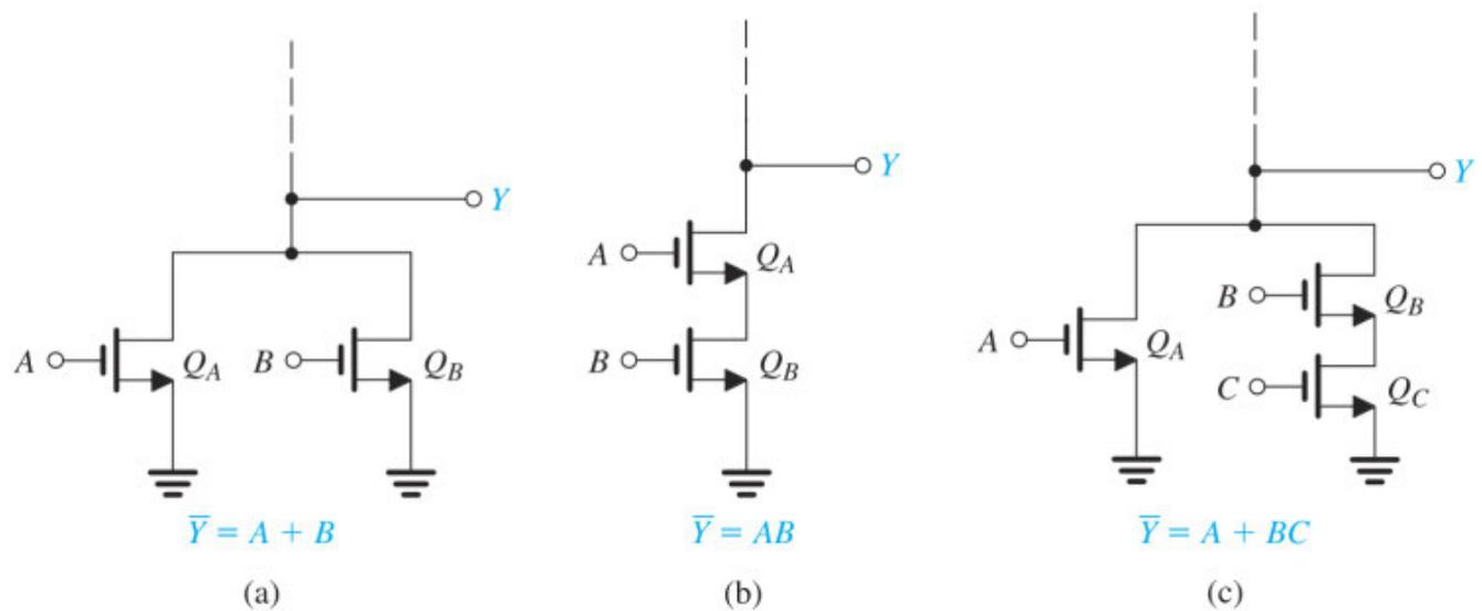
**Figure 16.4** Examples of pull-down networks.
