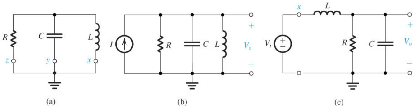
**Figure 14.18** (a) The second-order parallel LCR resonator. (b, c) Two ways of exciting the resonator of (a) without changing its *natural structure*; resonator poles are those poles of  $V_o/I$  and  $V_o/V_i$ .
