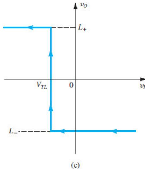
**Figure 15.21 (c)** The transfer characteristic for decreasing  $v_I$ .
