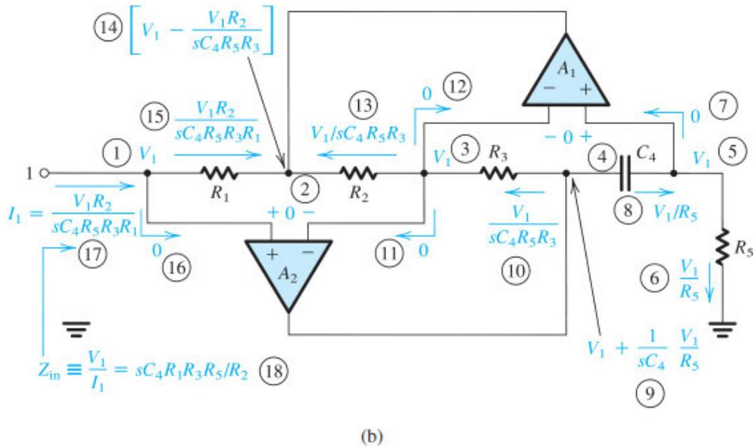
**Figure 14.20 (b)** Analysis of the circuit assuming ideal op amps. The order of the analysis steps is indicated by the circled numbers.
