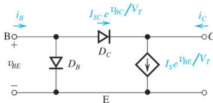
**Figure 6.9** Modeling the operation of an  $npn$  transistor in saturation by augmenting the model of Fig. 6.5(c) with a forward-conducting diode  $D_C$ . Note that the current through  $D_C$  increases  $i_B$  and reduces  $i_C$ .
