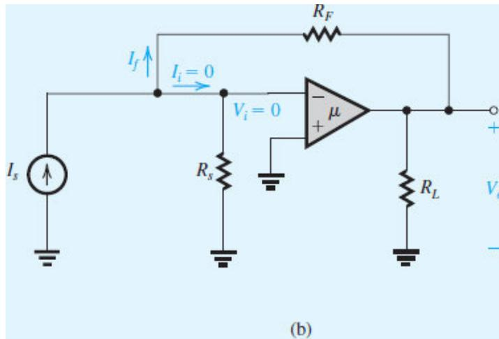
Figure 11.27 (b) Determining  $A_f|_{\text{ideal}}$  by setting  $A = \infty$ .
