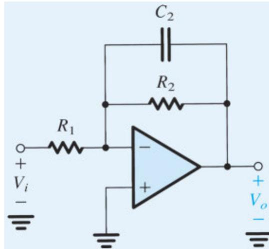
Figure 2.23 Circuit for Example 2.4.
