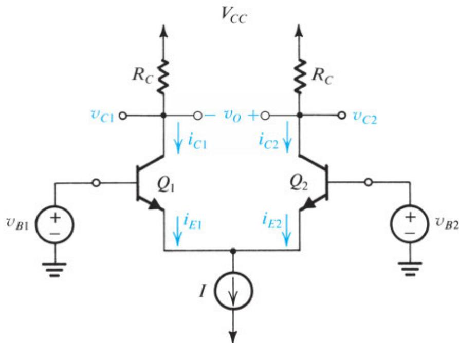
Figure 9.14 The basic BJT differential-pair configuration.
