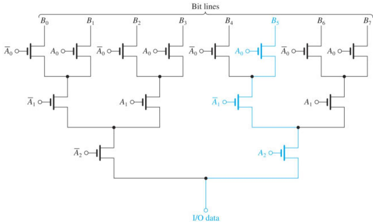
**Figure 18.38** A tree column decoder. Note that the colored path shows the transistors that are conducting when  $A_0 = 1$ ,  $A_1 = 0$ , and  $A_2 = 1$ , the address that results in connecting  $B_5$  to the data line.
