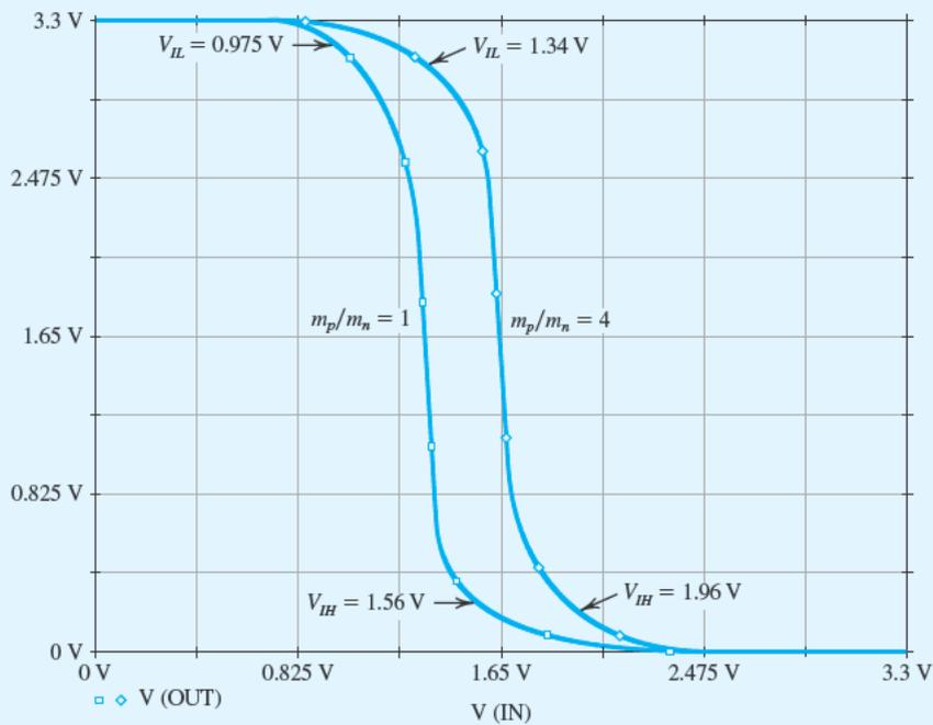
Figure B.77 Input-output voltage transfer characteristic (VTC) of the CMOS inverter in Example S.16.1 with  $m_p/m_n = 1$  and  $m_p/m_n = 4$ .
