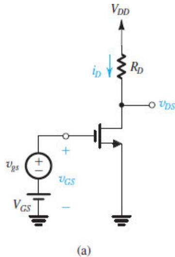
**Figure 7.4 (a)** The MOSFET amplifier with a small time-varying signal  $v_{gs}(t)$  superimposed on the dc bias voltage  $V_{GS}$ .
