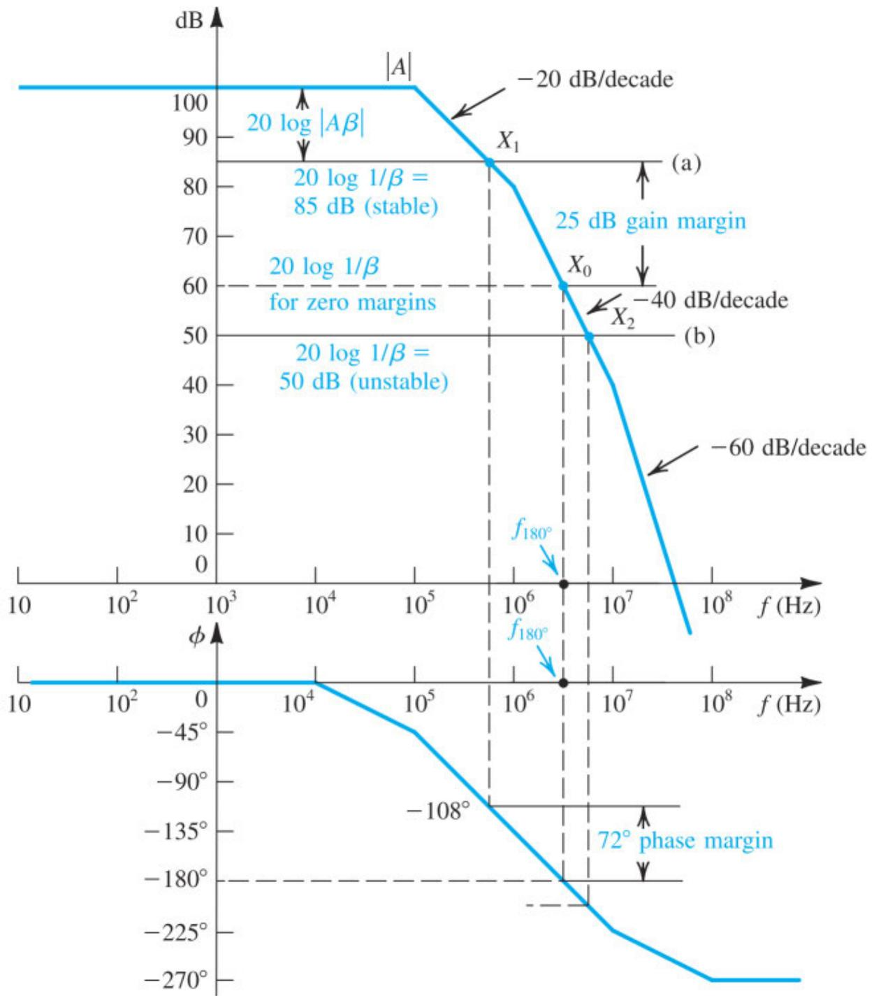
**Figure 11.38** Stability analysis using Bode plot of  $A$ .
