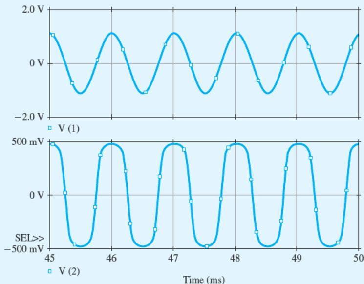
**Figure B.75** Output waveforms of the active-filter-tuned oscillator shown in Fig. B.74 for  $Q = 5$  ( $R_1 = 50 \text{ k}\Omega$ ).
