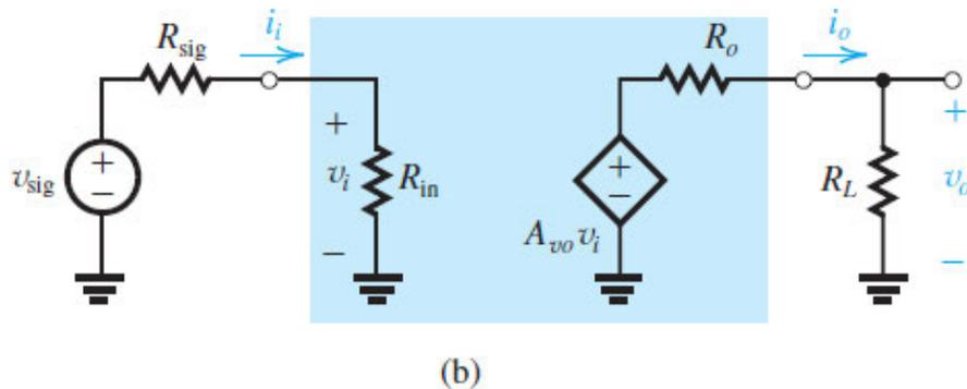
Figure 7.35 (b) Characterization of the amplifier as a functional block: equivalent-circuit representation of the circuit in (a).
