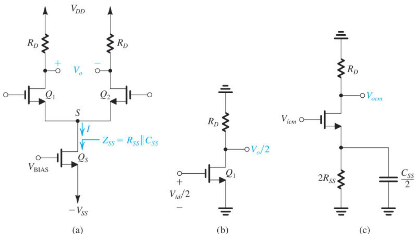
**Figure 10.26** (a) A resistively loaded MOS differential pair; the transistor supplying the bias current is explicitly shown. It is assumed that the total impedance between node  $S$  and ground,  $Z_{SS}$ , consists of a resistance  $R_{SS}$  in parallel with a capacitance  $C_{SS}$ . (b) Differential half-circuit. (c) Common-mode half-circuit.
