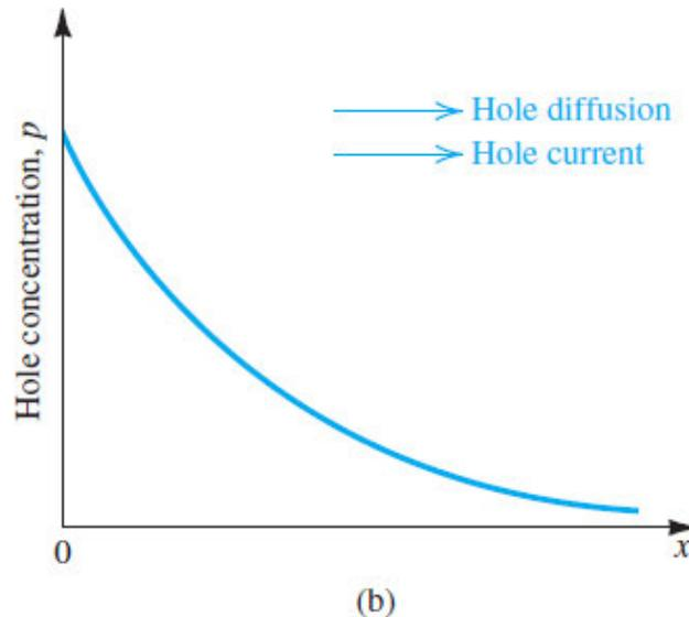
**Figure 3.6 (b)** A graphical representation of the hole concentration profile.
