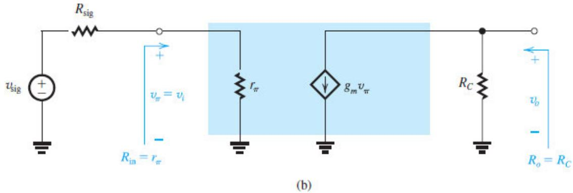
**Figure 7.37 (b)** The common-emitter amplifier circuit with the BJT replaced by its hybrid- $\pi$  model.
