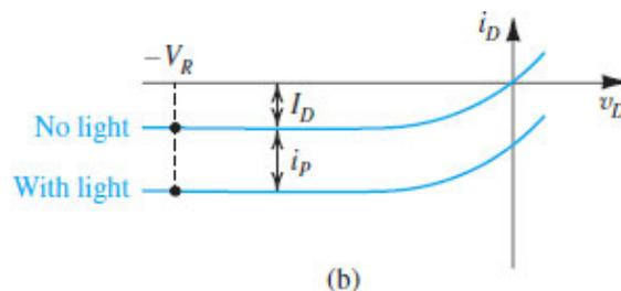
Figure 4.32 (b) Shifting  $i-v$  characteristic of the photodiode under illumination.
