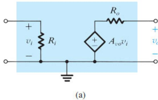
**Figure 1.16 (a)** Circuit model for the voltage amplifier.
