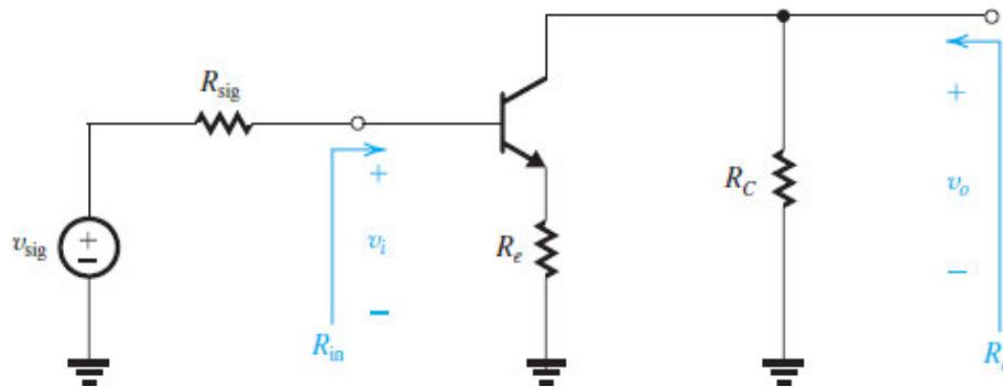
**Figure 7.39 (a)** The CE amplifier with an emitter resistance  $R_e$ ; circuit without bias details.
