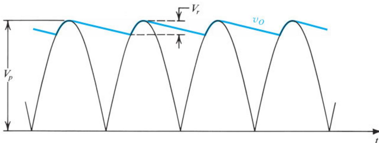
**Figure 4.26** Waveforms in the full-wave peak rectifier.
