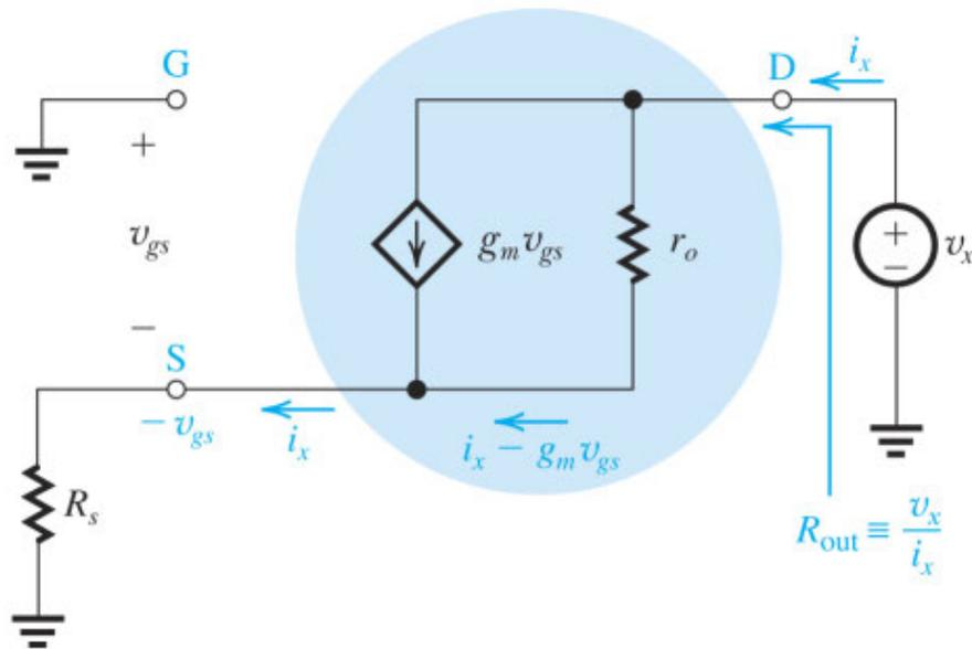
**Figure 8.21** Determining the output resistance  $R_{out}$  of the CG amplifier.
