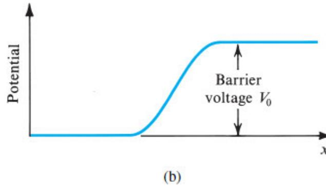
**Figure 3.9 (b)** The potential distribution along an axis perpendicular to the junction.
