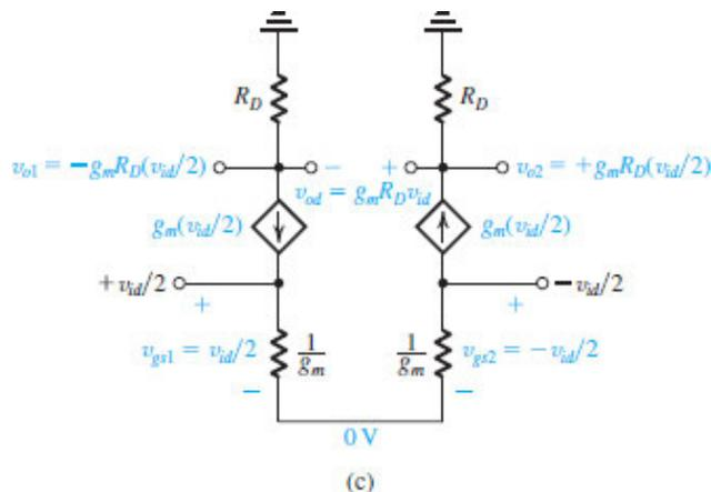
**Figure 9.8 (c)** Small-signal analysis of the MOS differential amplifier: The circuit in (b), with the MOSFETs replaced with T models.
