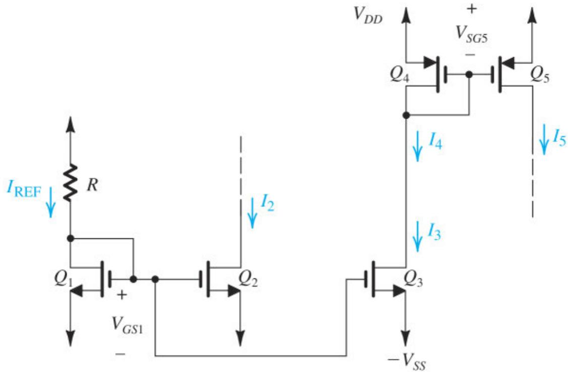
**Figure 8.4** A current-steering circuit.
