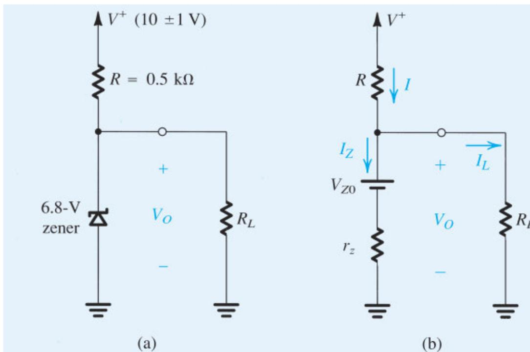
**Figure 4.19** (a) Circuit for Example 4.7. (b) The circuit with the zener diode replaced with its equivalent circuit model.
