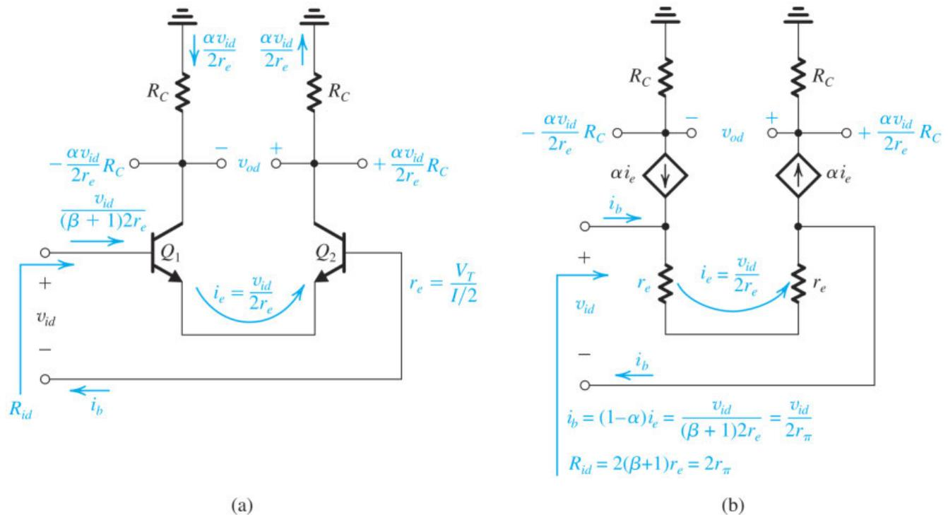
**Figure 9.19** A simple technique for determining the signal currents in a differential amplifier excited by a differential voltage signal  $v_{id}$ ; dc quantities are not shown. While Fig. 9.19(a) utilizes the BJT T model implicitly, the T model of both BJTs are shown explicitly in Fig. 9.19(b).
