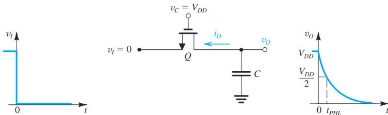
**Figure 18.4** Operation of the NMOS switch as the input goes low ( $v_I = 0$  V). Note that the drain of an NMOS transistor is always higher in voltage than the source; correspondingly, the drain and source terminals interchange roles in comparison to the circuit in Fig. 18.3.
