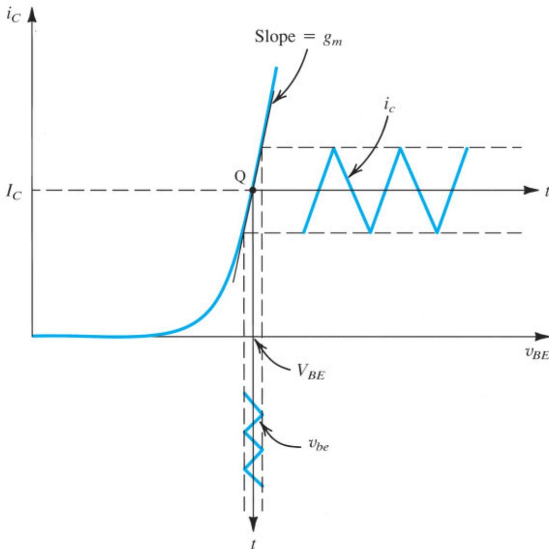
**Figure 7.22** Linear operation of the BJT under the small-signal condition: A small-signal  $v_{be}$  with a triangular waveform is superimposed on the dc voltage  $V_{BE}$ . It gives rise to a collector-signal current  $i_c$ , also of triangular waveform, superimposed on the dc current  $I_C$ . Here,  $i_c = g_m v_{be}$ , where  $g_m$  is the slope of the  $i_C$ - $v_{BE}$  curve at the bias point Q.
