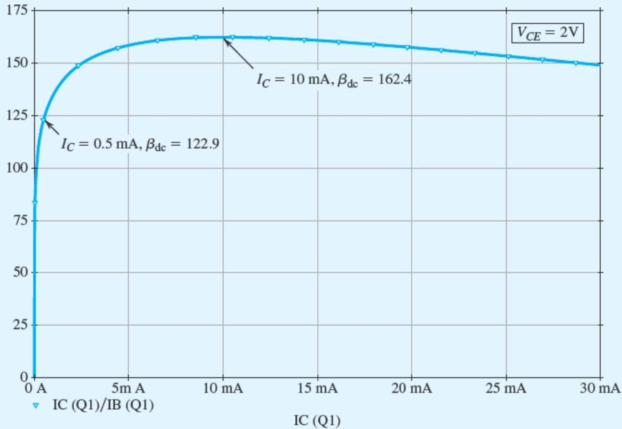
**Figure B.18** Dependence of  $\beta_{dc}$  on  $I_C$  (at  $V_{CE} = 2$  V) in the Q2N3904 discrete BJT (Example S.6.1).
