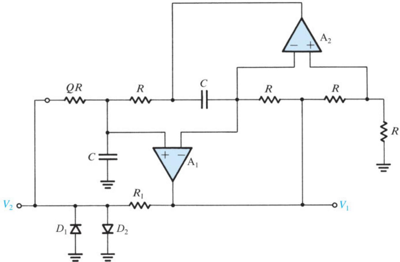
**Figure 15.13** A practical implementation of the active-filter-tuned oscillator.
