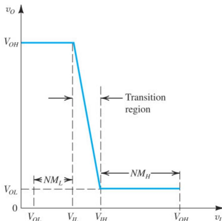
**Figure 16.13** Voltage-transfer characteristic of an inverter. The VTC is approximated by three straight-line segments. Note the four parameters of the VTC ( $V_{OH}$ ,  $V_{OL}$ ,  $V_{IL}$ , and  $V_{IH}$ ) and their use in determining the noise margins ( $NM_H$  and  $NM_L$ ).
