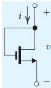
**Figure 5.22** Circuit for Example 5.4.
