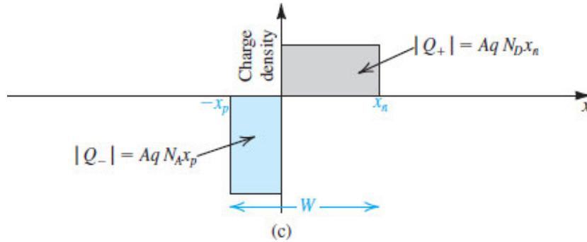
**Figure 3.10 (c)** The charge stored in both sides of the depletion region;  $Q_J = |Q_+| = |Q_-|$ .
