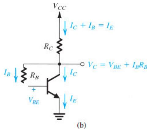
**Figure 7.56 (b)** A Analysis of the circuit in (a).
