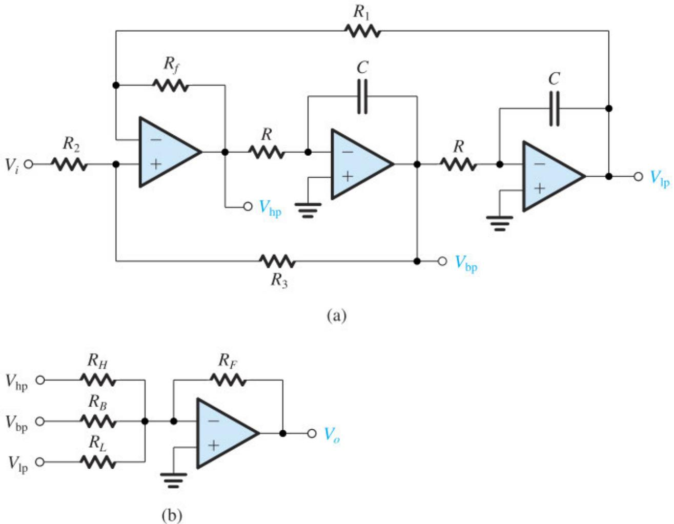
**Figure 14.24** (a) The KHN biquad circuit, obtained as a direct implementation of the block diagram of Fig. 14.23(c). The three basic filtering functions, HP, BP, and LP, are simultaneously realized. (b) To obtain notch and other functions, the three outputs are summed with appropriate weights using this op-amp summer.
