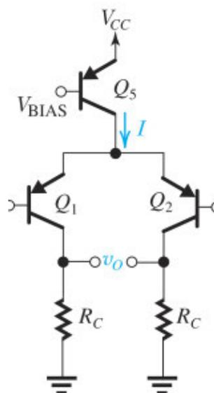
**Figure 13.16** For the input common-mode range to include ground voltage, the classical current-mirror-loaded input stage in Fig. 13.15 has to be replaced with the resistively loaded configuration with the dc-voltage drop across  $R_C$  limited to 0.2 V to 0.3 V.
