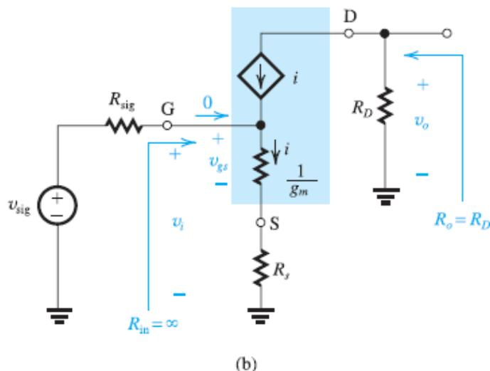
**Figure 7.38 (b)** The CS amplifier with a source resistance  $R_s$ : equivalent circuit with the MOSFET represented by its T model.
