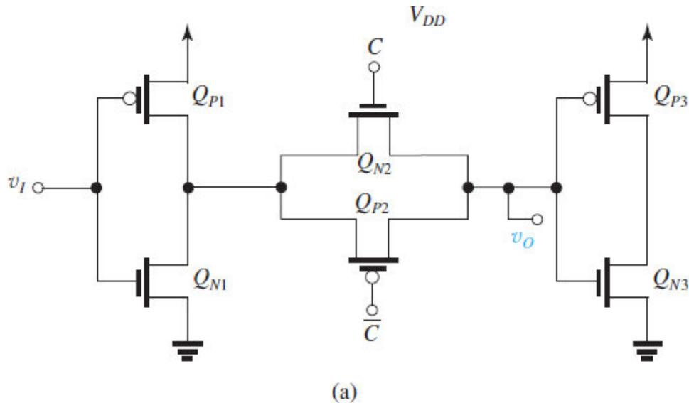
Figure 18.9 (a) A transmission gate connects the output of a CMOS inverter to the input of another.
