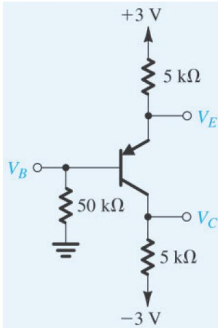
Figure VE6.3 Circuit for Video Example 6.3.
