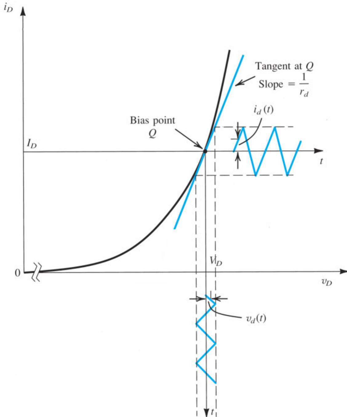
**Figure 4.15** Development of the diode small-signal model.
