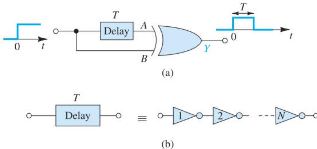
**Figure 18.33 (a)** A one-shot or monostable circuit. Utilizing a delay circuit with a delay  $T$  and an XOR gate, this circuit provides an output pulse of width  $T$ . **(b)** The delay circuit can be implemented as the cascade of  $N$  inverters where  $N$  is even, in which case  $T = N t_p$ .
