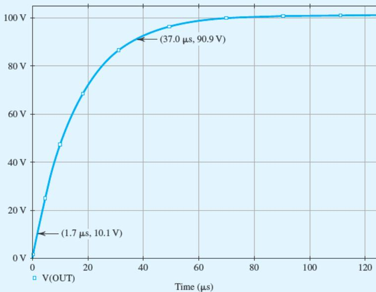
Figure B.8 Step response of the closed-loop amplifier in Example S.2.1.
