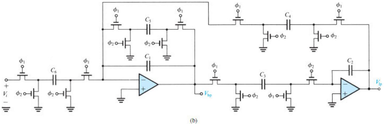
Figure 14.32 (b) The switched-capacitor counterpart of (a).
