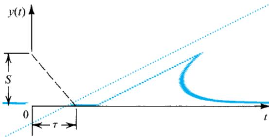
**Figure E.11** The output  $y(t)$  of a high-pass STC circuit excited by a step of height  $S$ .
