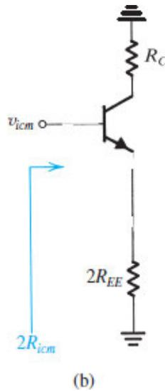
**Figure 9.26 (b)** The equivalent common-mode half-circuit.
