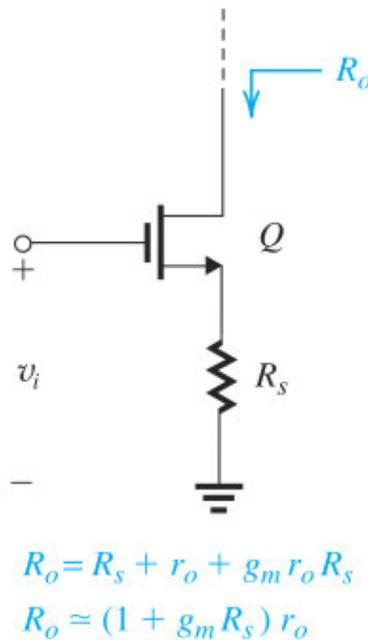
**Figure 8.23** The output resistance expression of the CG amplifier can be used to find the output resistance of a source-degenerated common-source amplifier. Here, a useful interpretation of the result is that  $R_s$  increases the output resistance by the factor  $(1 + g_m R_s)$ .
