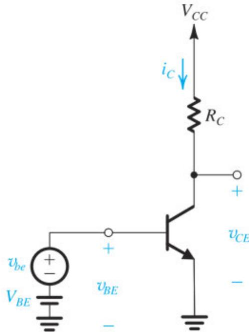
**Figure 7.6** BJT amplifier biased at a point Q, with a small voltage signal  $v_{be}$  superimposed on the dc bias voltage  $V_{BE}$ . The resulting output signal  $v_{ce}$  appears superimposed on the dc collector voltage  $V_{CE}$ . The amplitude of  $v_{ce}$  is larger than that of  $v_{be}$  by the voltage gain  $A_v$ .
