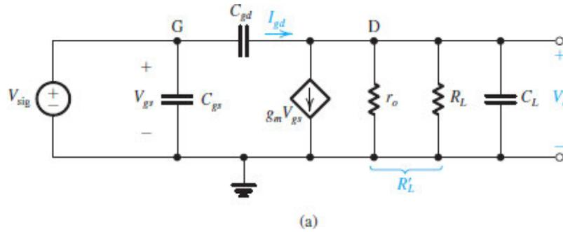
**Figure 10.12 (a)** High-frequency equivalent circuit of a CS amplifier fed with a signal source having a very low (effectively zero) resistance.
