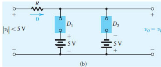
Figure 4.6 (b) The equivalent circuit when  $|v_I| < 5$  V.
