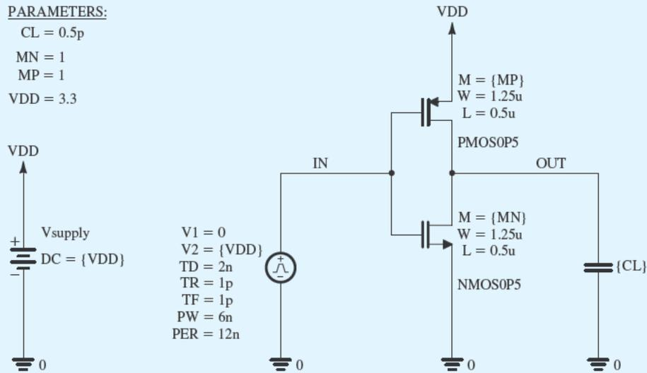
Figure B.76 Schematic capture of the CMOS inverter in Example S.16.1.
