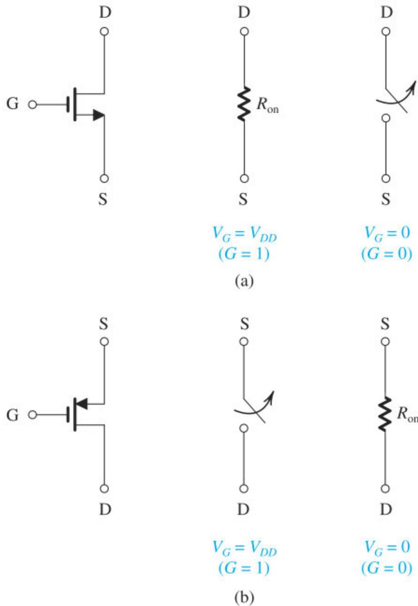
**Figure 16.1** Operation of the (a) NMOS and (b) PMOS transistor as an on/off switch. The gate voltage controls the operation of the transistor switch, with the voltage  $V_{DD}$  representing a logic 1 and 0 V representing a logic 0. Note that the connections of the drain and source terminals are not shown.
