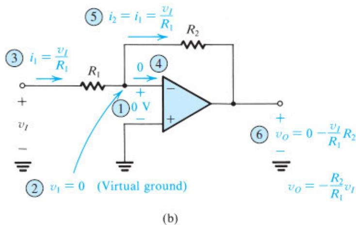
Figure 2.6 (b) Analysis of the inverting configuration. The circled numbers indicate the order of analysis steps.
