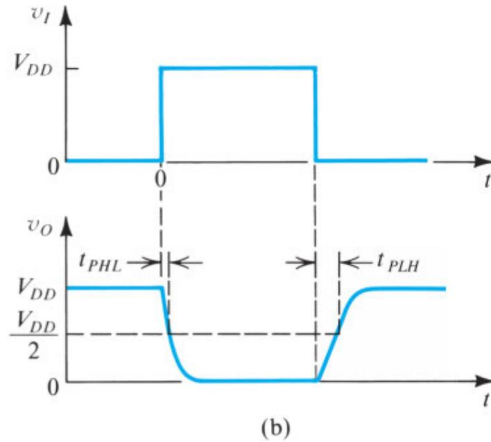
**Figure 17.4 (b)** Dynamic operation of a capacitively loaded CMOS inverter: input and output waveforms.
