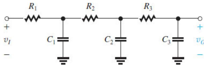
**Figure 18.10** A three-section RC ladder network used to illustrate Elmore delay.
