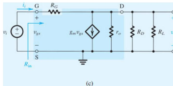
Figure 7.16 (c) Example 7.3: the amplifier small-signal equivalent circuit.
