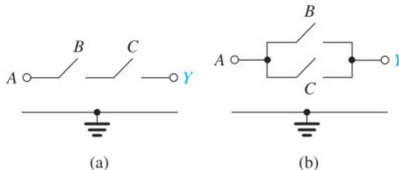
**Figure 18.1** Conceptual pass-transistor logic gates. **(a)** Two switches, controlled by the input variables  $B$  and  $C$ , when connected in series in the path between the input node to which an input variable  $A$  is applied and the output node (with an implied load to ground) realize the function  $Y = ABC$ . **(b)** When the two switches are connected in parallel, the function realized is  $Y = A(B + C)$ .
