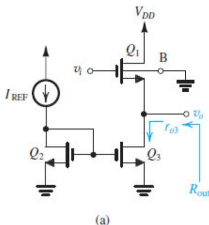
**Figure 8.35 (a)** A source follower biased with a current mirror  $Q_2$ – $Q_3$  and with the body terminal shown. Because the source cannot be connected to the body, the body effect should be taken into account.
