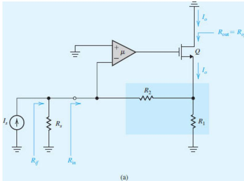
Figure 11.30 (a) Circuit for Example 11.10.
