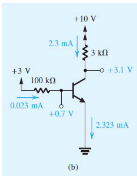
Figure 7.29 (b) Example 7.5: circuit for dc analysis.
