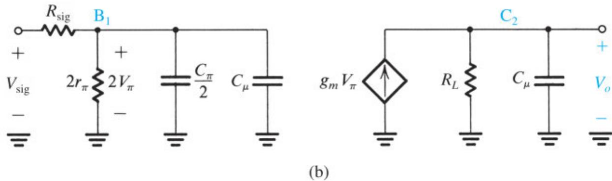
**Figure 10.35** (a) Equivalent circuit for the amplifier in Fig. 10.34(a). (b) Simplified equivalent circuit. Note that the equivalent circuits in (a) and (b) also apply to the circuit shown in Fig. 10.34(b). In addition, they can be easily adapted for the MOSFET circuit in Fig. 10.34(c), with  $2r_\pi$  eliminated,  $C_\pi$  replaced with  $C_{gs}$ ,  $C_\mu$  replaced with  $C_{gd}$ , and  $V_\pi$  replaced with  $V_{gs}$ .
