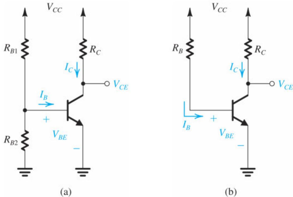
**Figure 7.53** Two obvious schemes for biasing the BJT: (a) by fixing  $V_{BE}$ ; (b) by fixing  $I_B$ . Both result in wide variations in  $I_C$  and hence in  $V_{CE}$  and therefore are considered to be “bad.” Neither scheme is recommended.
