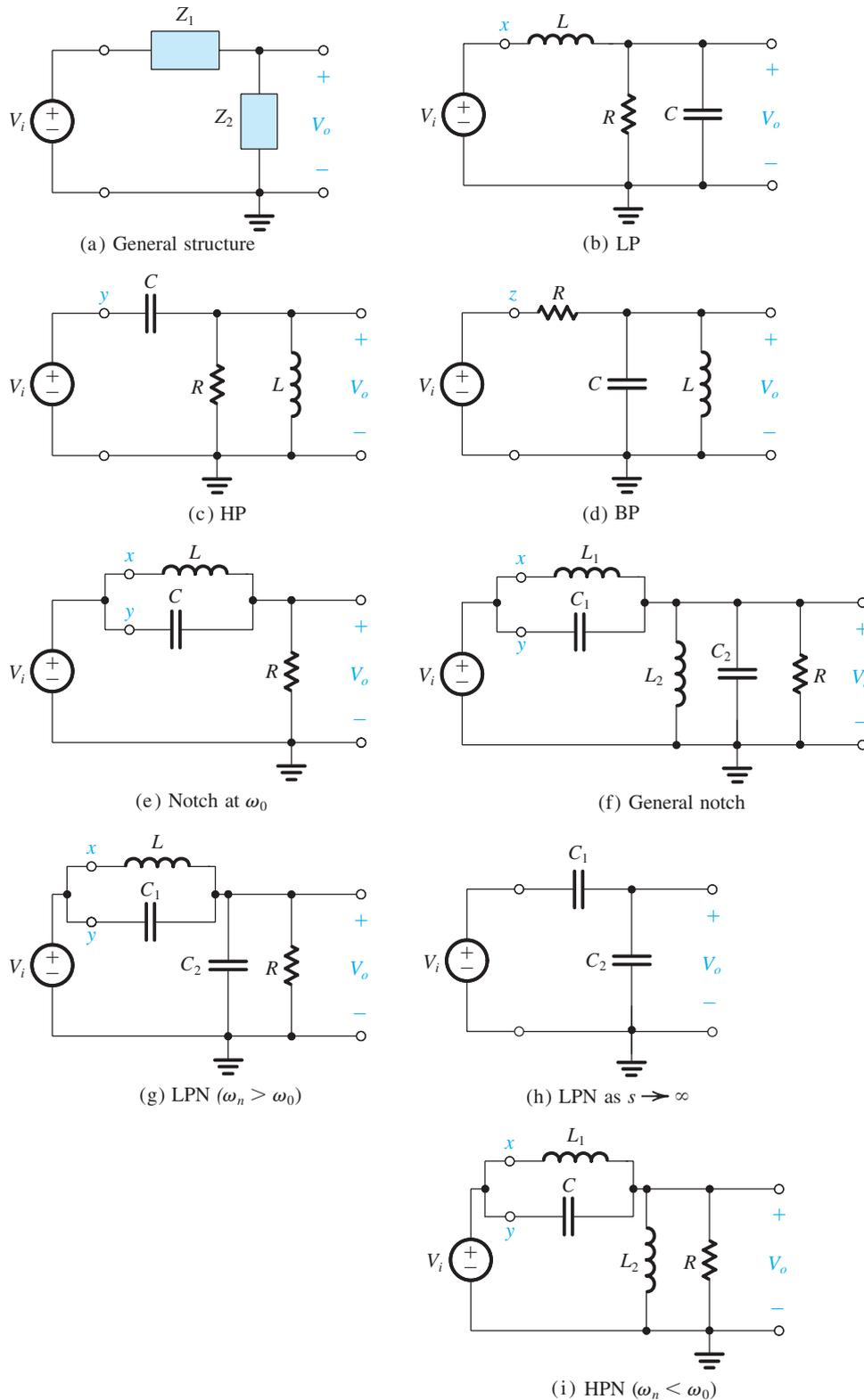
**Figure H.4** Realization of various second-order filter functions using the LCR resonator of Fig. 14.18(a): (a) general structure, (b) LP, (c) HP, (d) BP, (e) notch at  $\omega_0$ , (f) general notch, (g) LPN ( $\omega_n > \omega_0$ ), (h) LPN as  $s \rightarrow \infty$ , (i) HPN ( $\omega_n < \omega_0$ ).
