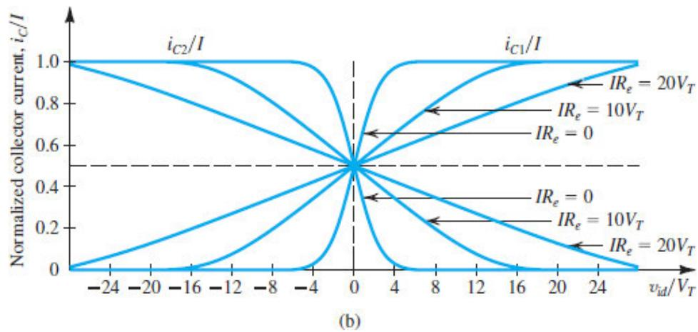
Figure 9.17 (b) The transfer characteristics of (a) can be linearized (i.e., the linear range of operation can be extended) by including resistances in the emitters.
