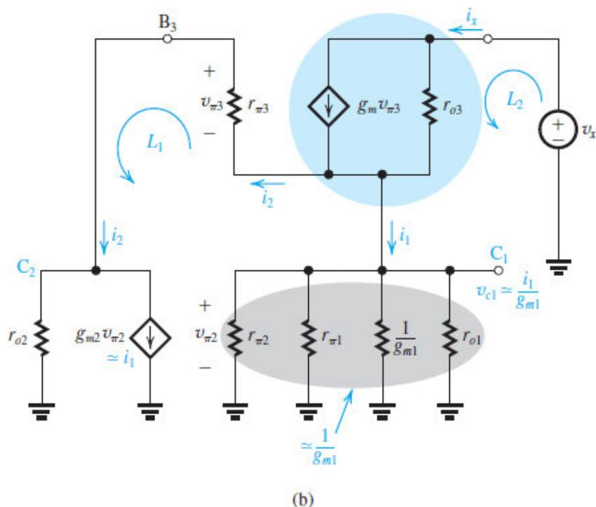
**Figure 8.37 (b)** The Wilson bipolar current mirror: determining the output resistance.
