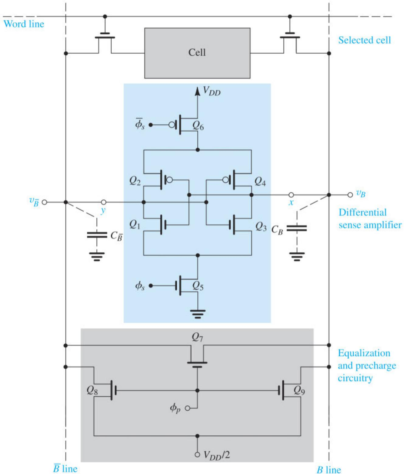
**Figure 18.34** A differential sense amplifier connected to the bit lines of a particular column. This arrangement can be used directly for SRAMs (which utilize both the  $B$  and  $\overline{B}$  lines). DRAMs can be turned into differential circuits by using a “dummy-cell” arrangement.
