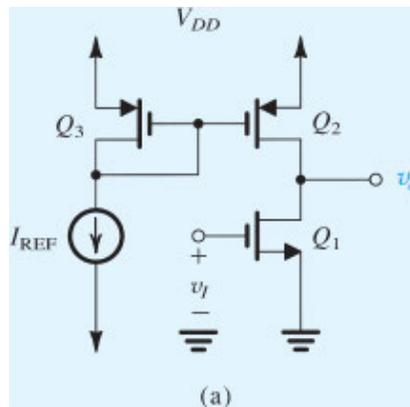
**Figure 8.16 (a)** Practical implementation of the common-source amplifier with a current-source load.
