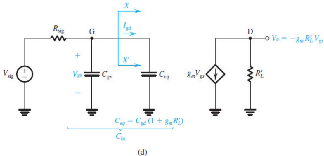
**Figure 10.11 (d)** The equivalent circuit with  $C_{gd}$  replaced at the input side with the equivalent capacitance  $C_{eq}$ .
