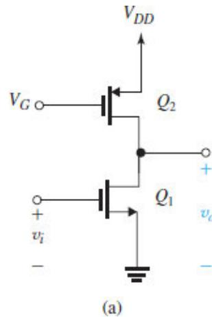
**Figure 8.15 (a)** The CS amplifier with the current-source load implemented with a  $p$ -channel MOSFET  $Q_2$ .
