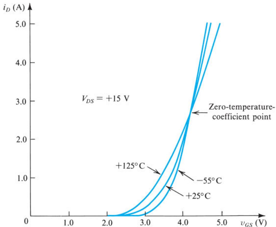
**Figure 12.28** The  $i_D$ - $v_{GS}$  characteristic curve of a power MOS transistor (IRF 630, Siliconix) at case temperatures of  $-55^\circ\text{C}$ ,  $+25^\circ\text{C}$ , and  $+125^\circ\text{C}$ . (Courtesy of Siliconix Inc.)
