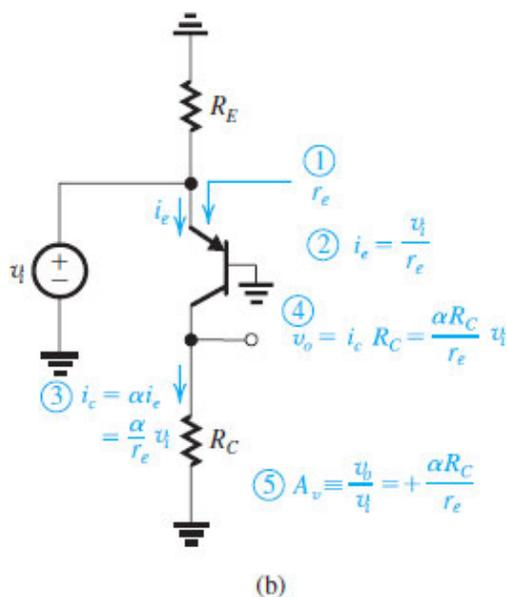
**Figure 7.33 (b)** Performing signal analysis directly on the circuit diagram with the BJT small-signal model implicitly employed: circuit for Example 7.7.
