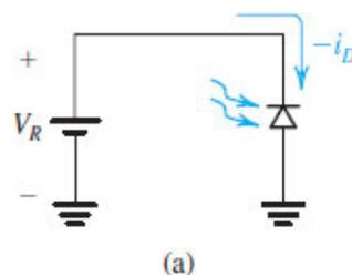
Figure 4.32 (a) Reverse-biased photodiode under illumination.
