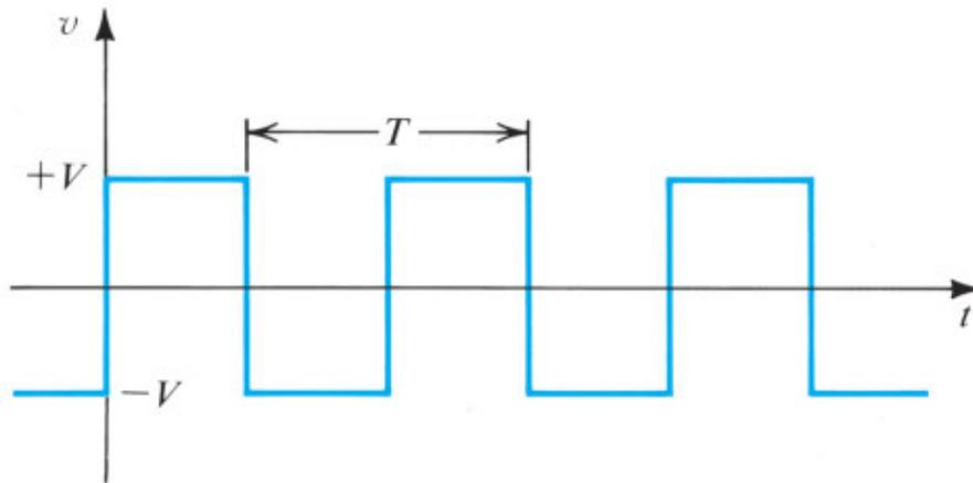
**Figure 1.5** A symmetrical square-wave signal of amplitude  $V$ .
