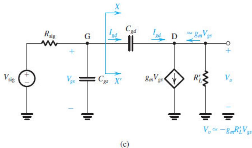
Figure 10.11 (c) The circuit of (b) simplified by combining  $R_L$  and  $r_o$  into a single resistance  $R'_L$ .
