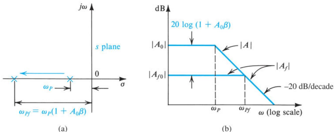
**Figure 11.32** Effect of feedback on (a) the pole location and (b) the frequency response of an amplifier having a single-pole, open-loop response.
