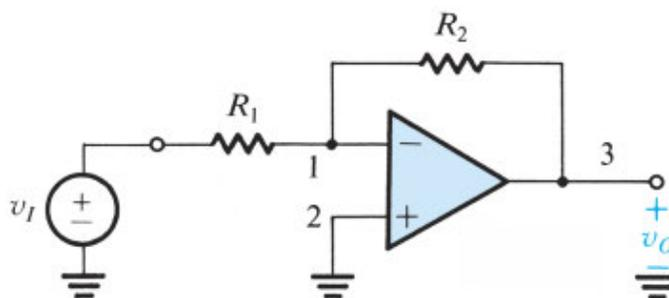
Figure 2.5 The inverting closed-loop configuration.
