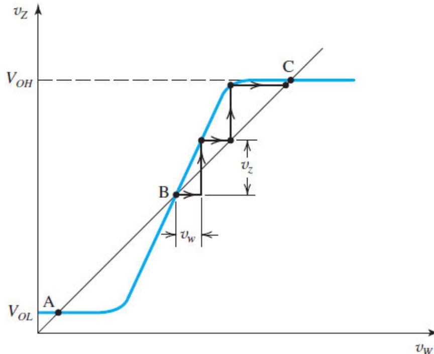
**Figure 18.12** Point B is an unstable operating point for the latch: A small positive increment  $v_w$  gets amplified around the loop and causes the operating point to shift to the stable operating point C. Had  $v_w$  been negative, the operating point would have shifted to the other stable point, A.
