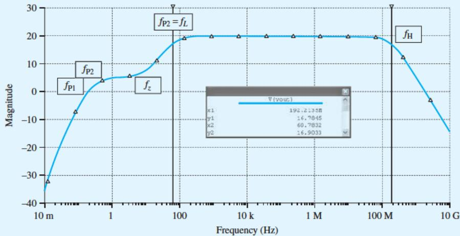
Figure B.41 Frequency response of the CS amplifier.
