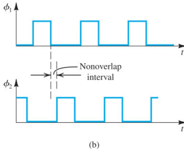
**Figure 18.20 (b)** Waveforms of the two-phase nonoverlapping clock required.
