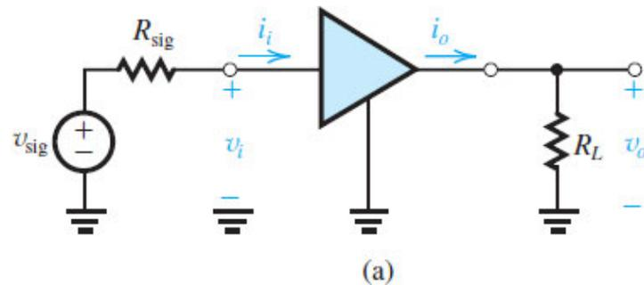
Figure 7.35 (a) Characterization of the amplifier as a functional block: An amplifier fed with a voltage signal  $v_{\text{sig}}$  having a source resistance  $R_{\text{sig}}$ , and feeding a load resistance  $R_L$ .
