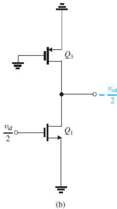
**Figure 9.12 (b)** Differential half-circuit of the amplifier in (a).
