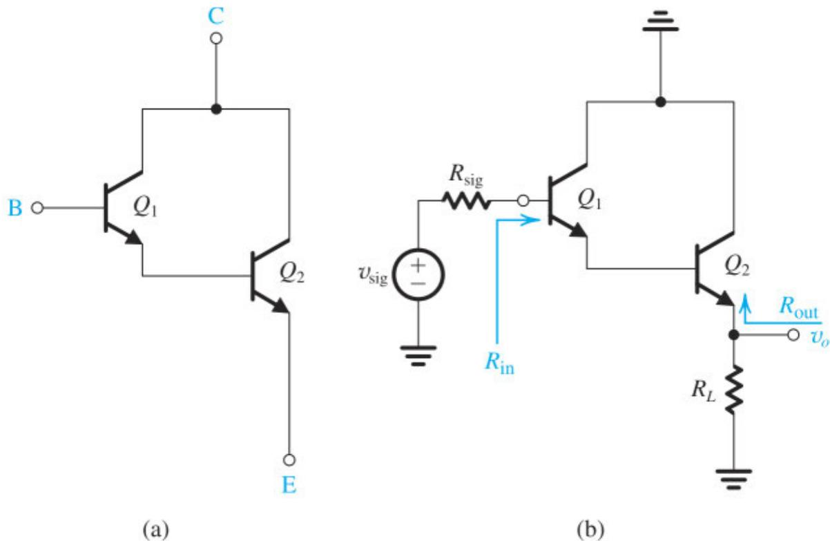
**Figure 7.48** (a) The Darlington configuration. (b) Voltage follower using the Darlington configuration.
