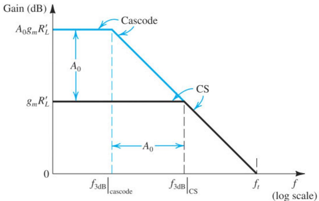
**Figure 10.21** Effect of cascoding on gain and bandwidth in the case  $R_{sig} = 0$ . Cascoding can increase the dc gain by a factor equal to the intrinsic gain  $A_0$  while keeping the unity-gain frequency constant. Note that to achieve the high gain, the load resistance must be increased by the factor  $A_0$ .
