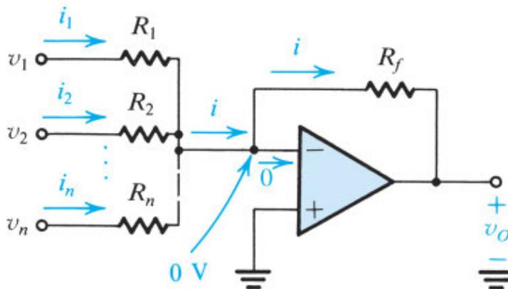
$$v_o = - \left( \frac{R_f}{R_1} v_1 + \frac{R_f}{R_2} v_2 + \dots + \frac{R_f}{R_n} v_n \right)$$
