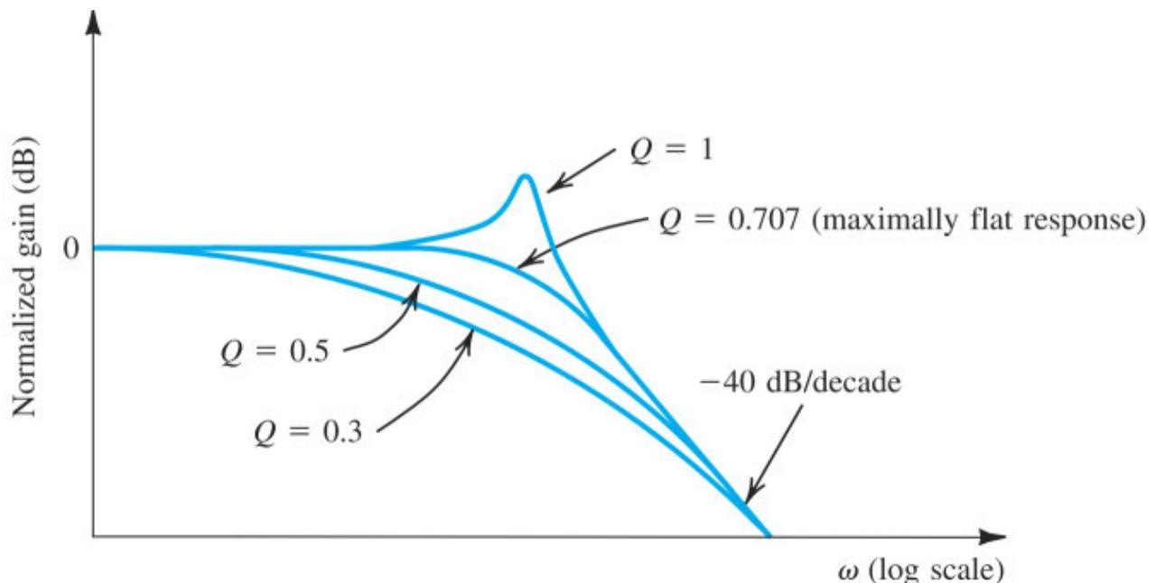
**Figure 11.35** Normalized gain of a two-pole feedback amplifier for various values of  $Q$ . Note that  $Q$  is determined by the loop gain according to Eq. (11.42).
