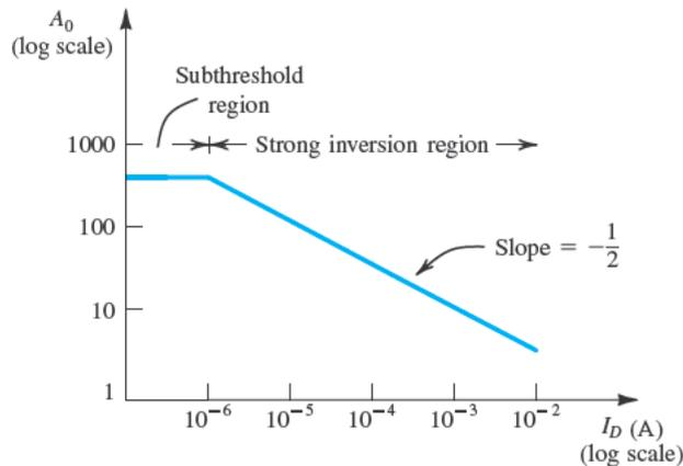
**Figure G.1** The intrinsic gain of the MOSFET versus bias current  $I_D$ . Outside the subthreshold region, this is a plot of  $A_0 = V'_A \sqrt{2\mu_n C_{ox} WL/I_D}$ , for the case:  $\mu_n C_{ox} = 20 \mu\text{A}/\text{V}^2$ ,  $V'_A = 20 \text{V}/\mu\text{m}$ ,  $L = 2 \mu\text{m}$ , and  $W = 20 \mu\text{m}$ .
