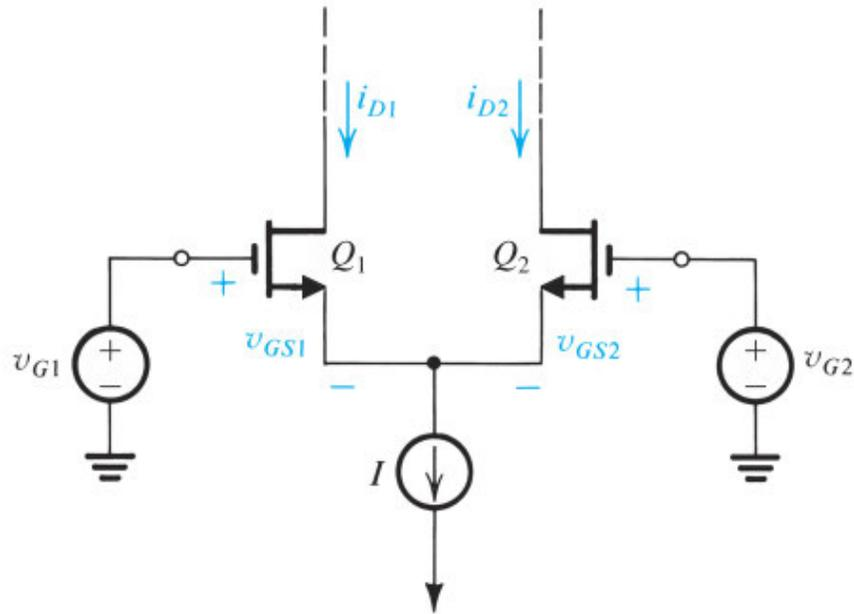
**Figure 9.5** The MOSFET differential pair for the purpose of deriving the transfer characteristics,  $i_{D1}$  and  $i_{D2}$  versus  $v_{id} = v_{G1} - v_{G2}$ .
