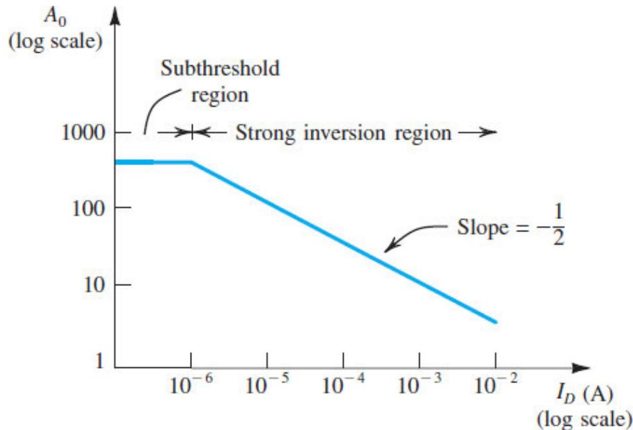
**Figure 8.14** The intrinsic gain of the MOSFET versus bias current  $I_D$ . Outside the subthreshold region, this is a plot of  $A_0 = V'_A \sqrt{2\mu_n C_{ox} W L I_D}$  for the case:  $\mu_n C_{ox} = 20 \mu\text{A}/\text{V}^2$ ,  $V'_A = 20 \text{V}/\mu\text{m}$ ,  $L = 2 \mu\text{m}$  and  $W = 20 \mu\text{m}$ .
