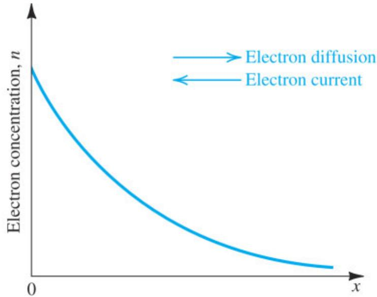
**Figure 3.7** If we establish the electron concentration profile shown in a bar of silicon, electrons diffuse in the  $x$  direction, giving rise to an electron diffusion current in the negative- $x$  direction.
