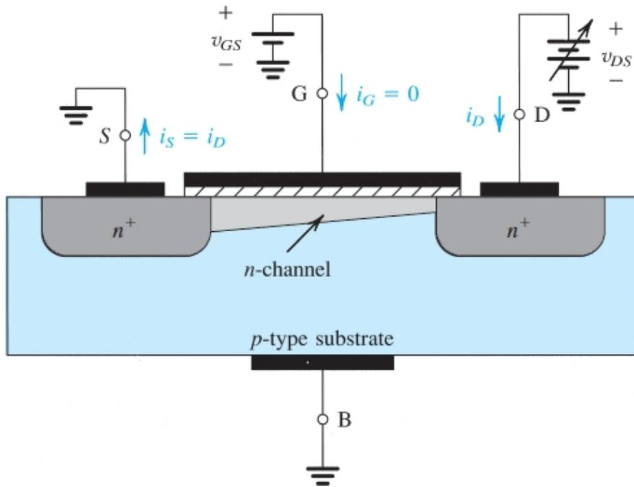
**Figure 5.5** Operation of the MOSFET as  $v_{DS}$  is increased. The induced channel acquires a tapered shape, and its resistance increases as  $v_{DS}$  is increased. Here,  $v_{GS}$  is kept constant at a value  $> V_t$ ;  $v_{GS} = V_t + v_{OV}$ . It is the widening of the depletion region (not shown) as a result of the increased  $V_{DS}$  that makes the channel shallower near the drain.
