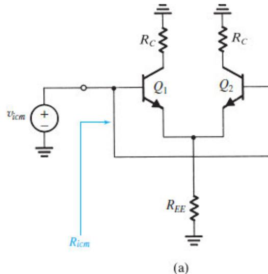
**Figure 9.26 (a)** Definition of the input common-mode resistance  $R_{icm}$ .
