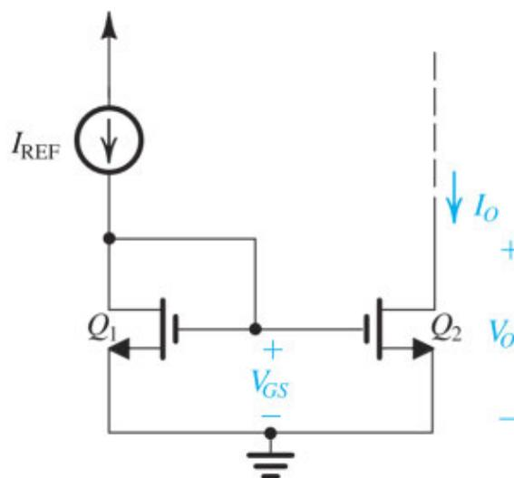
Figure 8.2 Basic MOSFET current mirror.
