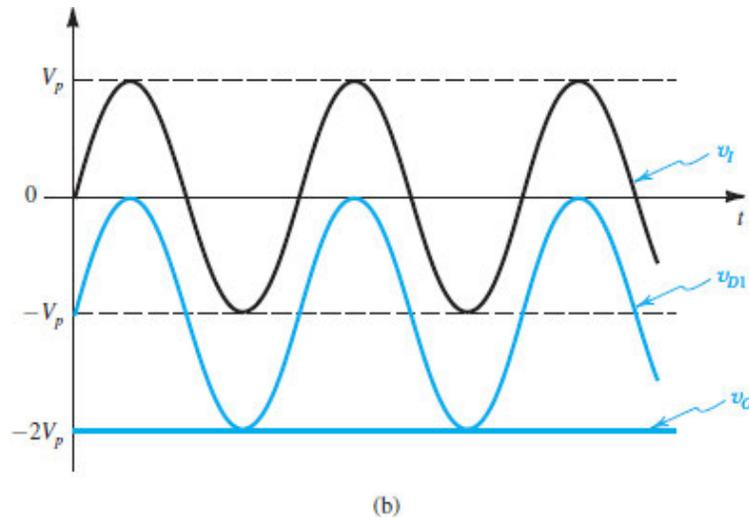
**Figure 4.31 (b)** Voltage doubler: waveforms of the input voltage, the voltage across  $D_1$ , and the output voltage  $v_o = -2V_p$ .
