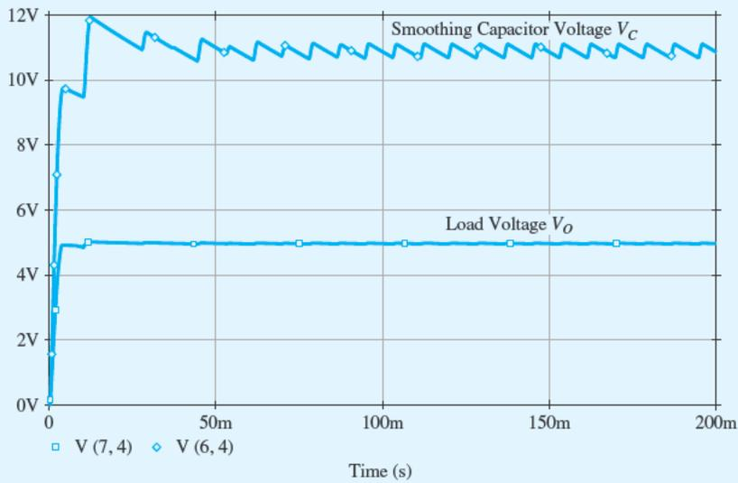
**Figure B.14** The voltage  $v_c$  across the smoothing capacitor  $C$  and the voltage  $v_o$  across the load resistor  $R_{\text{load}} = 200 \Omega$  in the 5-V power supply of Example S.4.1.
