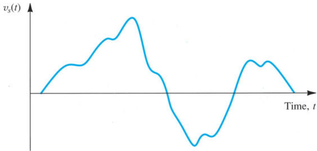
**Figure 1.3** An arbitrary voltage signal  $v_s(t)$ .
