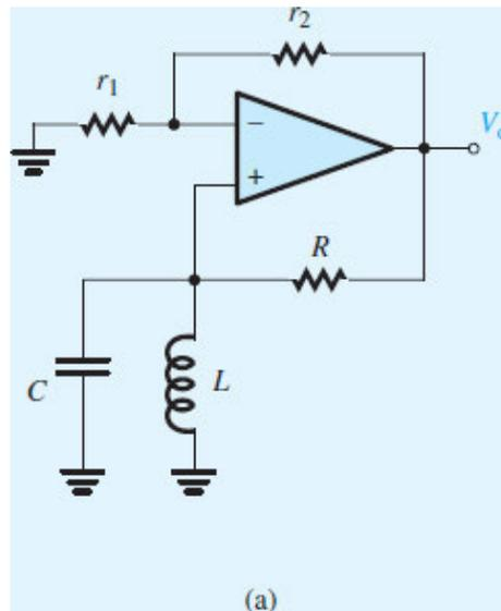
**Figure 15.2 (a)** An oscillator formed by connecting a positive-gain amplifier in a feedback loop with a bandpass RLC circuit.
