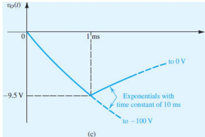
**Figure 2.27 (c)** Waveforms for Example 2.6: Output exponential ramp with resistor  $R_F$  connected across integrator capacitor.
