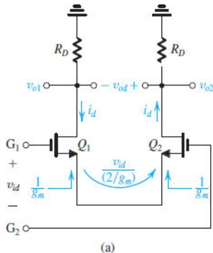
**Figure 9.9 (a)** An alternative view of the small-signal differential operation of the MOS differential pair: analysis done directly on the circuit.
