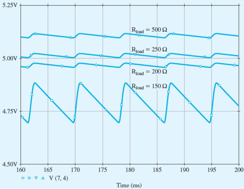
**Figure B.15** The output-voltage waveform from the 5-V power supply (in Example S.4.1) for various load resistances:  $R_{\text{load}} = 500 \Omega$ ,  $250 \Omega$ ,  $200 \Omega$ , and  $150 \Omega$ . The voltage regulation is lost at a load resistance of  $150 \Omega$ .
