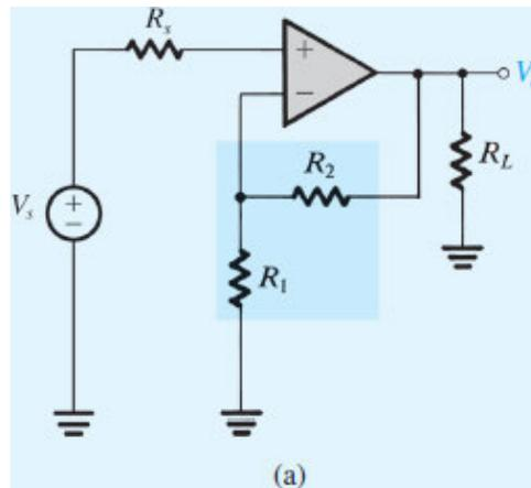
Figure 11.13 (a) A series–shunt feedback amplifier.
