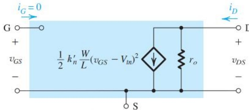
**Figure 5.18** Large-signal, equivalent-circuit model of the  $n$ -channel MOSFET in saturation, incorporating the output resistance  $r_o$ . The output resistance models the linear dependence of  $i_D$  on  $v_{DS}$  and is given by Eq. (5.27).
