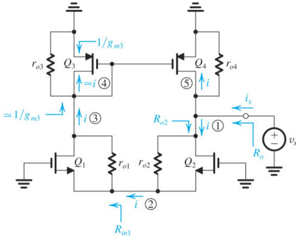
**Figure 9.34** Circuit for determining  $R_o$ . The circled numbers indicate the order of the analysis steps.
