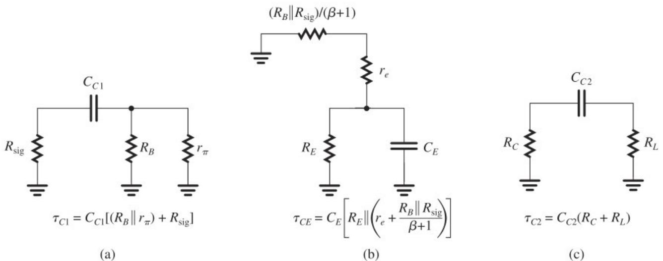
Figure 10.42 Circuits for determining the short-circuit time constants for the amplifier in Fig. 10.41.
