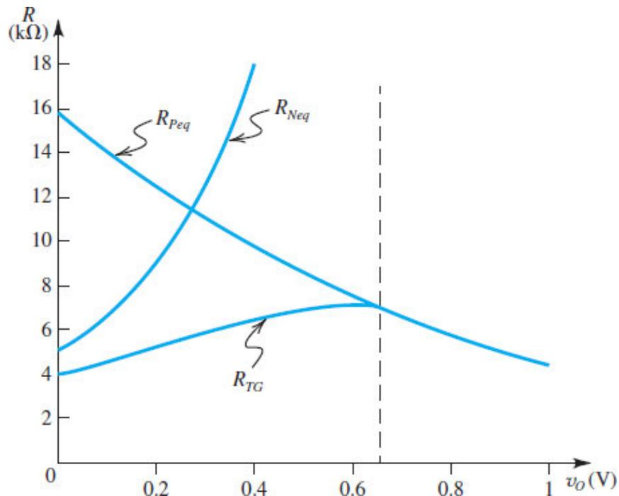
**Figure 18.8** Plot of the equivalent resistances of the two transistors of the transmission gate in Fig. 18.7(a) passing a high input, and the overall resistance  $R_{TG}$  versus  $v_O$ . The data apply to the situation specified in Exercise 18.3.
