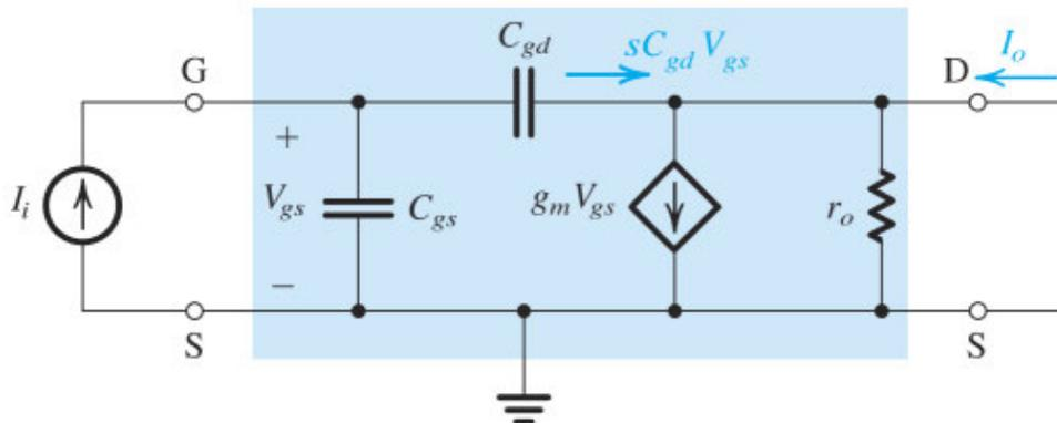
**Figure 10.5** Determining the short-circuit current gain  $I_o/I_i$ .
