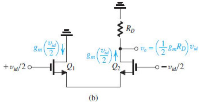
**Figure 9.30 (b)** The circuit with the power supplies eliminated for signal calculations. Note that the current signal in  $Q_1$  is not utilized, and as a result, the gain achieved is 6 dB lower than the differential-output case.
