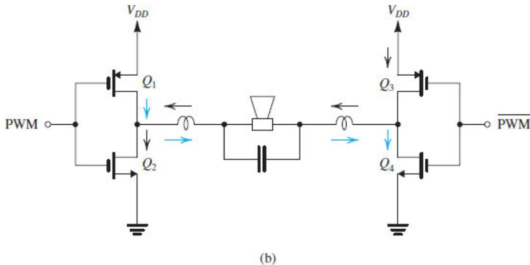
**Figure 12.24** Two schemes for driving the load of a class D amplifier. The differential scheme in (b) results in doubling the voltage excursion across the load.
