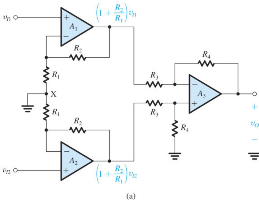
**Figure 2.20 (a)** A popular circuit for an instrumentation amplifier: Initial approach to the circuit.
