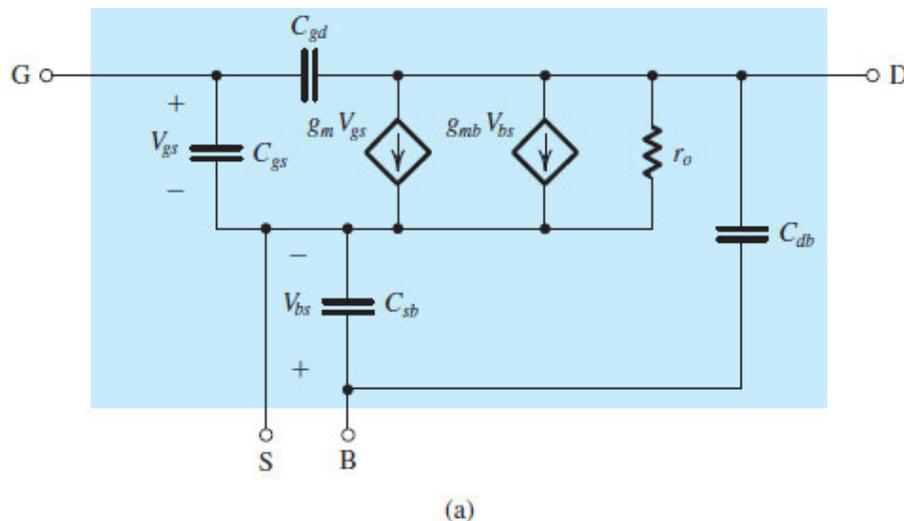
**Figure 10.4 (a)** High-frequency, equivalent-circuit model for the MOSFET.
