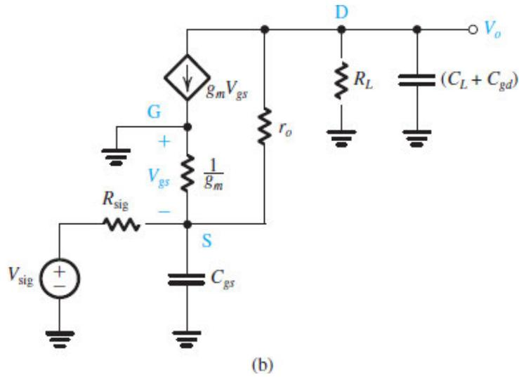
Figure 10.18 (b) Equivalent circuit of the CG amplifier with the MOSFET replaced with its T model.
