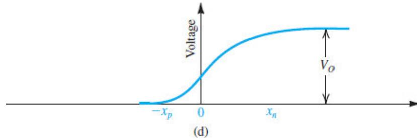
**Figure 3.10 (d)** The built-in voltage  $V_0$ .
