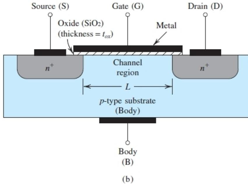
**Figure 5.1 (b)** Physical structure of the  $n$ -channel enhancement-type MOSFET: cross section. Typically,  $L = 20$  nm to  $1$   $\mu\text{m}$ ,  $W = 30$  nm to  $100$   $\mu\text{m}$ , and the thickness of the oxide layer ( $t_{ox}$ ) is in the range of  $1$  to  $10$  nm.
