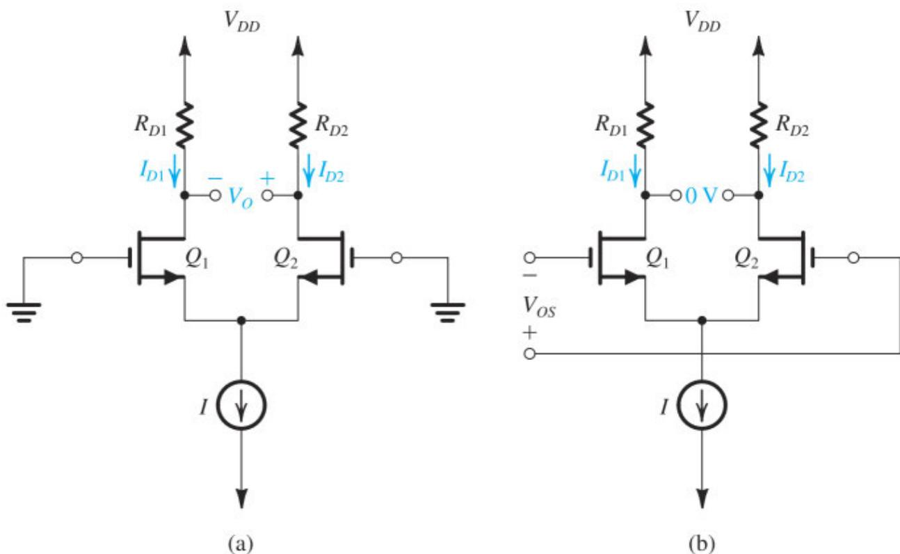
**Figure 9.27** (a) The MOS differential pair with both inputs grounded. Device and resistance mismatches result in a finite dc output  $V_O$ . (b) Application of the input offset voltage  $V_{OS}$  to the input terminals with appropriate polarity reduces  $V_O$  to zero.
