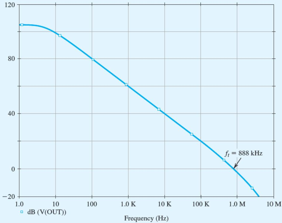
Figure B.10 Frequency response of the  $\mu$ A741 op amp in Example S.2.2.
