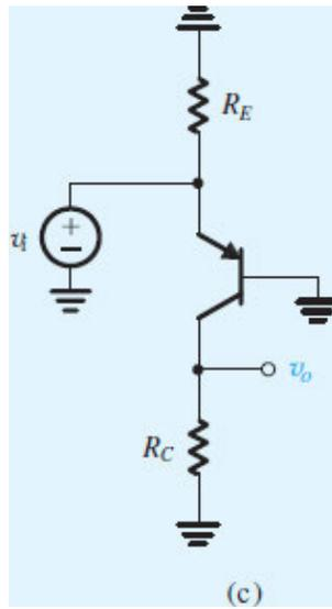
Figure 7.31 (c) Example 7.7: circuit with the dc sources eliminated.
