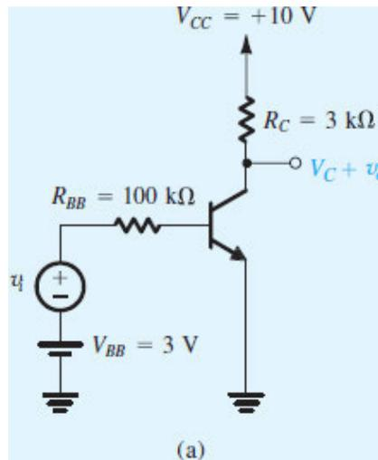
**Figure 7.29 (a)** Example 7.5: amplifier circuit.
