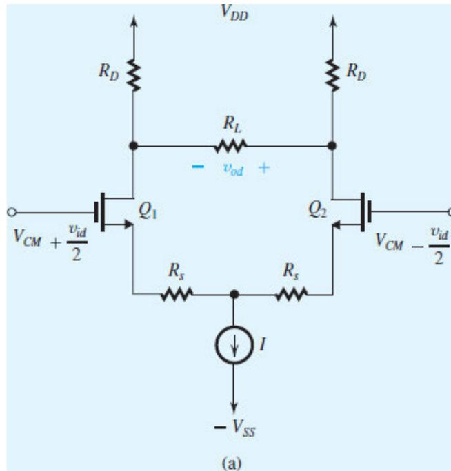
Figure 9.11 (a) Differential amplifier for Example 9.2.
