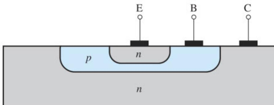
Figure 6.7 Cross section of an  $nnp$  BJT.
