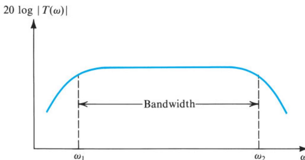
**Figure 1.21** Typical magnitude response of an amplifier:  $|T(\omega)|$  is the magnitude of the amplifier transfer function—that is, the ratio of the output  $V_o(\omega)$  to the input  $V_i(\omega)$ .
