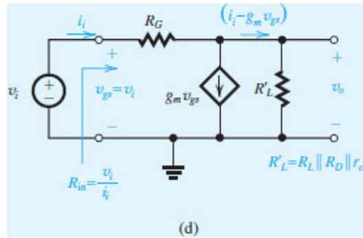
**Figure 7.16 (d)** Example 7.3: a simplified version of the circuit in (c).
