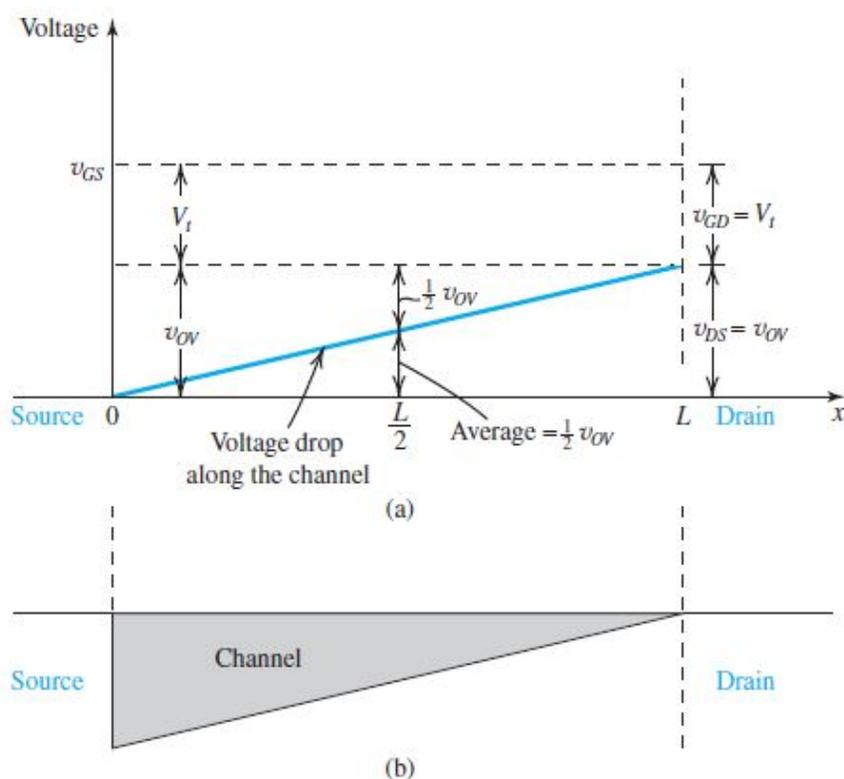
**Figure 5.8** Operation of MOSFET with  $v_{GS} = V_t + v_{OV}$ , as  $v_{DS}$  is increased to  $v_{OV}$ . At the drain end,  $v_{GD}$  decreases to  $V_t$  and the channel depth at the drain end reduces to zero (pinch-off). At this point, the MOSFET enters the saturation mode of operation. Further increasing  $v_{DS}$  (beyond  $v_{DSsat} = v_{OV}$ ) has no effect on the channel shape and  $i_D$  remains constant.
