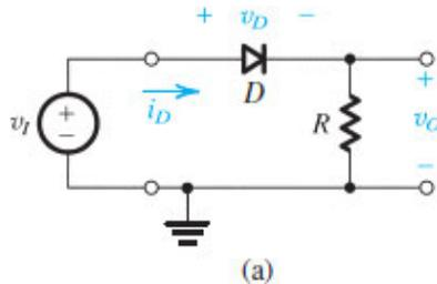
Figure 4.3 (a) Rectifier circuit.
