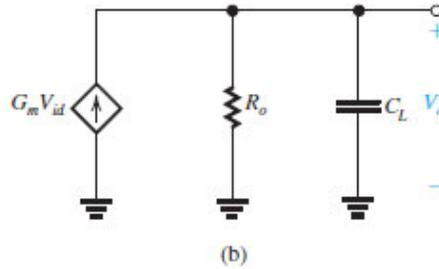
**Figure 10.29 (b)** Output equivalent circuit.
