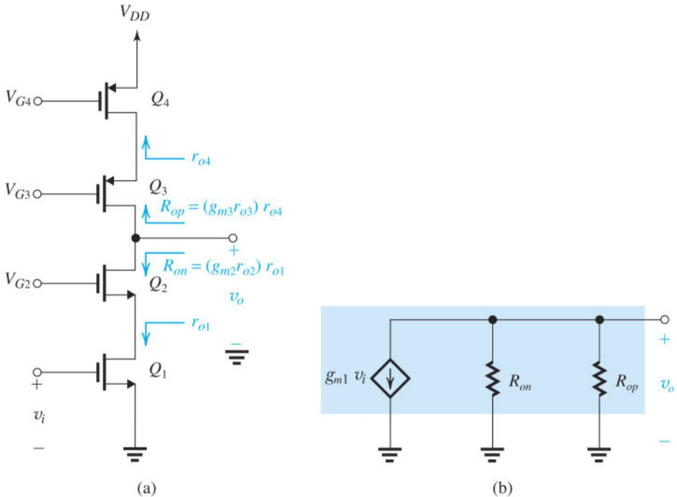
**Figure 8.31** A cascode amplifier with a cascode current-source load.
