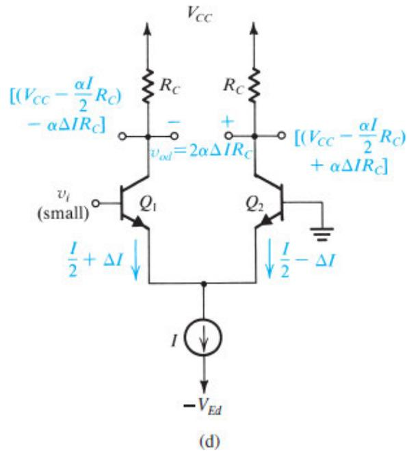
**Figure 9.15 (d)** Different modes of operation of the BJT differential pair: the differential pair with a small differential input signal  $v_i$ . Note that we have assumed the bias current source  $I$  to be ideal (i.e., it has an infinite output resistance) and thus  $I$  remains constant with the change in the voltage across it.
