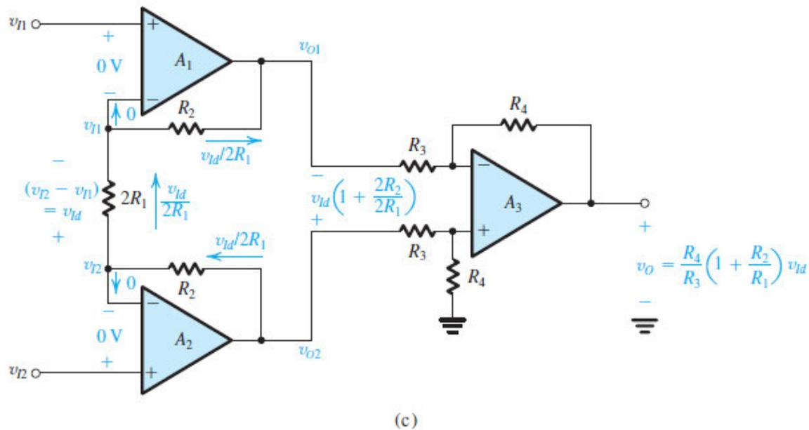
**Figure 2.20 (c)** A popular circuit for an instrumentation amplifier: Analysis of the circuit in (b) assuming ideal op amps.
