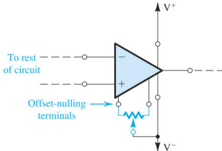
**Figure 2.31** The output dc offset voltage of an op amp can be trimmed to zero by connecting a potentiometer to the two offset-nulling terminals. The wiper of the potentiometer is connected to the negative supply of the op amp.
