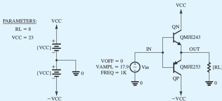
Figure B.54 Capture schematic of the class B output stage in Example S.12.1.
