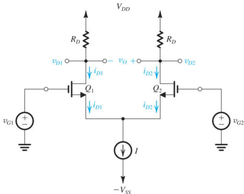
**Figure 9.1** The basic MOS differential-pair configuration.
