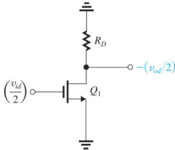
**Figure 9.10** The equivalent differential half-circuit of the differential amplifier of Fig. 9.8. Here  $Q_1$  is biased at  $I/2$  and is operating at  $V_{OV}$ . This circuit can be used to determine the differential voltage gain of the differential amplifier  $A_d = v_{od}/v_{id}$ .
