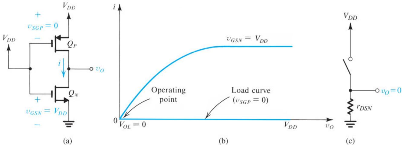
**Figure 16.23** Operation of the CMOS inverter when  $v_I$  is high: (a) circuit with  $v_I = V_{DD}$  (logic-1 level, or  $V_{OH}$ ); (b) graphical construction to determine the operating point; (c) equivalent circuit.
