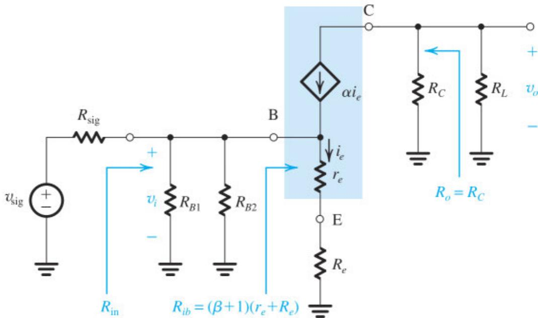
$$G_v = - \frac{R_{in}}{R_{in} + R_{sig}} \times \alpha \frac{(R_C || R_L)}{r_e + R_e}$$
