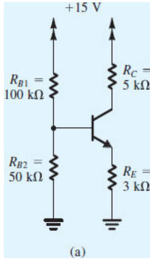
Figure 6.29 (a) Circuit for Example 6.10.
