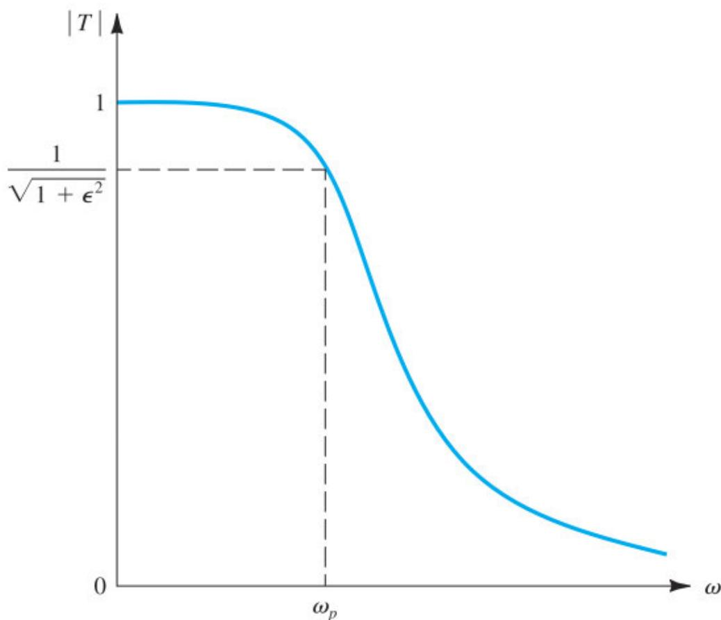
Figure 14.13 The magnitude response of a Butterworth filter.
