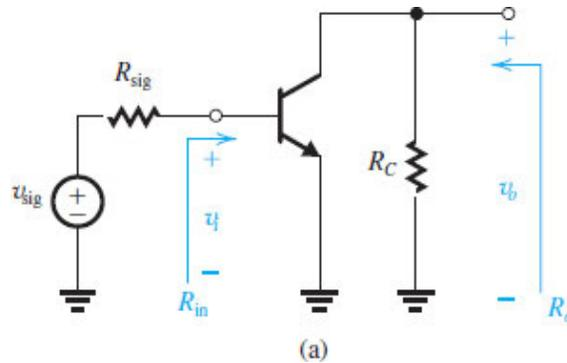
**Figure 7.37 (a)** Common-emitter amplifier fed with a signal  $v_{sig}$  from a generator with a resistance  $R_{sig}$ . The bias circuit is omitted.
