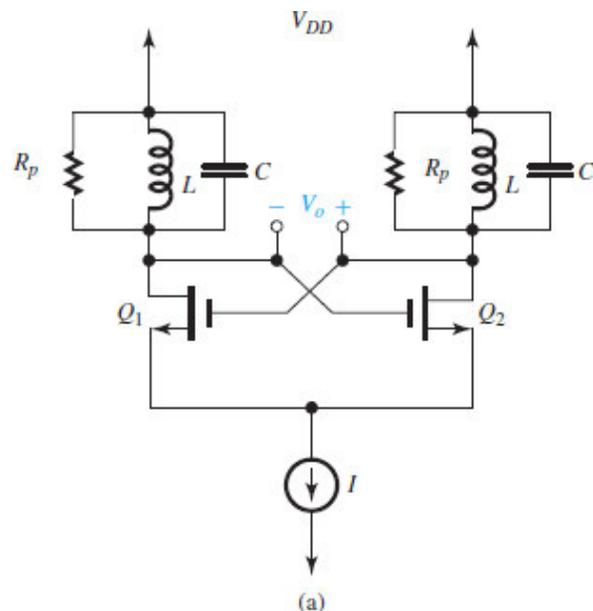
**Figure 15.16 (a)** The cross-coupled LC oscillator.
