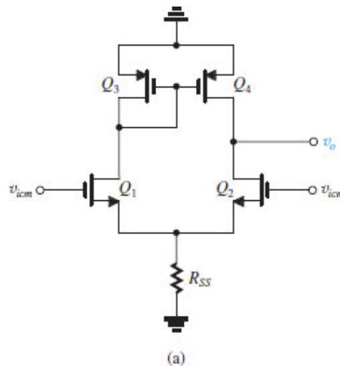
**Figure 9.36 (a)** Analysis of the current-mirror-loaded MOS differential amplifier to determine its common-mode gain: The circuit with  $v_{icm}$  applied and the dc sources removed.
