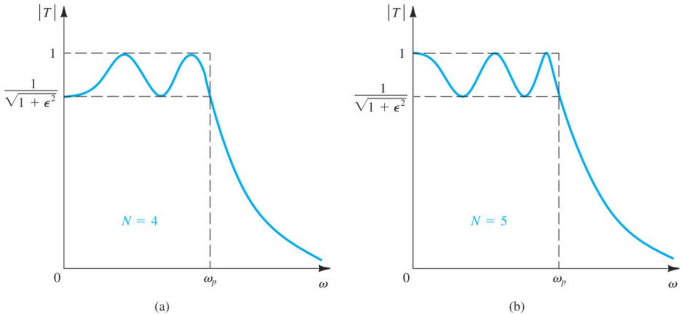
**Figure 14.17** Sketches of the transmission characteristics of representative (a) even-order and (b) odd-order Chebyshev filters.
