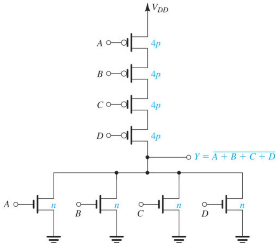
**Figure 17.8** Proper transistor sizing for a four-input NOR gate. Note that  $n$  and  $p$  denote the  $W/L$  ratios of  $Q_N$  and  $Q_P$ , respectively, of the basic inverter.
