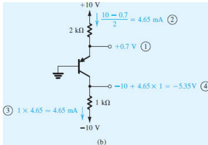
Figure 6.26 (b) Example 6.7: analysis with steps numbered. The value of  $\beta$  is assumed to be infinite.
