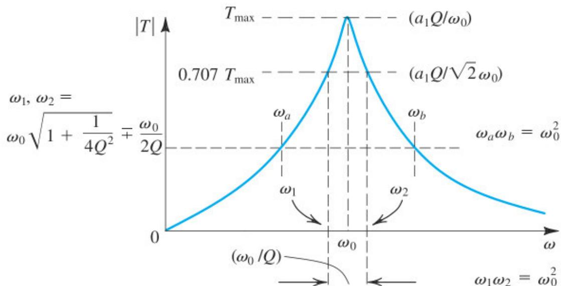
**Figure 14.11** Magnitude response of a second-order bandpass filter.
