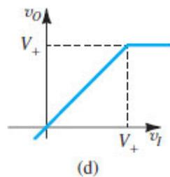
**Figure 4.5 (d)** The resulting input-output relationship.
