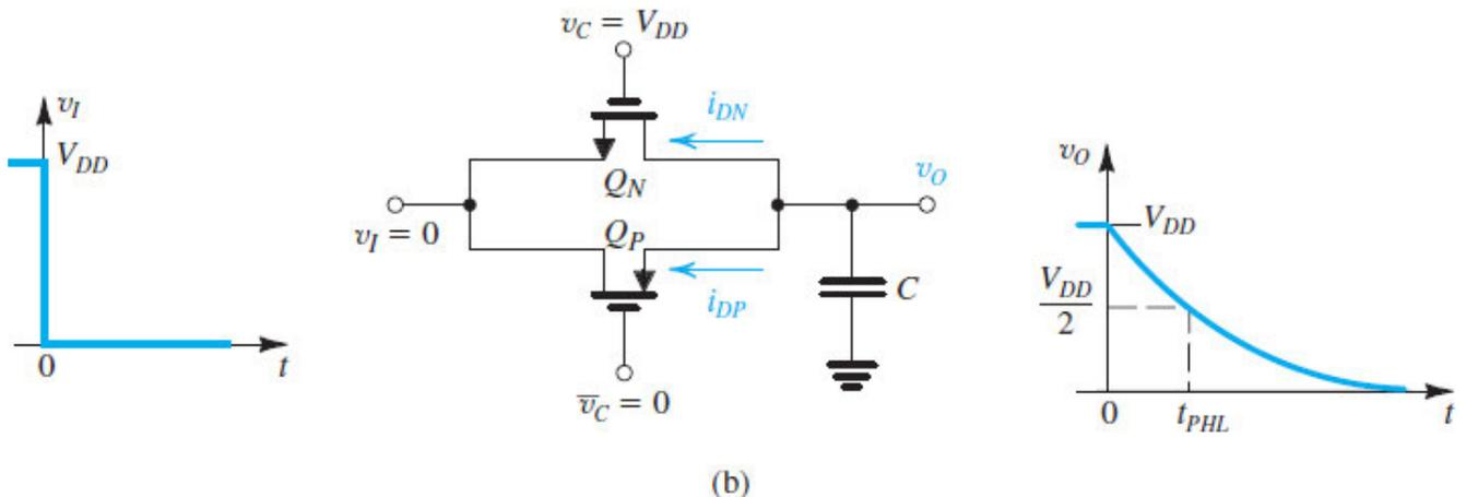
**Figure 18.7 (b)** Operation of the transmission gate as a switch with  $v_I$  low.
