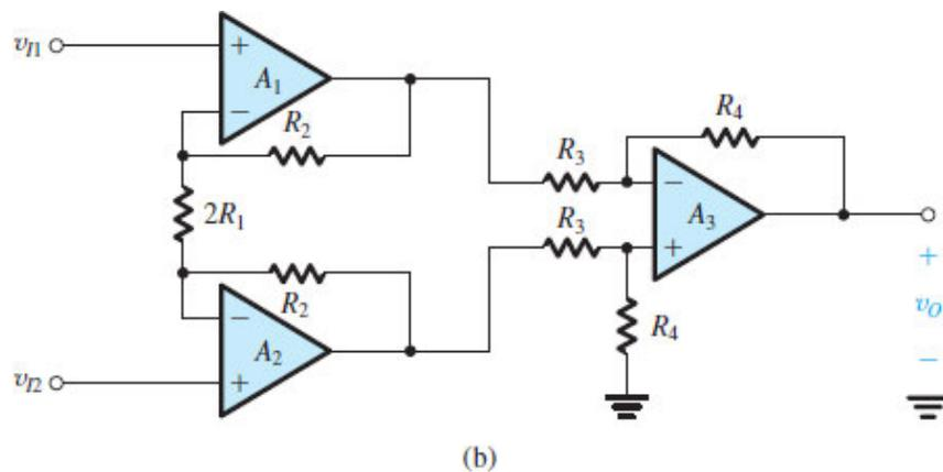
**Figure 2.20 (b)** A popular circuit for an instrumentation amplifier: The circuit in (a) with the connection between node X and ground removed and the two resistors  $R_1$  and  $R_1$  lumped together.
