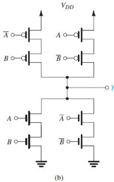
**Figure 16.10 (b)** Realization of the exclusive-OR (XOR) function. The complete XOR realization utilizing the PUN in (a) and a PDN that is synthesized directly from the expression in Eq. (16.6). Note that two inverters (not shown) are
