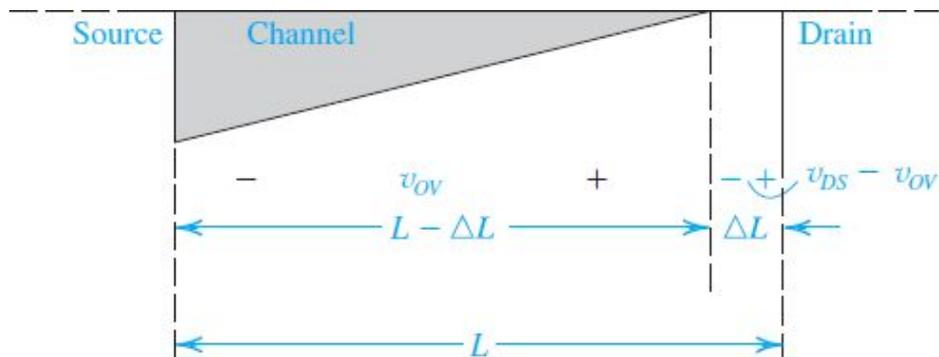
**Figure 5.16** Increasing  $v_{DS}$  beyond  $v_{DSsat}$  (which is equal to  $v_{OV}$ ) causes the channel pinch-off point to move slightly away from the drain, thus reducing the effective channel length (by  $\Delta L$ ).
