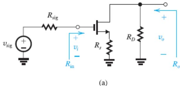
**Figure 7.38 (a)** The CS amplifier with a source resistance  $R_s$ : circuit without bias details.
