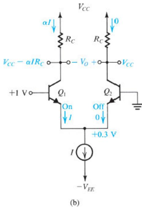
**Figure 9.15 (b)** Different modes of operation of the BJT differential pair: the differential pair with a “large” differential input signal.
