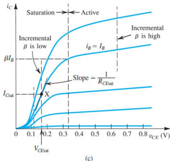
**Figure 6.20 (c)** Common-emitter characteristics. Common-emitter characteristics: Showing a much greater expansion of the saturation region.
