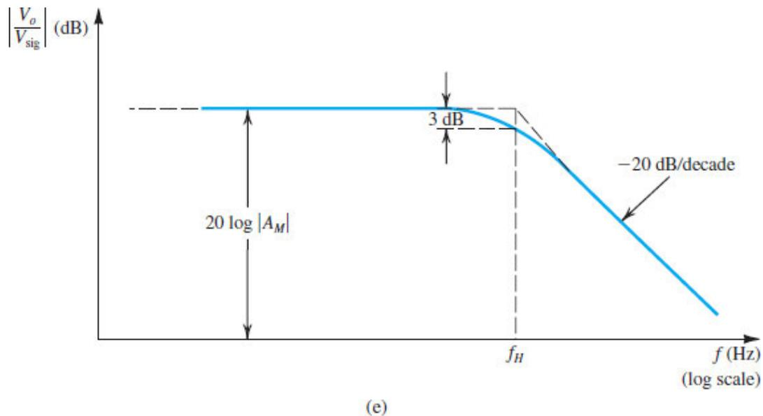
**Figure 10.11 (e)** The frequency-response plot, which is that of a low-pass, single-time-constant circuit.
