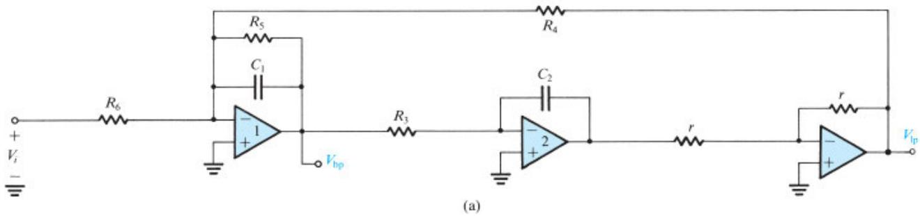
Figure 14.32 (a) A two-integrator-loop, active-RC biquad.
