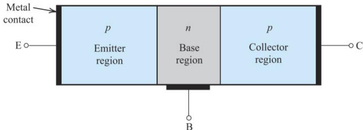
Figure 6.2 A simplified structure of the  $pnp$  transistor.
