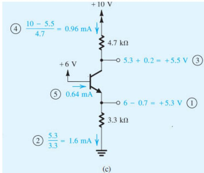
**Figure 6.24 (c)** Analysis of the circuit for Example 6.5. The circled numbers indicate the order of analysis steps.
