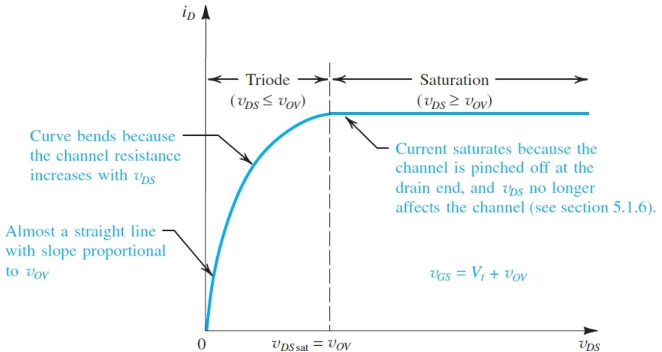
**Figure 5.7** The drain current  $i_D$  versus the drain-to-source voltage  $v_{DS}$  for an enhancement-type NMOS transistor operated with  $v_{GS} = V_t + v_{OV}$ .
