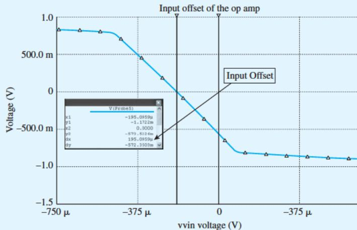
Figure B.36 Input offset voltage of the two-stage CMOS op amp.
