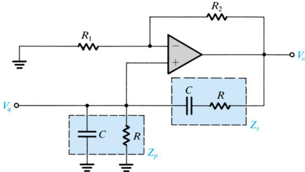
**Figure 15.6** A Wien-bridge oscillator without amplitude stabilization.
