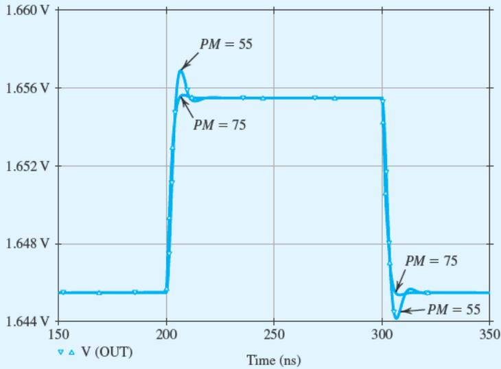
**Figure B.64** Small-signal step response (for a 10-mV step input) of the op-amp circuit in Fig. B.60 connected in a unity-gain configuration:  $PM = 55^\circ$  ( $C_c = 0.6$  pF,  $R = 1.53$  k $\Omega$ ) and  $PM = 75^\circ$  ( $C_c = 0.6$  pF,  $R = 3.2$  k $\Omega$ ).
