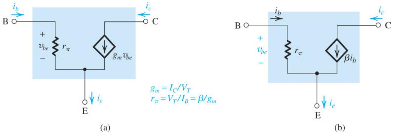
**Figure 7.25** Two slightly different versions of the hybrid- $\pi$  model for the small-signal operation of the BJT. The equivalent circuit in (a) represents the BJT as a voltage-controlled current source (a transconductance amplifier), and that in (b) represents the BJT as a current-controlled current source (a current amplifier).
