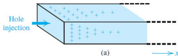
**Figure 3.6** A bar of silicon (a) into which we inject holes, thus creating the hole concentration profile along the  $x$  axis, shown in (b). The holes diffuse in the positive direction of  $x$  and give rise to a hole diffusion current in the same
