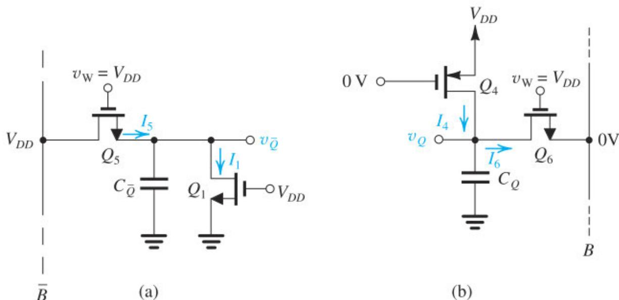
**Figure 18.26** Relevant parts of the 6T SRAM circuit of Fig. 18.22 during the process of writing a 0. It is assumed that the cell is originally storing a 1 and thus initially  $v_Q = V_{DD}$  and  $v_{\bar{Q}} = 0\text{ V}$ .
