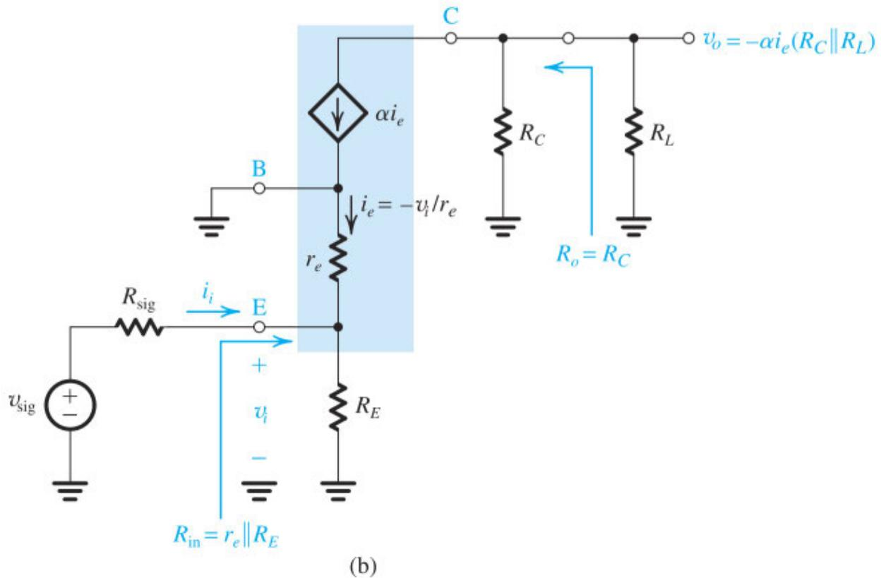
**Figure 7.60 (b)** Equivalent circuit obtained by replacing the transistor with its T model.
