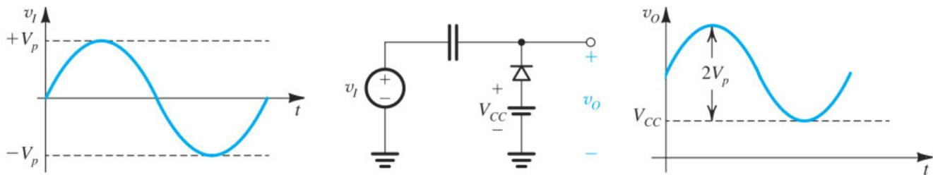
**Figure 4.30** Simple bootstrapping circuit using a clamped capacitor.
