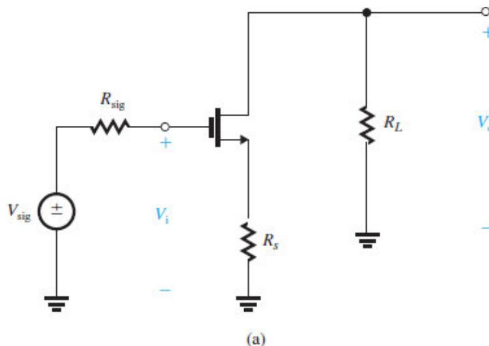
**Figure 10.30 (a)** The CS amplifier circuit, with a source resistance  $R_s$ .
