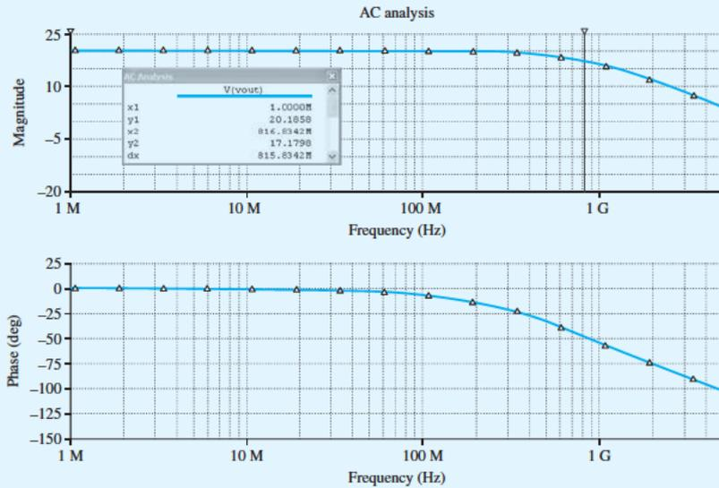
Figure B.53 Frequency response of the closed-loop circuit.
