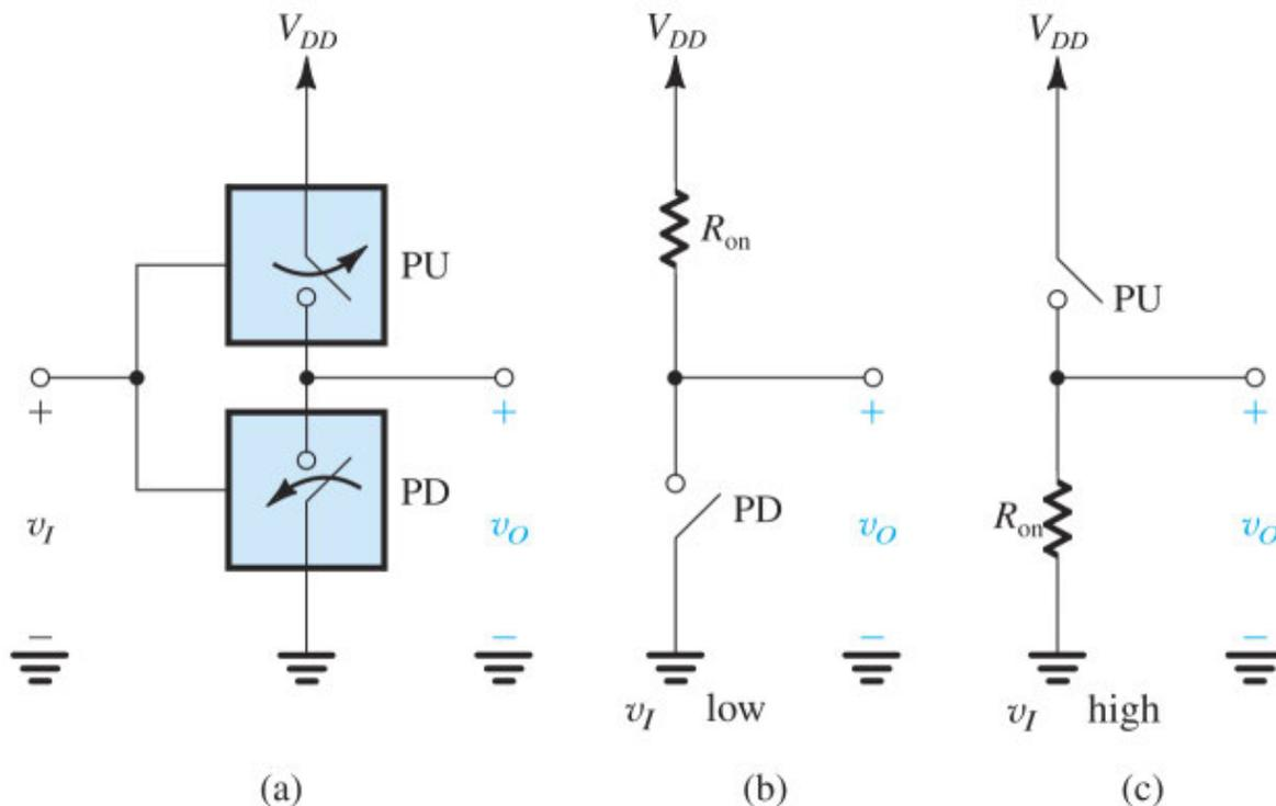
**Figure 16.18** A more elaborate implementation of the logic inverter utilizing two complementary switches. This is the basis of the CMOS inverter that we synthesized in the previous section [Fig. 16.2(b)] and shall study in Section 16.3.
