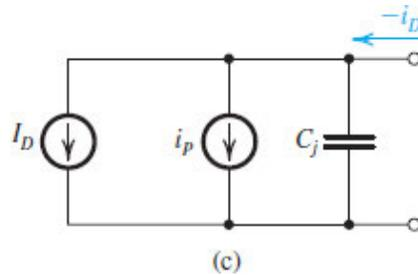
**Figure 4.32** (c) Model of the photodiode under illumination with dark current  $I_D$  and photocurrent  $i_p$ .
