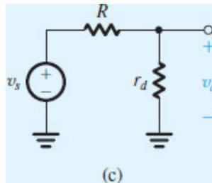
**Figure 4.17 (c)** Small-signal equivalent circuit.
