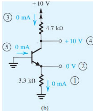
Figure 6.25 (b) Example 6.6: analysis with steps numbered.
