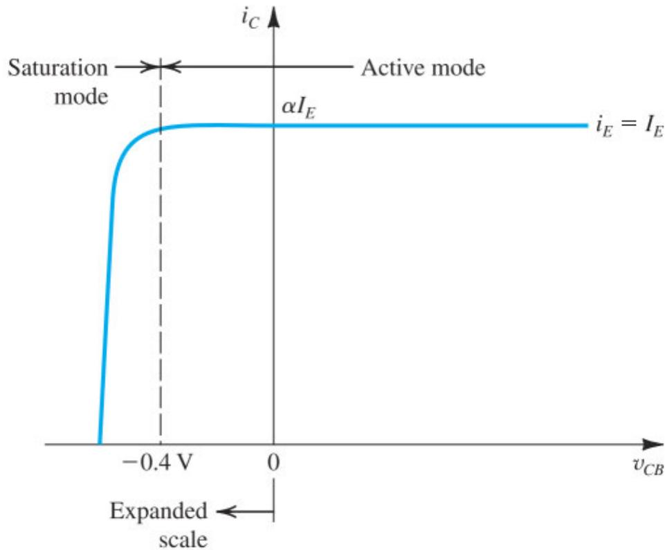
**Figure 6.8** The  $i_C$ - $v_{CB}$  characteristic of an  $npn$  transistor fed with a constant emitter current  $I_E$ . The transistor enters the saturation mode for  $v_{CB} < -0.4$  V, and the collector current diminishes.
