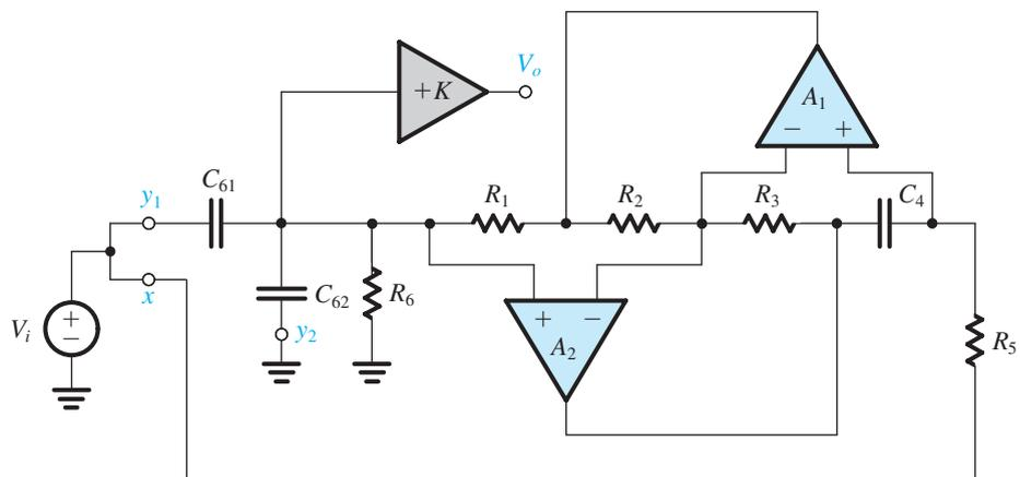
(e) LPN,  $\omega_n \geq \omega_0$
