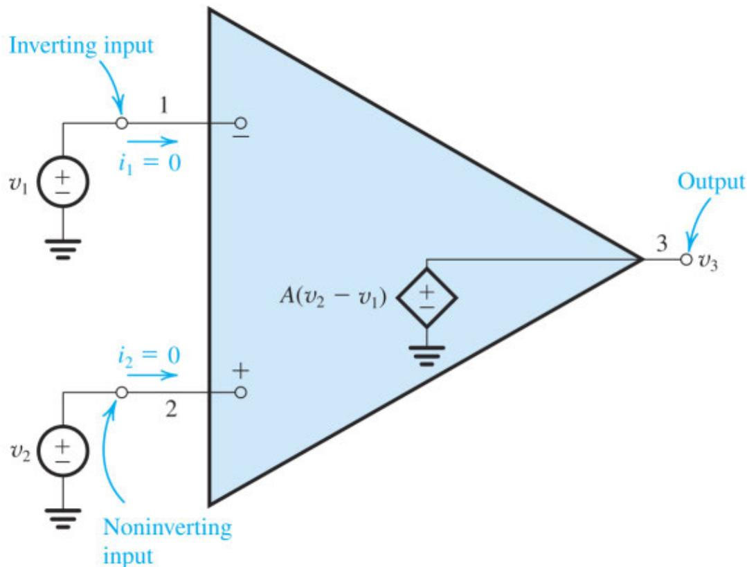
**Figure 2.3** Equivalent circuit of the ideal op amp.
