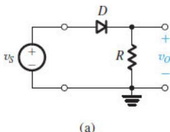
Figure 4.21 (a) Half-wave rectifier.
