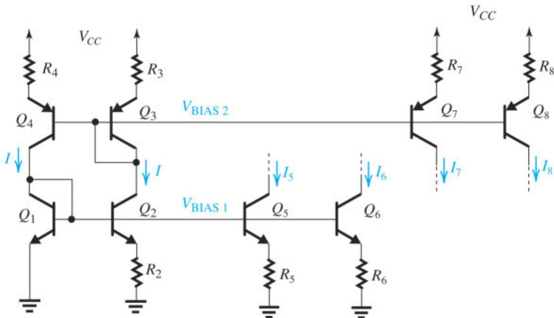
**Figure 13.14** A self-biased current-reference source using a Widlar circuit to generate  $I = (V_T/R_2) \ln(I_{S2}/I_{S1})$ . The bias voltages  $V_{BIAS1}$  and  $V_{BIAS2}$  are used to generate bias currents  $I_{5-8}$  used elsewhere in the op amp.
