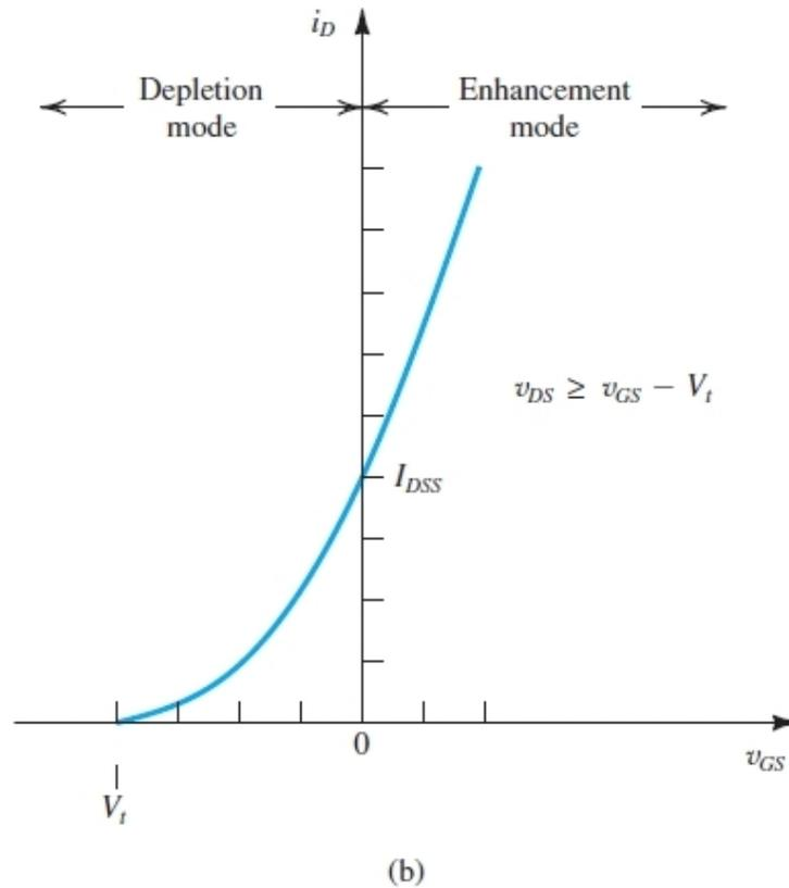
**Figure 5.29 (b)** The  $i_D - v_{GS}$  characteristic in saturation for an n-channel depletion-type MOSFET. Note that  $I_{DSS}$  denotes the drain current when  $v_{GS} = 0$ .
