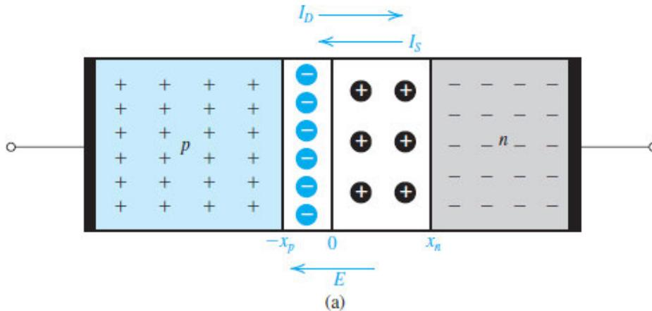
**Figure 3.10 (a)** A  $pn$  junction with the terminals open-circuited.
