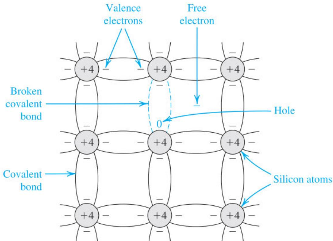
**Figure 3.2** At room temperature, some of the covalent bonds are broken by thermal generation. Each broken bond gives rise to a free electron and a hole, both of which become available for current conduction.
