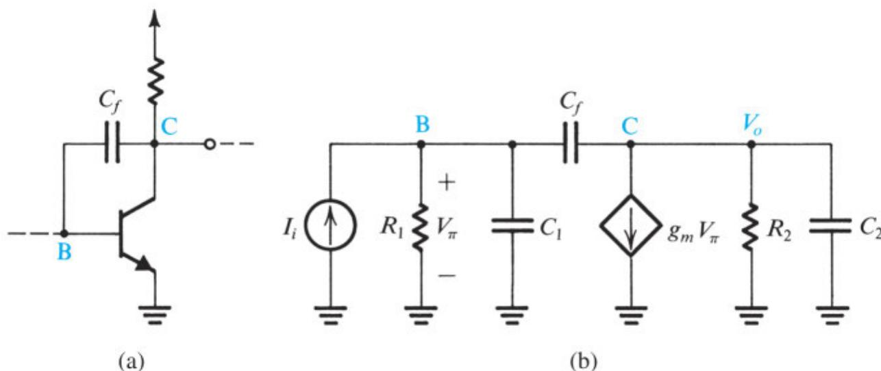
**Figure 11.41** (a) A gain stage in a multistage amplifier with a compensating capacitor connected in the feedback path, and (b) equivalent circuit. Note that although a BJT is shown, the analysis applies equally well to the MOSFET case.
