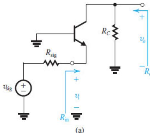
**Figure 7.41 (a)** CB amplifier with bias details omitted.
