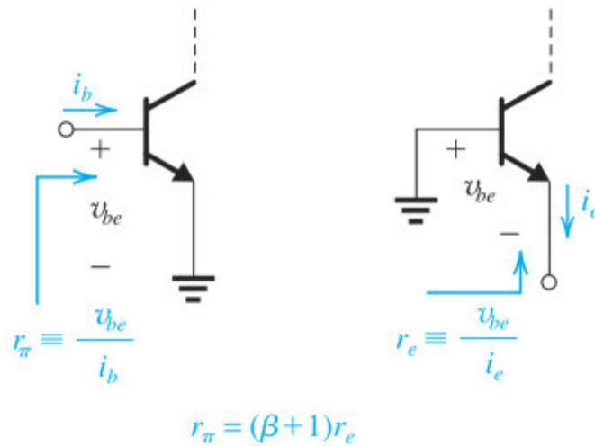
**Figure 7.23** Illustrating the definition of  $r_\pi$  and  $r_e$ .
