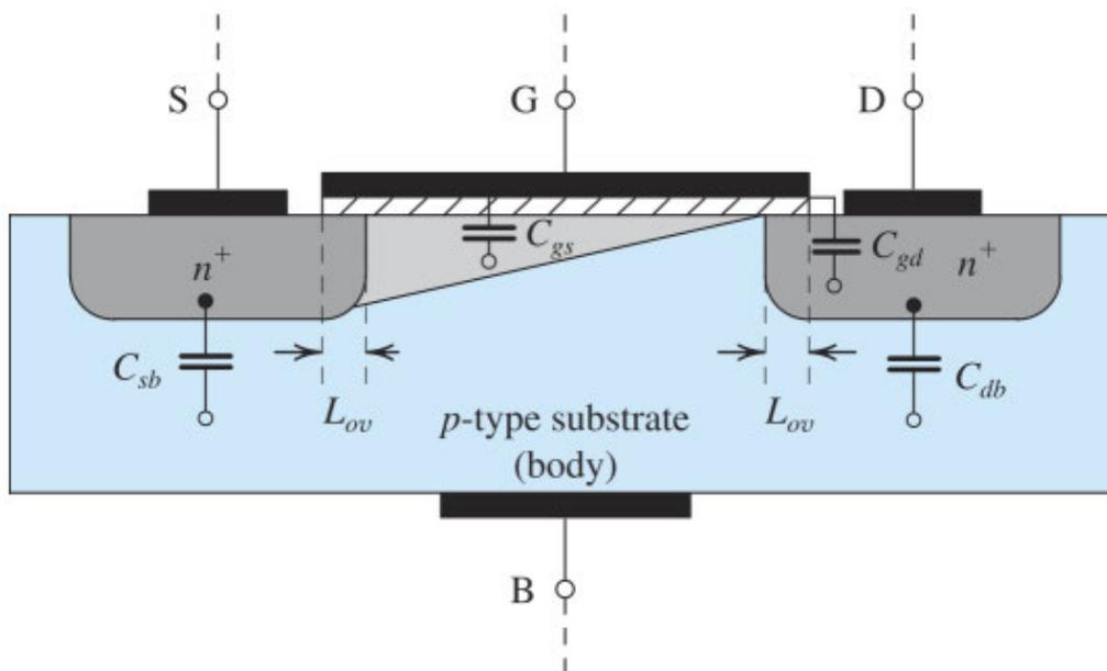
**Figure 10.3** Cross section of an  $n$ -channel MOSFET operating in the saturation region. The four internal capacitances,  $C_{gs}$ ,  $C_{gd}$ ,  $C_{sb}$ , and  $C_{db}$ , are indicated. Note that the bias voltages are not shown. Also not shown, to keep the diagram simple, is the depletion region.
