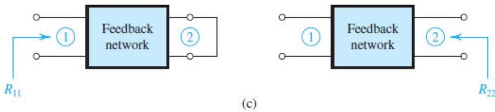
Figure 11.16 (c) Definition of  $R_{11}$  and  $R_{22}$ .
