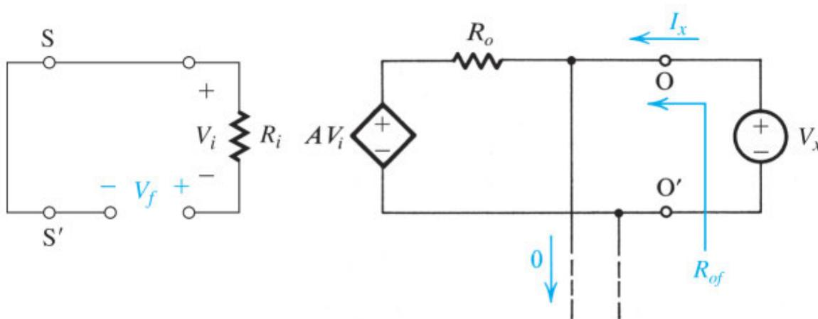
**Figure 11.15** Determining the output resistance of the feedback amplifier of Fig. 11.14(a):  $R_{of} = V_x/I_x$ .
