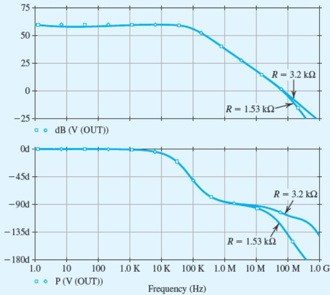
**Figure B.63** Magnitude and phase response of the op-amp circuit in Fig. B.60:  $C_C = 0.6 \text{ pF}$ ,  $R = 1.53 \text{ k}\Omega$  ( $PM = 55^\circ$ ), and  $R = 3.2 \text{ k}\Omega$  ( $PM = 75^\circ$ ).
