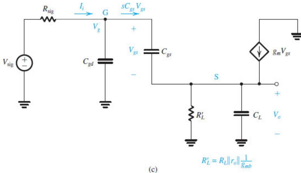
**Figure 10.23 (c)** A simplified version of the equivalent circuit.
