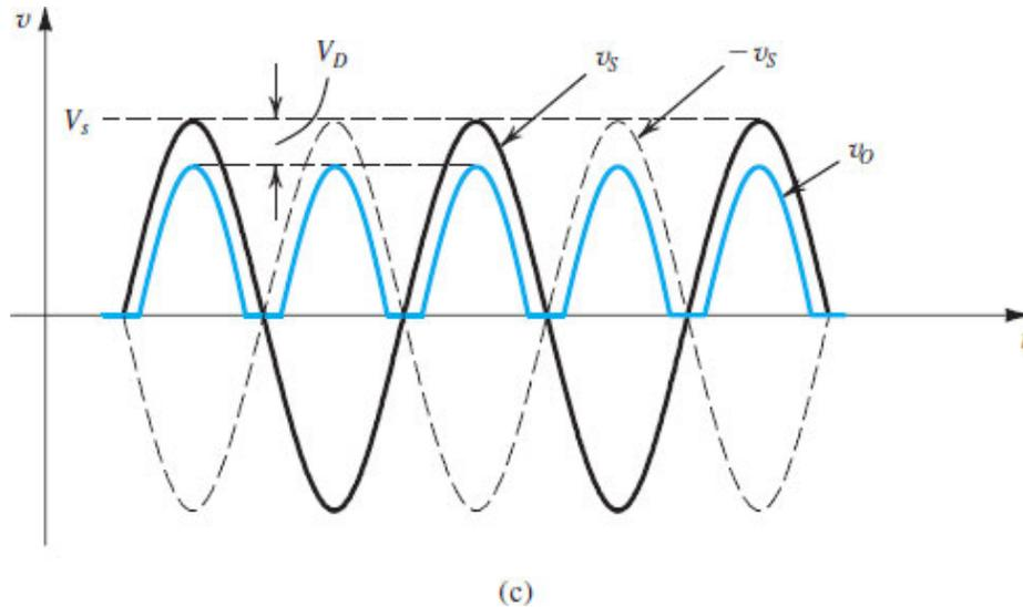
**Figure 4.22 (c)** Full-wave rectifier using a transformer with a center-tapped secondary winding: input and output waveforms.
