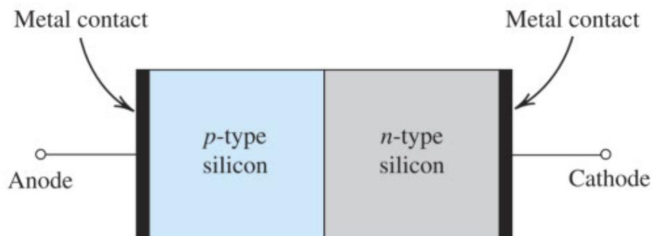
**Figure 3.8** Simplified physical structure of the  $pn$  junction. (Actual geometries are given in Appendix A.) As the  $pn$  junction implements the junction diode, its terminals are labeled anode and cathode.
