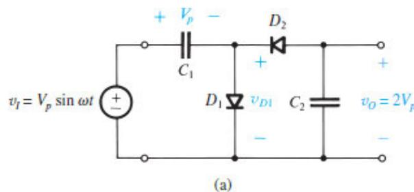
**Figure 4.31 (a)** Voltage doubler: circuit.
