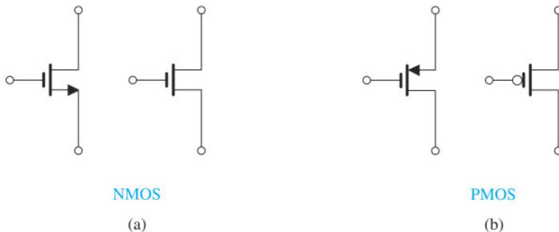
**Figure 16.6** Usual and alternative circuit symbols for MOSFETs.
