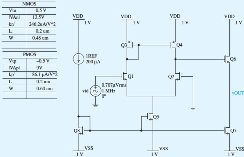
Figure B.47 Schematic capture of the two-stage CMOS op amp.
