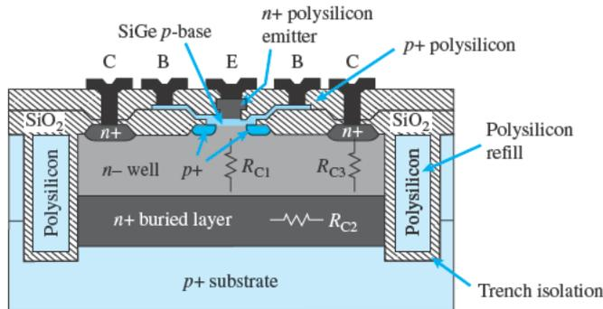
**Figure A.13** Cross-sectional diagram of a symmetric self-aligned SiGe heterojunction bipolar transistor, or HBT.
