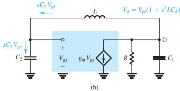
**Figure 15.15 (b)** Equivalent circuit of the Colpitts oscillator of (a). To simplify the analysis,  $\epsilon_{gd}$  is neglected. We can consider  $C_{gs}$  to be part of  $C_2$ , and we can include  $r_o$  in  $R$ .
