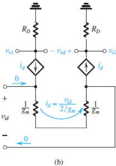
**Figure 9.9 (b)** An alternative view of the small-signal differential operation of the MOS differential pair: analysis using equivalent-circuit models.
