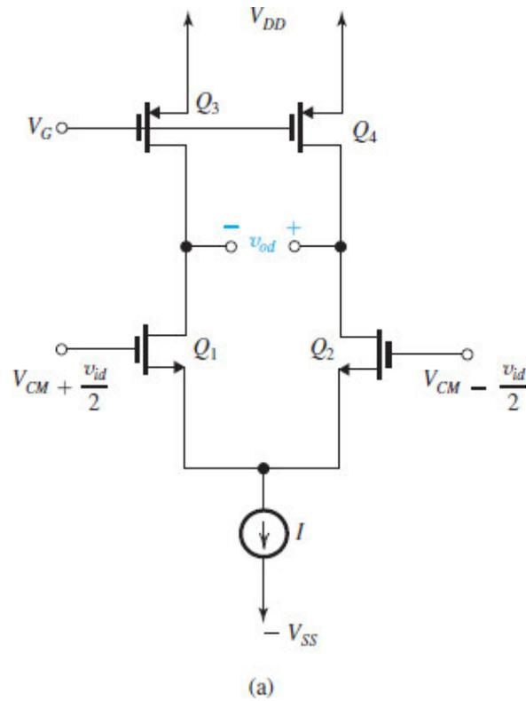
**Figure 9.12 (a)** Differential amplifier with current-source loads formed by  $Q_3$  and  $Q_4$ .
