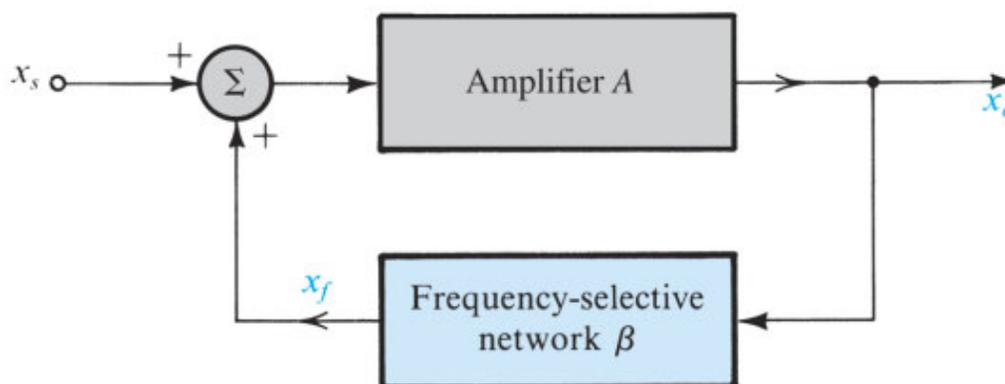
**Figure 15.1** The basic structure of a sinusoidal oscillator. A positive-feedback loop is formed by an amplifier and a frequency-selective network. In an actual oscillator circuit, no input signal will be present; here we are showing an input signal  $x_s$  to help explain the principle of operation.
