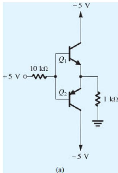
Figure 6.31 (a) Example 6.12: circuit.
