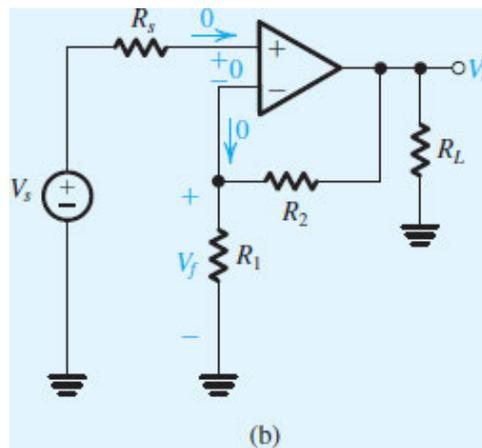
Figure 11.13 (b) The feedback amplifier with the open-loop gain  $A$  assumed infinite.
