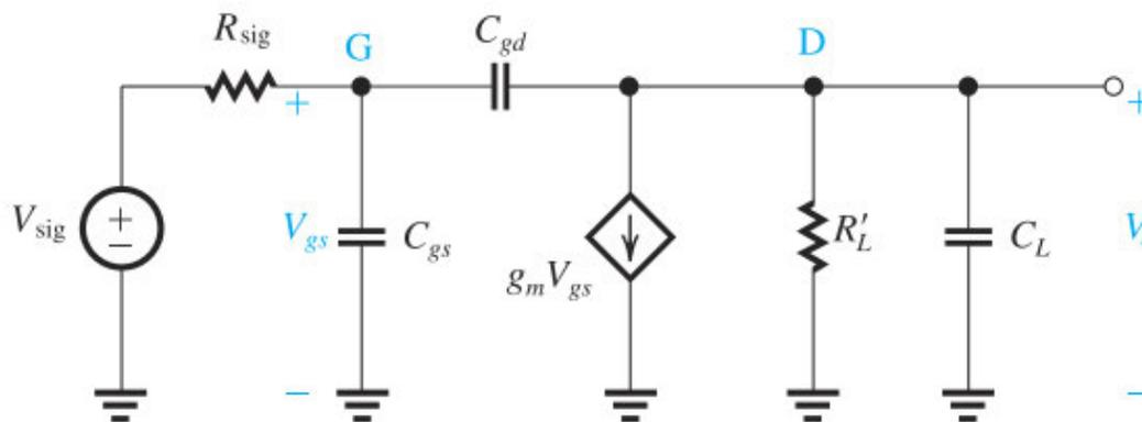
Figure 10.16 High-frequency equivalent circuit for the CS amplifier.
