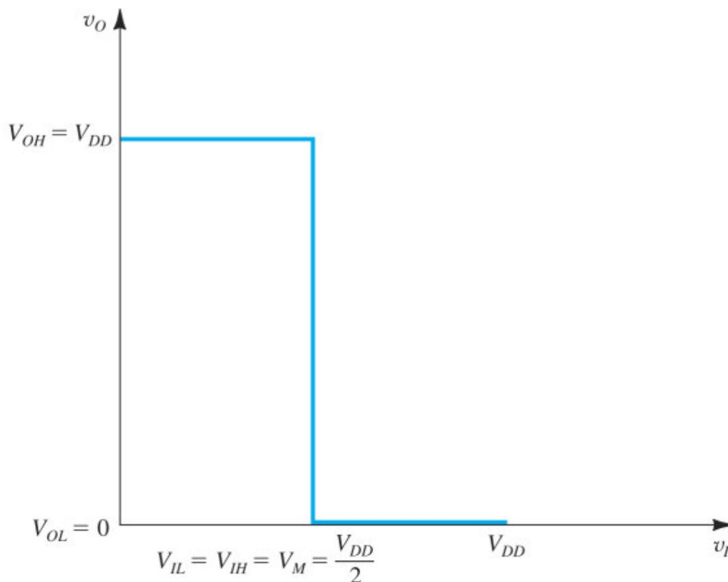
**Figure 16.16** The VTC of an ideal inverter.
