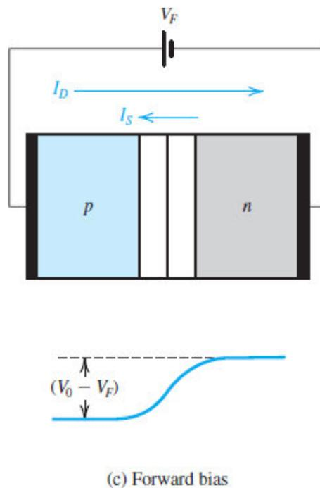
**Figure 3.11 (c)** The  $pn$  junction in forward bias.
