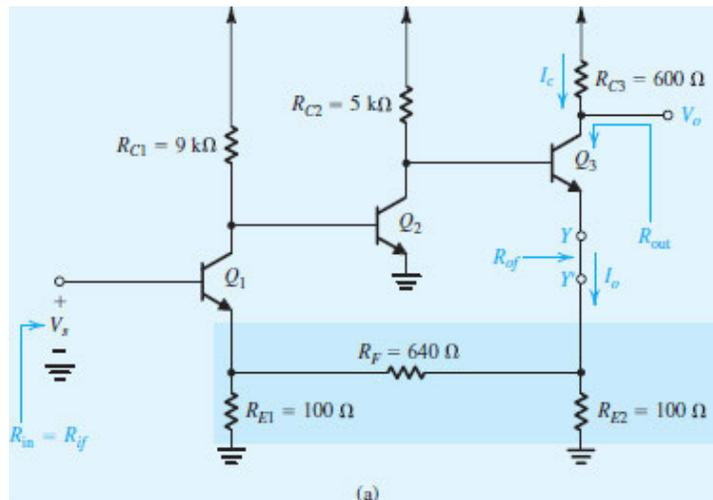
Figure 11.24 (a) Circuit for Example 11.8.
