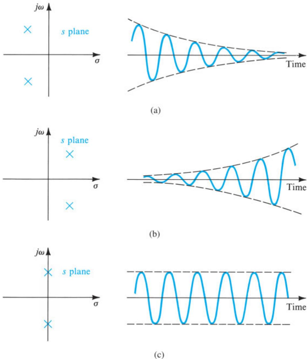
**Figure 11.31** Relationship between pole location and transient response.
