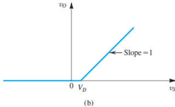
Figure 4.21 (b) Transfer characteristic of the rectifier circuit.
