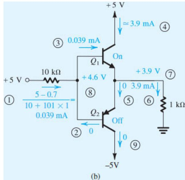
Figure 6.31 (b) Example 6.12: analysis with steps numbered.
