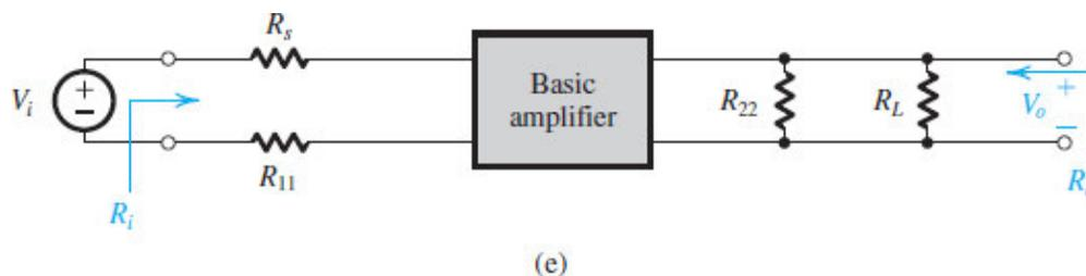
**Figure 11.16 (e)** The  $A$  circuit, showing the open-loop resistances  $R_i$  and  $R_o$ .
