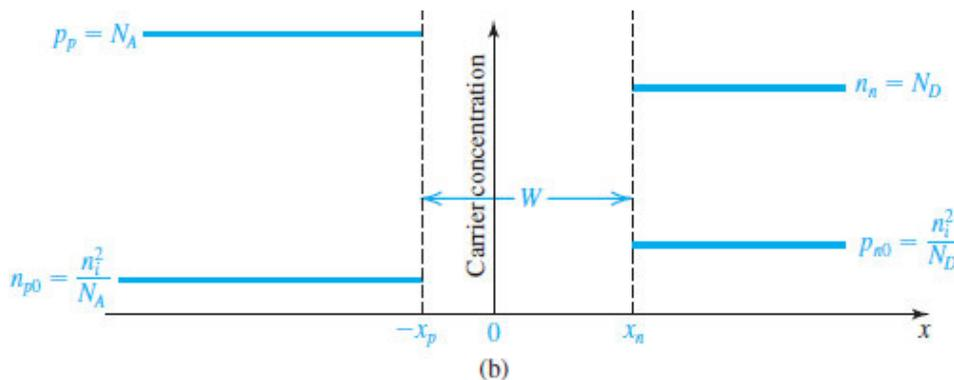
**Figure 3.10 (b)** Carrier concentrations; note that  $N_A > N_D$ .
