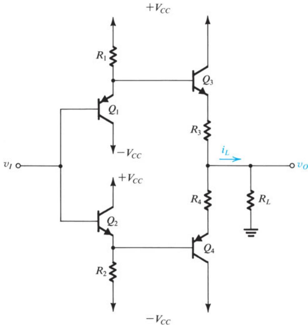
**Figure 12.16** A class AB output stage with an input buffer. In addition to providing a high input resistance, the buffer transistors  $Q_1$  and  $Q_2$  bias the output transistors  $Q_3$  and  $Q_4$ .
