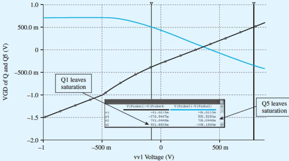
Figure B.34 Input common-mode range of the two-stage CMOS op amp.
