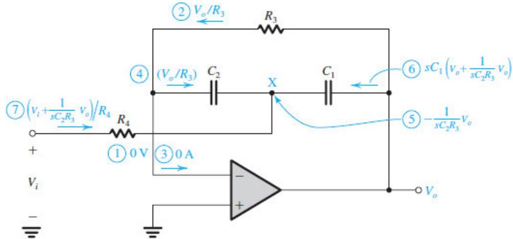
**(b)****Figure 14.27 (b)** Analysis of the circuit in (a) to determine the transfer function  $T(s) \equiv V_o/V_i$ . The order of the analysis steps is indicated by the circled numbers.
