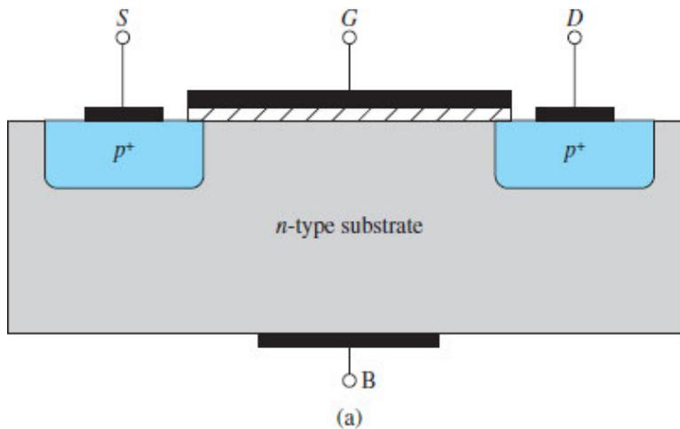
**Figure 5.9 (a)** Physical structure of the PMOS transistor. Note that it is similar to the NMOS transistor shown in Fig. 5.1(b) except that all semiconductor regions are reversed in polarity.
