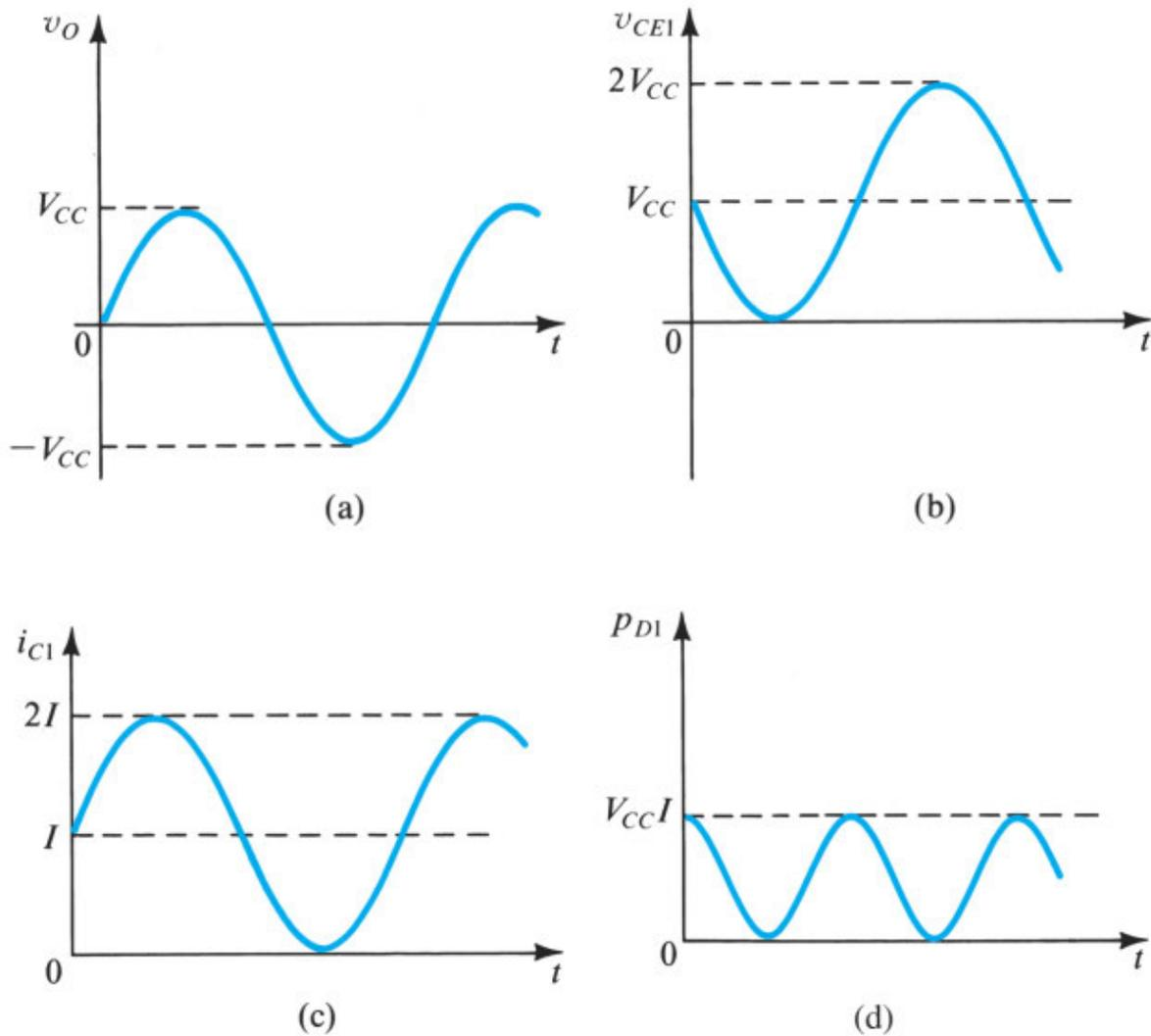
**Figure 12.5** Maximum signal waveforms in the class A output stage of Fig. 12.3 under the condition  $I = V_{CC}/R_L$  or, equivalently,  $R_L = V_{CC}/I$ . Note that we have neglected the transistor saturation voltages.
