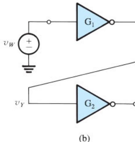
**Figure 18.11 (b)** The latch with the feedback loop opened.
