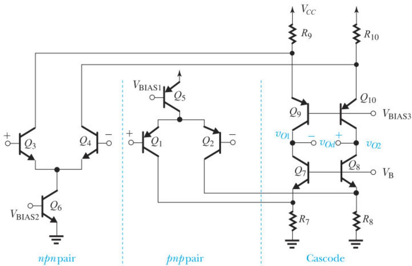
**Figure 13.18** Input stage with rail-to-rail input common-mode range and a folded-cascode stage to increase the gain. Note that all the bias voltages including  $V_{BIAS3}$  and  $V_B$  are generated elsewhere on the chip.
