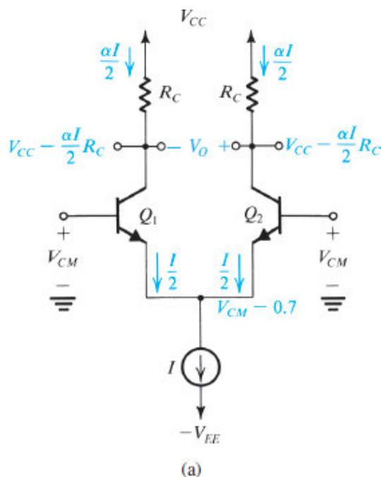
**Figure 9.15 (a)** Different modes of operation of the BJT differential pair: the differential pair with a common-mode input voltage  $V_{CM}$ .
