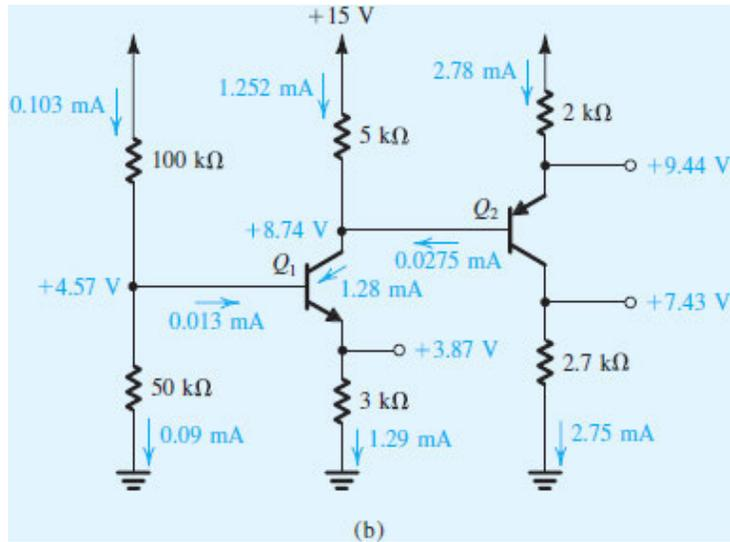
Figure 6.30 (b) Circuit for Example 6.11.
