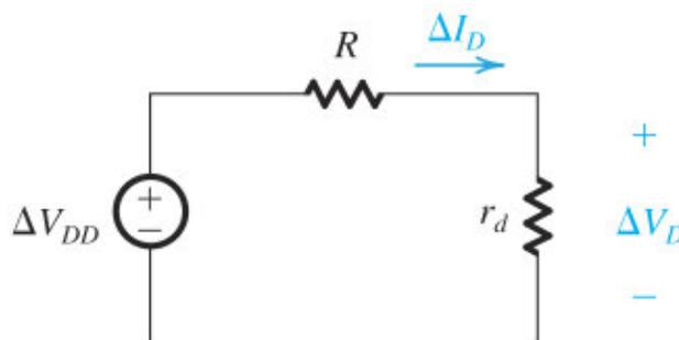
**Figure 4.16** Circuit for determining the incremental quantities  $\Delta I_D$  and  $\Delta V_D$  for the circuit in Figure 4.14(b). Note that replacing the diode with its small-signal resistance  $r_d$  results in a linear circuit.
