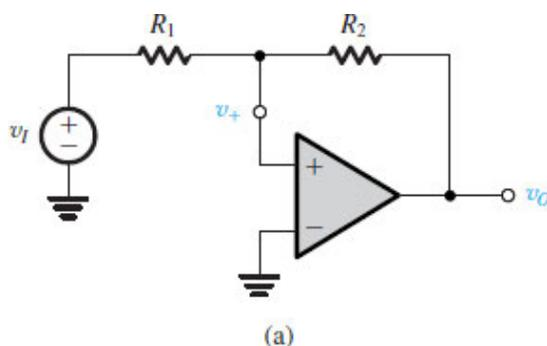
**Figure 15.22 (a)** A bistable circuit derived from the positive-feedback loop of Fig. 15.19 by applying  $v_I$  through  $R_1$ .
