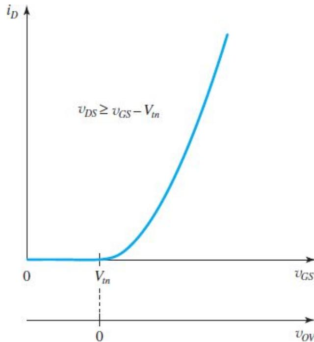
**Figure 5.14** The  $i_D$ - $v_{GS}$  characteristic of an NMOS transistor operating in the saturation region. The  $i_D$ - $v_{OV}$  characteristic can be obtained by simply relabeling the horizontal axis, that is, shifting the origin to the point  $v_{GS} = V_{tn}$ .
