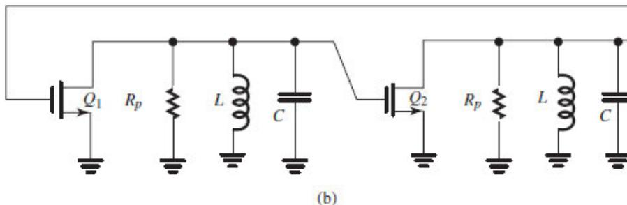
**Figure 15.16 (b)** Signal equivalent circuit of the cross-coupled oscillator in (a).
