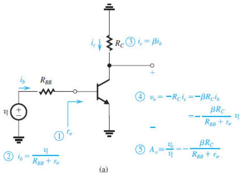
**Figure 7.33 (a)** Performing signal analysis directly on the circuit diagram with the BJT small-signal model implicitly employed: circuit for Example 7.5.
