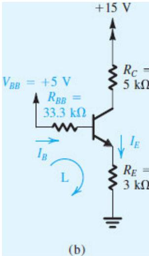
Figure 6.29 (b) Circuit for Example 6.10.
