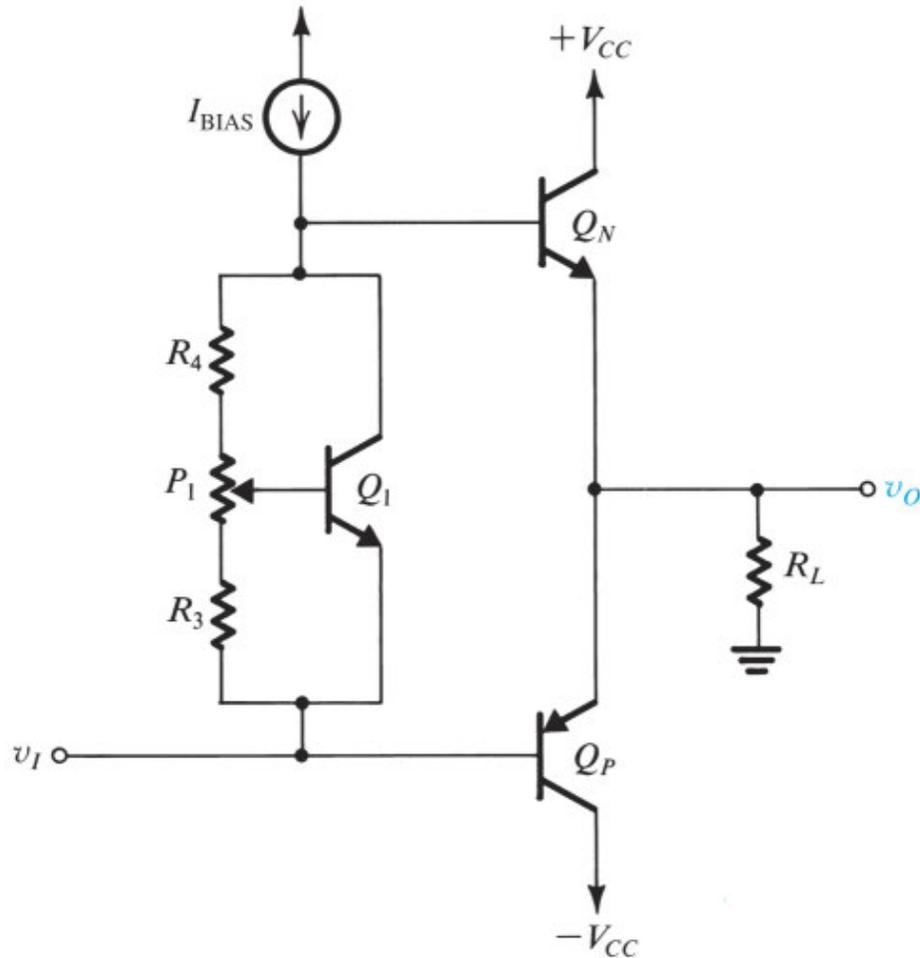
**Figure 12.15** A discrete-circuit class AB output stage with a potentiometer used in the  $V_{BE}$  multiplier. We adjust the potentiometer to give the desired value of quiescent current in  $Q_N$  and  $Q_P$ .
