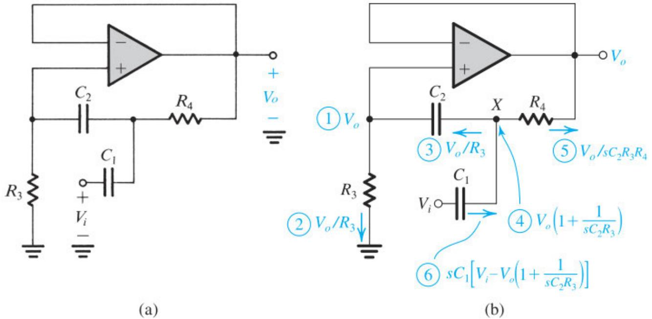
**Figure 14.28** (a) Circuit for realizing the second-order high-pass filter function. (b) Analysis of the circuit in (a) to determine its transfer function  $T(s) = V_o/V_i$ . The circled numbers indicate the order of the analysis steps.
