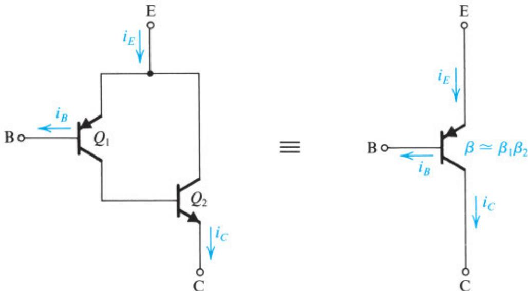
**Figure 12.18** The compound-*pn*p configuration.
