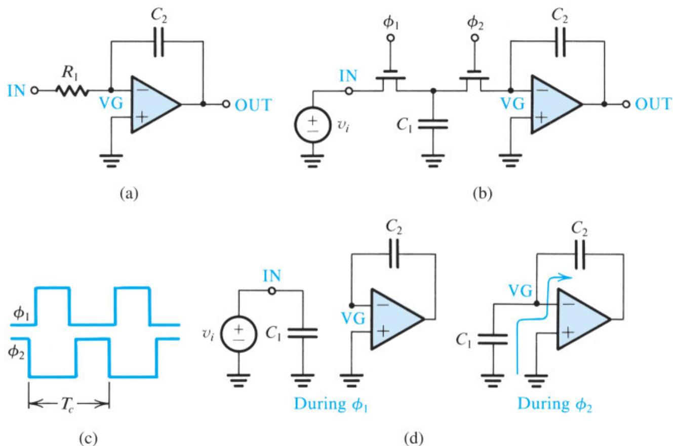
**Figure 14.30** Basic principle of the switched-capacitor filter technique. (a) Active-RC integrator. (b) Switched-capacitor integrator. (c) Two-phase clock (nonoverlapping). (d) During  $\phi_1$ ,  $C_1$  charges up to the current value of  $v_i$  and then, during  $\phi_2$ , discharges into  $C_2$ .
