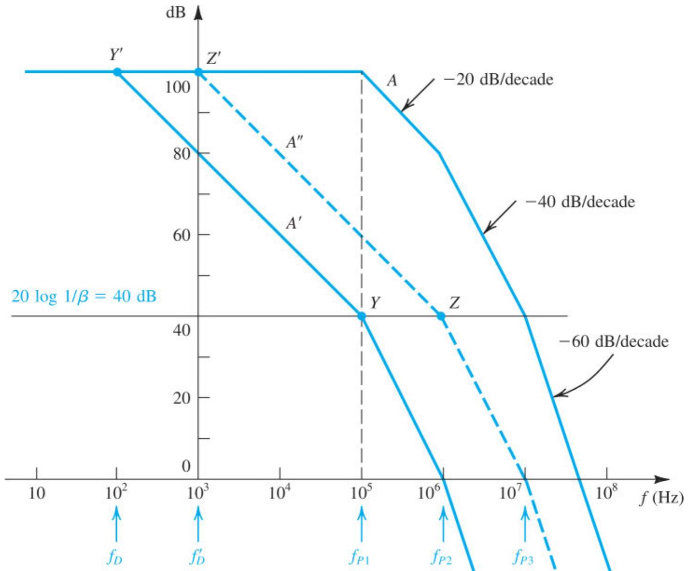
**Figure 11.39** Frequency compensation for  $\beta = 10^{-2}$ . The response labeled  $A'$  is obtained by introducing an additional pole at  $f_D$ . The  $A''$  response is obtained by moving the original low-frequency pole to  $f'_D$ .
