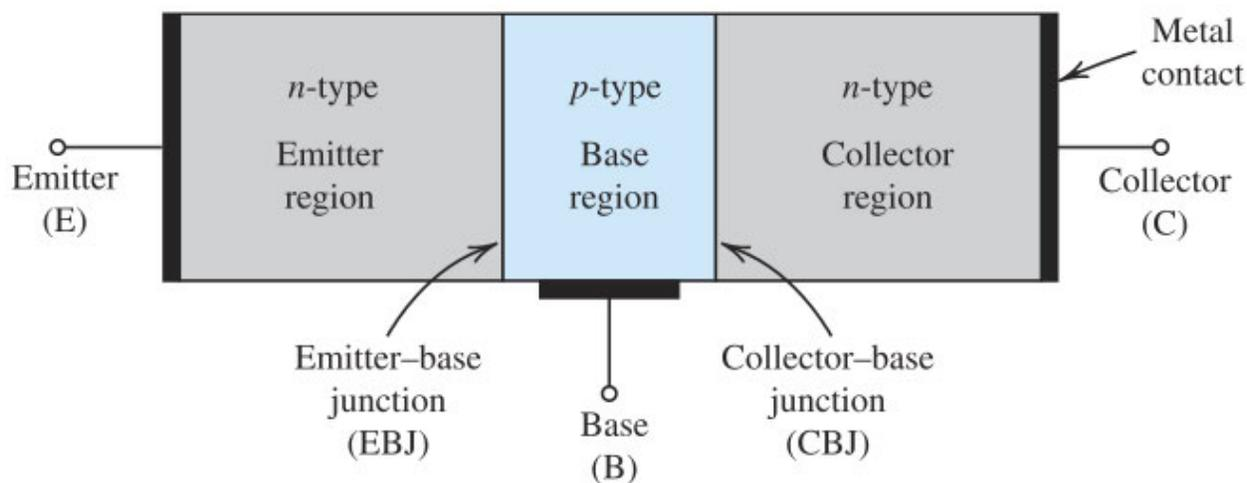
Figure 6.1 A simplified structure of the  $npn$  transistor.
