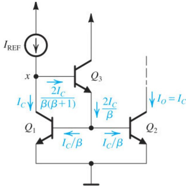
**Figure 8.11** A current mirror with base-current compensation.
