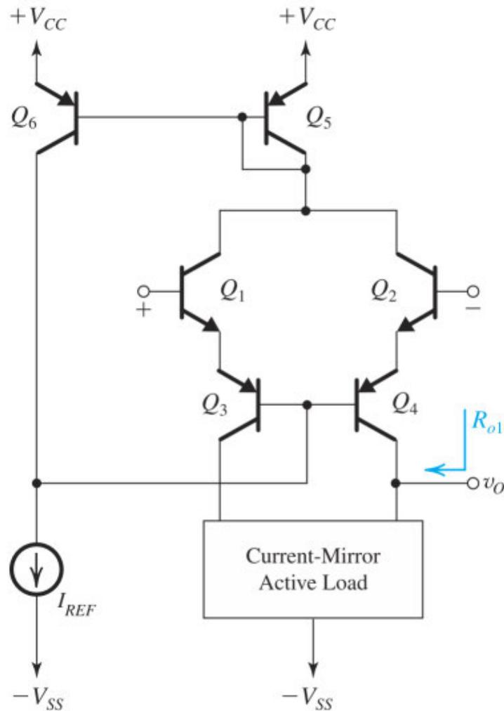
**Figure 13.22** The 741 input stage.
