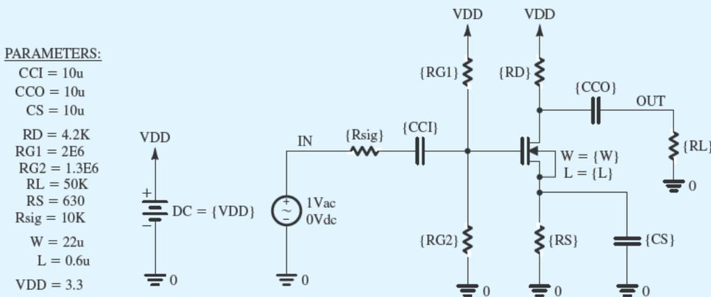
Figure B.19 Schematic capture of the CS amplifier in Example S.7.1.
