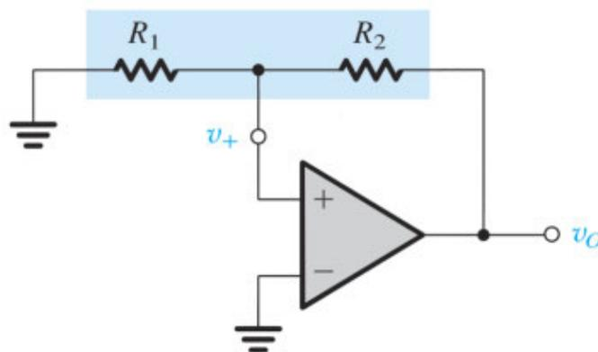
**Figure 15.19** A positive-feedback loop capable of bistable operation.
