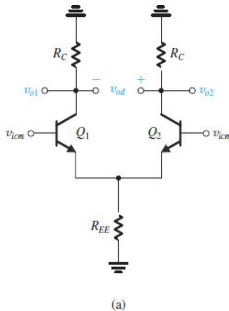
**Figure 9.25 (a)** The differential amplifier fed by a common-mode input signal  $v_{icm}$ .
