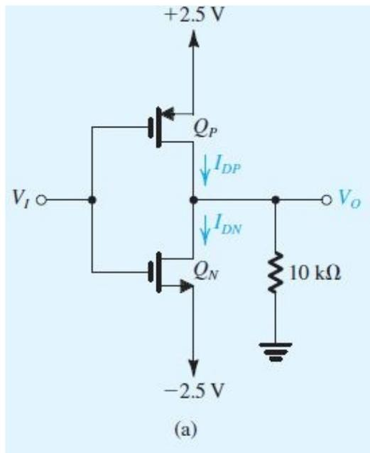
Figure 5.26 (a) Circuit for Example 5.8.
