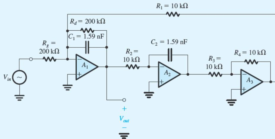
**Figure B.69** Circuit for Example S.14.2 Second-order bandpass filter implemented with a Tow-Thomas biquad circuit having  $f_0 = 10$  kHz,  $Q = 20$ , and unity center-frequency gain.
