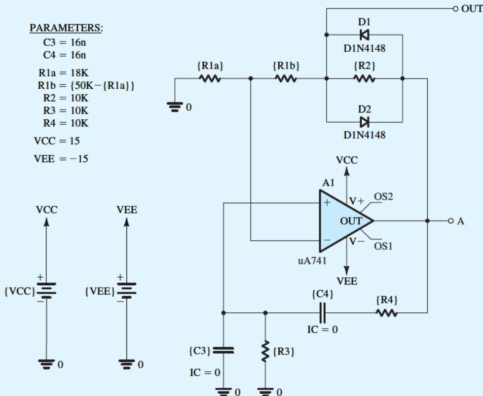
Figure B.72 Example S.15.1: Schematic capture of a Wien-bridge oscillator.
