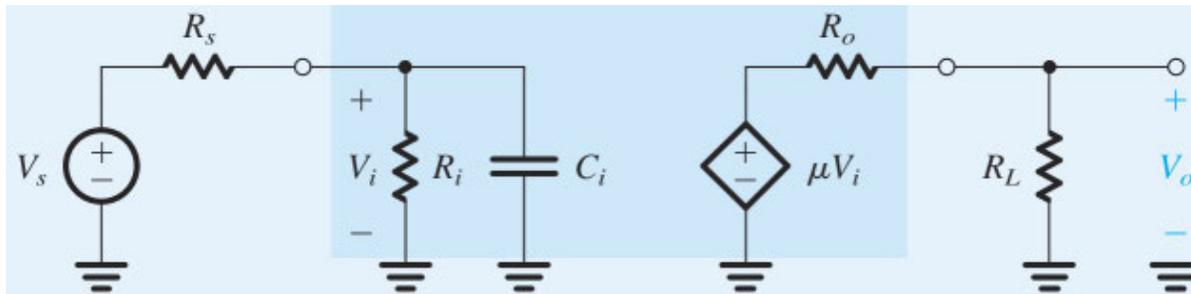
**Figure 1.25** Circuit for Example 1.5.
