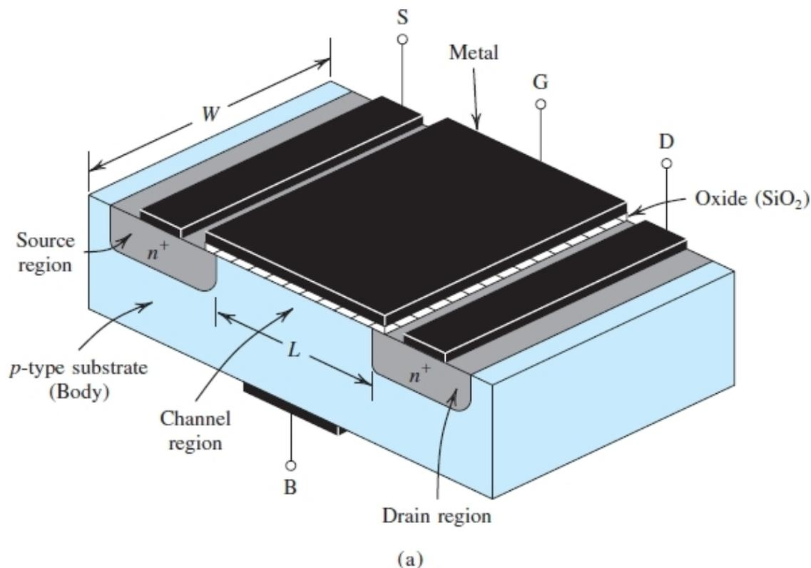
**Figure 5.1 (a)** Physical structure of the *n*-channel enhancement-type MOSFET: perspective view. Typically,  $L = 20$  nm to  $1\ \mu\text{m}$ ,  $W = 30$  nm to  $100\ \mu\text{m}$ , and the thickness of the oxide layer ( $t_{ox}$ ) is in the range of 1 to 10 nm.
