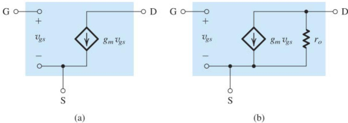
**Figure 7.13** Small-signal models for the MOSFET: **(a)** neglecting the dependence of  $i_D$  on  $v_{DS}$  in the active region (the channel-length modulation effect) and **(b)** including the effect of channel-length modulation, modeled by output resistance  $r_o = |V_A|/I_D$ . These models apply equally well for both NMOS and PMOS transistors.
