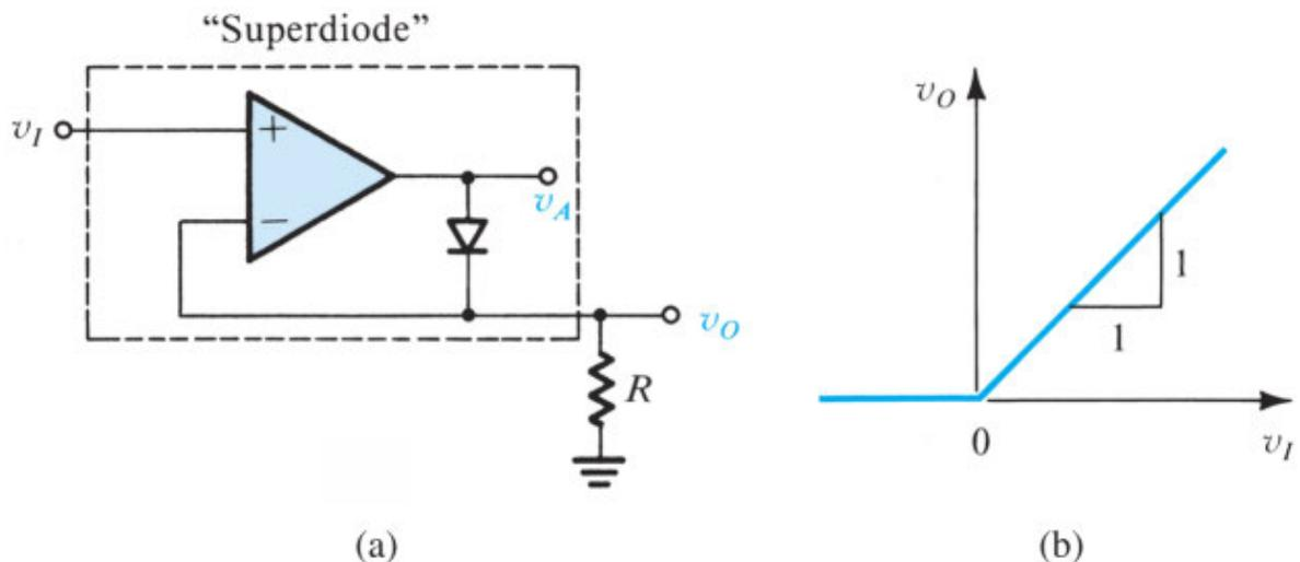
**Figure 4.28** (a) The “superdiode” precision half-wave rectifier and (b) its almost-ideal transfer characteristic. Note that when  $v_I > 0$  and the diode conducts, the op amp supplies the load current, and the source is conveniently buffered, an added advantage. Not shown are the op-amp power supplies.
