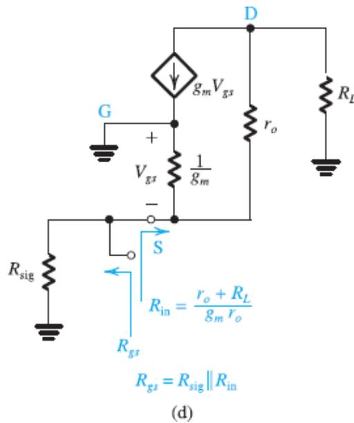
Figure 10.18 (d) Circuit for determining the resistance  $R_{gs}$  seen by  $C_{gs}$ .
