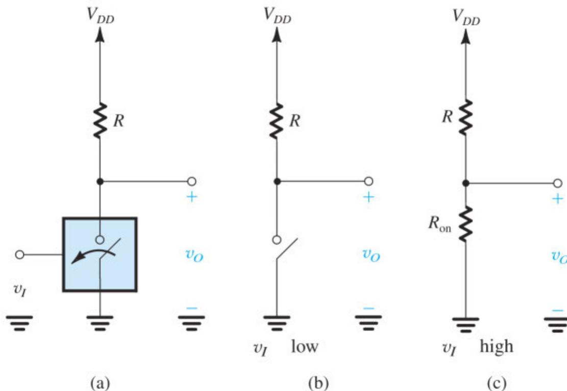
**Figure 16.17** (a) The simplest implementation of a logic inverter using a voltage-controlled switch; (b) equivalent circuit when  $v_I$  is low; (c) equivalent circuit when  $v_I$  is high. Note that the switch is assumed to close when  $v_I$  is high.
