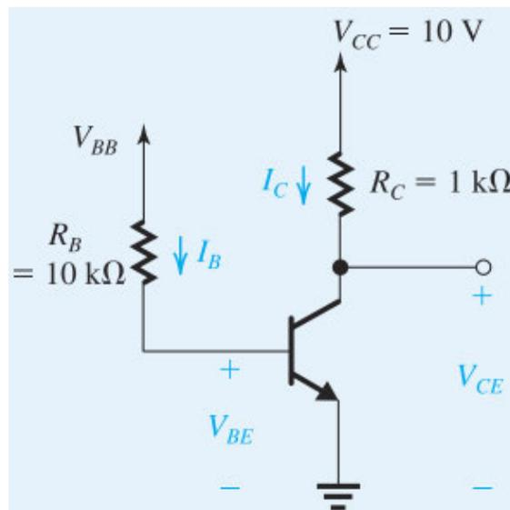
**Figure 6.22** Circuit for Example 6.3.
