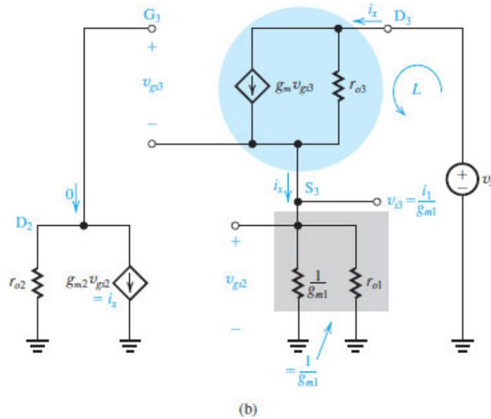
**Figure 8.38 (b)** The Wilson MOS mirror: analysis to determine output resistance.
