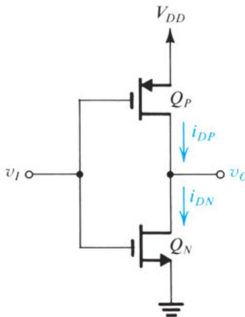
Figure 16.22 The CMOS inverter.
