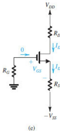
**Figure 7.50 (e)** Biasing using a fixed voltage at the gate,  $V_G$ , and a resistance in the source lead,  $R_S$ : practical implementation using two supplies.
