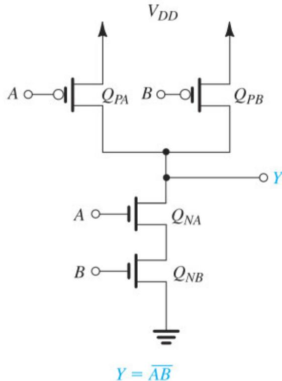
**Figure 16.8** A two-input CMOS NAND gate.
