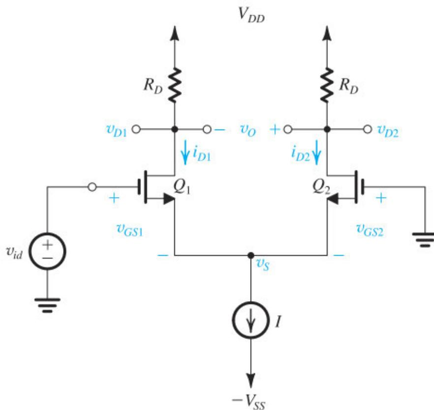
**Figure 9.4** The MOS differential pair with a differential input signal  $v_{id}$  applied. With  $v_{id}$  positive:  $v_{GS1} > v_{GS2}$ ,  $i_{D1} > i_{D2}$ , and  $v_{D1} < v_{D2}$ ; thus  $v_O$  will be positive. With  $v_{id}$  negative:  $v_{GS1} < v_{GS2}$ ,  $i_{D1} < i_{D2}$ , and  $v_{D1} > v_{D2}$ ; thus  $v_O$  will be negative.
