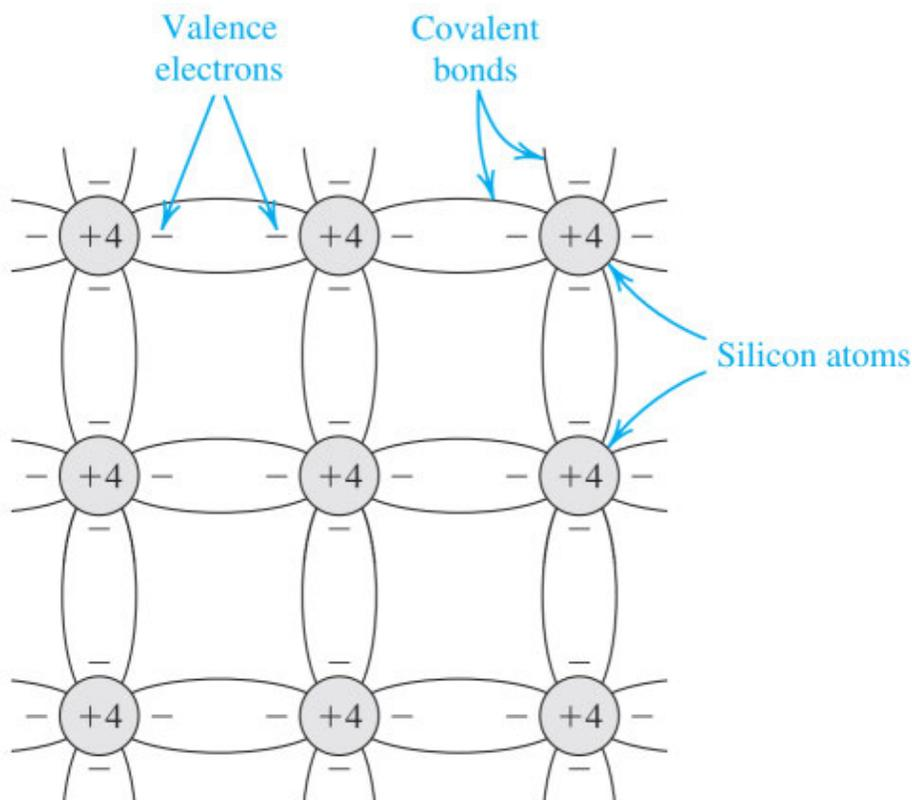
**Figure 3.1** Two-dimensional representation of the silicon crystal. The circles represent the inner core of silicon atoms, with +4 indicating its positive charge of  $+4q$ , which is neutralized by the charge of the four valence electrons. Observe how the covalent bonds are formed by sharing of the valence electrons. At 0 K, all bonds are intact and no free electrons are available for current conduction.
