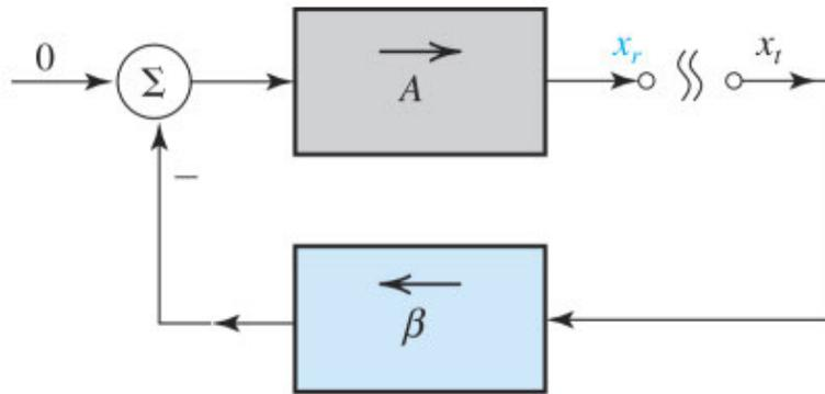
**Figure 11.2** Determining the loop gain by breaking the feedback loop at the output of the basic amplifier, applying a test signal  $x_t$ , and measuring the returned signal  $x_r$ :  $A\beta \equiv -x_r/x_t$ .
