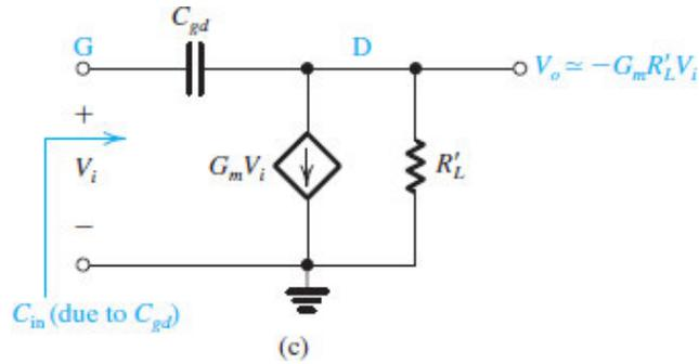
**Figure 10.30 (c)** Determining the component of  $C_{in}$  due to  $C_{gd}$ .
