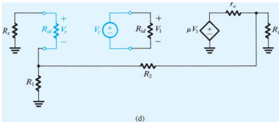
**Figure 11.13 (d)** Breaking the feedback loop to determine the loop gain  $A\beta = -V_r/V_t$ .
