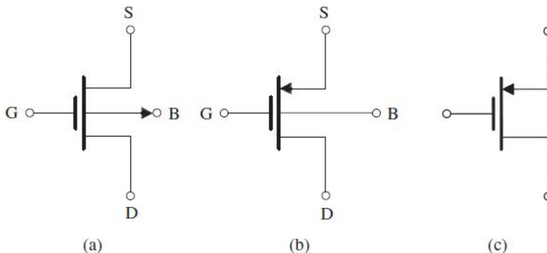
**Figure 5.19** (a) Circuit symbol for the  $p$ -channel enhancement-type MOSFET. (b) Modified symbol with an arrowhead on the source lead. (c) Simplified symbol for cases where the source is connected to the body.
