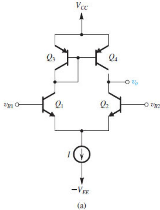
Figure 9.35 (a) Current-mirror-loaded bipolar differential pair.
