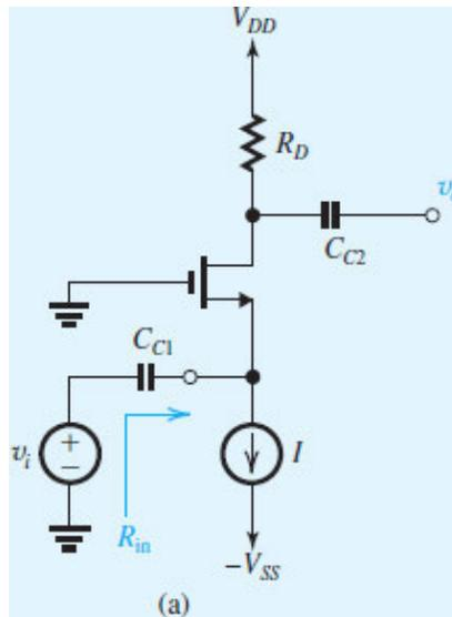
Figure 7.19 (a) Amplifier circuit for Example 7.4.
