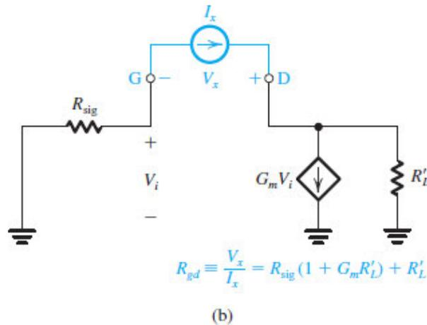
**Figure 10.31 (b)** Determining  $R_{gd}$ .
