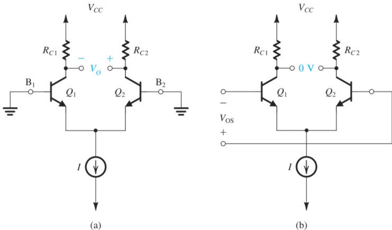
**Figure 9.28** (a) The BJT differential pair with both inputs grounded. Device and resistance mismatch result in a finite dc output  $V_O$ . (b) Application of the input offset voltage  $V_{OS}$  to the input terminals with appropriate polarity reduces  $V_O$  to zero.
