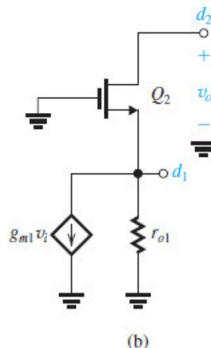
**Figure 8.28 (b)** The amplifier equivalent circuit with  $Q_1$  replaced with its output equivalent circuit, and the dc sources eliminated. Note that  $R_L$  of the cascode amplifier is infinite.
