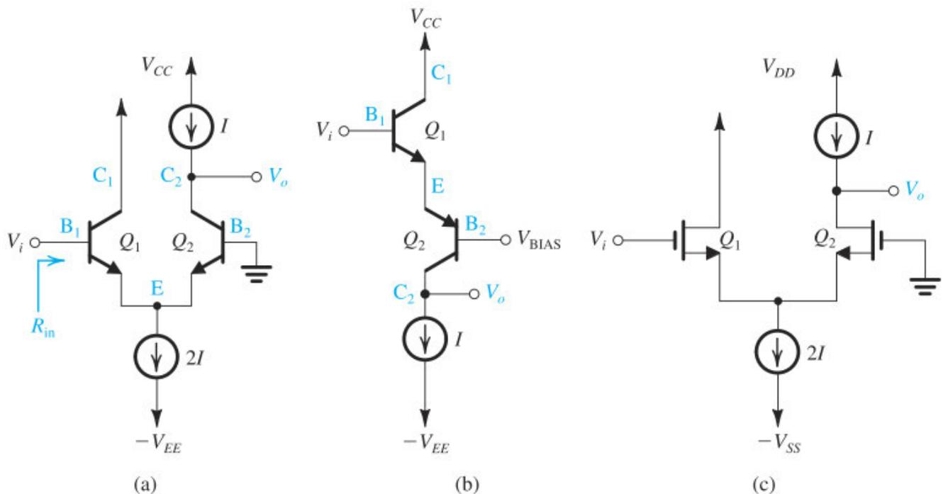
**Figure 10.34** (a) A CC–CB amplifier. (b) Another version of the CC–CB circuit with  $Q_2$  implemented using a *pnp* transistor. (c) The MOSFET version of the circuit in (a). Notice that the circuits in (a) and (c) can be considered as differential amplifiers with the load resistance of  $Q_1$  eliminated.
