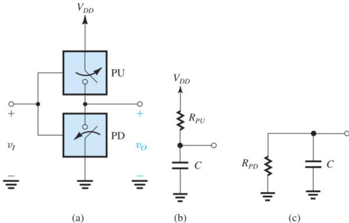
**Figure 17.12** (a) Switch-level model of a CMOS inverter. (b) Equivalent circuit for calculating the dynamic power dissipation when  $v_I$  is low. (c) Equivalent circuit for calculating the dynamic power dissipation when  $v_I$  is high.
