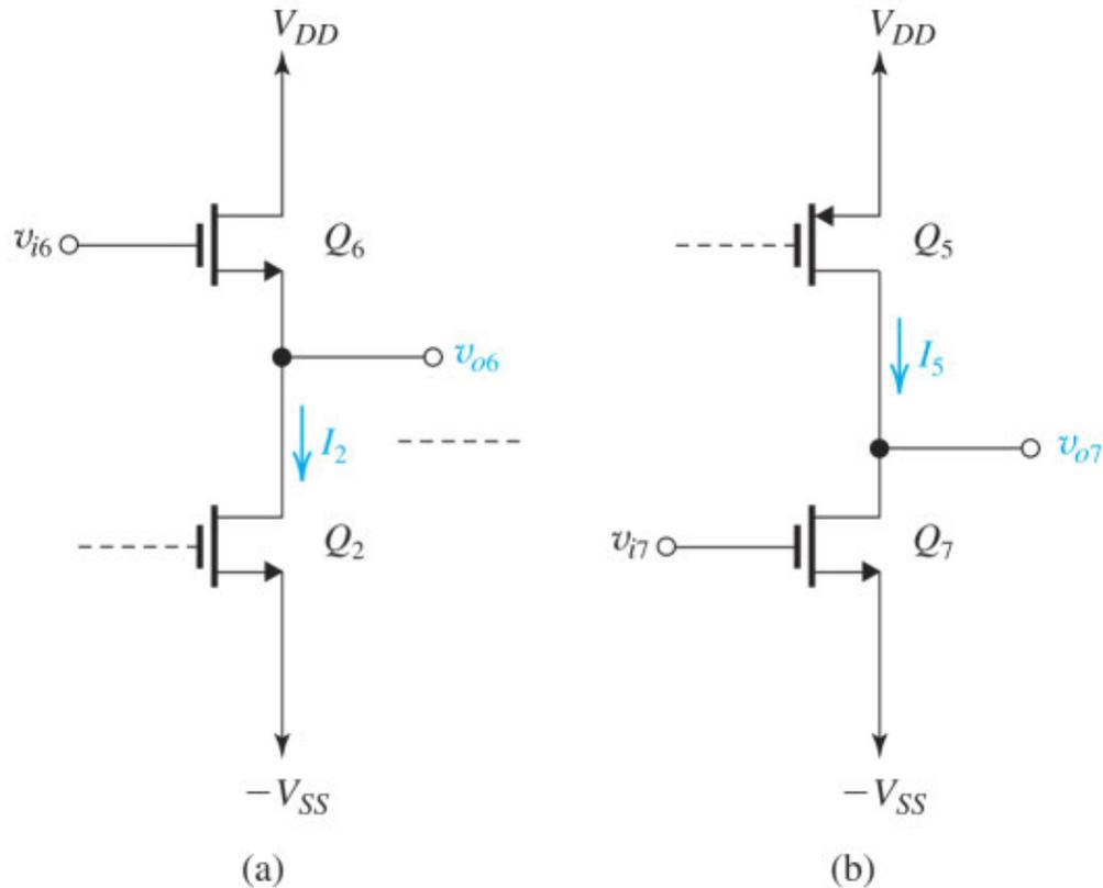
**Figure 8.5** Application of the constant currents  $I_2$  and  $I_5$  generated in the current-steering circuit of Fig. 8.4: (a) Constant-current  $I_2$  is the bias current for the source follower  $Q_6$ , and (b) constant-current  $I_5$  is the load current for the common-source amplifier  $Q_7$ .
