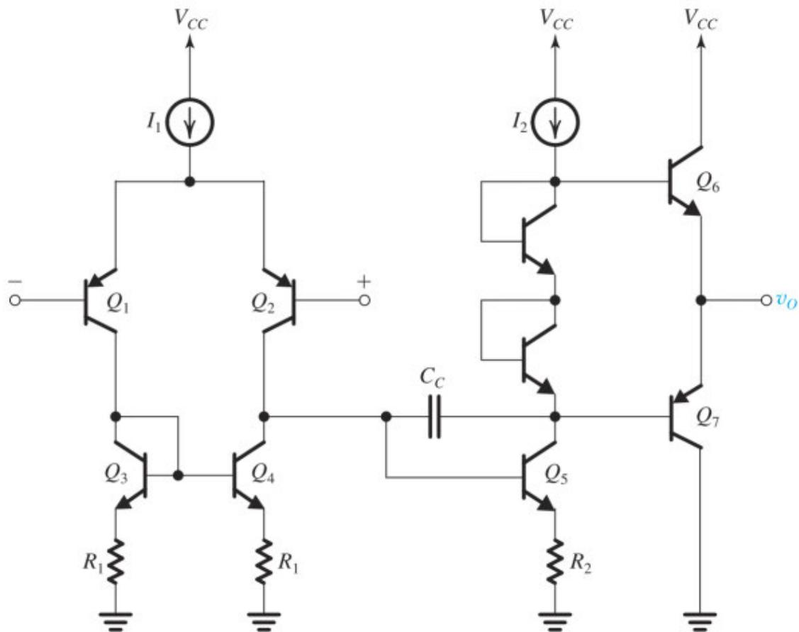
**Figure 13.15** A bipolar two-stage op amp with class AB output stage. The input common-mode range is limited by the input differential pair with current-mirror load, and the output swing is limited by the class AB output stage.
