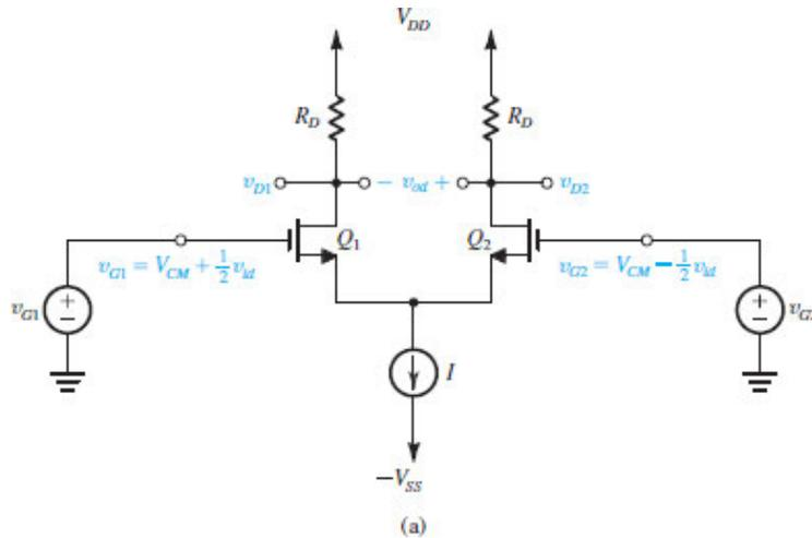
**Figure 9.8 (a)** Small-signal analysis of the MOS differential amplifier: The circuit with a common-mode voltage applied to set the dc bias voltage at the gates and with  $v_{id}$  applied in a complementary (or balanced) manner.
