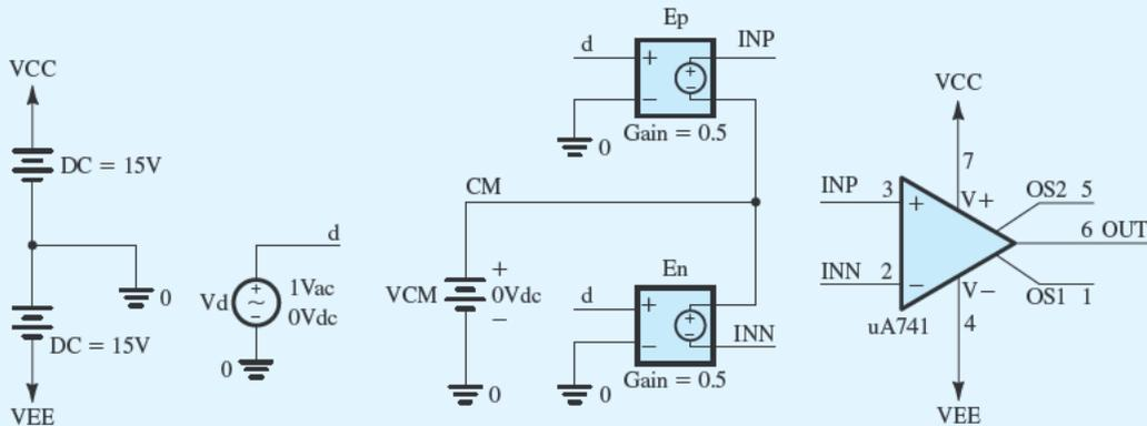
**Figure B.9** Simulating the frequency response of the  $\mu\text{A}741$  op-amp in Example S.2.2.
