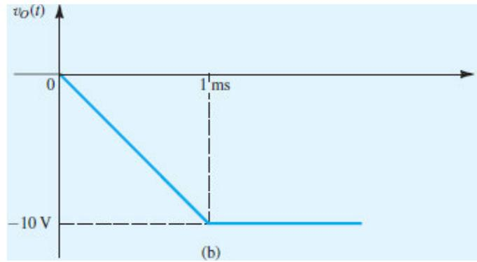
**Figure 2.27 (b)** Waveforms for Example 2.6: Output linear ramp of ideal integrator with time constant of 0.1 ms.
