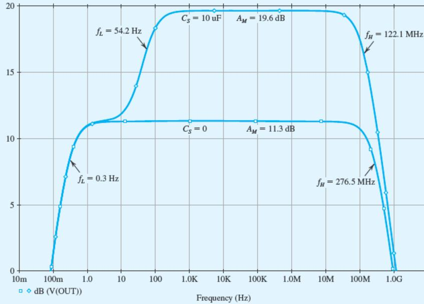
**Figure B.20** Frequency response of the CS amplifier in Example S.7.1 with  $C_S = 10 \mu\text{F}$  and  $C_S = 0$  (i.e.,  $C_S$  removed).
