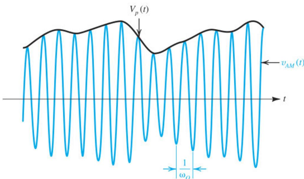
**Figure 4.27** The amplitude modulated (AM) signal  $v_{AM}$  is a sinusoid at a frequency  $\omega_0$ , called the carrier frequency, and has an amplitude modulated by the information-bearing signal  $V_p$ .
