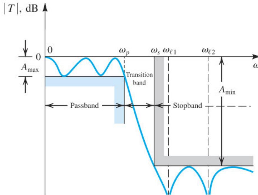
**Figure 14.3** Specification of the transmission characteristics of a low-pass filter. The magnitude response of a filter that just meets specifications is also shown.
