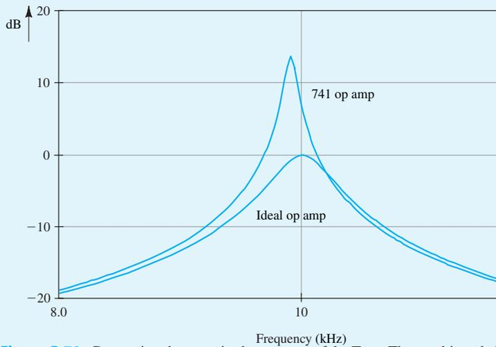
**Figure B.70** Comparing the magnitude response of the Tow–Thomas biquad circuit (shown in Fig. B.69) constructed with 741-type op amps, with the ideal magnitude response. These results illustrate the effect of the finite dc gain and bandwidth of the 741 op amp on the frequency response of the Tow–Thomas biquad circuit.
