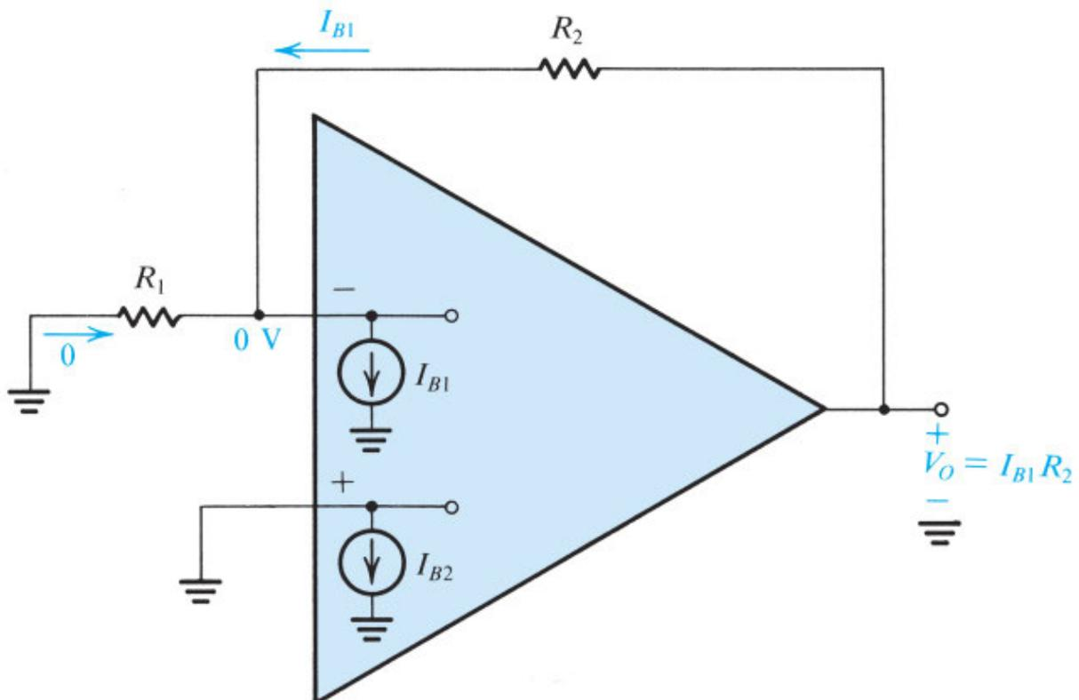
**Figure 2.34** Analysis of the closed-loop amplifier, taking into account the input bias currents.
