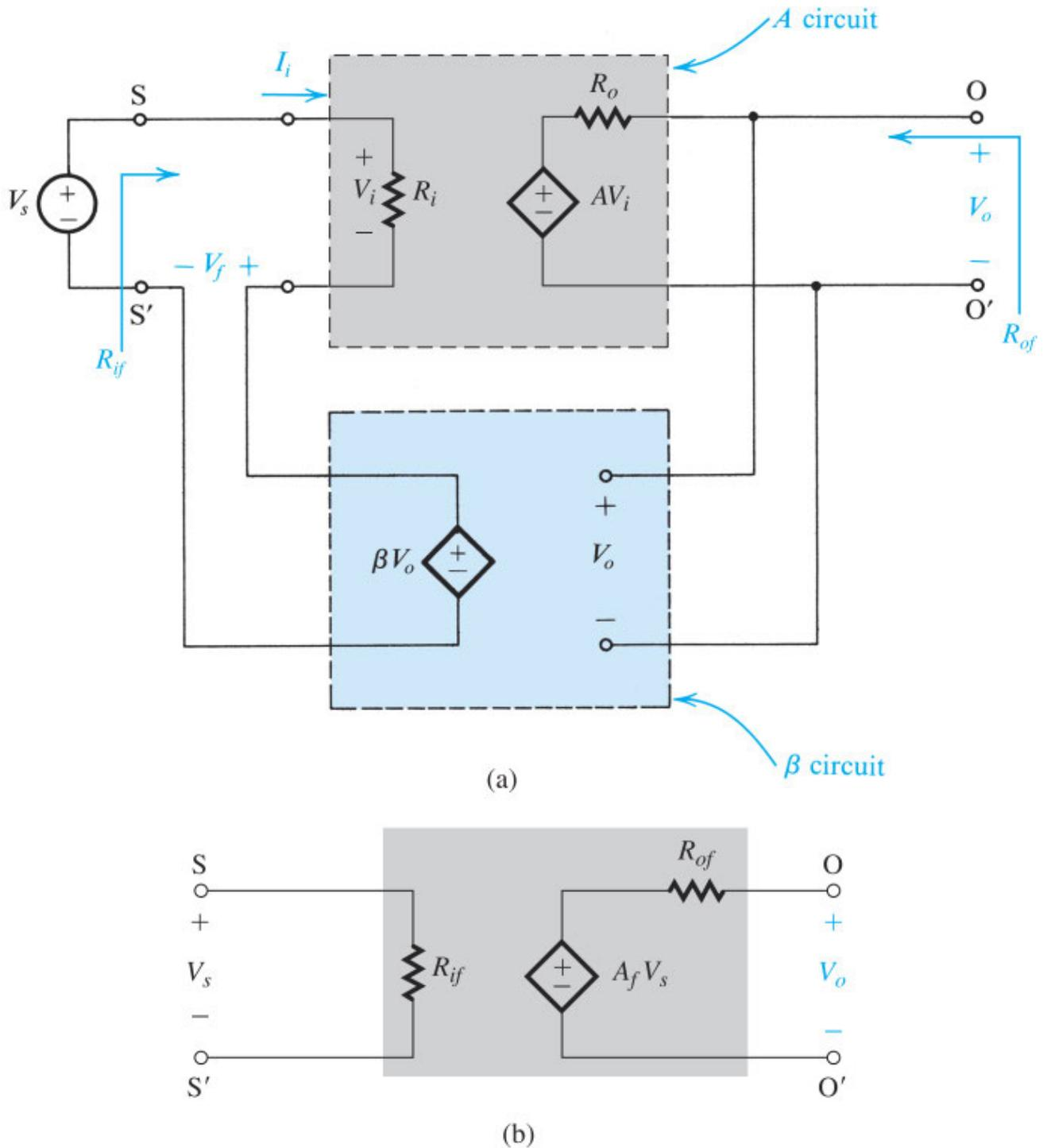
**Figure 11.14** The series–shunt feedback amplifier: (a) ideal structure; (b) equivalent circuit.
