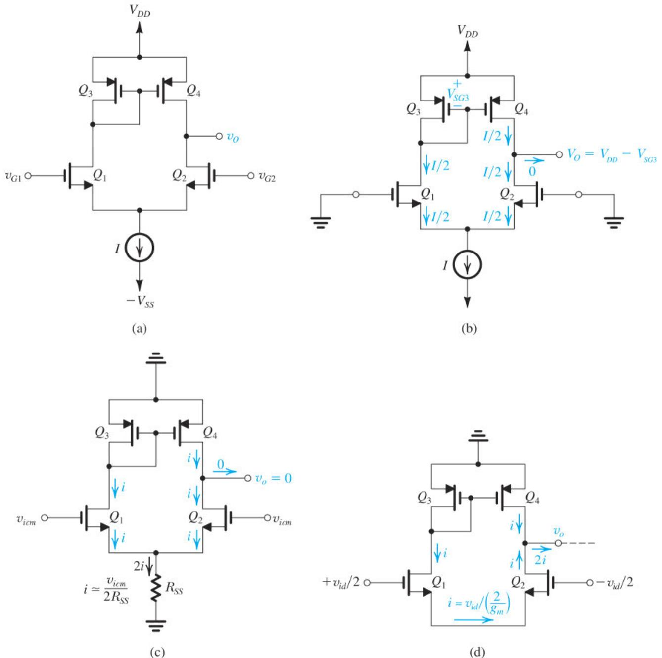
**Figure 9.31** (a) The current-mirror-loaded MOS differential pair. Assuming perfect matching and neglecting the Early effect, in all transistors, we show in (b) the circuit at equilibrium, (c) the circuit with a common-mode input signal  $v_{icm}$ , and (d) the circuit with a differential input signal  $v_{id}$ .
