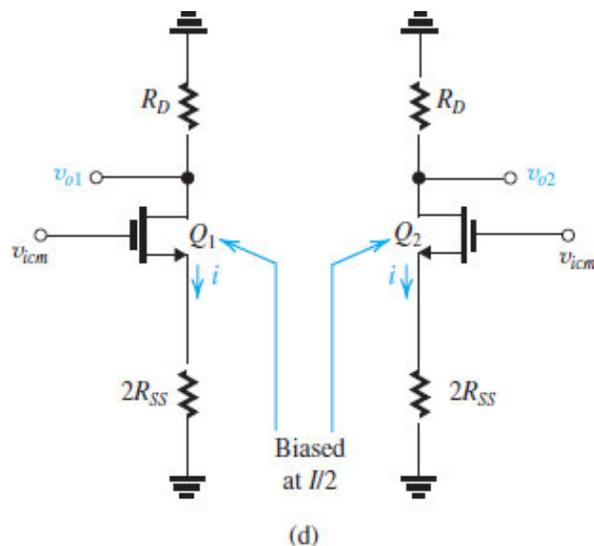
**Figure 9.24 (d)** The circuit in (b) split into its two halves; each half is said to be a “CM half-circuit.”
