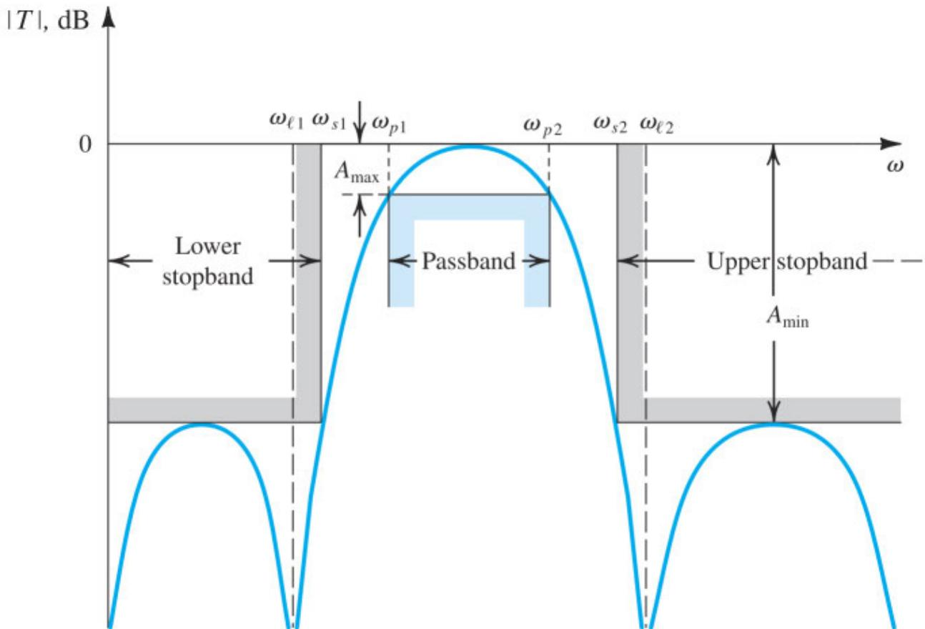
**Figure 14.4** Transmission specifications for a bandpass filter. The magnitude response of a filter that just meets specifications is also shown. Note that this particular filter has a monotonically decreasing transmission in the passband on both sides of the peak frequency.
