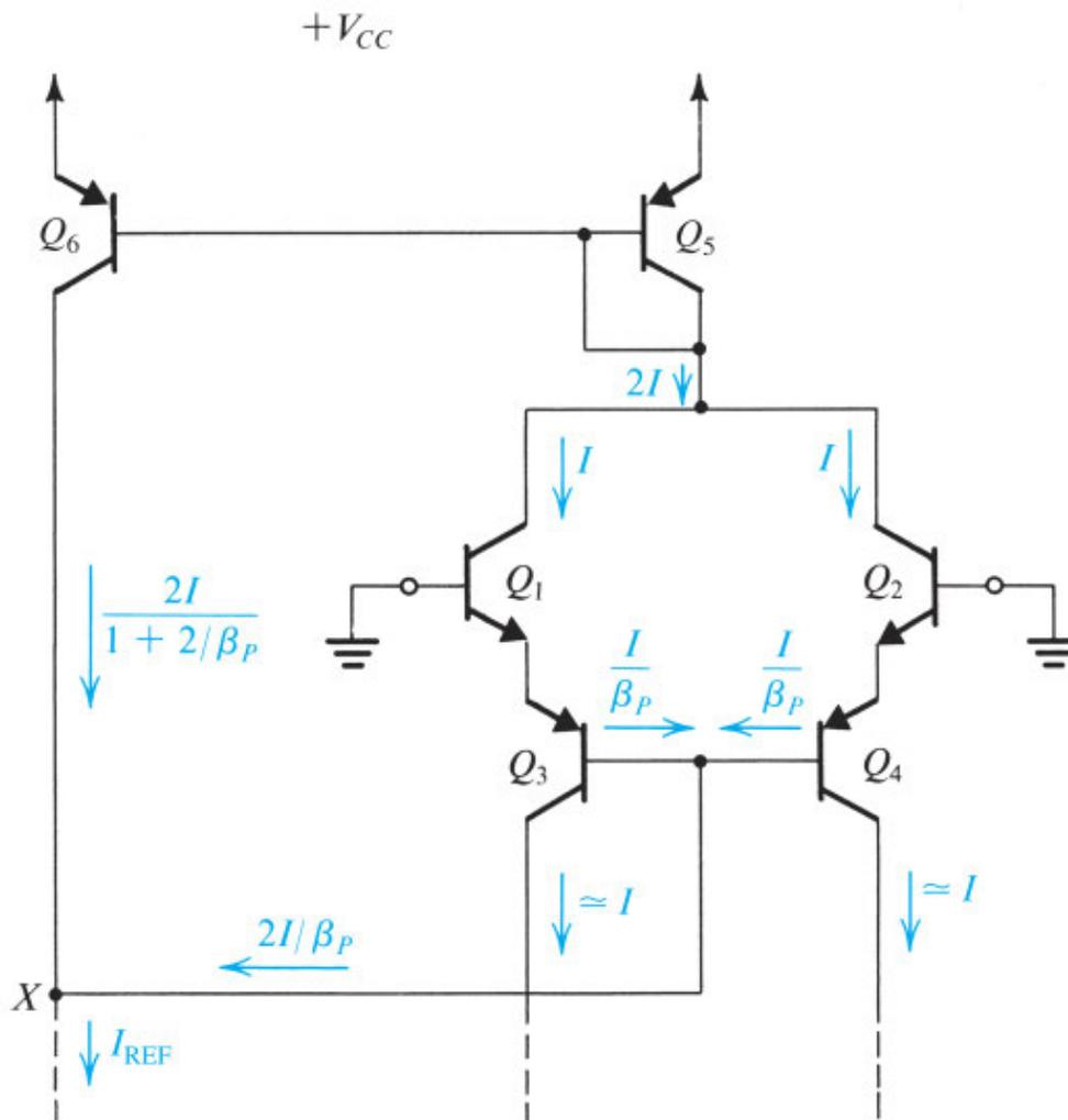
**Figure 13.23** The dc analysis of the 741 input stage.
