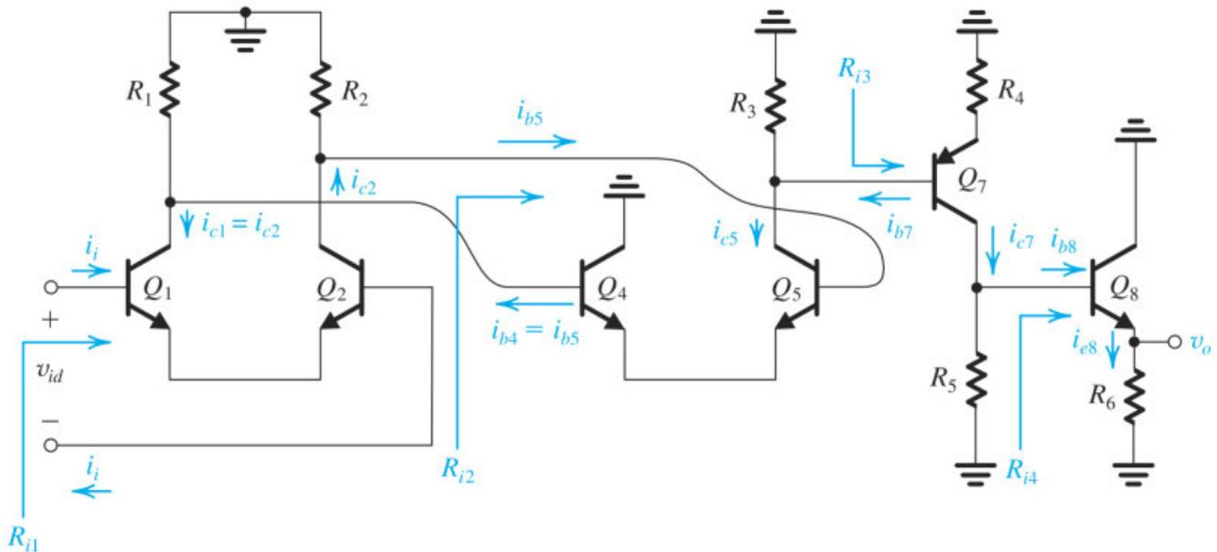
**Figure 9.44** The circuit of the multistage amplifier of [Fig. 9.38](#) prepared for small-signal analysis. Indicated are the signal currents throughout the amplifier and the input resistances of the four stages.
