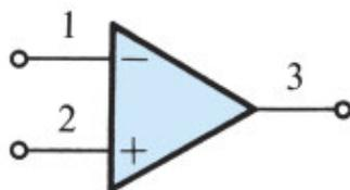
**Figure 2.1** Circuit symbol for the op amp.
