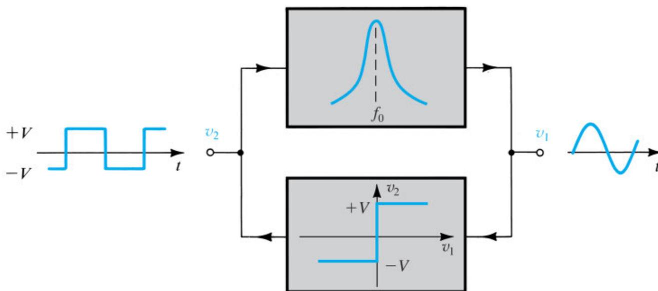
**Figure 15.12** Block diagram of the active-filter-tuned oscillator.
