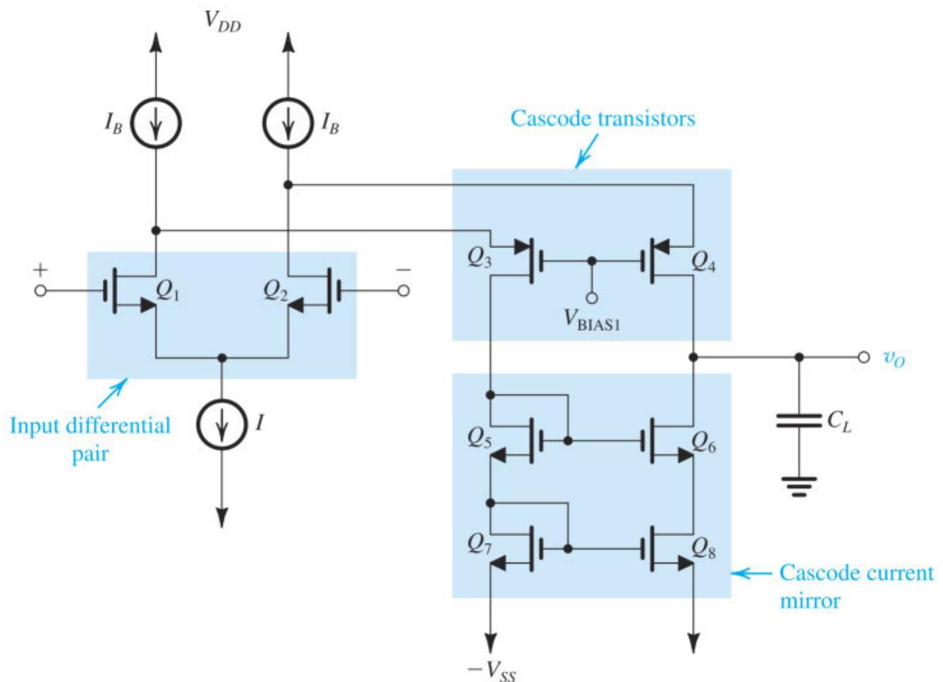
Figure 13.9 Structure of the folded-cascode CMOS op amp.
