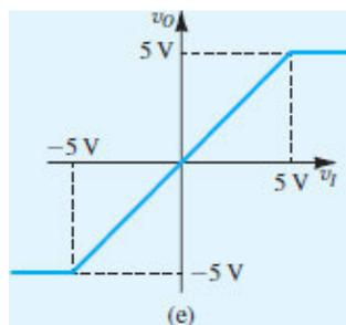
Figure 4.6 (e) The input–output relationship.
