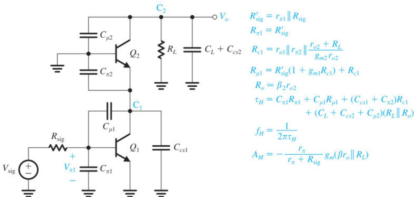
**Figure 10.22** Determining the frequency response of the BJT cascode amplifier. Note that in addition to the BJT capacitances  $C_{\pi}$  and  $C_{\mu}$ , the capacitances between the collector and the substrate  $C_{cs}$  for each transistor are included.
