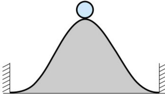
**Figure 15.20** A physical analogy for the operation of the bistable circuit. The ball cannot remain at the top of the hill for any length of time (a state of unstable equilibrium or metastability); the inevitably present disturbance will cause the ball to fall to one side or the other, where it can remain indefinitely (the two stable states).
