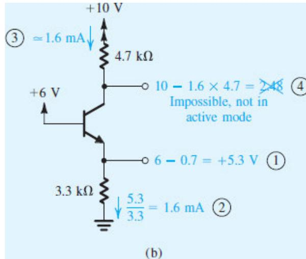
**Figure 6.24 (b)** Analysis of the circuit for Example 6.5. The circled numbers indicate the order of analysis steps.
