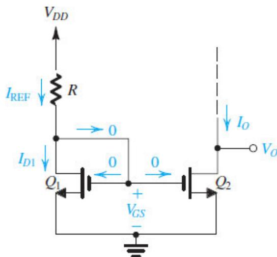
**Figure 8.1** Circuit for a basic MOSFET constant-current source. For proper operation, the output terminal, that is, the drain of  $Q_2$ , must be connected to a circuit that ensures that  $Q_2$  operates in saturation.
