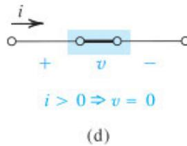
**Figure 4.1 (d)** The ideal diode: equivalent circuit in the forward direction.
