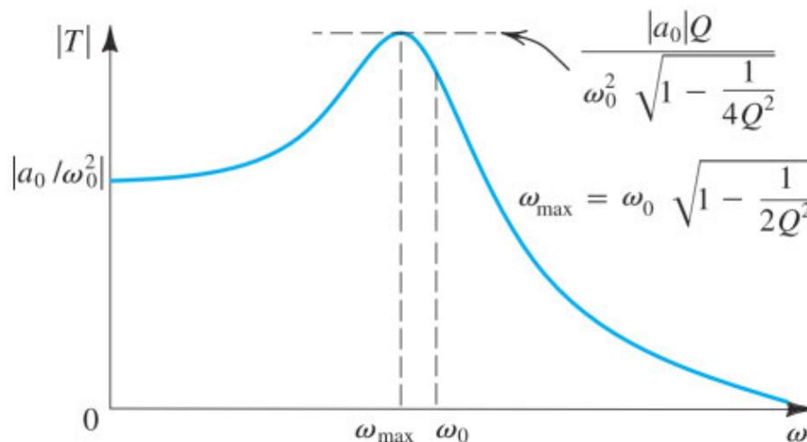
**Figure 14.10** Magnitude response of a second-order low-pass filter.
