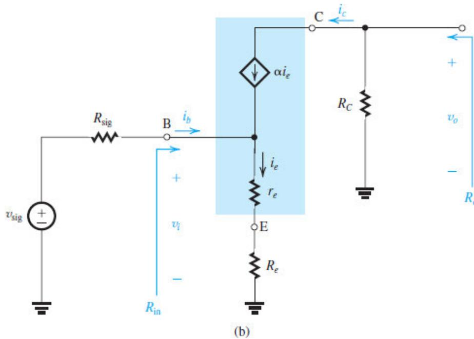
**Figure 7.39 (b)** The CE amplifier with an emitter resistance  $R_e$ : equivalent circuit with the BJT replaced with its T model.
