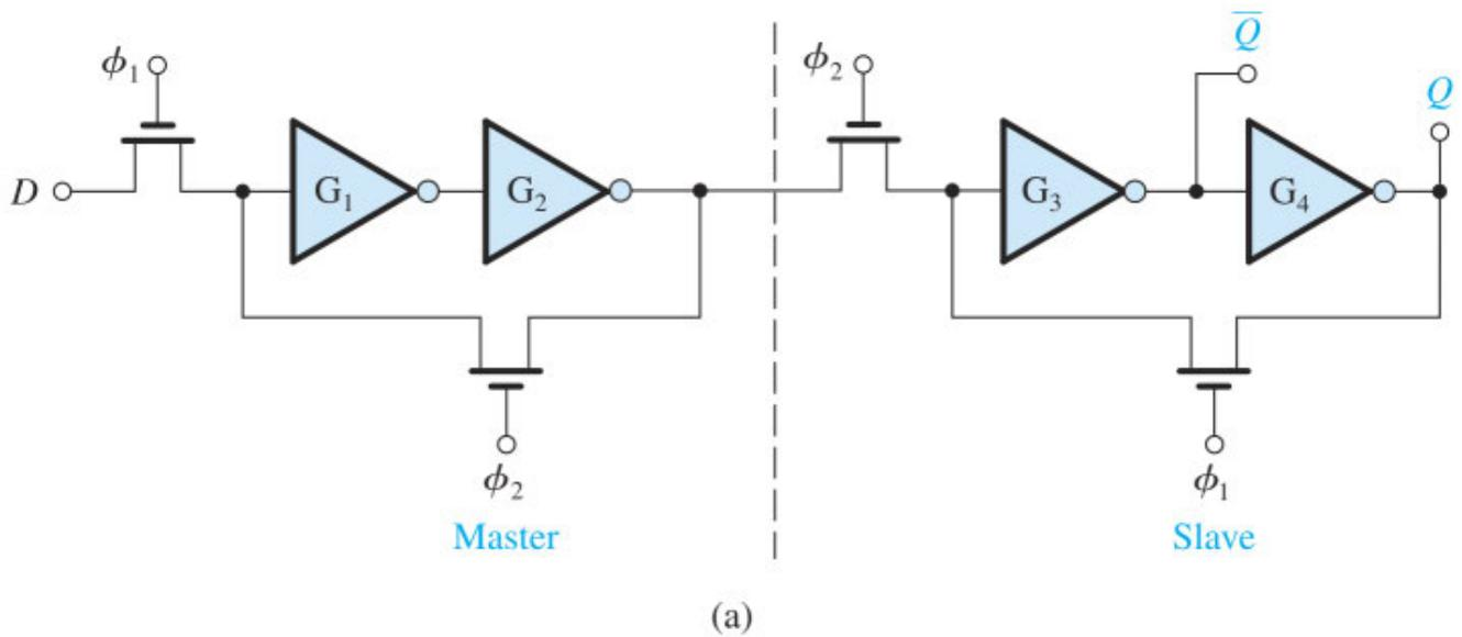
**Figure 18.20 (a)** A master–slave D flip-flop. The switches can be, and usually are, implemented with CMOS transmission gates.
