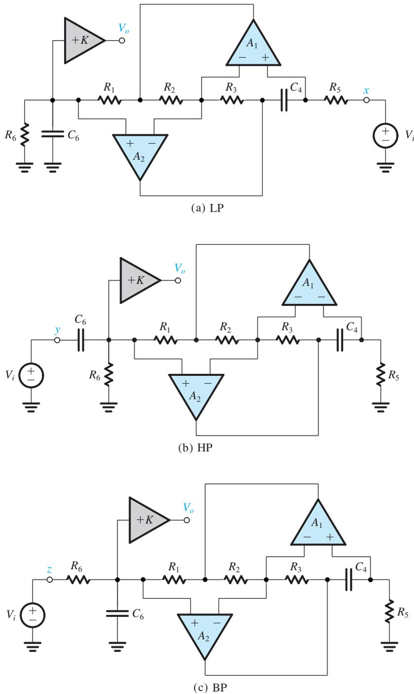
**Figure H.6** Realizations for the various second-order filter functions using the op amp-RC resonator of Fig. 14.21(b): (a) LP, (b) HP, (c) BP. The circuits are based on the LCR circuit in Fig. 14.18. Design considerations are given in Table H.1.
