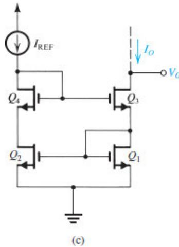
**Figure 8.38 (c)** The Wilson MOS mirror: modified circuit.
