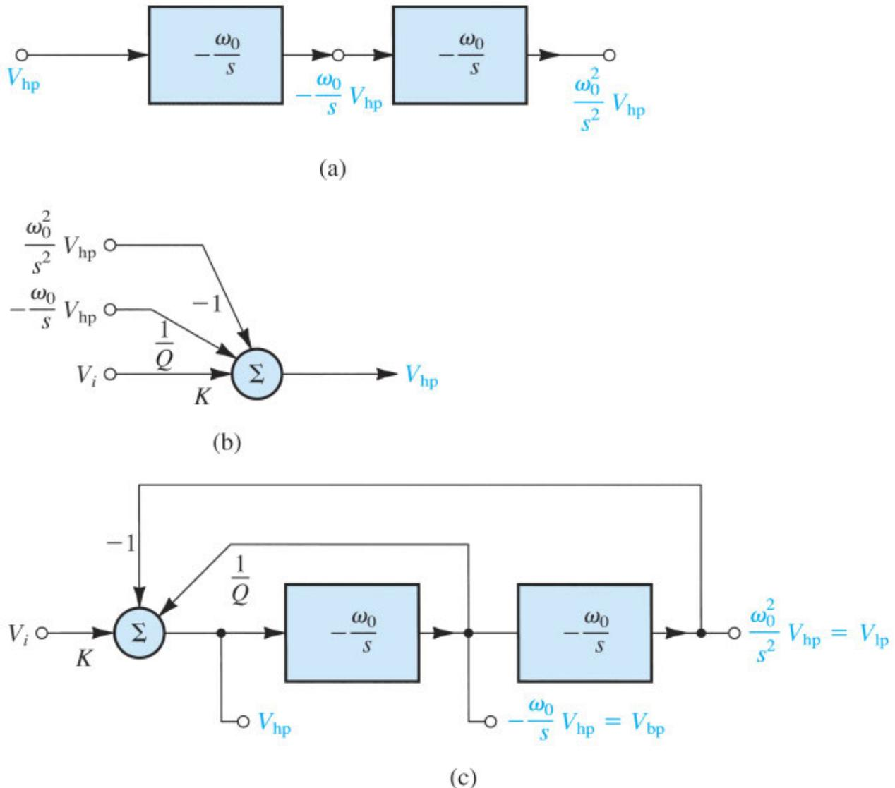
**Figure 14.23** Derivation of a block diagram realization of the two-integrator-loop biquad.
