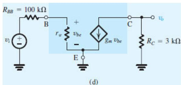
Figure 7.29 (d) Example 7.5: amplifier circuit with the transistor replaced by its hybrid- $\pi$ , small-signal model.
