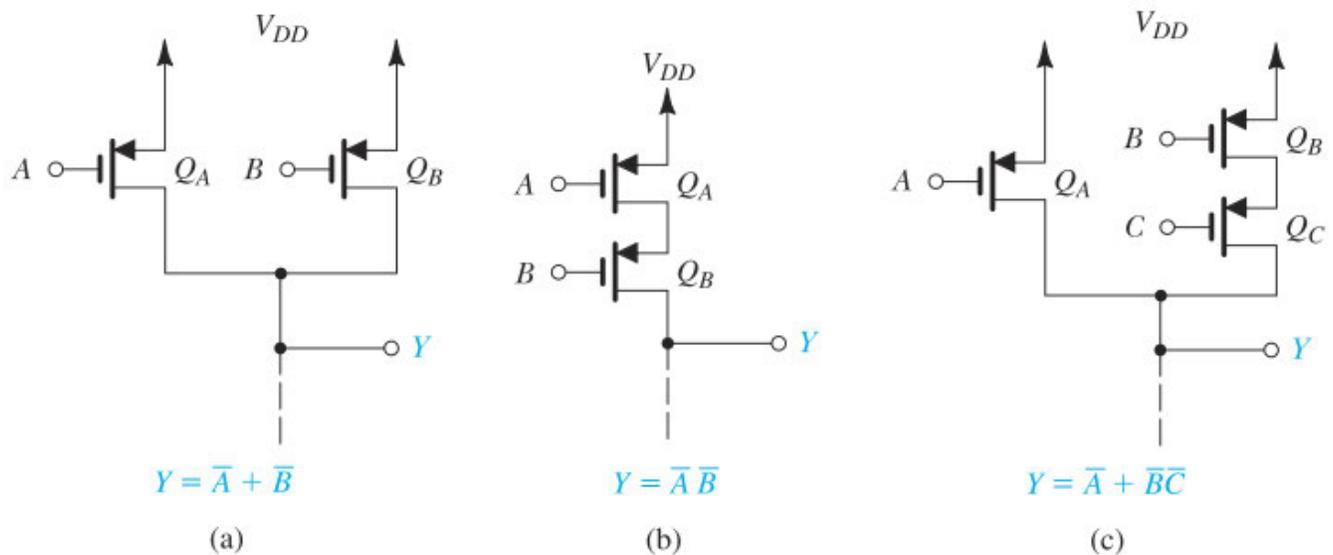
**Figure 16.5** Examples of pull-up networks.
