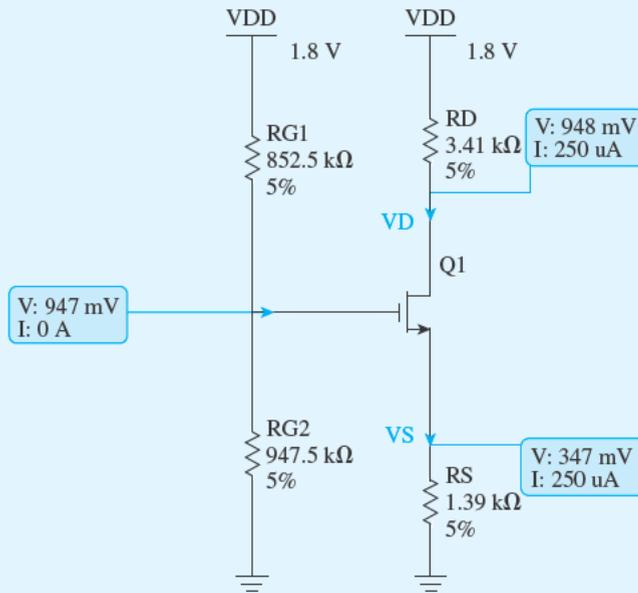
**Figure B.24** DC bias-point analysis of the CS amplifier.
