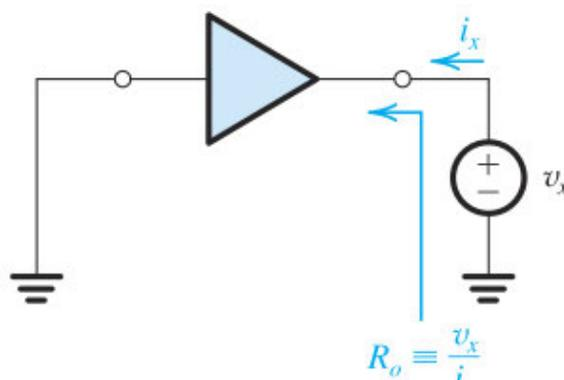
Figure 1.18 Determining the output resistance.
