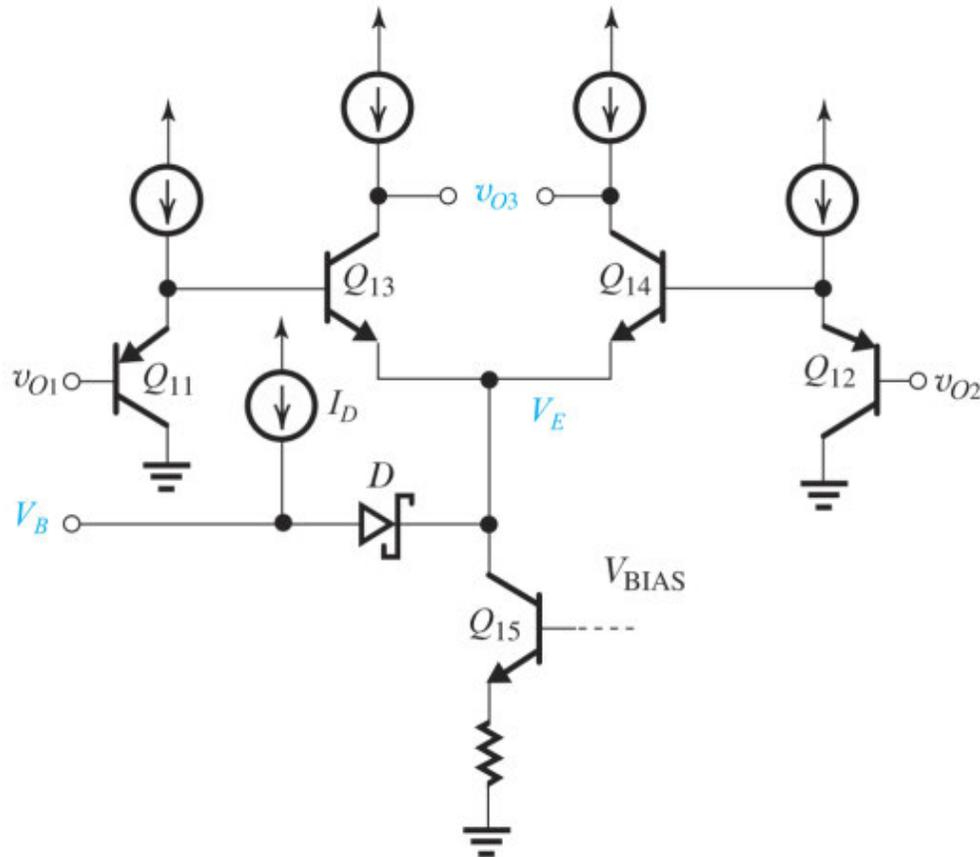
**Figure 13.21** An op-amp second stage incorporating the common-mode feedback circuit for the input stage. Note that the circuit generates the voltage  $V_B$  needed to bias the cascode circuit in the first stage. Diode  $D$  is a Schottky-barrier diode, which exhibits a forward voltage drop of about 0.4 V.
