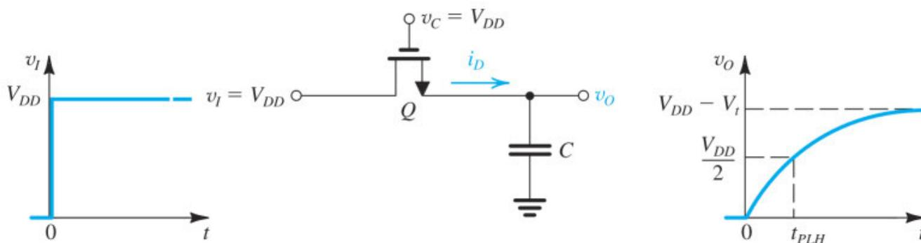
**Figure 18.3** Operation of the NMOS transistor as a switch in the implementation of PTL circuits. This analysis is for the case with the switch closed ( $v_C$  is high) and the input going high ( $v_I = V_{DD}$ ).
