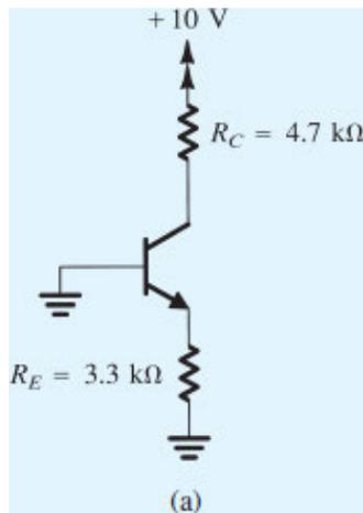
**Figure 6.25 (a)** Example 6.6: circuit.
