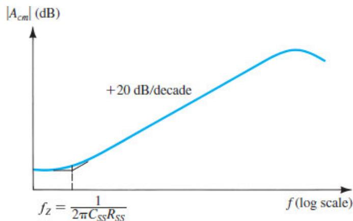
**Figure 10.27 (a)** Common-mode gain with frequency.
