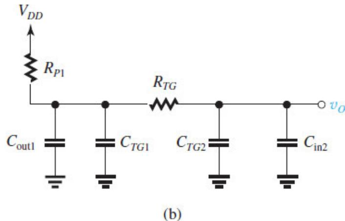
Figure 18.9 (b) Equivalent circuit for the purpose of analyzing the propagation delay of the circuit in (a).
