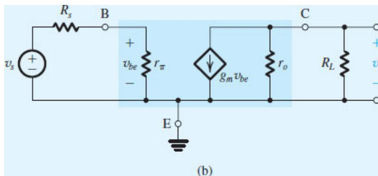
**Figure 1.19 (b)** The BJT connected as an amplifier with the emitter as a common terminal between input and output (called a common-emitter amplifier).
