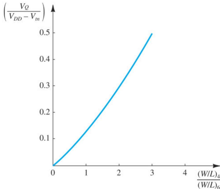
**Figure 18.27** The normalized value of  $V_Q$  versus the ratio  $(W/L)_4/(W/L)_6$  for the circuit in Fig. 18.26(b). The graph applies for process technologies for which  $\mu_n \simeq 4\mu_p$ . It can be used to determine the maximum  $(W/L)_4/(W/L)_6$  for which  $V_Q$  is guaranteed to fall below a desired value.
