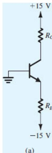
**Figure 6.15 (a)** Circuit for Example 6.2.
