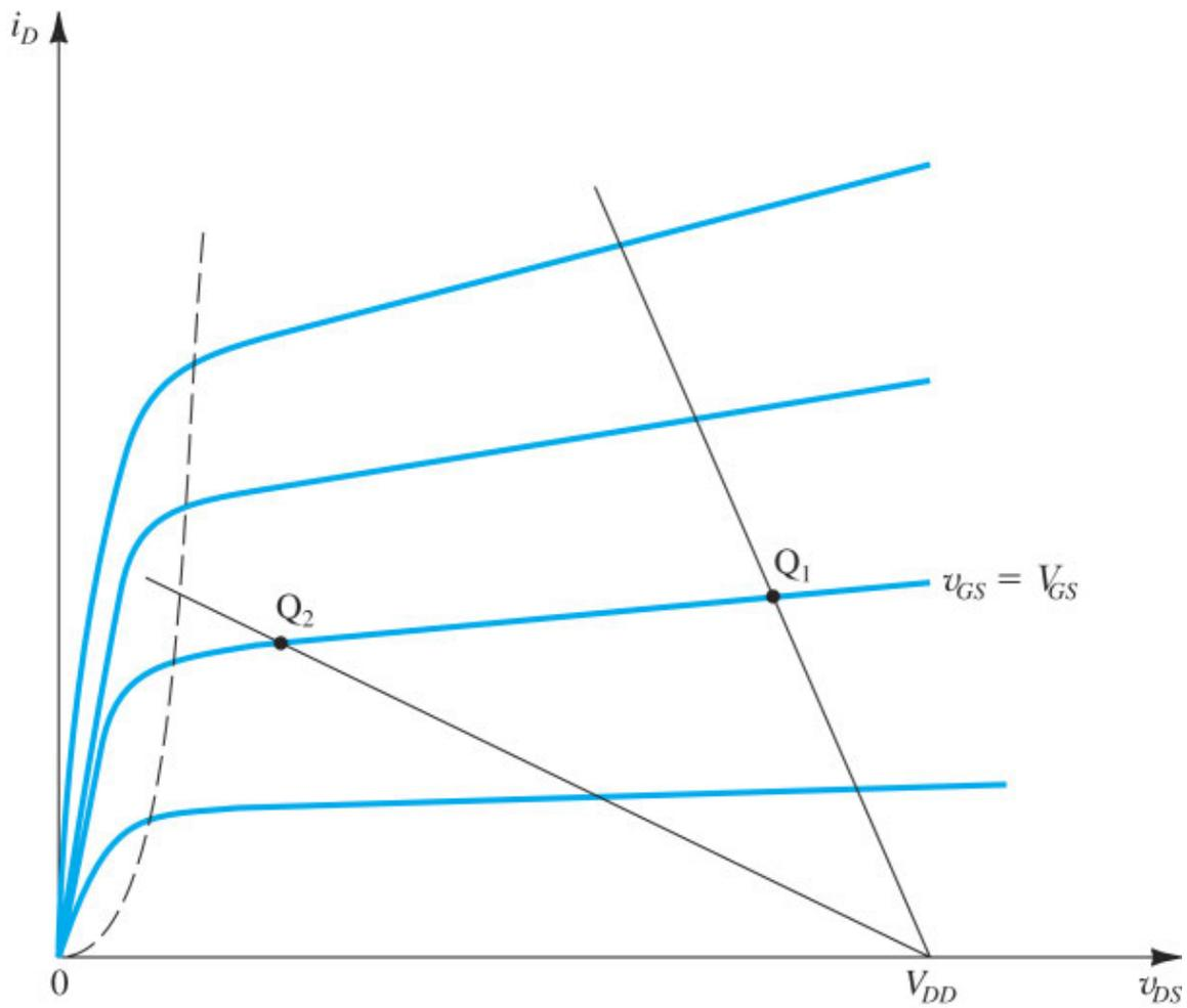
**Figure 7.9** Two load lines and corresponding bias points. Bias point  $Q_1$  does not leave sufficient room for positive signal swing at the drain (too close to  $V_{DD}$ ). Bias point  $Q_2$  is too close to the boundary of the triode region and might not allow for sufficient negative signal swing.
