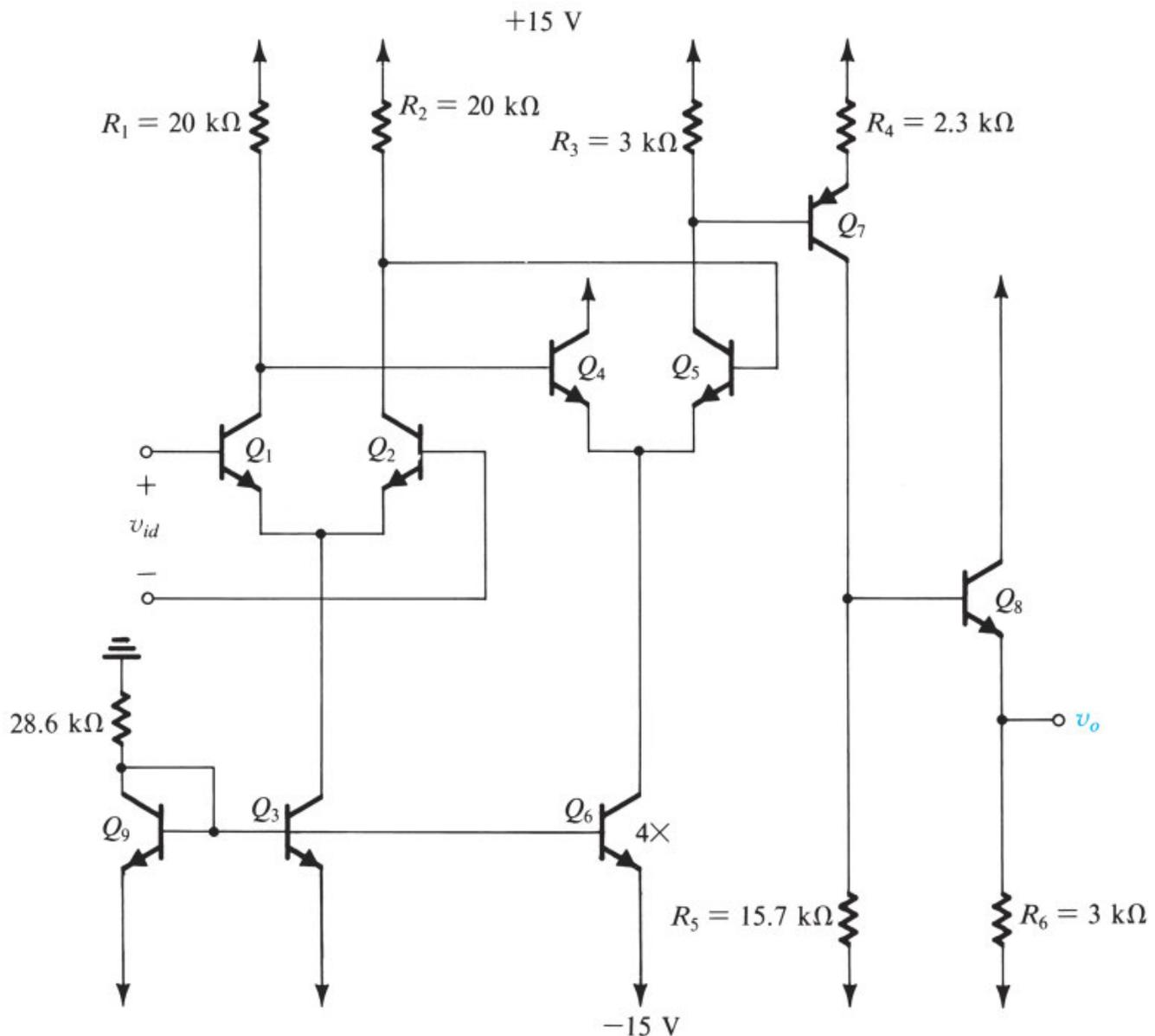
**Figure 9.38** A four-stage bipolar op amp.
