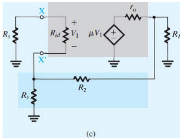
**Figure 11.13 (c)** The feedback loop obtained by setting  $V_s = 0$  and replacing the op amp with its equivalent-circuit model.
