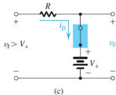
**Figure 4.5 (c)** When  $v_I > V_+$ , the diode turns on limiting  $v_O$  to  $V_+$ .
