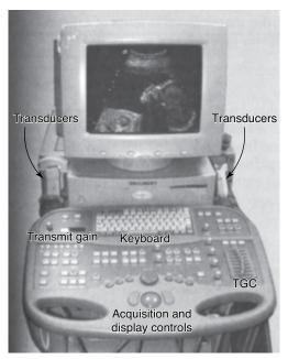
Figure 11.10 • A portable ultrasound system. (Reprinted with permission from Bushberg, J. T., et al.: The Essential Physics of Medical Imaging, 2nd ed. Philadelphia: Lippincott Williams and Wilkins, 2002.)
