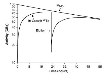
Figure 11.2 • Time-activity curve of a molybdenum-99/technetium-99m generator system demonstrating the in-growth of technetium-99m and subsequent elution. (Reprinted with permission from Bushberg, J. T., et al.: The Essential Physics of Medical Imaging, 2nd ed. Philadelphia: Lippincott Williams and Wilkins, 2002.)
