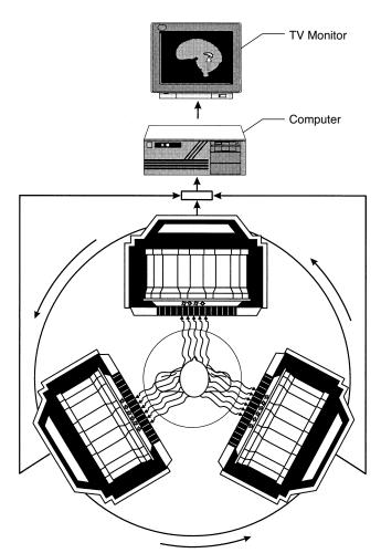
Figure 11.4 • Schematic diagram of a rotating tripledetector scintillation camera system for single photon emission computed tomography (SPECT).
