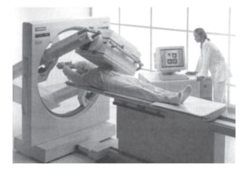
Figure 11.3 • Patient being imaged with a scintillation (Anger) camera. (Reprinted with permission from Bushberg, J. T., et al.: The Essential Physics of Medical Imaging, 2nd ed. Philadelphia: Lippincott Williams and Wilkins, 2002.)
