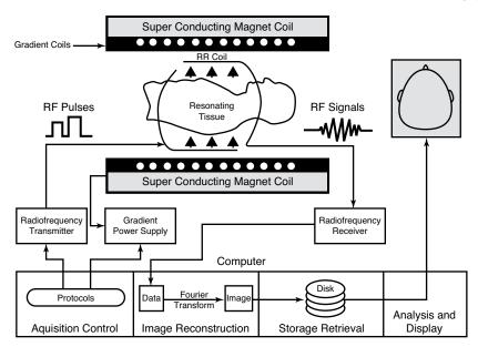
Figure 11.9 • Schematic diagram of an MRI system demonstrating radiofrequency pulses and the strong magnetic field.
