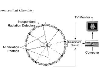
**Figure 11.5** • Schematic diagram of a PET imaging system with multiple scintillation detectors that localize positron decay by coincident detection of annihilation photons.
