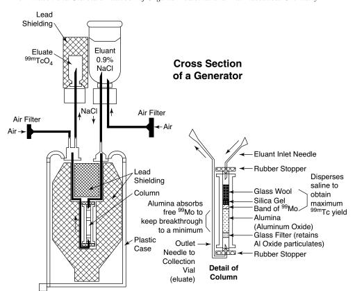
Figure 11.1 • Crosssectional diagram of a molybdenum-99/technetium-99m generator. (Reprinted with permission from Bushberg, J. T., et al.: The Essential Physics of Medical Imaging, 2nd ed. Philadelphia: Lippincott Williams and Wilkins, 2002.)
