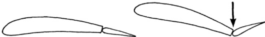
Figure 14. An aileron applies large vertical loads near the trailing edge of a wing and well aft of the wing's flexural centre. It therefore tends to twist the wing in such a way as to provide aerodynamic forces which are the opposite of those desired by the pilot.
